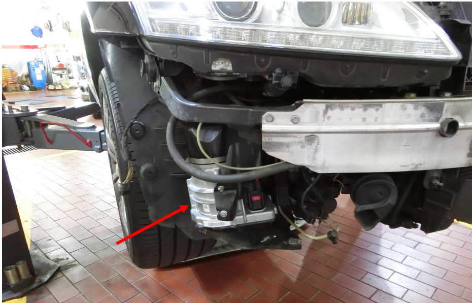
Photo 12 shows the power steering pump of the Insured Vehicle, which was found to be newly replaced during initial investigations by AIG in-house surveyor and Cycle & Carriage Industries Pte Ltd (photograph provided to me).
