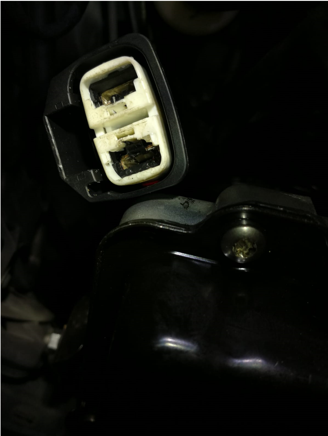
Photo 14 shows the wiring socket of the power steering pump that was found to be slightly melted with burn marks during initial investigations by AIG in-house surveyor and Cycle & Carriage Industries Pte Ltd (photograph provided to me).
