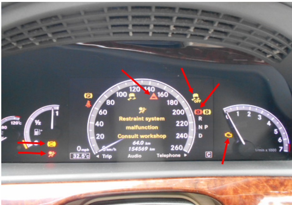
Photo 10 shows the various warning messages (arrowed) appearing on the instrument panel of the Insured Vehicle. This was after about 1min to 2mins upon starting the engine of the Insured Vehicle.
