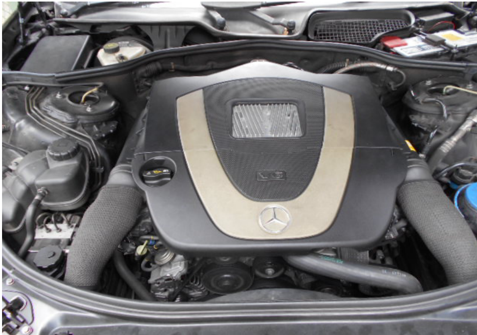
Photo 9 shows a general view of the Insured Vehicle's engine compartment. I did not find any burn mark(s) within the engine compartment of the Insured Vehicle.
