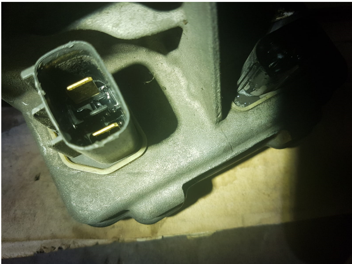
Photo 13 shows the connector for the wiring socket of the power steering pump with water trapped at the bottom of the connector (photograph provided to me).
