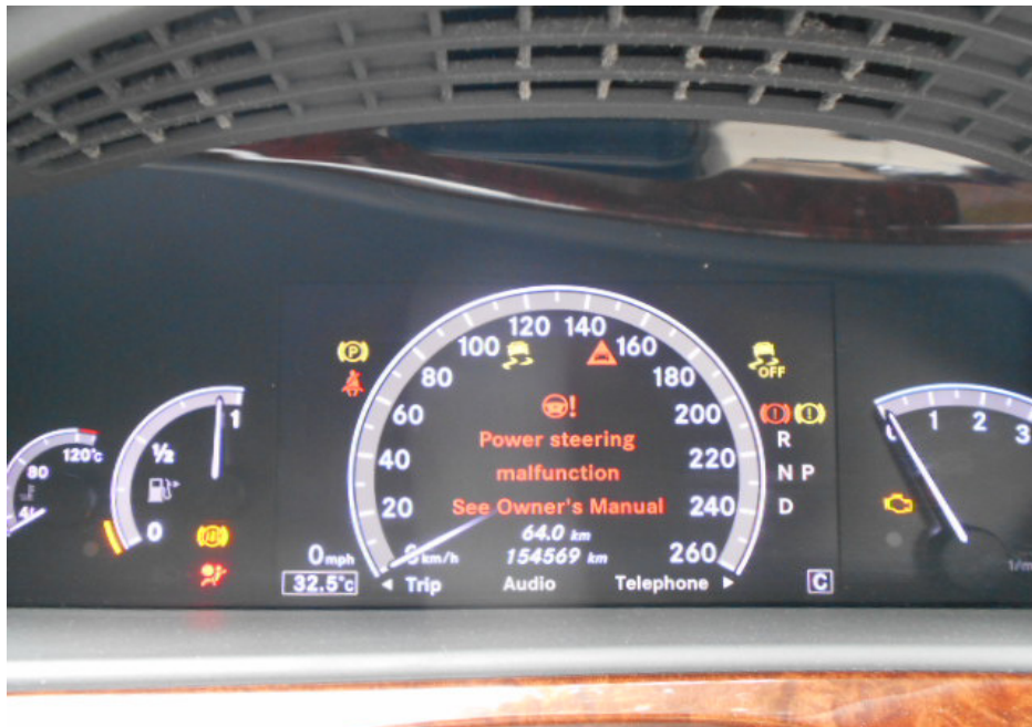
Photo 11 shows the “power steering malfunction” warning message appearing on the instrument panel of the Insured Vehicle. This was after about 1min to 2mins upon starting the engine of the Insured Vehicle.
