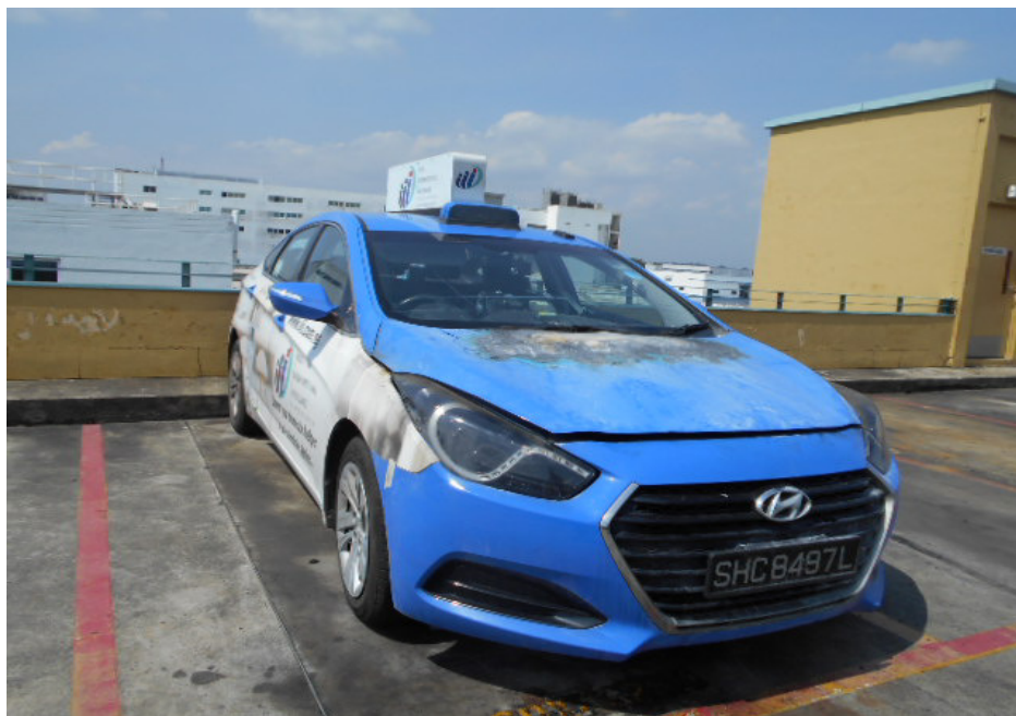
Photo 1 shows a general view of the front right body of the Insured Vehicle at the time of my inspection. The fire damage was confined to the engine compartment of the Insured Vehicle. Exteriorly, only the front bonnet and front windscreen were affected by the incident. The interior compartment and the rear portion of the Insured Vehicle were unaffected.
