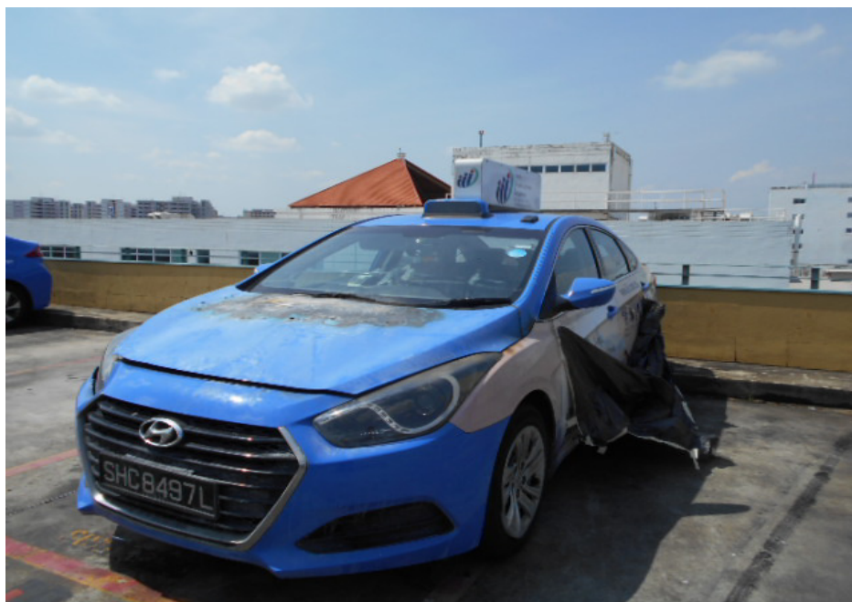
Photo 2 shows a general view of the front left body of the Insured Vehicle at the time of my inspection. The fire damage was confined to the engine compartment of the Insured Vehicle. Exteriorly, only the front bonnet and front windscreen were affected by the incident. The mileage of the Insured Vehicle could not be recorded due to its wirings being affected by the fire.
