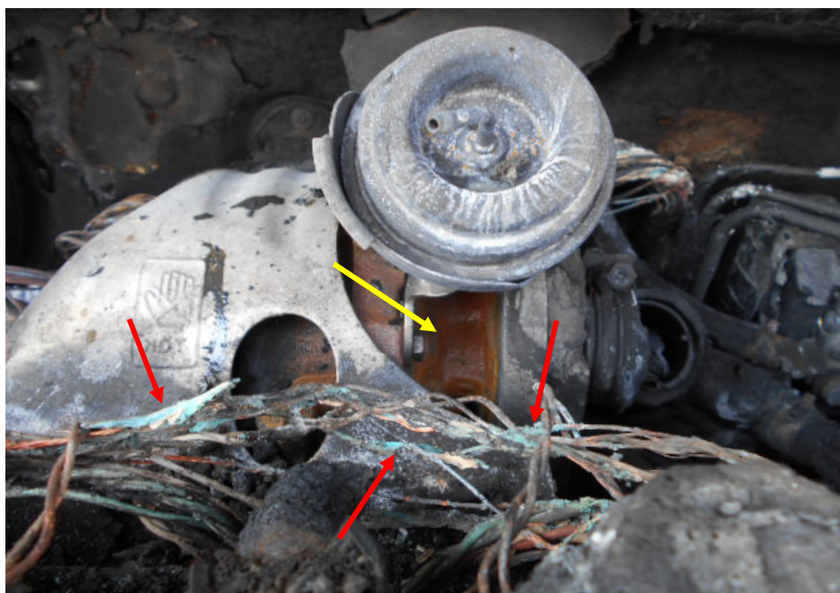
Photo 8 shows a closer view of the original factory fitted wirings with greenish residue (red arrow) and bright red colour of the turbocharger housing (yellow arrow). The presence of greenish residue suggests occurrence of an electrical short circuit while the bright red colour of the turbocharger housing indicates that the turbocharger had overheated (unable to cool down sufficiently).
