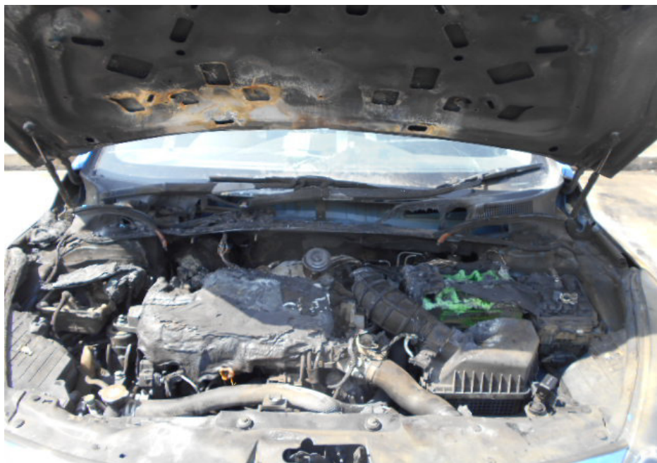
Photo 3 shows a general view of the Insured Vehicle's engine compartment at the time of my inspection. Most of the parts and components within the engine compartment were burnt and/or melted. This had included various rubber hoses, wiper panel, battery, air intake duct, bonnet insulator, brake fluid reservoir, cooling fan, radiator, intake manifold and alternator amongst others.
