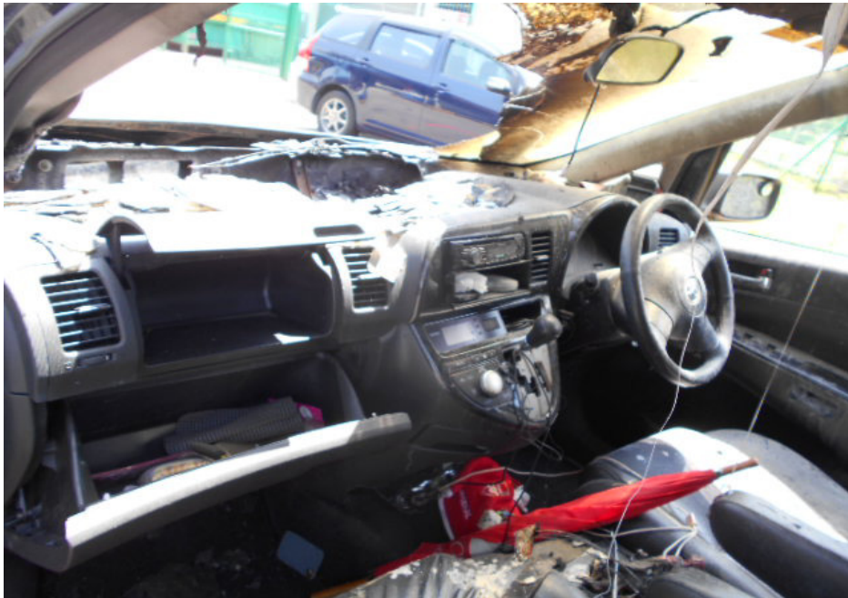
Photo 4 shows the interior compartment of the Insured Vehicle, which was observed to be partially burnt and/or melted at the front area. The front dashboard, various trims and roof upholstery were amongst the parts that were burnt and/or melted as a result of the fire.
