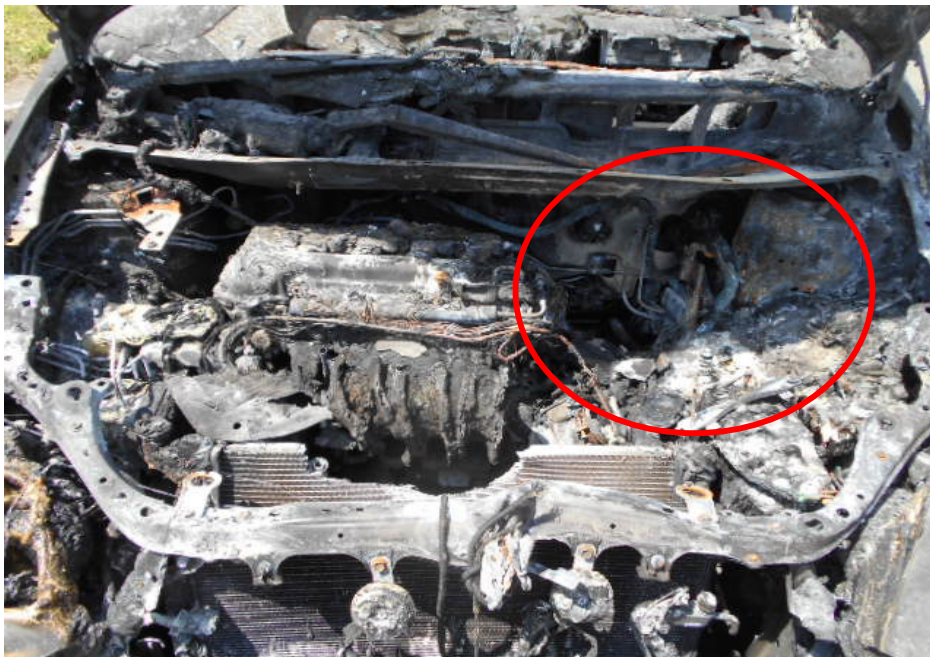
Photo 9 shows a general view of where the fire to the Insured Vehicle had originated, which was around the rear left area of the engine compartment (circled). This was established basing on the burn pattern (whitish burn marks and rust) that was formed on the Insured Vehicle's front bonnet.
