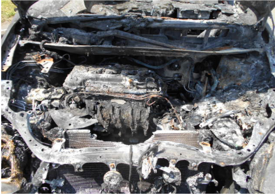
Photo 3 shows the engine compartment of the Insured Vehicle at the time of my inspection. The entire engine compartment of the Insured Vehicle was observed to be severely burnt. Most of the parts inside the engine compartment were burnt and/or melted as a result of the fire. This include the radiator, air intake manifold, fuse box, various rubber hoses and pipes amongst others.
