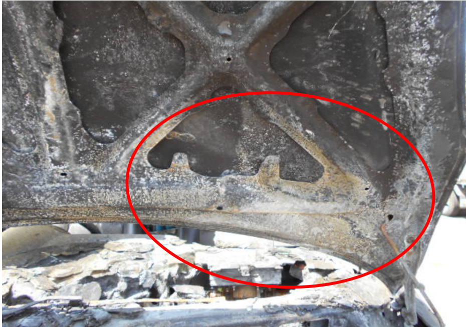
Photo 8 shows the whitish burn marks and rust that had developed (circled) on the underside of the front bonnet, directly under the area where similar whitish burn marks were formed. These whitish burn marks are a result of exposure to prolong heat intensity and can typically be used to determine the origin of fire.
