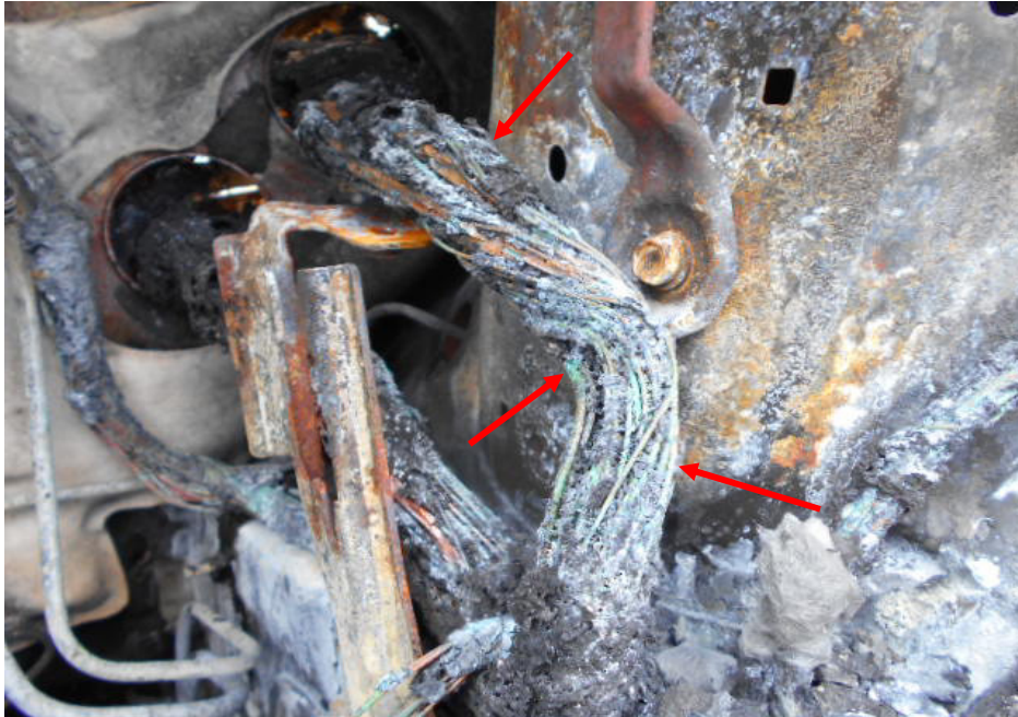
Photo 11 shows a closer view the wirings at the rear left area of the Insured Vehicle's engine compartment that were found with greenish residue (arrowed) The presence of such greenish residue suggests occurrence of an electrical short circuit.
