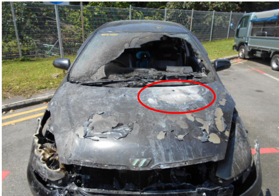
Photo 7 shows the whitish burn marks (circled) that were formed on the rear left area of the Insured Vehicle's front bonnet. Such whitish burn marks are a result of exposure to prolong heat intensity. Following the characteristic of heat rising upwards, the fire to the Insured Vehicle can then be determined to have originated around the rear left area of the engine compartment.
