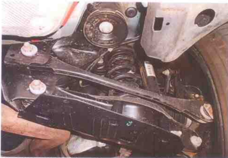
Photo 9 shows a general view of the control arms and linkages at the rear right wheel of the Motor Car. I did not observe any fluid leak and/or fluid stain on the underside of the Motor Car. All of the Motor Car's undercarriage components were observed to be intact and secured in an appropriate manner.
