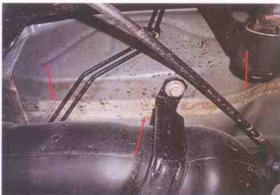
Photo 13 shows the structural body at the underside left centre of the Motor Car. Visually, I did not find any weld marks other than original spot weld marks on the chassis body of the Motor Car. The original factory sealant (arrowed) at the joints along the chassis body was also untouched, indicating no work was done on the chassis body of the Motor Car and that the chassis body was originally fitted.
