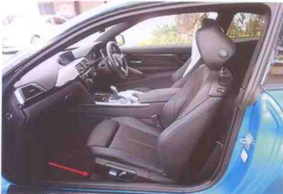
Photo 5 shows the front seats of the Motor Car, which were secured via seat rails (arrowed) to the floor board. All the seats of the Motor Car were fitted with a retractable seat belt reel and pre-tensioner. The seat belts were also able to be fastened to the pretension that were fitted on the side of each individual seat.
