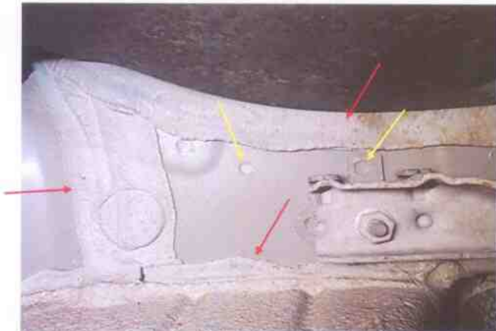
Photo 15 shows the structural body at the rear centre of the Motor Car. Visually, I did not find any weld marks other than original spot weld marks (yellow arrow) on the chassis body of the Motor Car. The original factory sealant (red arrow) at the joints along the chassis body was also untouched, indicating no work was done on the chassis body of the Motor Car and that the chassis body was originally fitted.
