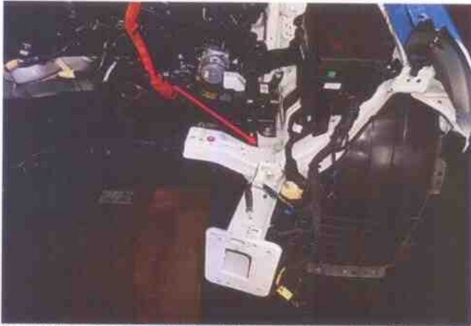
Photo 5 shows a top view of the front left chassis of the motor taxi. The front left chassis was bent towards the right. The centre section (arrowed) of the front left chassis was found to be bent.
