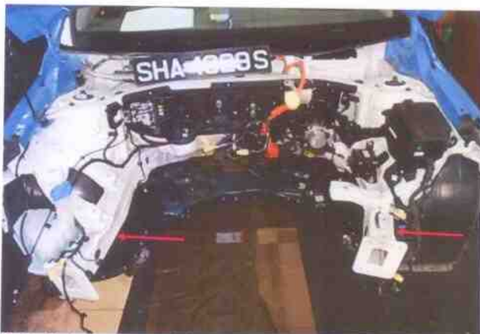
Photo 2 shows a general view of the motor taxi's front chassis. Upon examination of the front chassis, I had observed that the left and right front chassis (arrowed) were both bent towards the right, indicating an impact force that was from a left to right direction, at the frontal portion of the motor taxi.
