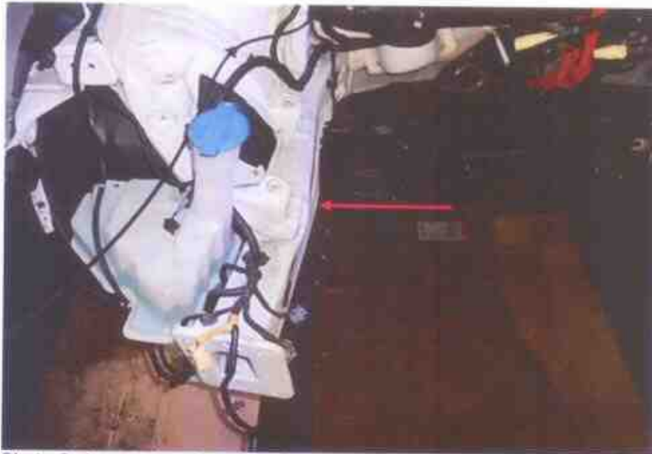
Photo 3 shows a top view of the front right chassis of the motor taxi. The front right chassis was bent towards the right. The centre section (arrowed) of the front right chassis was found to be bent.
