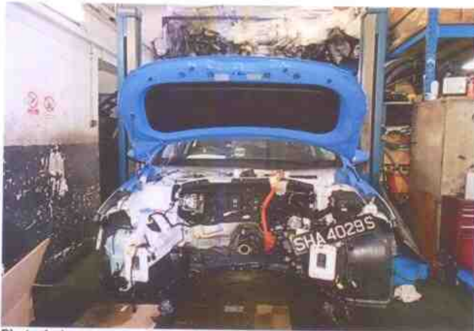
Photo 1 shows a general view of the motor taxi SHA 4029S. Parts at the frontal portion of the motor taxi were removed prior to my inspection. This had included all wiring harness, the engine and the transmission. As a result, the front chassis of the motor taxi was visible
