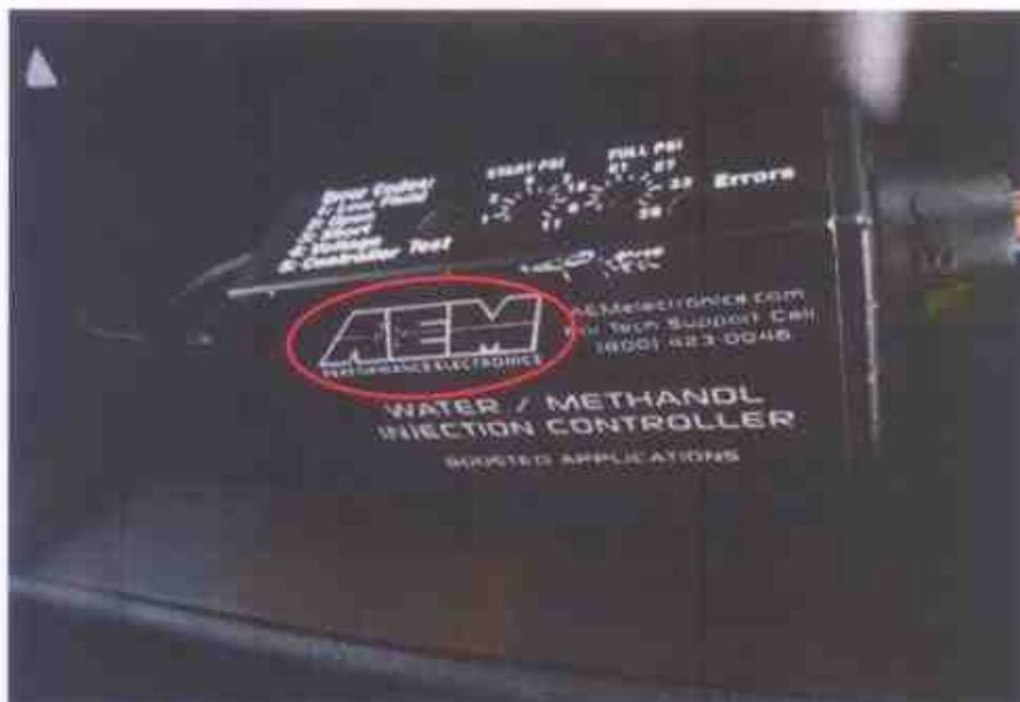
Photo 16 shows a close up view of the controller for the water injection system that was found to be additionally fitted under the steering wheel of the Insured Vehicle upon our inspection. The brand of the controller was 'AEM' (circled).
