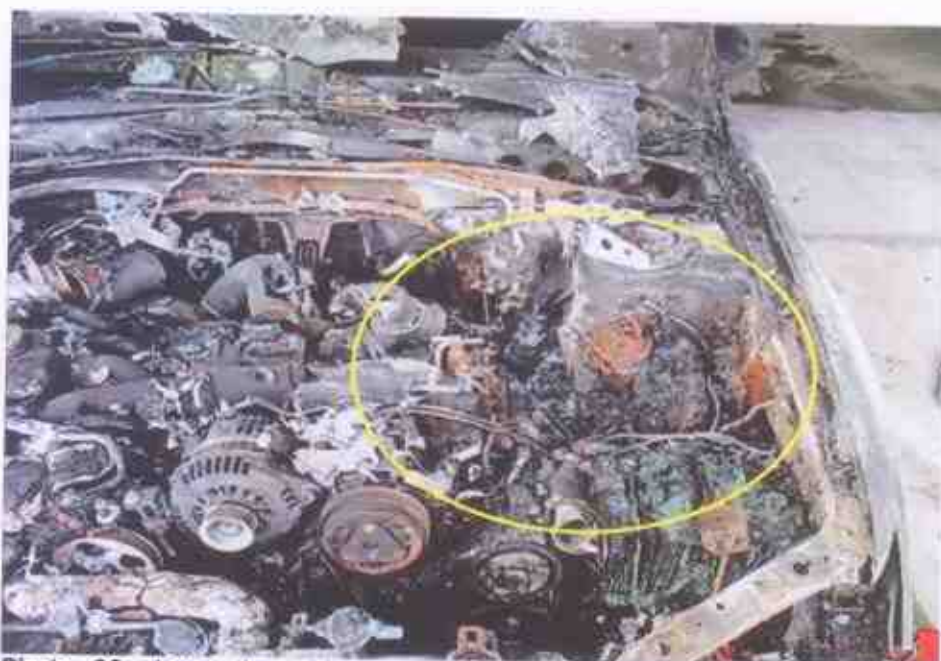
Photo 36 shows the wirings around the left rear portion of the engine compartment which is near to the vicinity where the fire to the Insured Vehicle had likely started. We observed greenish residue on the wirings at the left rear portion of the engine compartment (circled). The presence of greenish residue indicates internal heating of copper wires, a sign of an electrical short circuit occurring. The greenish residue is normally left behind from oxidation as a result of chemical reaction involving the copper wires.
