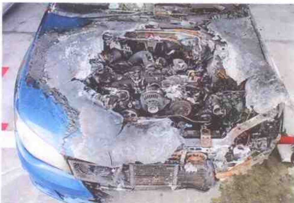
Photo 8 shows a general view of the engine compartment of the Insured Vehicle at the time of our inspection. Most of the components inside the engine compartment were found to be severely burnt and/or melted as a result of the fire.
