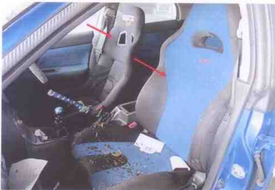
Photo 10 shows the aftermarket front seats (red arrows) that were fitted onto the Insured Vehicle upon our inspection.
