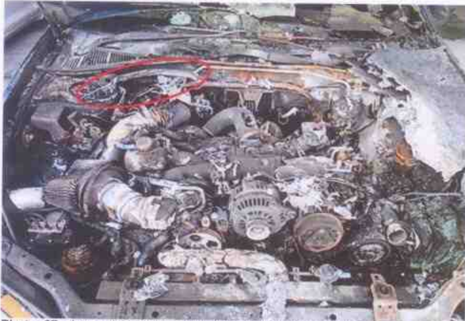
Photo 27 shows the engine strut bar (circled) fitted on the Insured Vehicle. However it had sustained serious fire damage.
