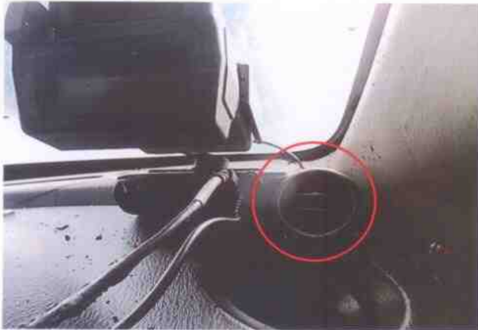
Photo 18 shows the 1st aftermarket twitter fitted onto the right corner of the dashboard of the Insured Vehicle upon our inspection which had sustained minor fire damage (circled).
