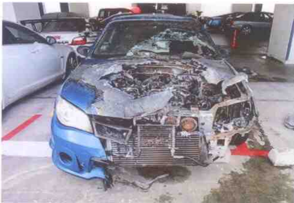
Photo 2 shows the general view of the front portion of the Insured Vehicle at the time of our inspection. The exterior body of the Insured Vehicle had sustained visible fire damage. This included its front windscreen, front bonnet, headlights, front bumper, side panels, front rims and front tires.
