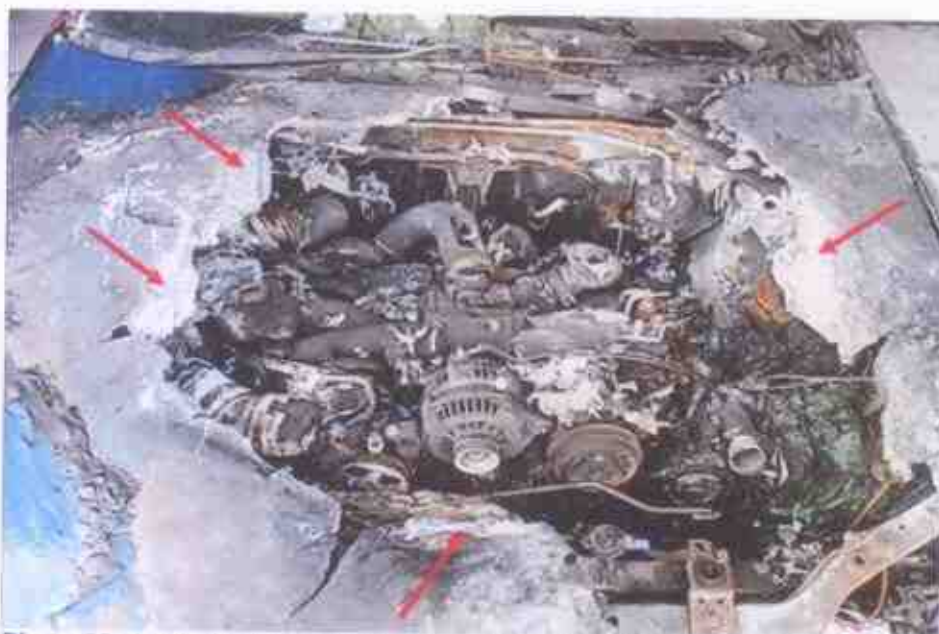
Photo 32 shows the hole found in the front bonnet of the Insured Vehicle which indicates that the front portion of the Insured Vehicle was exposed to prolonged high heat intensity. The whitish burn marks (arrowed) are a result of exposure to prolonged heat intensity.
