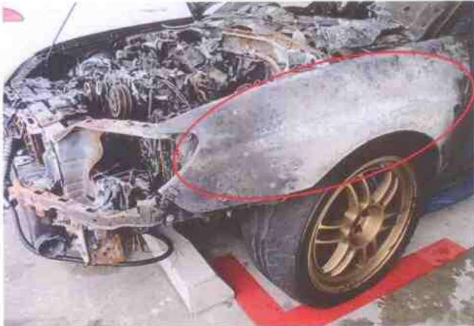
Photo 34 shows the whitish burn marks that were found on the left front fender of the Insured Vehicle (circled). Such whitish burn marks are a result of exposure to prolonged heat intensity, which may indicate where the fire had started. Rust would also begin to develop on these areas soon after the fire.
