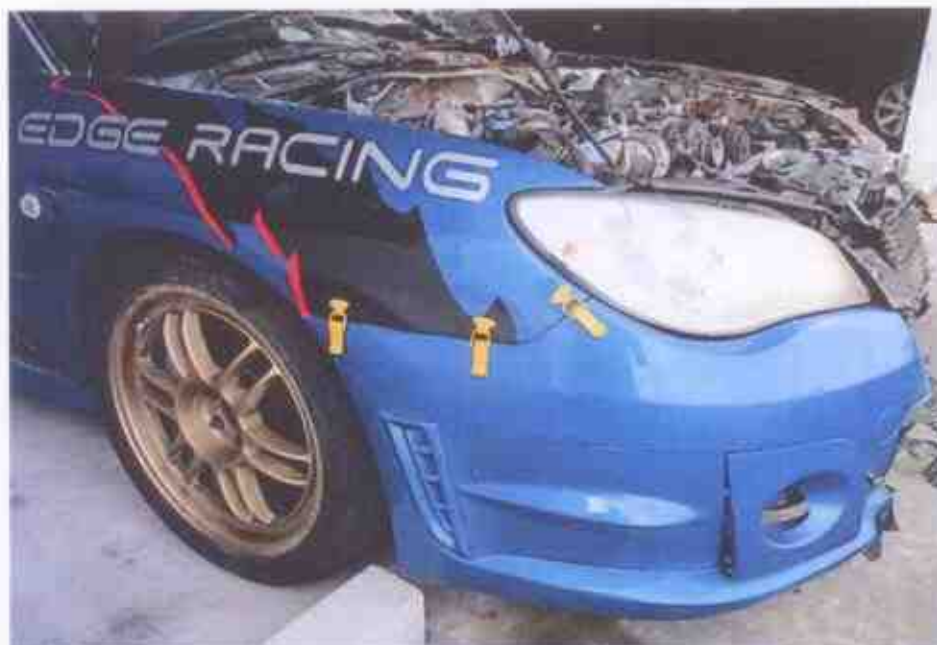
Photo 35 shows the right front fender of the Insured Vehicle which had sustained minimal fire damage.
