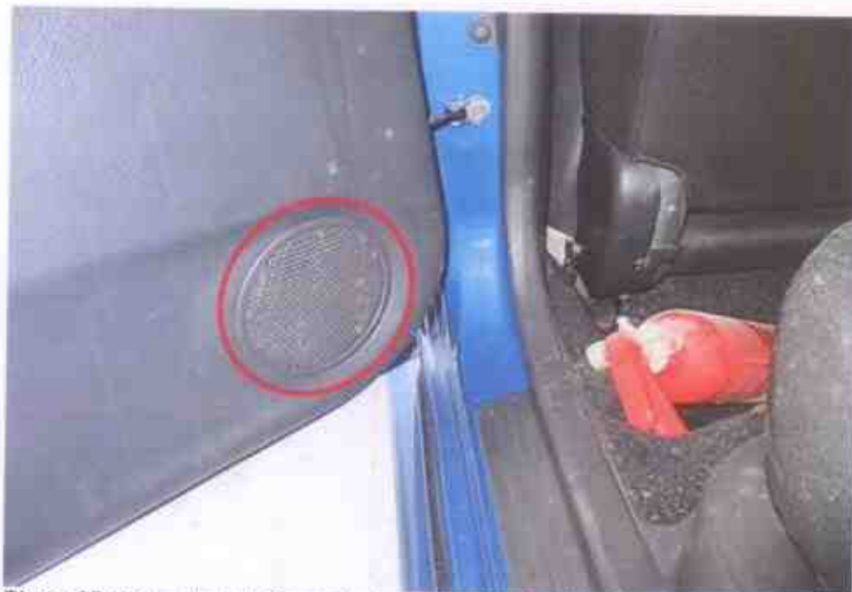
Photo 25 shows the 3rd aftermarket speaker fitted at the left rear passenger door panel (circled).
