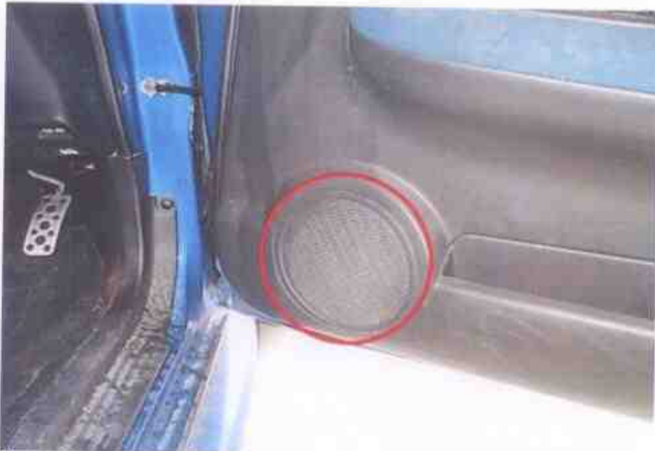
Photo 24 shows the 2nd aftermarket speaker fitted at the driver door panel (circled).
