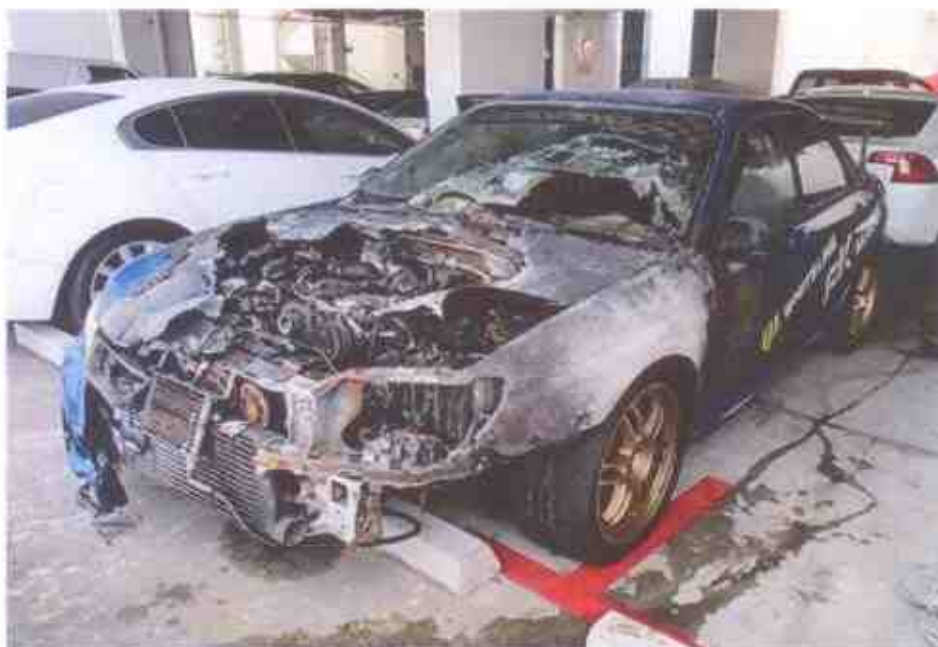
Photo 3 shows the general view of the left portion of the Insured Vehicle at the time of our inspection. The exterior body of the Insured Vehicle had sustained visible fire damage. This included its front windscreen, front bonnet, left headlight, front bumper, left side panel, left front rim and left front tire.
