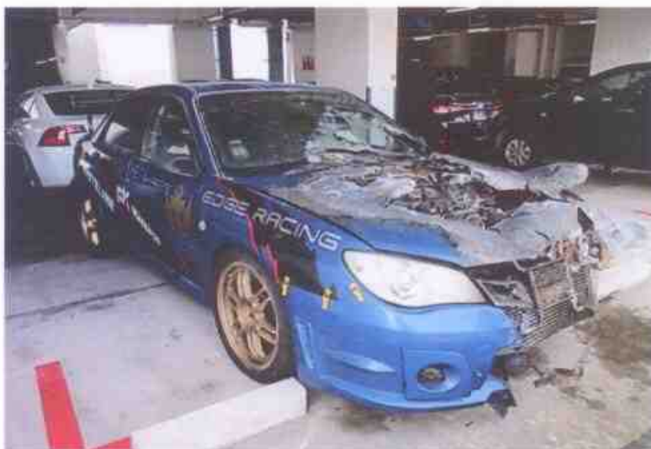
Photo 4 shows the general view of the right portion of the Insured Vehicle at the time of our inspection. The exterior body of the Insured Vehicle had sustained visible fire damage. This included its front windscreen, front bonnet, right headlight, front bumper, right side panel, right front rim and right front tire.
