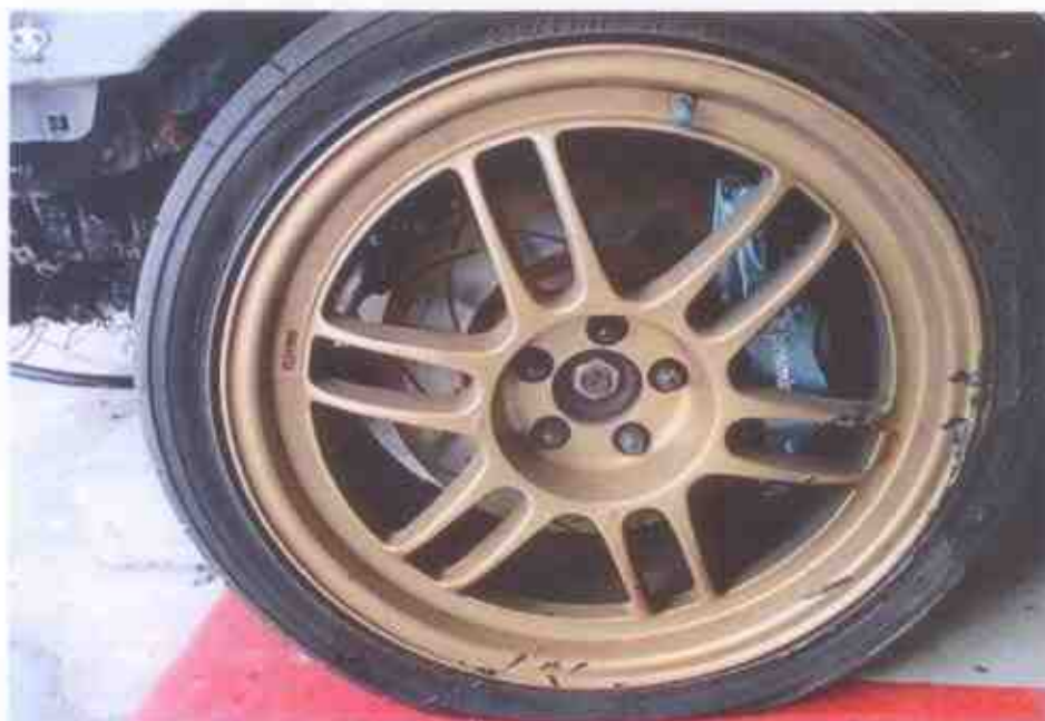
Photo 29 shows the non-standard rim found to be fitted on the Insured Vehicle at the time of our inspection. The 18- inch alloy rims fitted on the Insured Vehicle were not the standard type for the Insured Vehicle.
