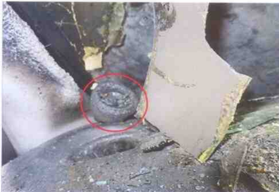
Photo 19 shows the 2nd aftermarket twitter fitted onto the left corner of the dashboard of the Insured Vehicle upon our inspection which had sustained serious fire damage (circled).
