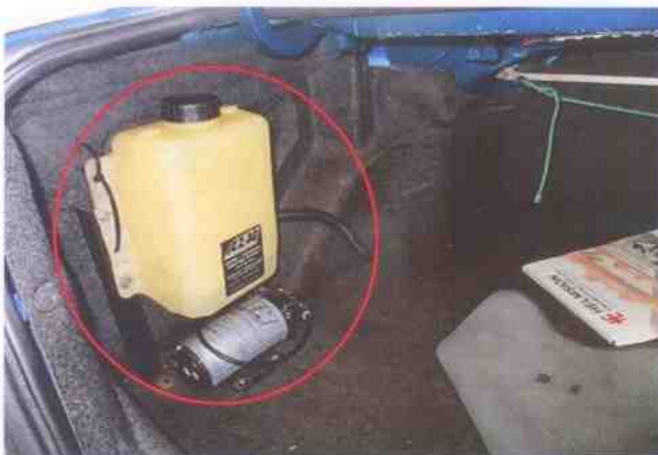
Photo 17 shows the water tank and motor for the water injection system that was found to be additionally fitted at the left portion of the Insured Vehicles' rear boot compartment upon our inspection (circled).
