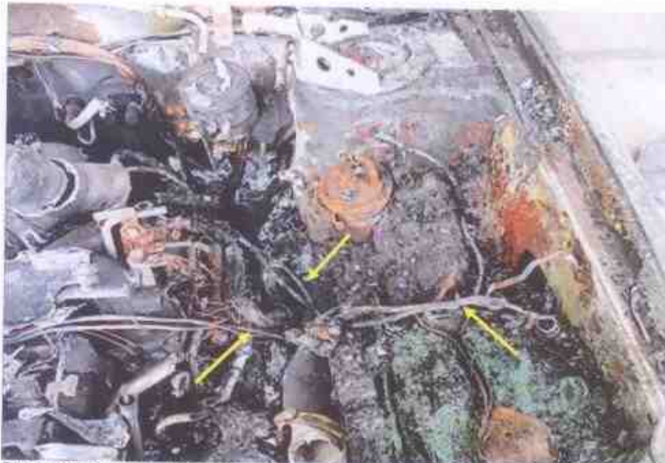
Photo 37 shows a closer view the greenish residue on the wirings at the left rear portion of the engine compartment (yellow arrows). The presence of such greenish residue suggests occurrence of an electrical short circuit.
