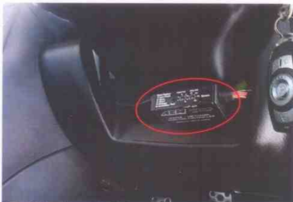
Photo 15 shows the controller for the water injection system that was found to be additionally fitted under the steering wheel of the Insured Vehicle upon our inspection (circled).
