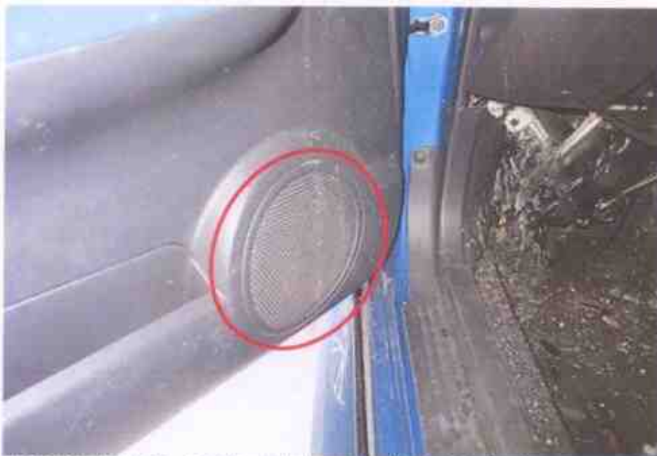
Photo 23 shows the 1st aftermarket speaker fitted at the front passenger door panel (circled).
