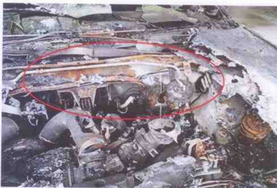
Photo 33 shows a closer view of the rust that had developed on the left rear portion of the engine compartment (circled). The development of rust is an indication that this area was subjected to prolonged exposure to high heat intensity, which had caused the steel/metal material of the front bonnet to be exposed to natural environmental condition. Hence the fire to the Insured Vehicle can be determined to have originated towards the left rear portion of the engine compartment.
