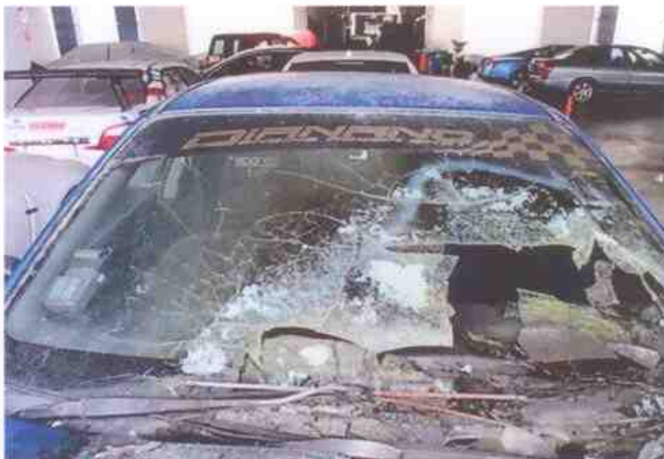
Photo 5 shows a closer view of the front windscreen of the Insured Vehicle at the time of our inspection. The front windscreen had sustained serious fire damage.
