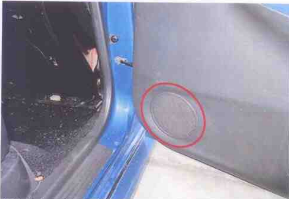
Photo 26 shows the 4th aftermarket speaker fitted at the right rear door panel (circled).
