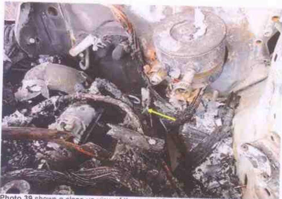
Photo 39 shows a close up view of the greenish residue on the wirings (arrowed) at the left rear portion of the engine compartment arrows). The presence of such greenish residue suggests occurrence of an electrical short circuit.
