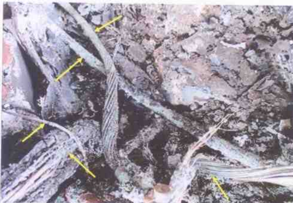
Photo 38 shows a close up view of the greenish residue on the wirings (yellow arrows) at the left rear portion of the engine compartment. The presence of such greenish residue suggests occurrence of an electrical short circuit.
