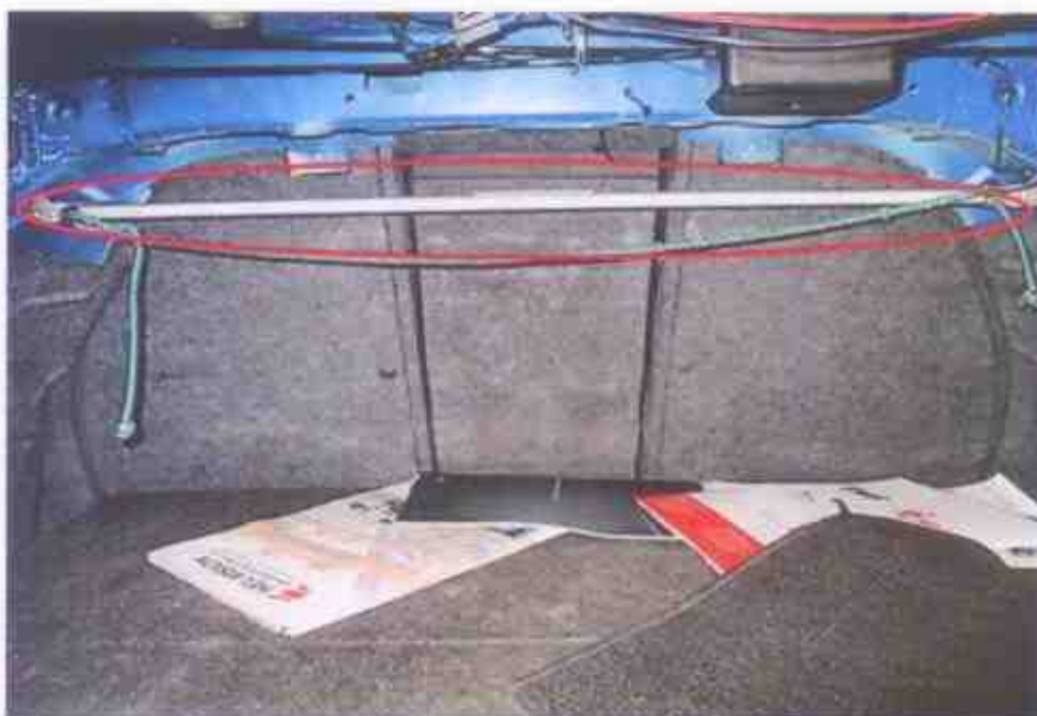
Photo 28 shows the rear strut bar (circled) fitted onto the rear boot compartment of the Insured Vehicle. The rear strut bar was found to be relatively unaffected by the fire.
