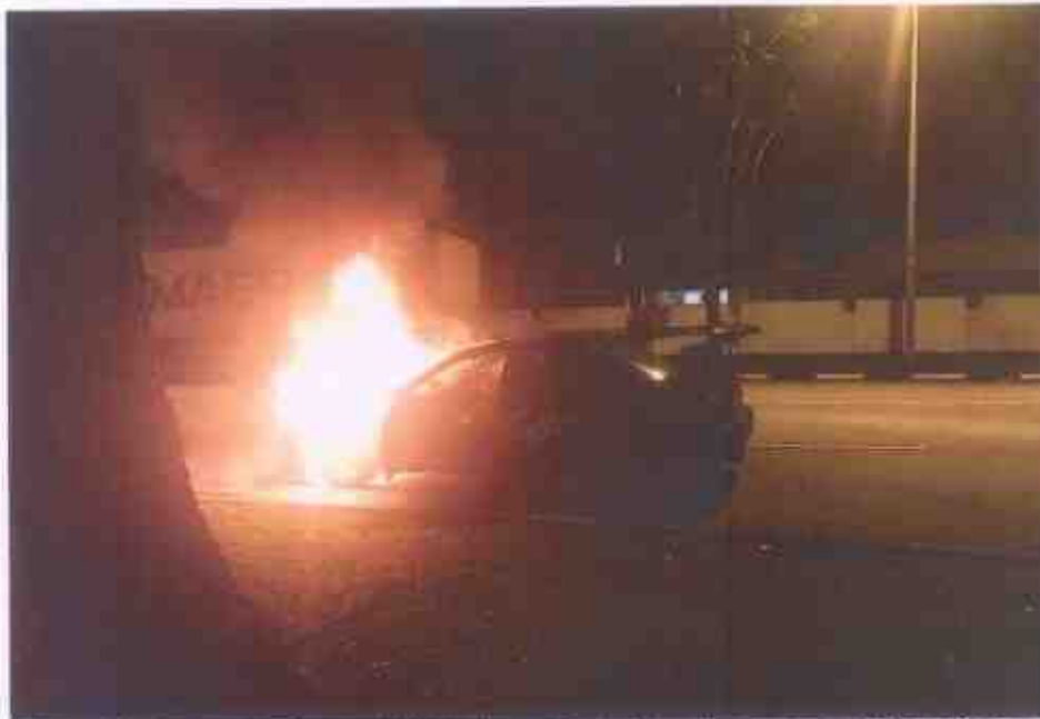
Photo 43 shows the Insured Vehicle on fire before the arrival of the SCDF. In general, the information that could be gathered from this photograph had corresponded to the events that were related to us by Mr Poh, which is the fire started from the front bonnet.
