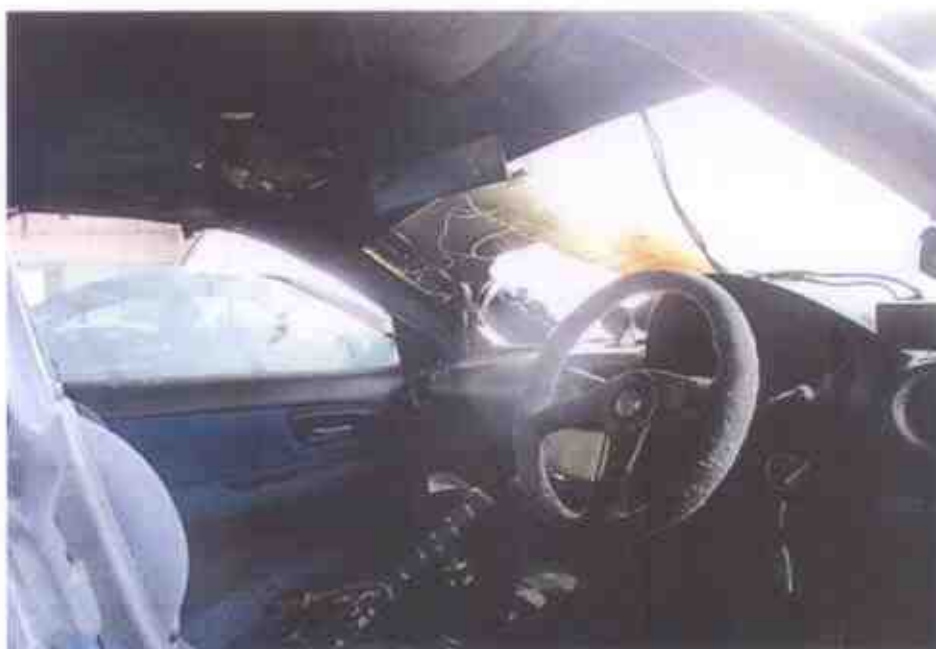
Photo 6 shows the interior compartment of the Insured Vehicle at the time of our inspection. The interior compartment of the Insured Vehicle was relatively unaffected by the fire, except for the left portion.
