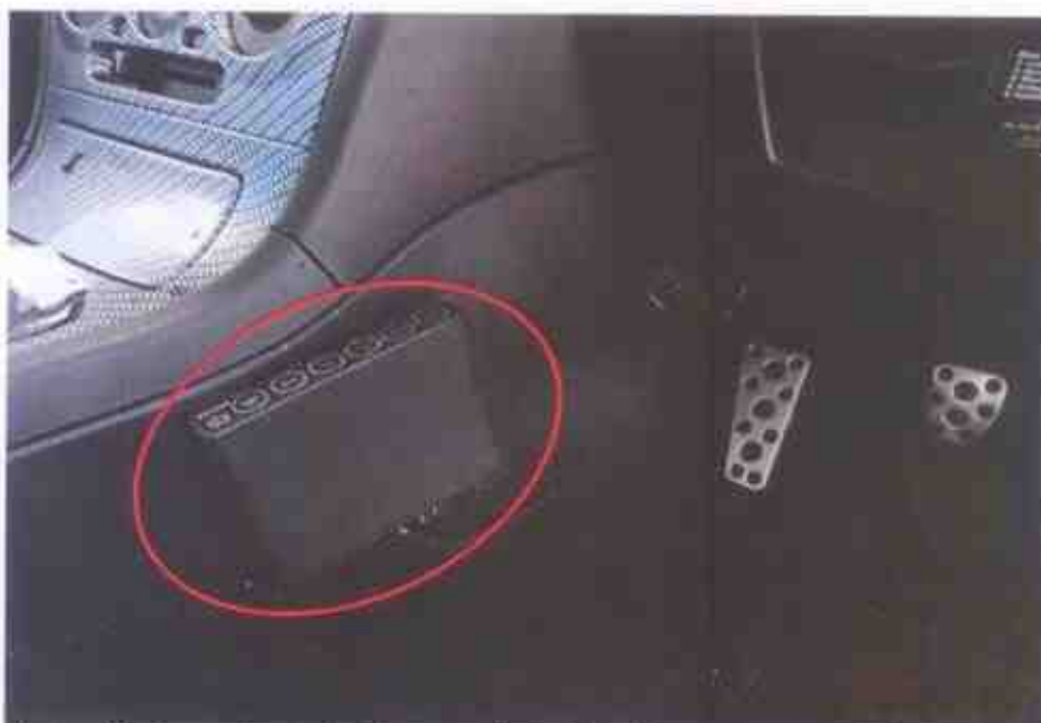
Photo 12 shows the controller console for the aftermarket gauges (circled) that was found to be additionally fitted onto the Insured Vehicle upon our inspection. The brand of the controller console was 'DEFI' (circled).
