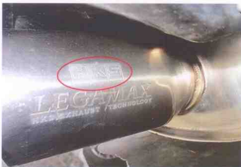
Photo 31 shows a close up side view of the non-standard rear exhaust muffler that was found to be fitted on the Insured Vehicle at the time of our inspection. The brand of the rear exhaust muffler was 'HKS' (circled).
