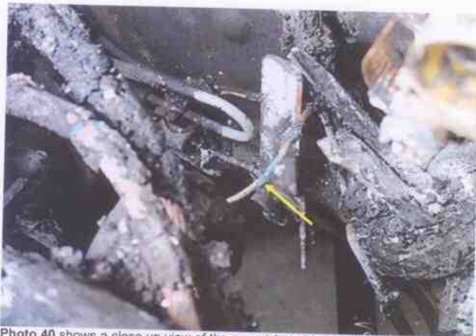
Photo 40 shows a close up view of the greenish residue on the wirings (arrowed) at the left rear portion of the engine compartment. The presence of such greenish residue suggests occurrence of an electrical short circuit.
