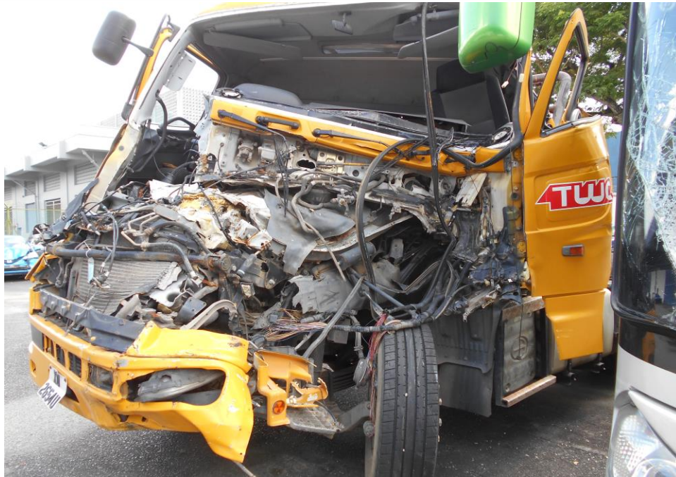
Photo 2 shows a closer view of the frontal left portion of the Motor Trailer at the time of our inspection. A number of mechanical parts and components at the frontal portion were also severely damaged as a result of the accident.
