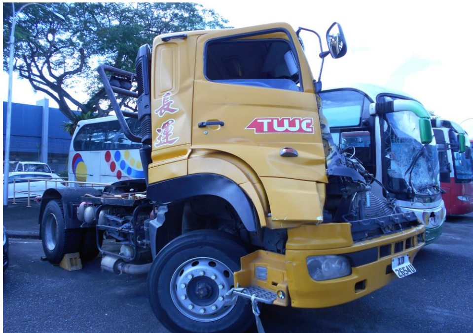
Photo 3 shows a general view of the front right portion of the Motor Trailer at the time of our inspection. The Motor Trailer was observed to have sustained extensive impact damage at its front right portion. The impact force was relatively significant, causing its entire front portion to be buckled and crumpled.
