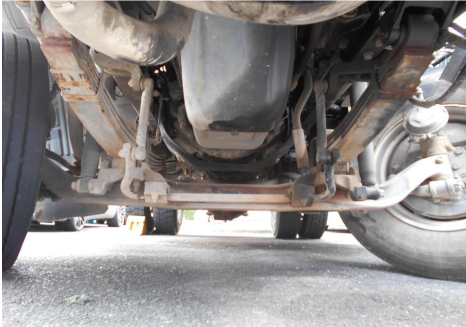
Photo 12 shows the underside of the Motor Trailer, at the area where the engine is located. We were not able to closely inspect the engine compartment of the Motor Trailer due to the extensive damage to its front cabin. Our visual checks from the underside had however appear to indicate that the engine assembly and transmission assembly were both intact and unaffected by the collision.
