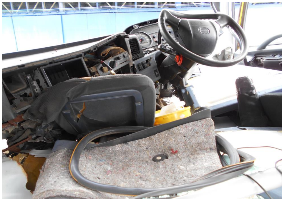
Photo 5 shows the interior of the front cabin. The dashboard, steering wheel, seats, floor panel and roof panel inside the front cabin were all observed to be pushed/buckled inwards, towards the rear of the Motor Trailer. This is consistent to the nature of this accident where the direction of impact onto the Motor Trailer was from the front to rear direction.
