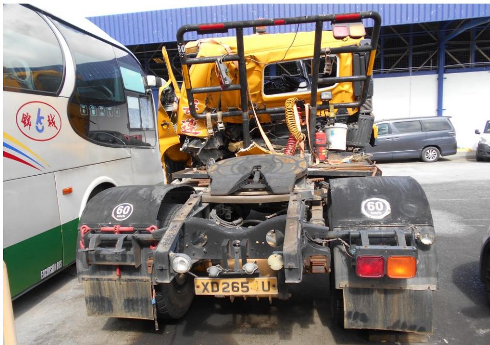
Photo 7 shows a general view of the rear portion of the Motor Trailer at the time of my inspection. The rear portion was observed to be relatively unaffected by the accident.
