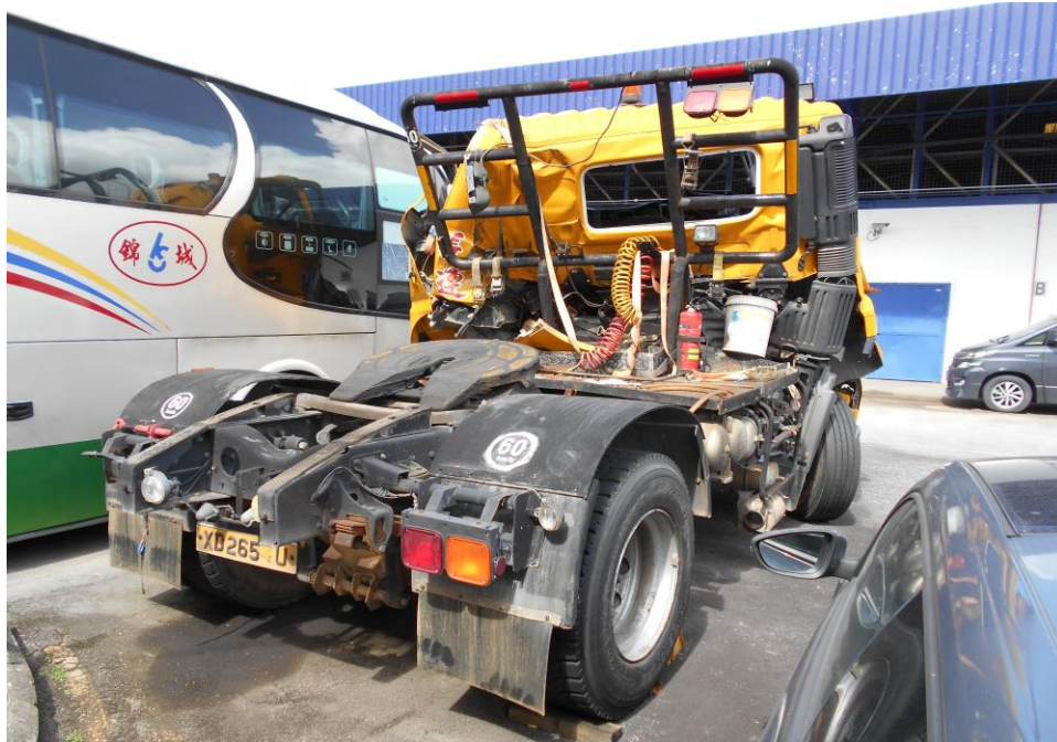
Photo 6 shows a general view of the rear right portion of the Motor Trailer at the time of our inspection. The rear portion was observed to be relatively unaffected by the accident.
