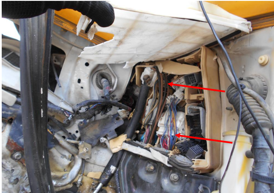
Photo 21 shows the damaged electrical module which caused ignition failure that disabled the ignition system & related systems due to the accident.
