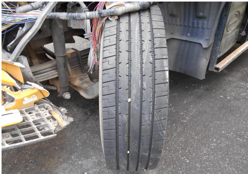
Photo 10 shows the condition of the front left tyre of the Motor Trailer, which was observed to be in serviceable condition with remaining tread depth of approximately 7mm. There was also no tear, cut or burst mark(s) on the outer and the inner sidewalls as well as across the tread of this tyre.
