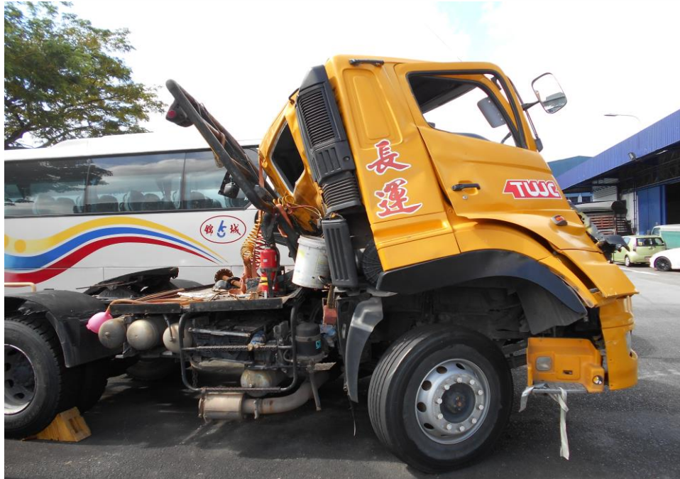
Photo 4 shows from a right side view of the Motor Trailer at the time of our inspection. The Motor Trailer was observed to have sustained extensive impact damage at its front portion. The impact force was relatively significant, causing its entire front cabin to be buckled and crumpled.
