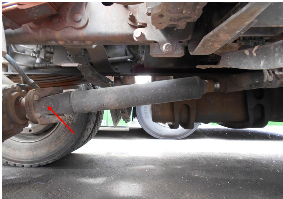
Photo 13 shows the transmission assembly (arrowed) of the Motor Trailer intact and unaffected by the collision.
