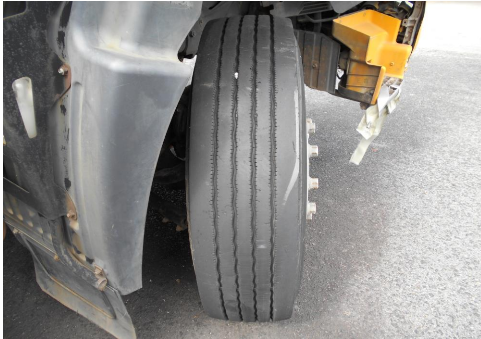
Photo 11 shows the condition of the front right tyre of the Motor Trailer. The front right tyre was observed to be in serviceable condition with remaining tread depth of approximately 7mm. There was also no tear, cut or burst mark(s) on the outer and the inner sidewalls as well as across the tread of this tyre.
