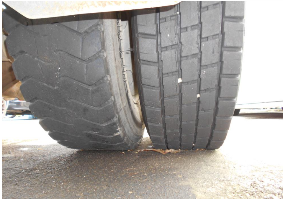
Photo 9 shows the condition of the rear left tyres of the Motor Trailer, which was observed to be in serviceable condition with remaining tread depth of approximately 7mm. There was no tear, cut or burst mark(s) on the outer and the inner sidewalls as well as across the tread of these 2 tyres, which were also observed to be sufficiently inflated for vehicular operation.
