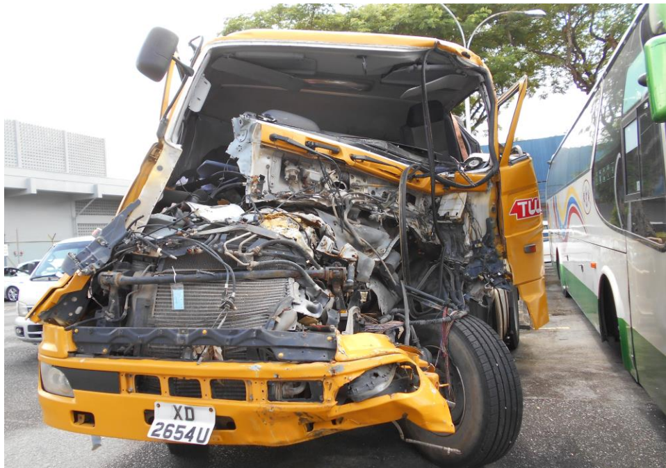
Photo 1 shows a general view of the frontal portion of the Motor Trailer at the time of our inspection. The Motor Trailer was observed to have sustained extensive impact damage at its frontal portion. The impact force was relatively significant, causing its entire front portion to be buckled and crumpled pushed inwards towards to rear portion of the Motor Trailer.
