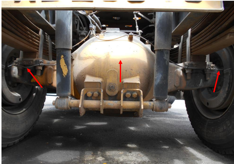
Photo 18 shows the brake hose (arrowed) at the rear right wheel of the Motor Trailer. At the time of our inspection, we did not find any sign(s) of brake fluid leakage along the brake hoses and brake pipes.
