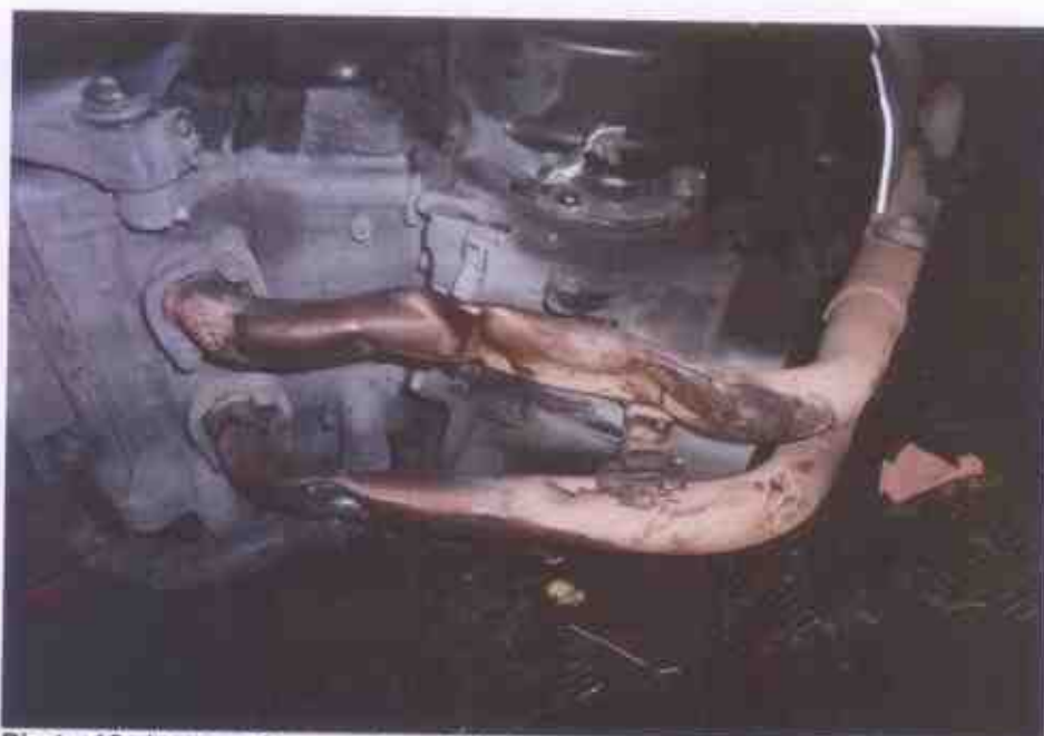
Photo 10 shows a close-up view of the front portion of the Motorcycle at the time of our inspection. The Motorcycle's engine components such as exhaust manifold observed to have sustained relatively extensive impact due to the accident collision.
