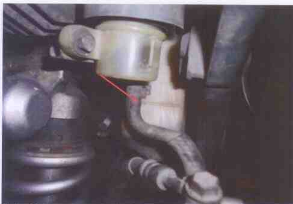
Photo 24 shows the rear brake fluid reservoir of the Motorcycle. Our visual checks had revealed that it was still at a sufficient level & without contamination at time of our examination.
