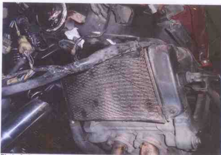
Photo 9 shows a close-up view of the front portion of the Motorcycle at the time of our inspection. The Motorcycle engine components such as radiator, front fork & other components were observed to have sustained relatively extensive impact due to the accident collision.
