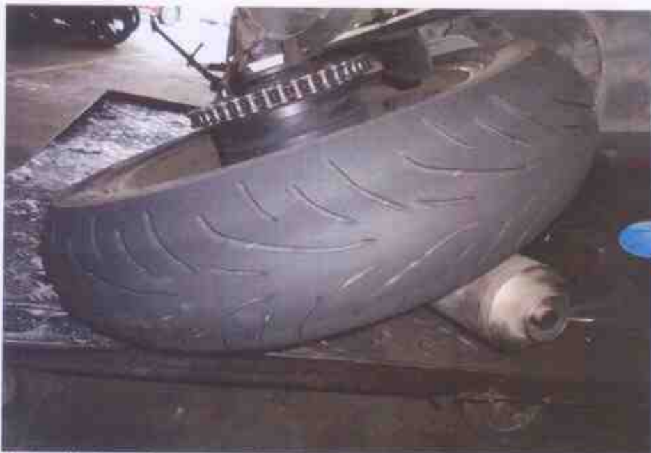
Photo 11 shows the rear tyre of the Motorcycle at the time of our inspection. The rear tyre was observed to be in serviceable condition with remaining tread depth of approximately 5mm. The tyre was also observed to be sufficiently inflated for vehicular operation. There was no significant damage observed on the rear wheel rim & tyre.
