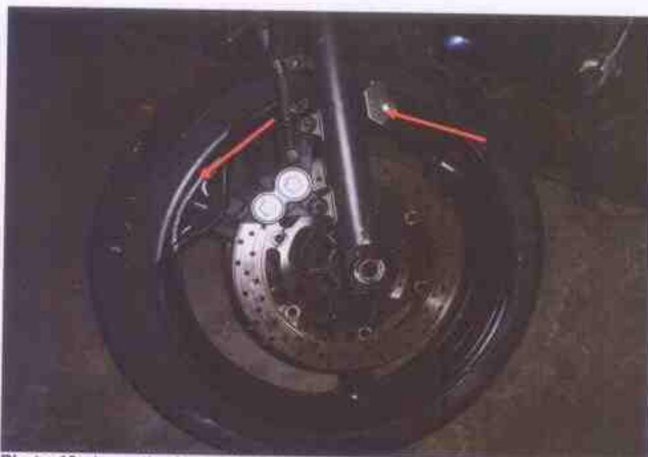
Photo 19 shows the front wheel rim (arrowed) was observed to be broken as a result of the accident. Hence, we are unable to conduct any tests on the braking system of the Motorcycle.
