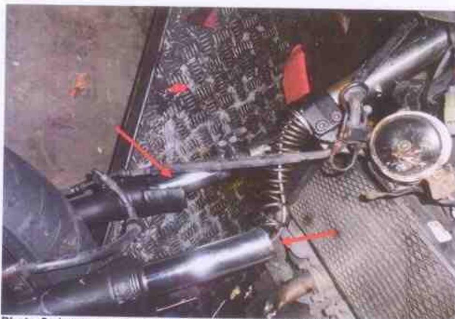
Photo 3 shows a general view of the front body of the Motorcycle at the time of our inspection. The Motorcycle was observed to have sustained with relatively extensive impact due to the accident collision. Amongst the body parts damaged was its front fork (arrowed), which was observed to be dislodged from the Motorcycle body.
