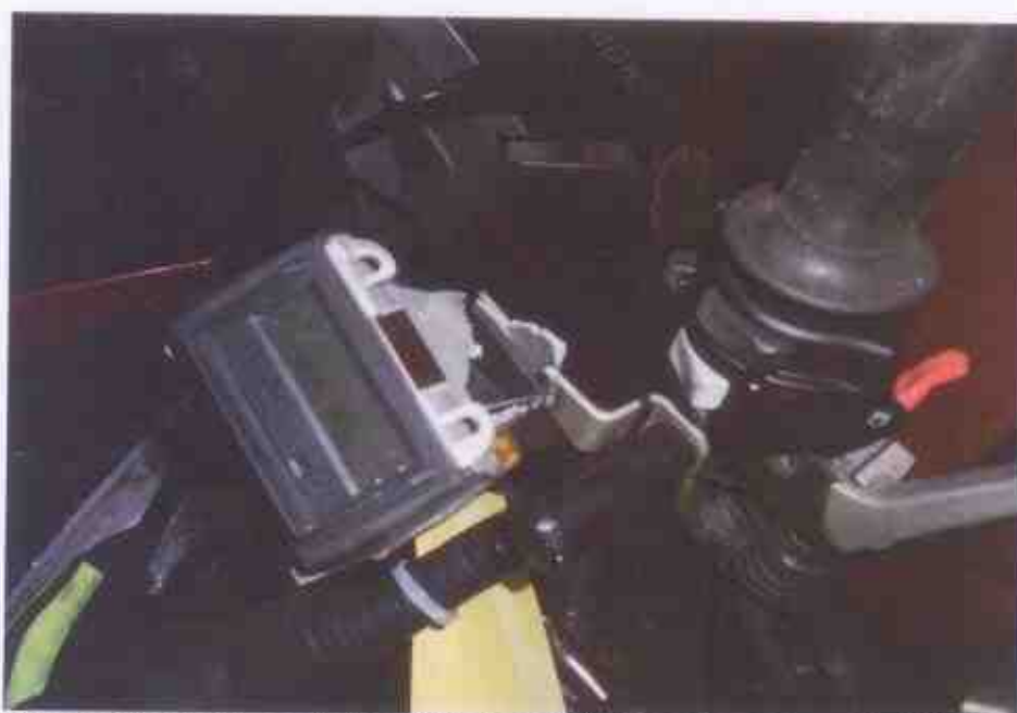
Photo 7 shows a close-up view of the in-vehicle unit of the Motorcycle at the time of our inspection. It was observed to have sustained relatively extensive impact damages to the in-vehicle unit due to the accident collision.
