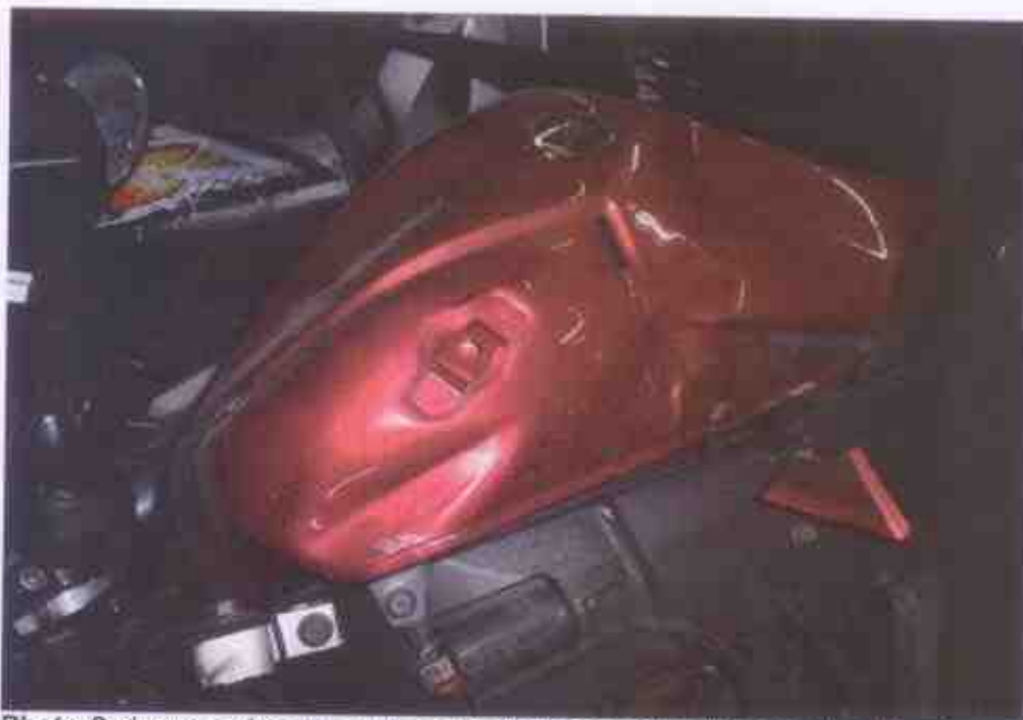
Photo 8 shows a close-up view of the fuel tank of the Motorcycle at the time of our inspection. It was observed to have sustained relatively extensive impact including damages to the fuel tank due to the accident collision.
