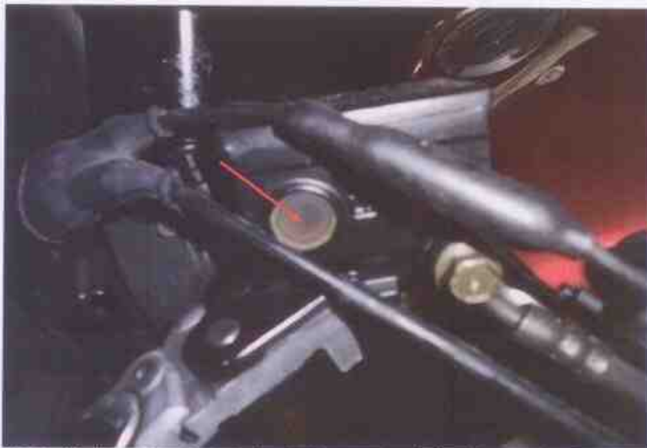
Photo 22 shows the front brake fluid reservoir of the Motorcycle. Our visual checks had revealed that it was still at a sufficient level & without contamination at time of our examination.
