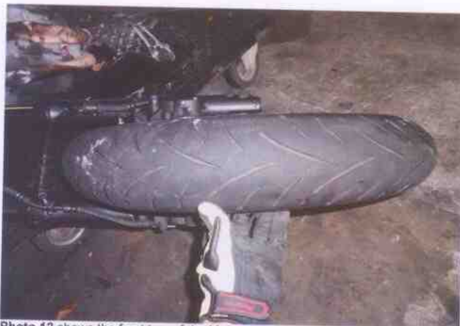
Photo 12 shows the front tyre of the Motorcycle and the tread pattern was clearly visible. There was no tear, burst mark(s) and/or punctured hole(s) on the sidewalls as well as across the tread of the front tyre with remaining tread depth of approximately 4mm. However, the wheel rim was observed to be broken & deflated as a result of the accident.
