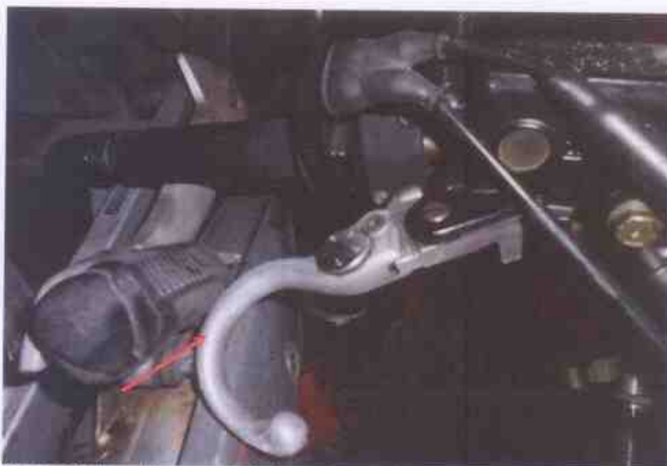
Photo 18 shows the hand brake lever (arrowed) was observed to be broken due to the result of the accident. Hence, we are unable to conduct any tests on the braking system of the Motorcycle.
