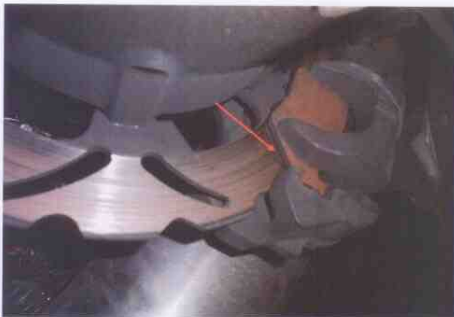
Photo 23 shows the rear brake pad of the Motorcycle which was observed to be in serviceable condition. No damages were found at time of our inspection to the rear braking components.
