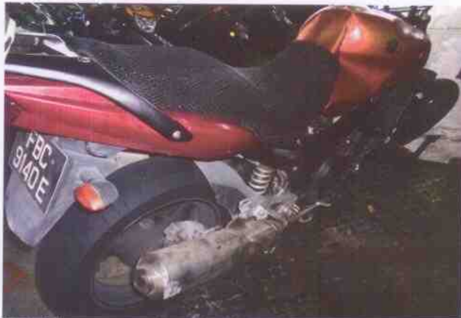
Photo 5 shows a general view of the right body of the Motorcycle at the time of our inspection. The Motorcycle was observed to have sustained damages at the frontal portion, rear portion, along both its left side and right side.
