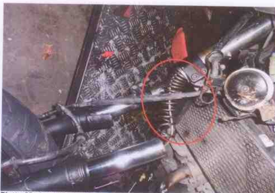
Photo 20 shows the front fork (circled) was observed to be dislodged as a result of the accident. Hence, we are unable to conduct any tests on the steering system of the Motorcycle.
