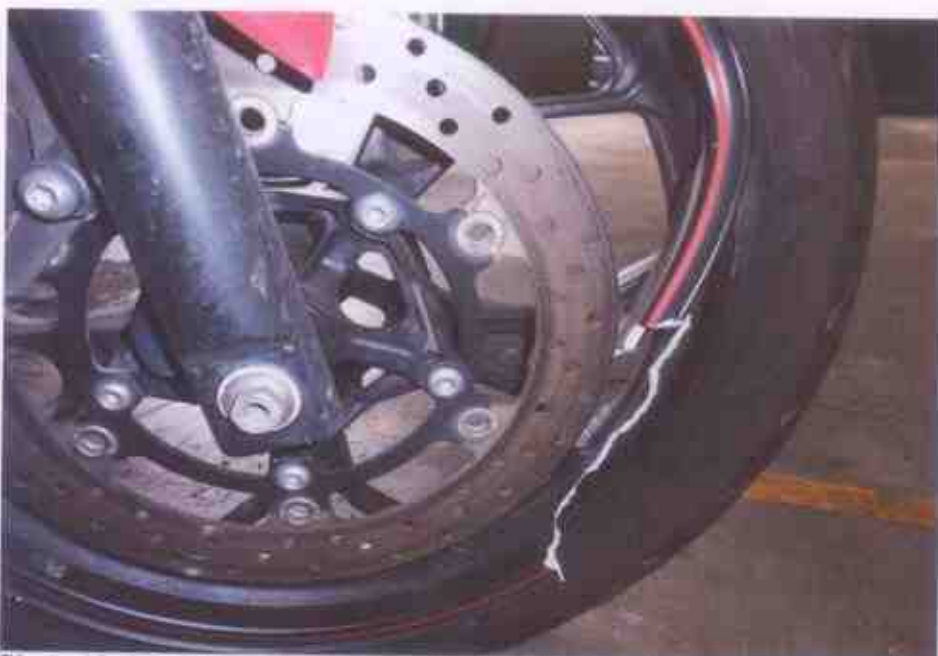
Photo 12 shows the cracked wheel rim on front tyre of the Motorcycle at the time of our inspection.
