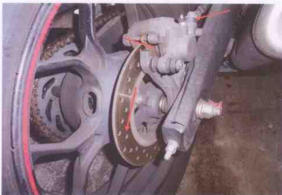
Photo 19 shows the rear brake calliper, rear brake disc and rear brake hose of the Motorcycle (arrowed), which are all part of the components in the front brake system of the Motorcycle. Our visual checks of these various components had revealed all to be intact with no visible damage. No leakage of brake fluid was also observed.
