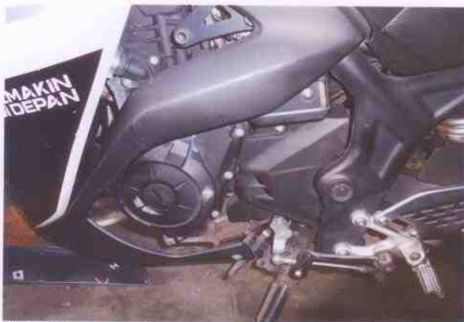
Photo 13 shows no sign(s) or indication(s) of fluid leakage stain observed around the engine undercarriage area of the Motorcycle.
