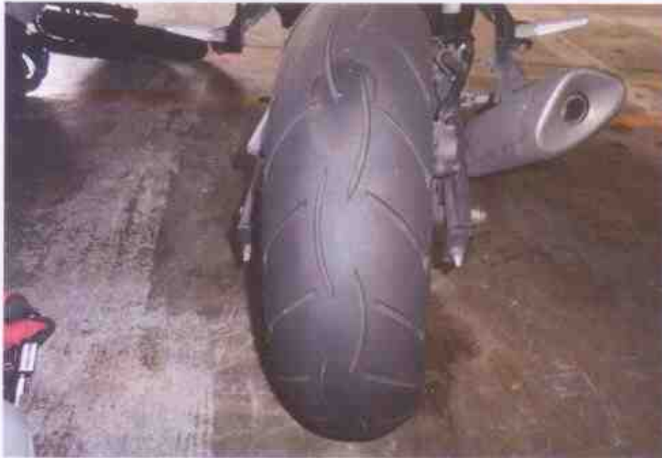
Photo 9 shows the rear tyre of the Motorcycle at the time of our inspection. The rear tyre was observed to be in serviceable condition with remaining tread depth of approximately 6mm. The tyre was also observed to be sufficiently inflated for vehicular operation. There was no significant damage observed on the rear wheel rim & tyre.
