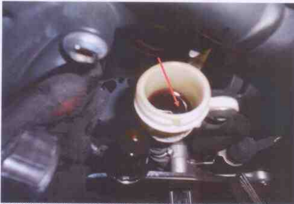
Photo 22 shows the rear brake fluid reservoir of the Motorcycle. It was observed to be of sufficient level without any contamination at time of our inspection.
