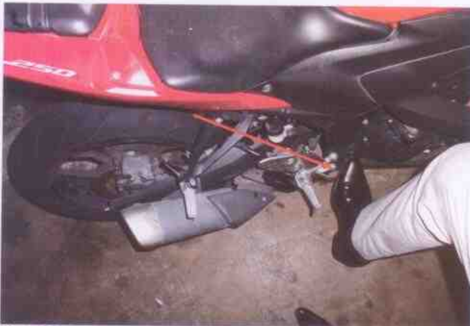
Photo 25 shows the rear brake static test. It had appeared to indicate that the brake system of the Motorcycle was in serviceable condition. There was some resistance felt (spongy like feel) upon stepping on the rear brake foot paddle. This would indicate that there was no abnormality in the brake system also on the rear brake drum mechanical parts.
