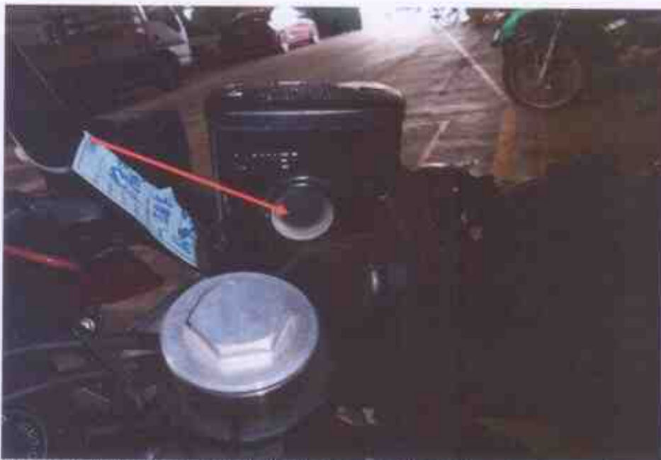
Photo 23 shows the front brake fluid reservoir of the Motorcycle. It was observed to be of sufficient level without any contamination at time of our inspection.
