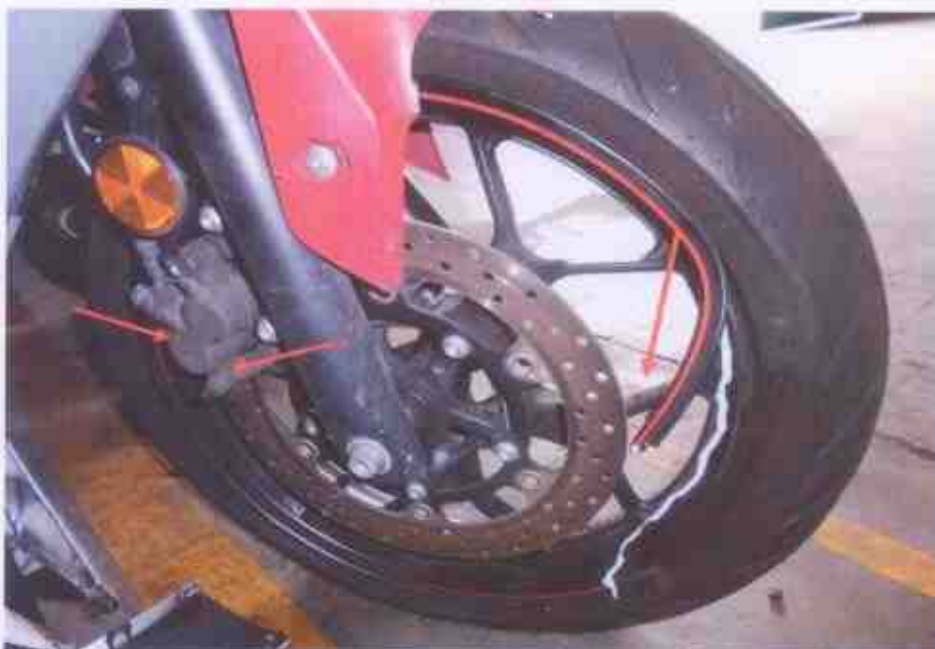
Photo 18 shows the front brake calliper, front brake disc and front brake hose of the Motorcycle (arrowed), which are all part of the components in the front brake system of the Motorcycle. Our visual checks of these various components had revealed all to be intact with no visible damage. No leakage of brake fluid was also observed.
