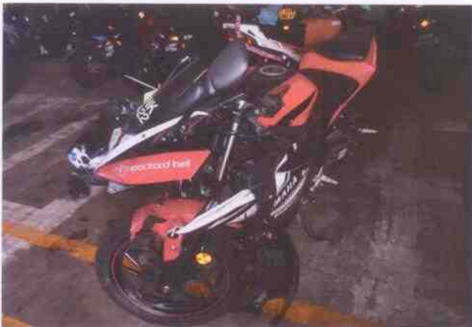
Photo 1 shows a general view of the front body of the Motorcycle at the time of our inspection. The Motorcycle was observed to be sustained with relatively extensive impact due to the accident collision. Amongst the body parts damaged was its steering system, which was observed to be buckled inwards.
