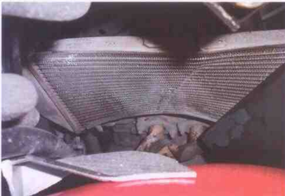
Photo 6 shows a close-up view of the radiator of the Motorcycle at the time of our inspection. It was observed to have sustained with damages due to the accident collision.
