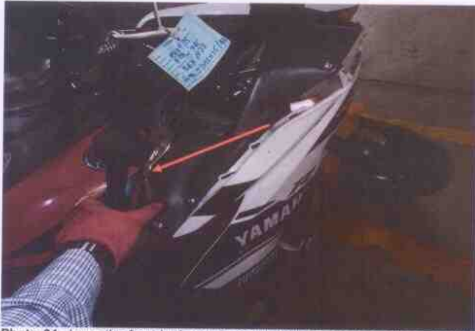
Photo 24 shows the front brake static test. It had appeared to indicate that the brake system of the Motorcycle was in serviceable condition. There was some resistance felt (spongy like feel) upon gripping the hand brake lever.
