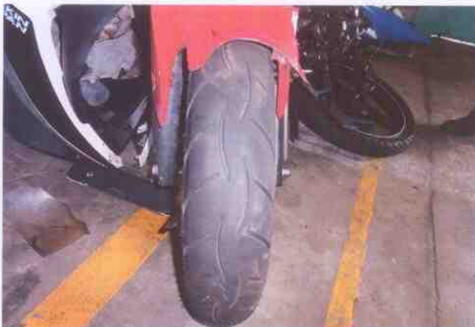
Photo 10 shows the front tyre of the Motorcycle at the time of our inspection. The pattern of the tread was clearly visible. There was no tear, burst mark(s) and/or punctured hole(s) on the sidewalls as well as across the tread of the front tyre with remaining tread depth of approximately 6mm. However, it was observed to be deflated as a result of the accident.
