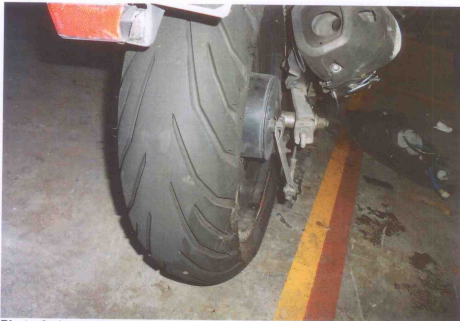
Photo 9 shows the rear tyre of the Motorcycle at the time of our inspection. The rear tyre was observed to be in serviceable condition with remaining tread depth of approximately 5mm. The tyre was also observed to be sufficiently inflated for vehicular operation. There was no significant damage observed on the rear wheel rim & tyre.
