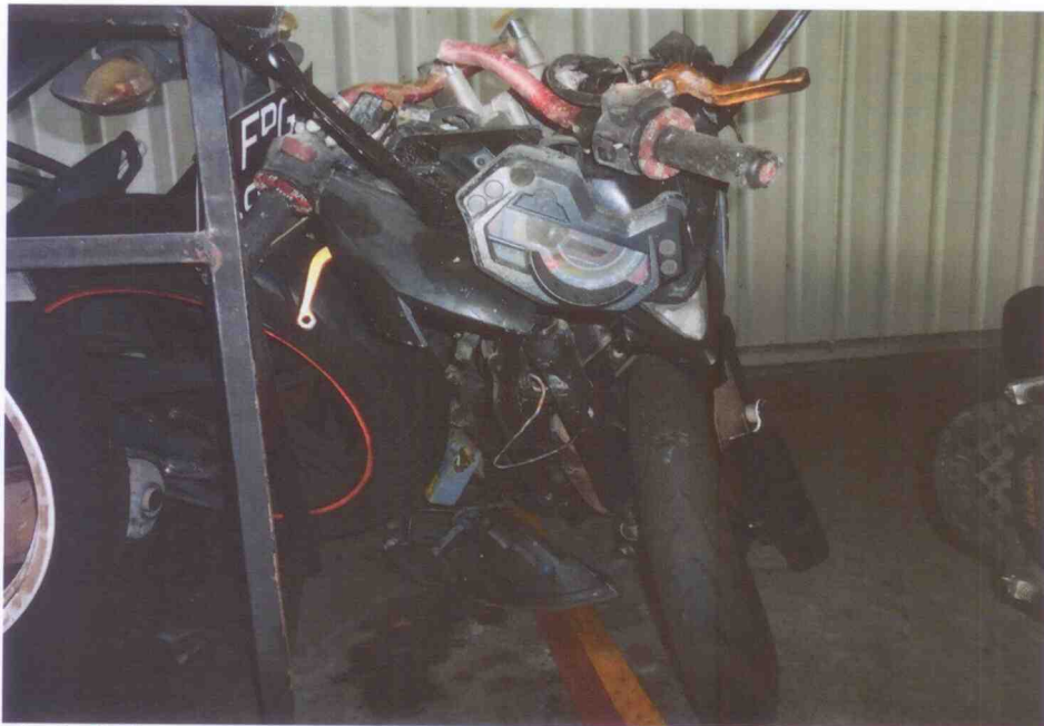
Photo 1 shows the general view of the frontal portion of the Motorcycle at time of our examination. It was observed to sustained severe damages due to the accident's impact collision.
