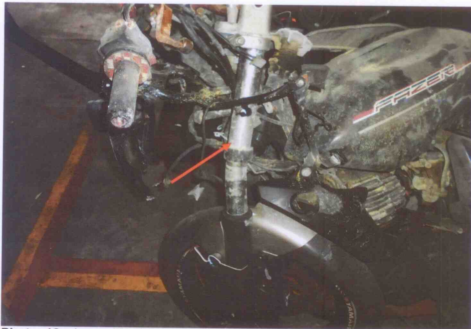
Photo 18 shows the front fork (arrowed) that was observed to be buckled inwards as a result of the accident. Hence, we are unable to conduct any tests on the steering system of the Motorcycle.
