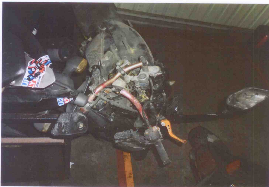
Photo 7 shows a semi close-up view of the front portion of the Motorcycle at the time of our inspection. The Motorcycle was observed to have sustained relatively extensive impact due to the accident collision which includes a broken handle bar.
