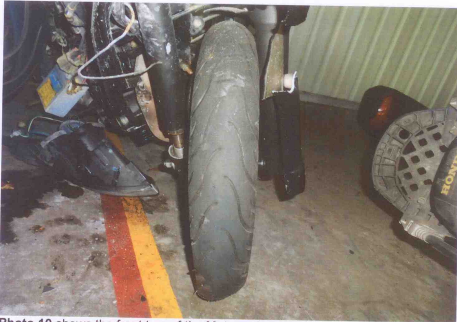
Photo 10 shows the front tyre of the Motorcycle at the time of our inspection. The pattern of the tread was clearly visible. There was no tear, burst mark(s) and/or punctured hole(s) on the sidewalls as well as across the tread of the front tyre with remaining tread depth of approximately 5mm. It was also observed to be deflated as a result of the accident.
