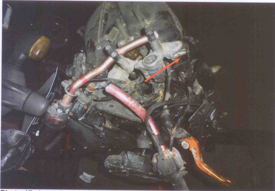
Photo 17 shows the handle bar that was observed to be broken due to the result of the accident. Hence, we are unable to conduct any tests on the steering system & braking system of the Motorcycle.
