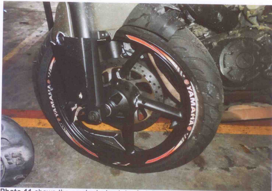
Photo 11 shows the cracked wheel rim & deflated front tyre of the Motorcycle at the time of our inspection.
