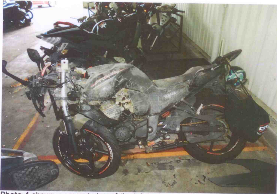
Photo 4 shows a general view of the left body of the Motorcycle at the time of our inspection. The Motorcycle was observed to have sustained damages at the frontal portion, rear portion, along both its left side and right side.
