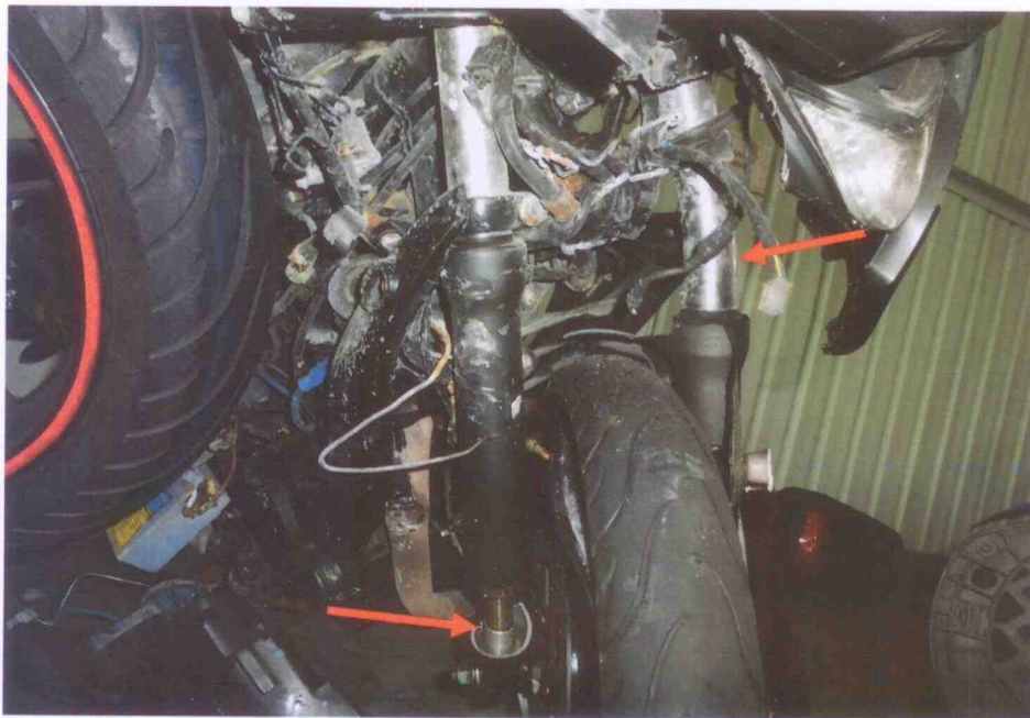
Photo 3 shows a general view of the front portion of the Motorcycle at the time of our inspection. The Motorcycle was observed to have sustained with relatively extensive impact due to the accident collision. Amongst the body parts damaged was its front fork (arrowed), which was observed to be broken and buckled inwards.
