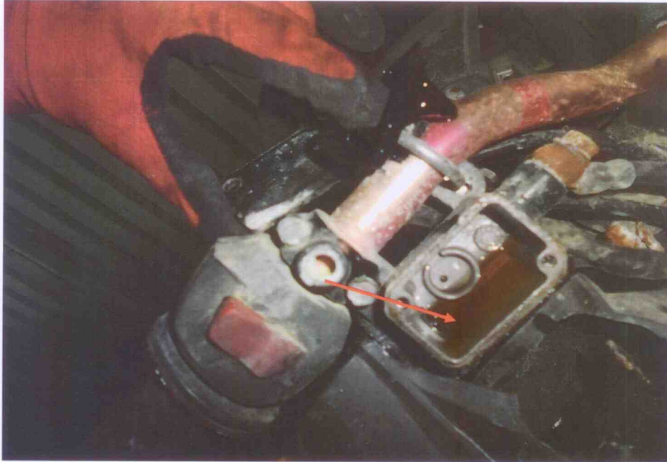
Photo 21 shows the front brake fluid reservoir of the Motorcycle. The brake fluid was observed to be in an insufficient level due to the damages sustained as a result of the accident.
