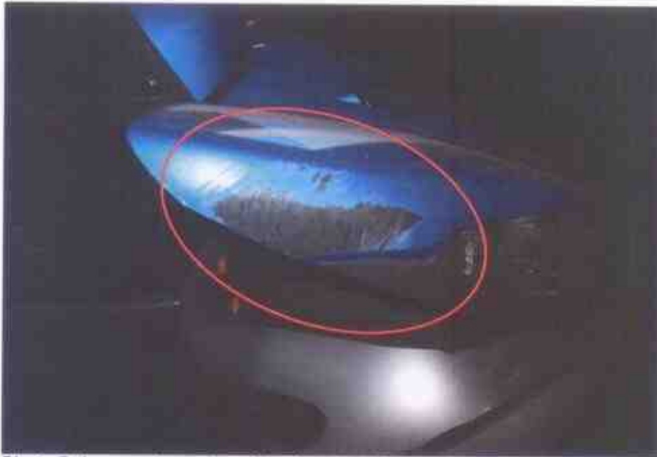
Photo 7 shows a closer view of the front right fairing of the Motorcycle at the time of our inspection. The Motorcycle was observed to have sustained with relatively minor damages due to the accident collision. (Circled)
