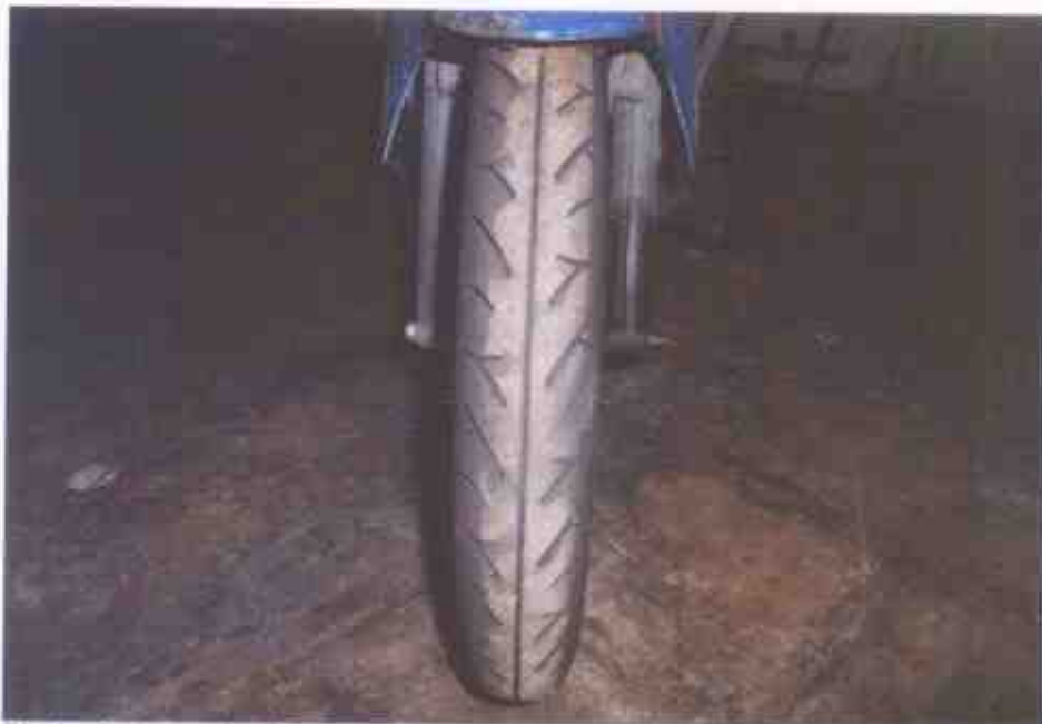
Photo 9 shows the front tyre of the Motorcycle. The front tyre was observed to be in serviceable condition with remaining tread depth of approximately 4mm. The tyre was also observed to be sufficiently inflated for vehicular operation.
