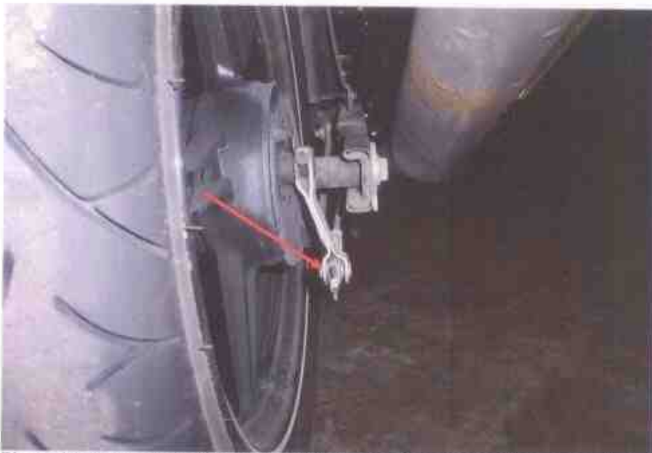
Photo 15 shows our checks on the braking component (rear) had also indicated that the braking system was of serviceable condition for operational purposes, and without abnormalities.
