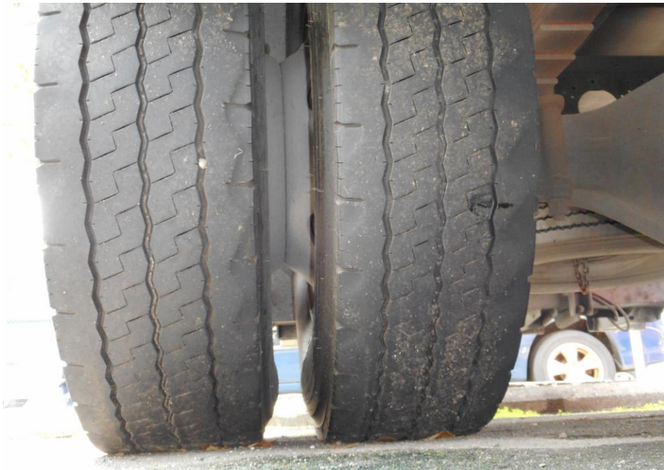
Photo 9 shows the condition of the rear right tyres of the Motor Lorry, which were observed to be in serviceable condition with remaining tread depth of approximately 7.2mm. There was also no tear, cut or burst mark(s) on the outer and the inner sidewalls as well as across the tread of the 6 tyres that were fitted on the Motor Lorry.
