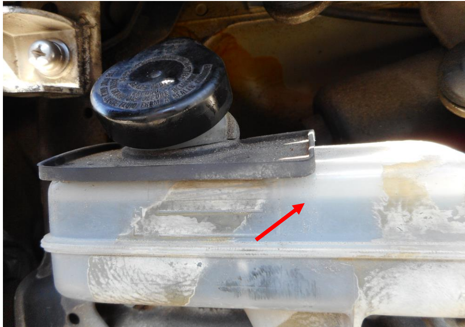
Photo 11 shows the brake fluid reservoir of the Motor Lorry at the time of my inspection. The brake fluid was observed to be of sufficient level (arrowed) and without any visible contamination.
