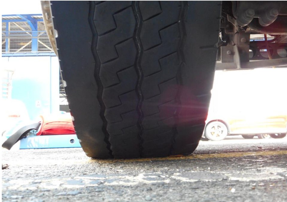
Photo 6 shows the condition of the front left tyre of the Motor Lorry, which was observed to be in serviceable condition with remaining tread depth of approximately 7.4mm. The tyre, which was wrapped around standard alloy wheel rim, was also observed to be sufficiently inflated for vehicular operation. There was no tear, cut or burst mark(s) on the outer and the inner sidewalls as well as across the tread of the 6 tyres that were fitted on the Motor Lorry.
