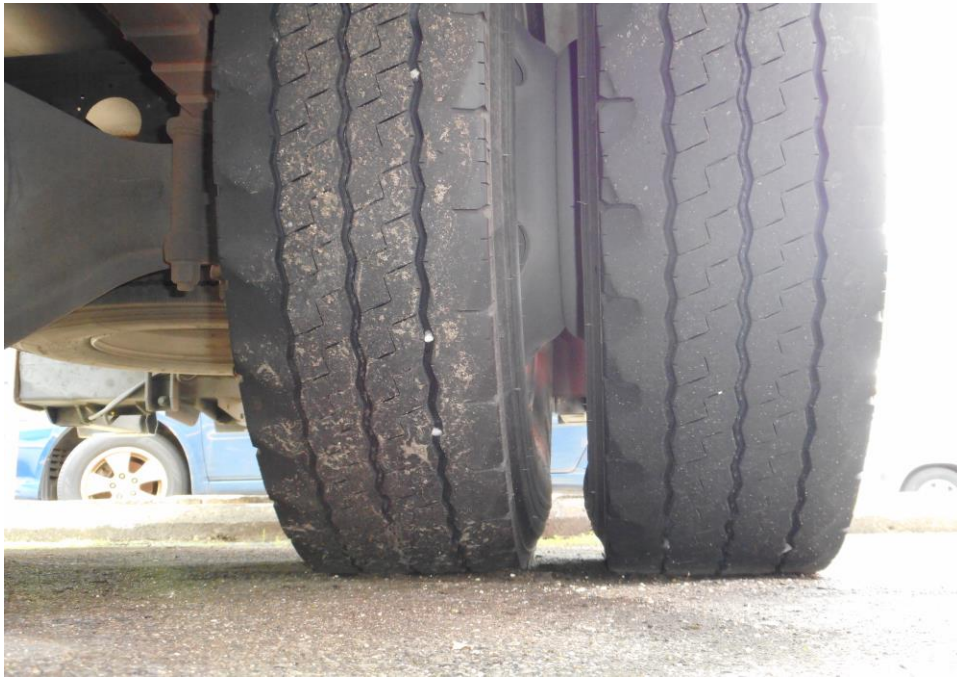
Photo 8 shows the condition of the rear left tyres of the Motor Lorry, which was observed to be in serviceable condition with remaining tread depth of approximately 6.3mm. The tyres, which were wrapped around standard alloy wheel rim, were also observed to be sufficiently inflated for vehicular operation. There was also no damage found on all 6 alloy wheel rims of the Motor Lorry.
