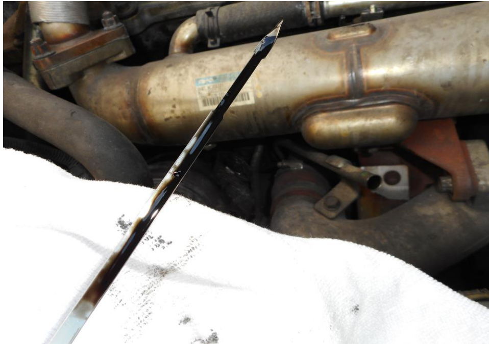
Photo 15 shows the engine dip stick of the Motor Lorry at the time of my inspection. The engine oil was observed to be of sufficient level and without any visible contamination.
