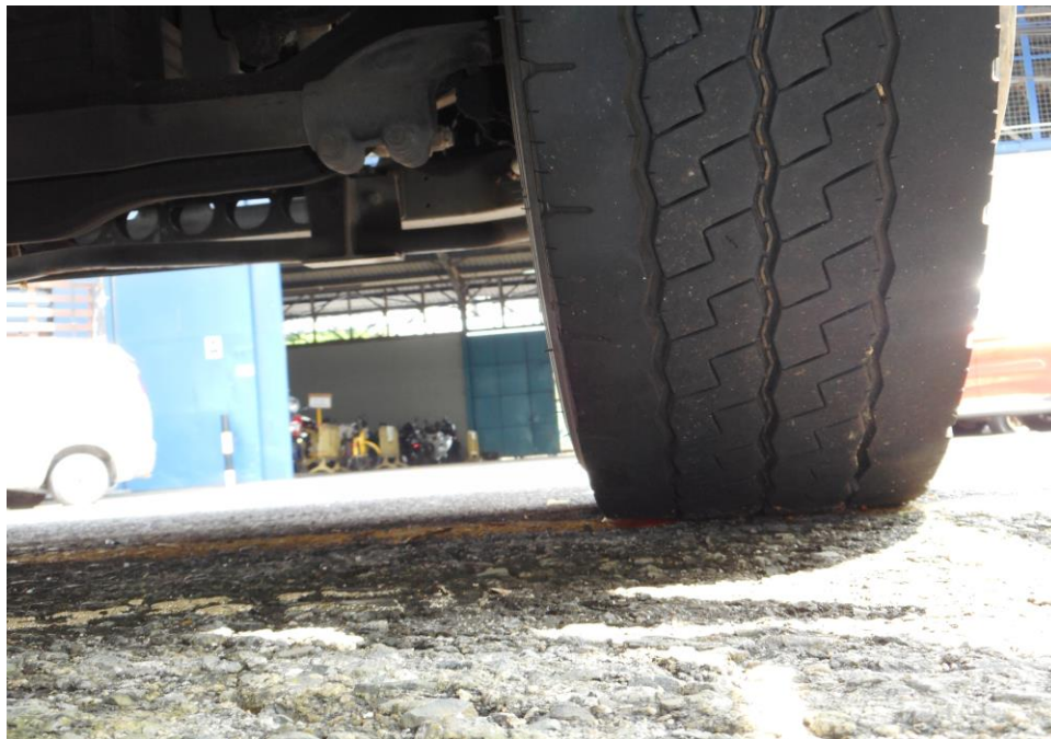
Photo 7 shows the condition of the front right tyre of the Motor Lorry, which was observed to be in serviceable condition with remaining tread depth of approximately 6.7mm. The tyre, which was wrapped around standard alloy wheel rim, was also observed to be sufficiently inflated for vehicular operation.
