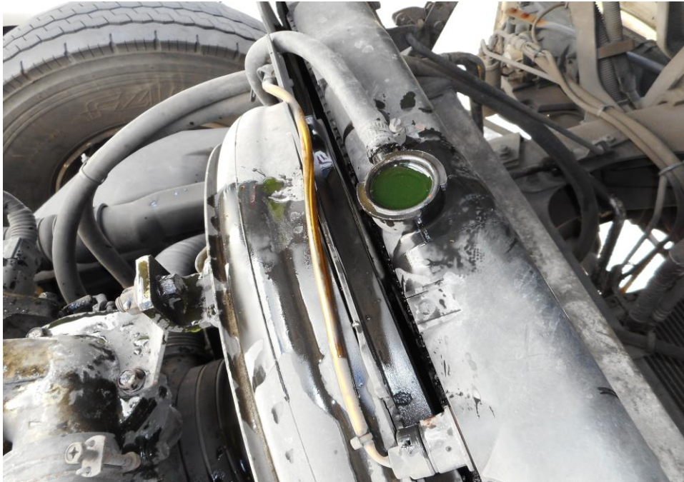
Photo 13 shows the engine coolant reservoir of the Motor Lorry at the time of my inspection. The engine coolant was observed to be of sufficient level and without any visible contamination.
