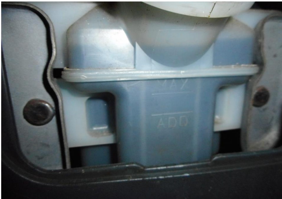
Photo 13 shows the brake fluid reservoir of the Motor Lorry at the time of my inspection. The brake fluid was observed to be of sufficient level and without any visible contamination.
