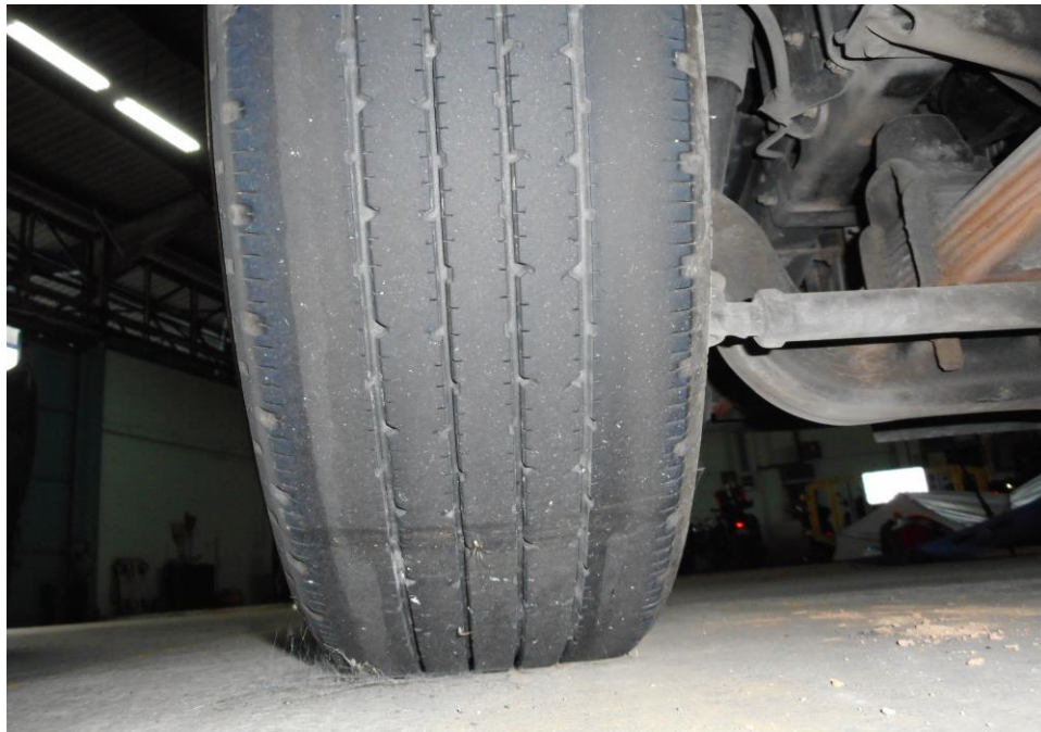
Photo 7 shows the condition of the front left tyre of the Motor Lorry, which was observed to be in serviceable condition with remaining tread depth of approximately 5.3mm. The tyre, which was wrapped around standard alloy wheel rim, was also observed to be sufficiently inflated for vehicular operation. There was no tear, cut or burst mark(s) on the outer and the inner sidewalls as well as across the tread of the 6 tyres that were fitted on the Motor Lorry.
