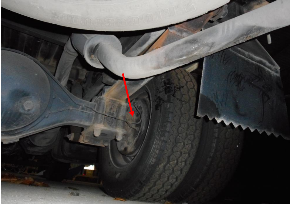
Photo 17 shows the brake pipe (arrowed) at the rear right wheel of the Motor Lorry. I did not observe any leakage of brake fluid at the time of my inspection of the Motor Lorry. My static tests of the Motor Lorry's braking system, along with my visual examination of the various mechanical components in the braking system, had indicated that there was no internal leakage of pressure/vacuum. Hence the braking system of the Motor Lorry was likely to be in serviceable condition at the material time of accident.
