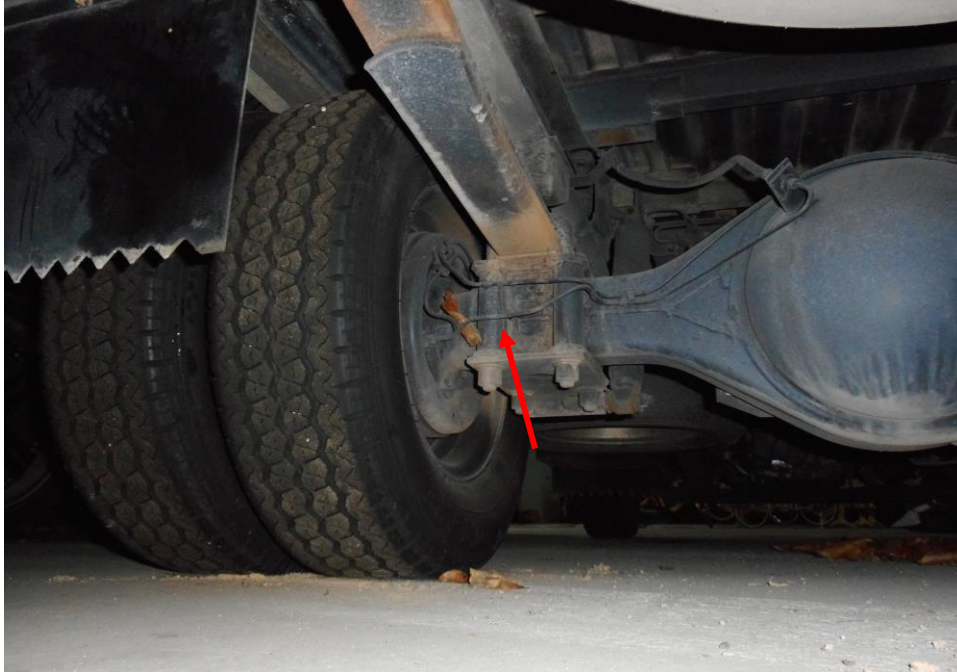
Photo 18 shows the brake pipe (arrowed) at the rear left wheel of the Motor Lorry. I did not observe any leakage of brake fluid at the time of my inspection of the Motor Lorry. My static tests of the Motor Lorry's braking system, along with my visual examination of the various mechanical components in the braking system, had indicated that there was no internal leakage of pressure/vacuum. Hence the braking system of the Motor Lorry was likely to be in serviceable condition at the material time of accident.
