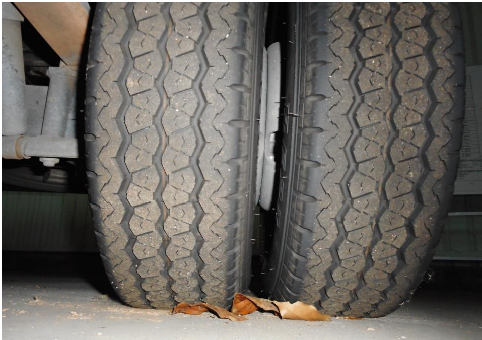
Photo 9 shows the condition of the rear left tyres of the Motor Lorry, which was observed to be in serviceable condition with remaining tread depth of approximately 6mm. The tyres, which were wrapped around standard alloy wheel rim, were also observed to be sufficiently inflated for vehicular operation. There was also no damage found on all 6 alloy wheel rims of the Motor Lorry.
