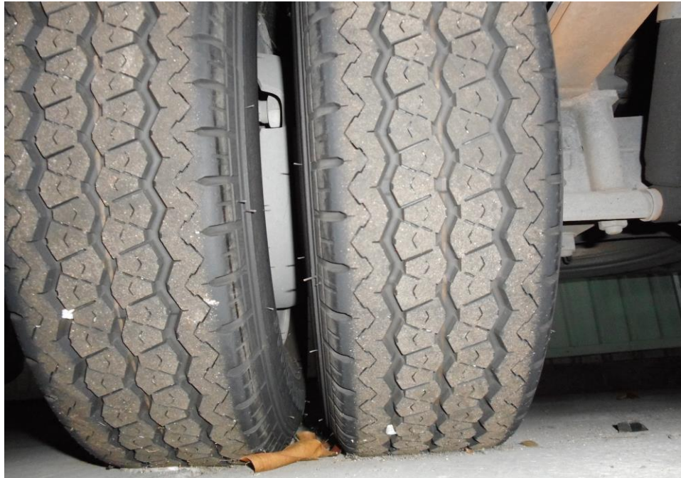
Photo 10 shows the condition of the rear right tyres of the Motor Lorry, which were observed to be in serviceable condition with remaining tread depth of approximately 5.9mm. There was also no tear, cut or burst mark(s) on the outer and the inner sidewalls as well as across the tread of the 6 tyres that were fitted on the Motor Lorry.
