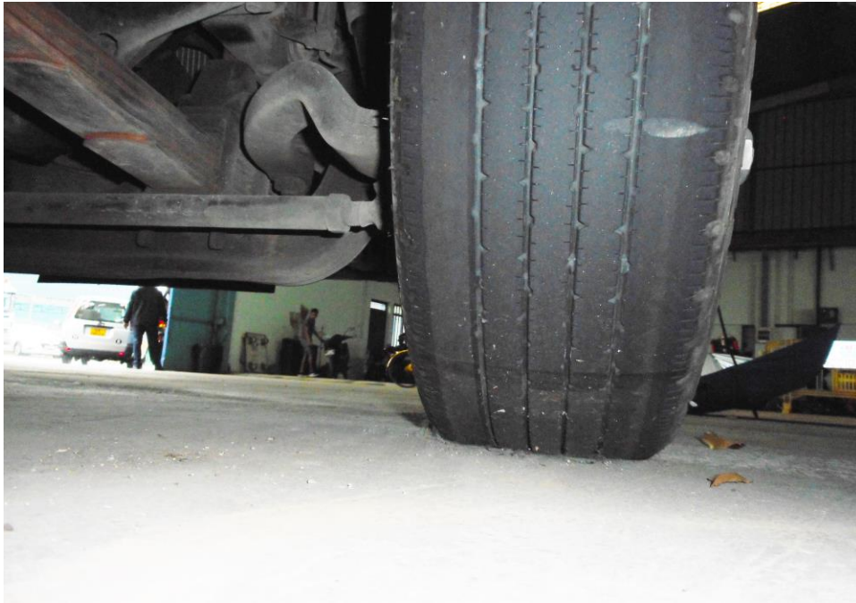
Photo 8 shows the condition of the front right tyre of the Motor Lorry, which was observed to be in serviceable condition with remaining tread depth of approximately 4.9mm. The tyre, which was wrapped around standard alloy wheel rim, was also observed to be sufficiently inflated for vehicular operation.
