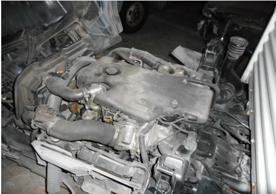
Photo 12 shows a general view of the Motor Lorry's engine compartment, which was accessed by lifting the front cabin of the Motor Lorry. The various parts and components inside the engine compartment were unaffected by the accident. There was also no sign(s) or indication(s) of fresh fluid leakage and/or fluid stain within the engine compartment (photograph shows the engine compartment as viewed from the front left side of the Motor Lorry).
