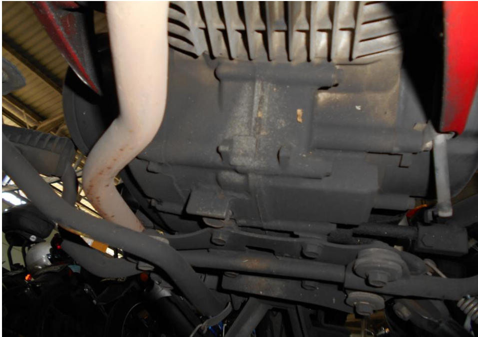
Photo 10 shows no sign(s) or indication(s) of fluid leak observed around the underside of the engine area of the Motorcycle.
