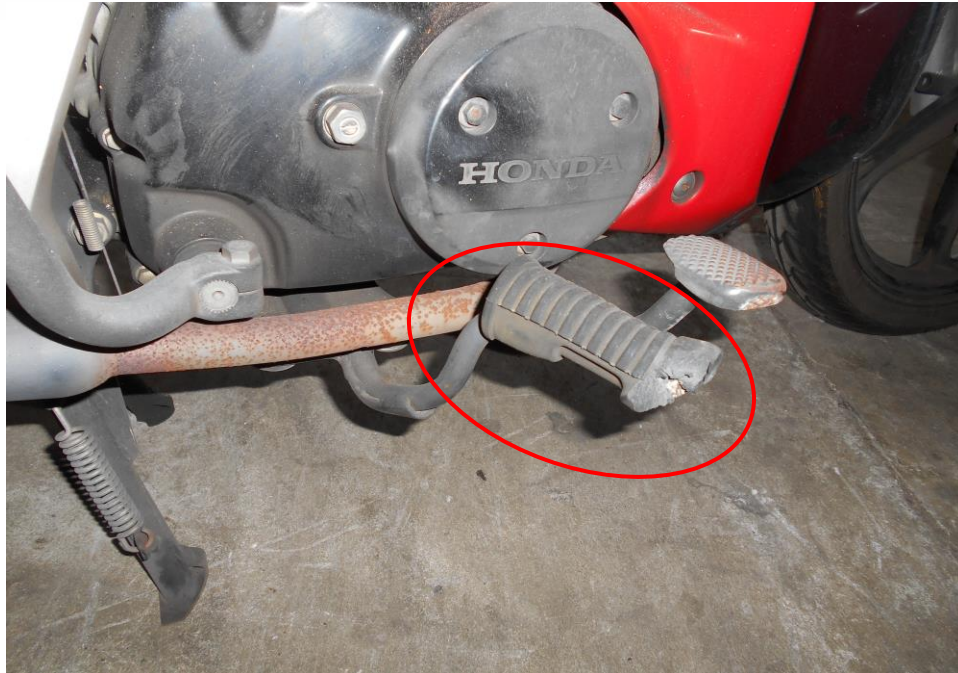
Photo 7 shows a closer view of the right rider's foot rest of the Motorcycle at the time of our inspection. The Motorcycle was observed to have sustained with relatively minor damages due to the accident collision. (Circled)
