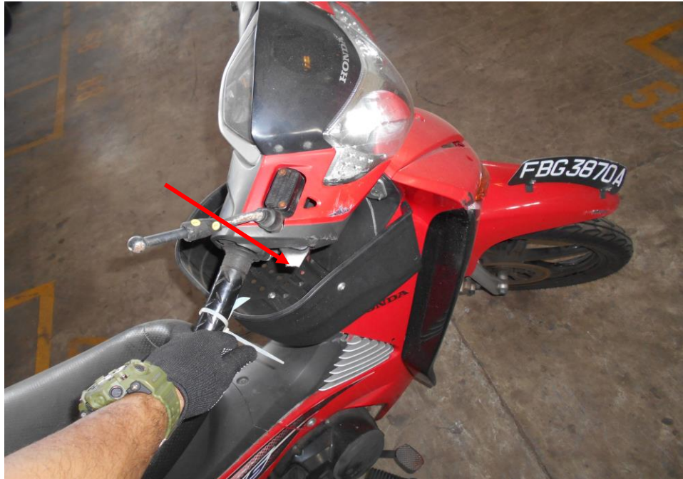
Photo 16 shows broken front brake lever as a result of the accident. This had disabled the static test on the front braking system.
