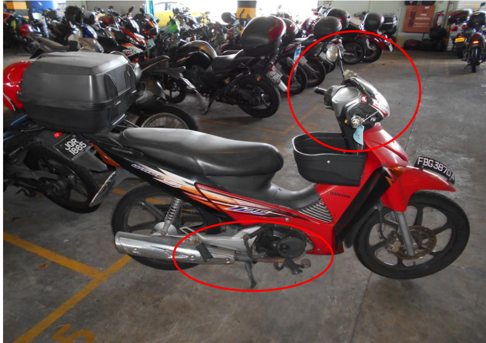
Photo 3 shows a general view of the right body of the Motorcycle at the time of our inspection. The Motorcycle was observed to have sustained relatively minor damages on the right side fairing, foot rest, handle, mud guard & brake lever at time of our inspection.
