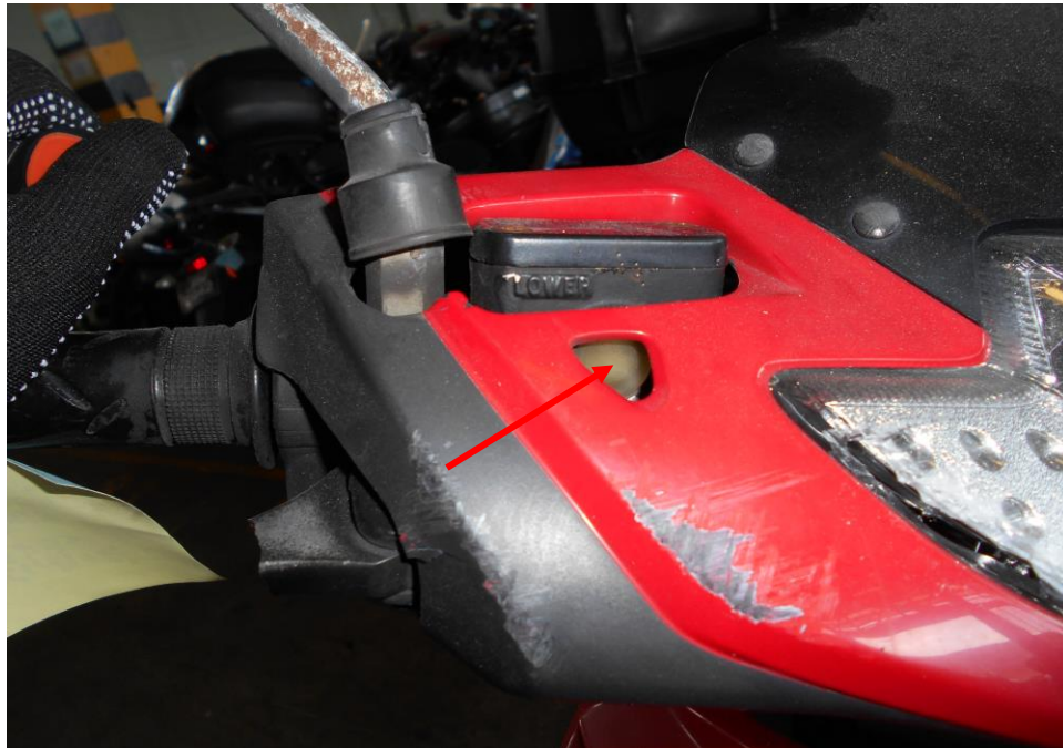
Photo 14 shows our checks on the brake fluid (front) reservoir had also indicated that the brake fluid was of sufficient level for operational purposes, and without contamination.
