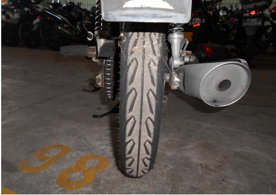
Photo 8 shows the rear tyre of the Motorcycle. The rear tyre was observed to be in serviceable condition with remaining tread depth of approximately 4mm. The tyre was also observed to be sufficiently inflated for vehicular operation.
