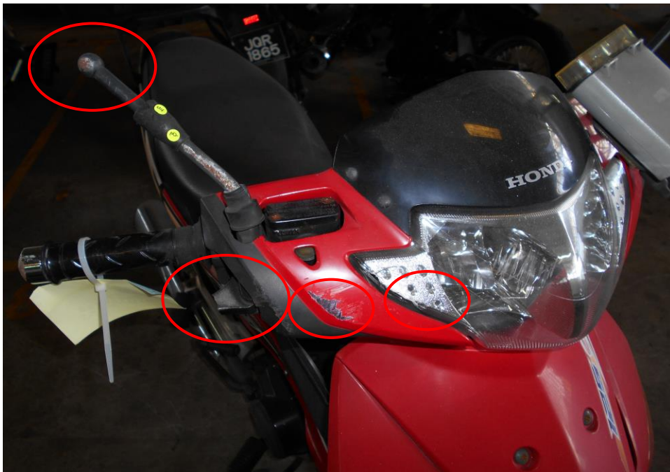
Photo 6 shows a closer view of the right damaged components of the Motorcycle at the time of our inspection. The Motorcycle was observed to have sustained with relatively minor damages due to the accident collision. (Circled)
