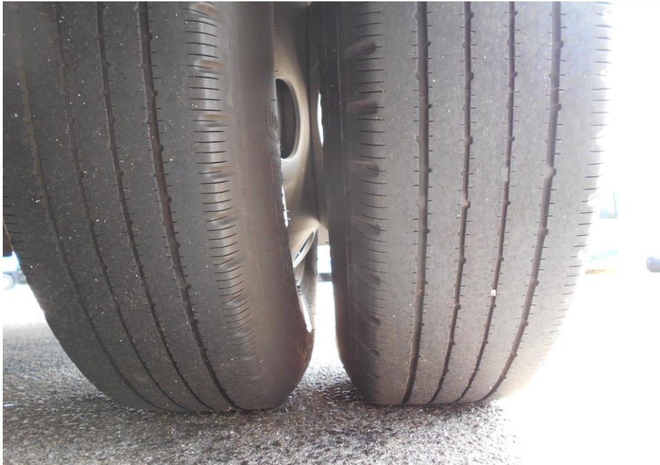
Photo 9 shows the condition of the rear left tyre of the Motor Bus, which was observed to be in serviceable condition with remaining tread depth of approximately 4mm. The tyre, which was wrapped around standard wheel rim, was also observed to be sufficiently inflated for vehicular operation. There was also no significant damage found on the 6 wheel rims of the Motor Bus.
