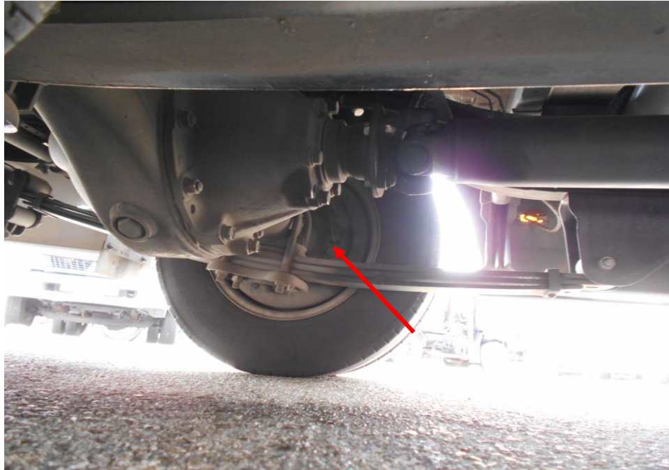
Photo 15 shows the various undercarriage components at the rear left wheel of the Motor Bus, in particular the brake hose (arrowed). We did not observe any leakage of brake fluid at the time of our inspection of the Motor Bus.
