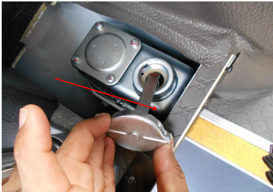
Photo 13 shows the power steering fluid of the Motor Bus at the time of our inspection. It was observed to be of sufficient level and without any visible contamination.
