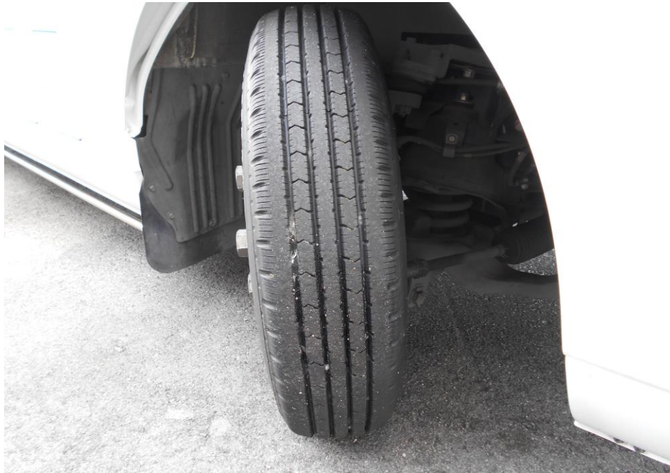
Photo 7 shows the condition of the front right tyre of the Motor Bus, which was observed to be in serviceable condition with remaining tread depth of approximately 8mm. The tyres were all observed to be sufficiently inflated for vehicular operation with no tear, cut or burst mark(s) on the outer and the inner sidewalls as well as across the tread.
