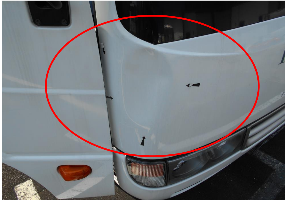
Photo 3 shows a close-up view of the damages on the front right panel of the Motor Bus at the time of our inspection. It was likely due to the accident's impact collision.
