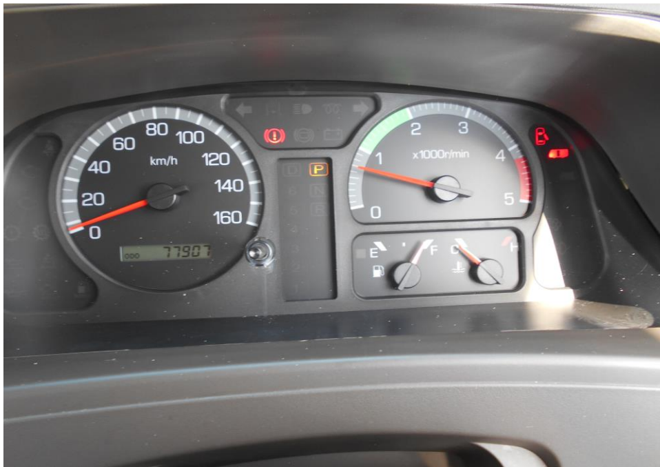
Photo 20 shows no warning lights illuminated on the instrument panel of the Motor Bus after the engine was cranked. This would suggest that there was no abnormality to the various electronic operating systems of the Motor Car.
