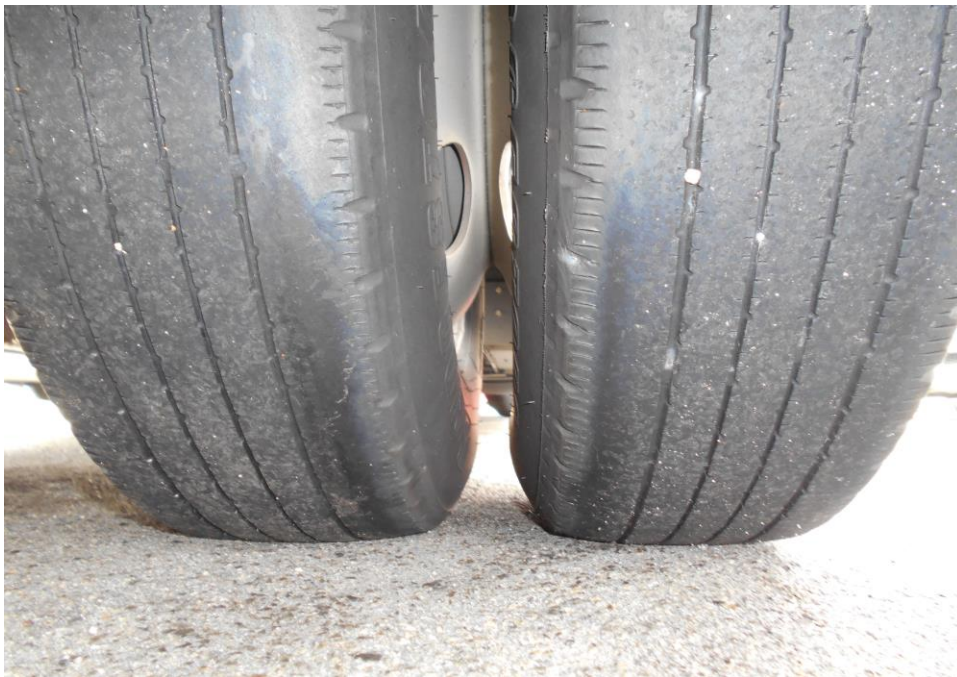
Photo 10 shows the condition of the rear right tyre of the Motor Bus, which was observed to be in serviceable condition with remaining tread depth of approximately 3mm. There was also no tear, cut or burst mark(s) on the outer and the inner sidewalls as well as across the tread of the tyre, which was also sufficiently inflated for vehicular operation.
