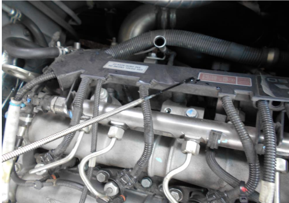
Photo 14 shows the engine dip stick of the Motor Bus at the time of our inspection. The engine oil was observed to be of sufficient level and without any visible contamination.
