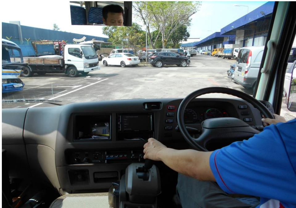
Photo 22 shows a short operational test of the Motor Bus, the test was conducted by driving the Motor Bus forward, stopping, before reversing and coming to a stop again.
