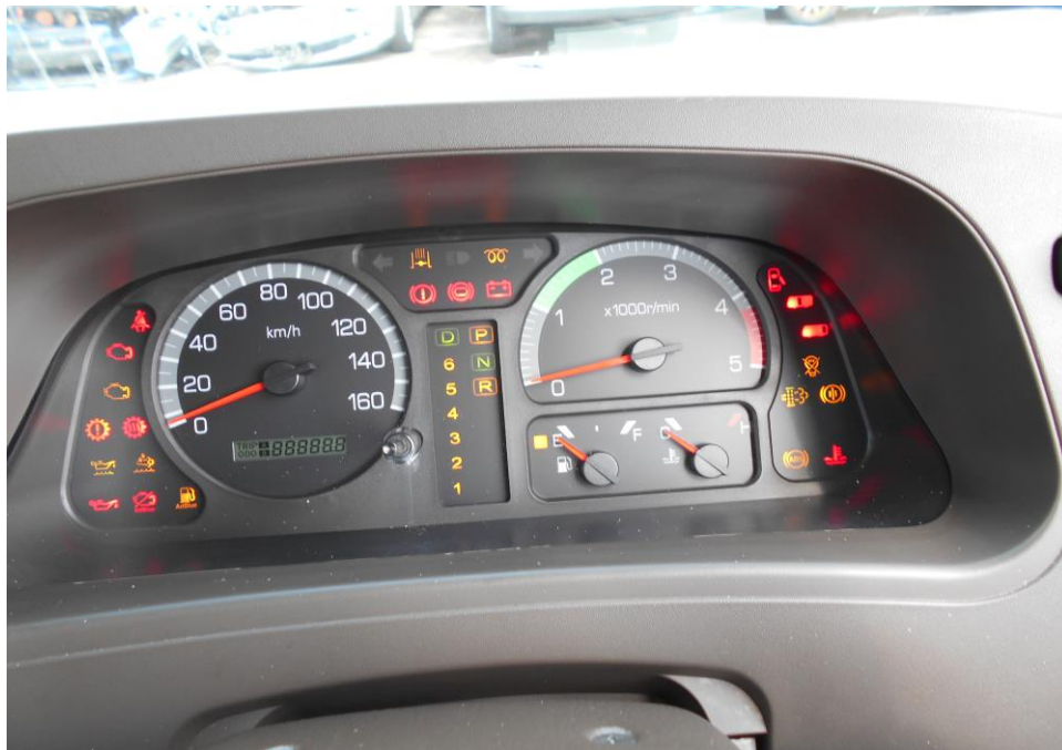
Photo 19 shows the warning lights for the various electronic operating systems of the Motor Bus appearing on its instrument panel during the self-test when the engine was cranked.
