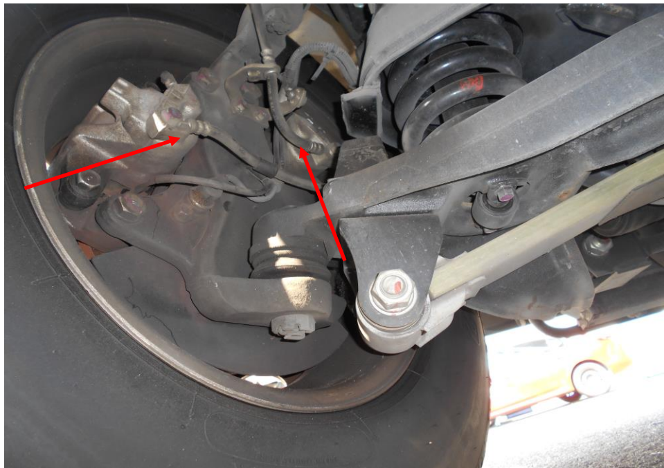
Photo 16 shows the brake hose at the front left wheel of the Motor Bus. We did not observe any leakage of brake fluid. Our visual inspection of the various mechanical components of the Motor Bus's braking system revealed all to be intact and without visible damage, indicating that the braking system was likely to be in serviceable condition at the material time of accident.
