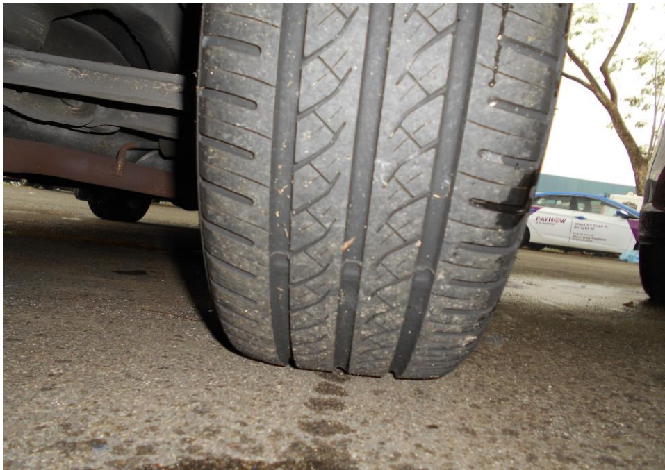
Photo 11 shows the condition of the rear right tyre of the Motor Car, which was observed to be in serviceable condition with remaining tread depth of approximately 5mm. There was also no tear, cut or burst mark(s) on the outer and the inner sidewalls as well as across the tread of the 4 tyres.
