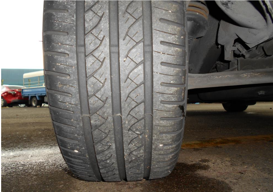
Photo 10 shows the condition of the rear left tyre of the Motor Car, which was observed to be in serviceable condition with remaining tread depth of approximately 5mm. The tyre, which was wrapped around alloy wheel rim, was also observed to be sufficiently inflated for vehicular operation.
