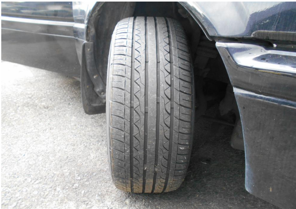
Photo 9 shows the condition of the front right tyre of the Motor Car, which was observed to be in serviceable condition with remaining tread depth of approximately 5mm. The tyre, which was wrapped around alloy wheel rim, was also observed to be sufficiently inflated for vehicular operation.
