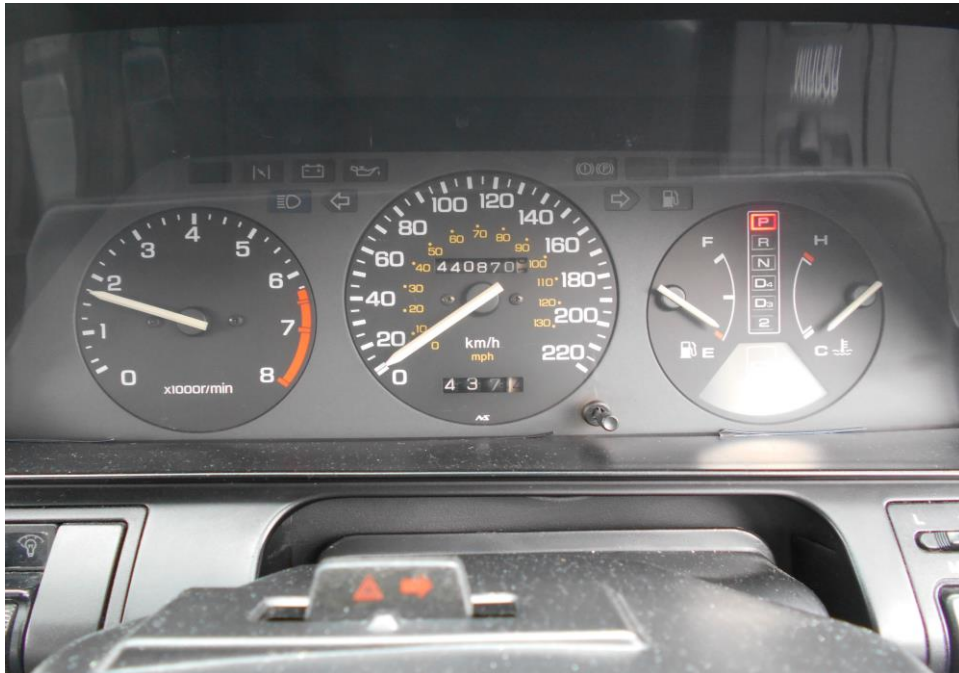
Photo 22 shows no warning lights illuminated on the instrument panel of the Motor Car after the engine was cranked. This would suggest that there was no abnormality to the various electronic operating systems of the Motor Car.
