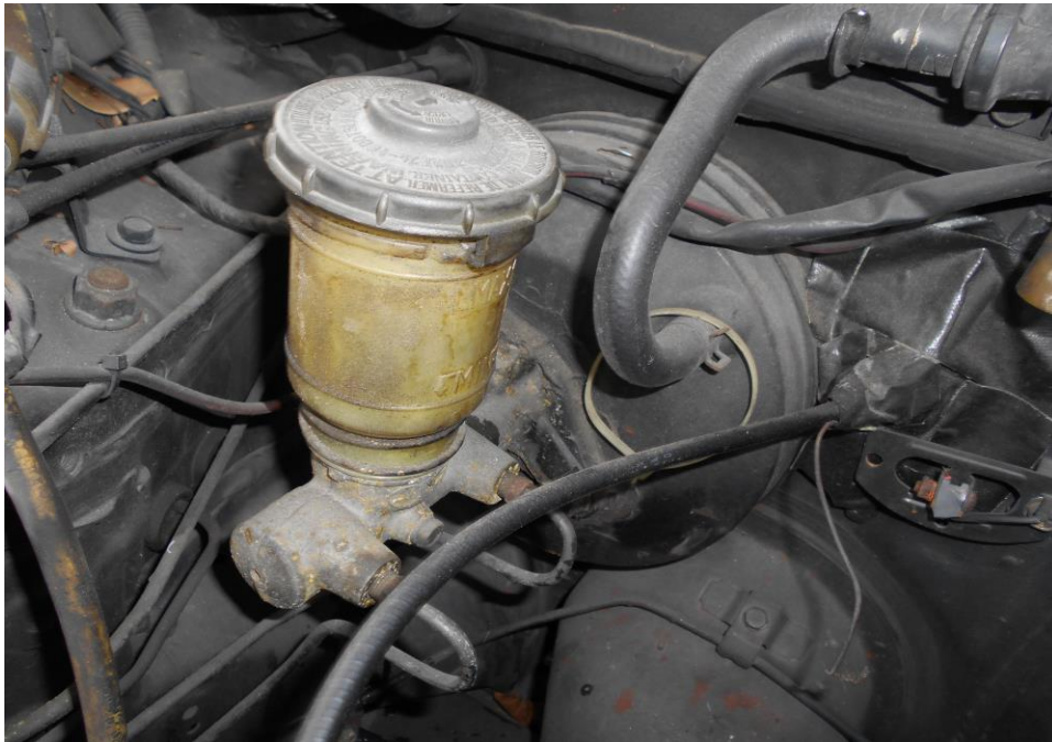
Photo 13 shows the brake fluid reservoir of the Motor Car at the time of our inspection. The brake fluid was observed to be empty at time of our inspection.
