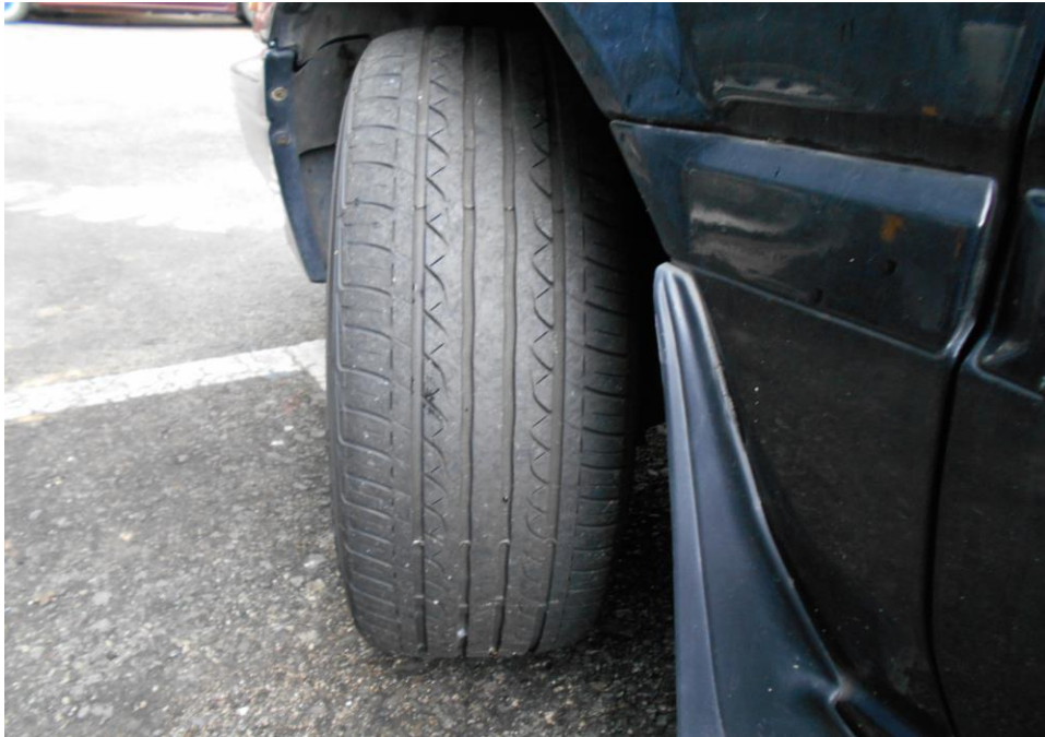
Photo 8 shows the condition of the front left tyre of the Motor Car, which was observed to be in serviceable condition with remaining tread depth of approximately 4mm. The tyre, which was wrapped around alloy wheel rim, was also observed to be sufficiently inflated for vehicular operation. There was no tear, cut or burst mark(s) on the outer and the inner sidewalls as well as across the tread of the 4 tyres.
