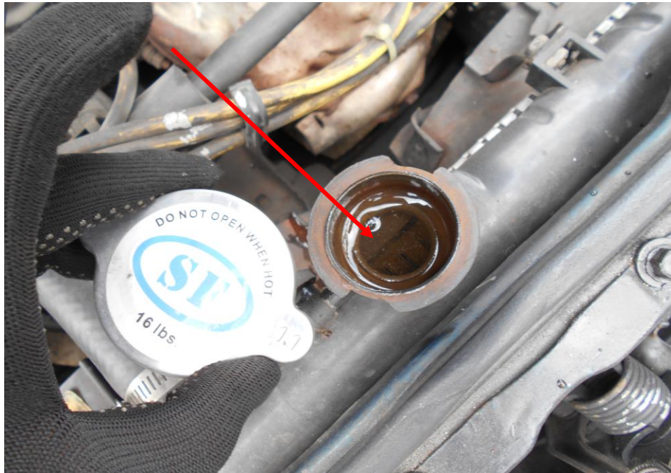
Photo 15 shows the coolant fluid reservoir of the Motor Car at the time of our inspection. The coolant fluid was observed to be of sufficient level and without any visible contamination.
