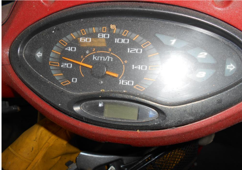
Photo 1 shows a close-up view of the mileage meter at time of our inspection. It was unable to be operated likely due to the accident's impact which affects the ignition system.
