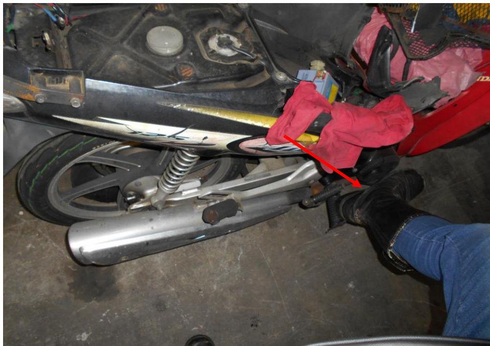
Photo 16 shows testing of the braking of the rear brake in progress. There was some resistance felt (spongy like feel) upon stepping on the brake pedal.
