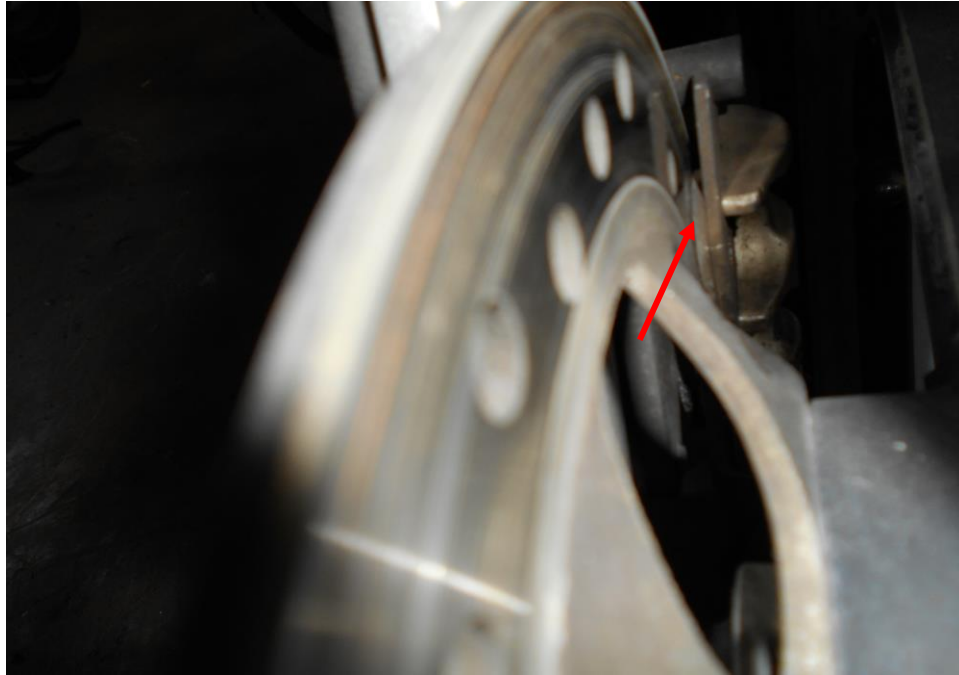
Photo 17 shows the front brake pad at time of our inspection. The frictional material was observed to be sufficient for operational purposes.
