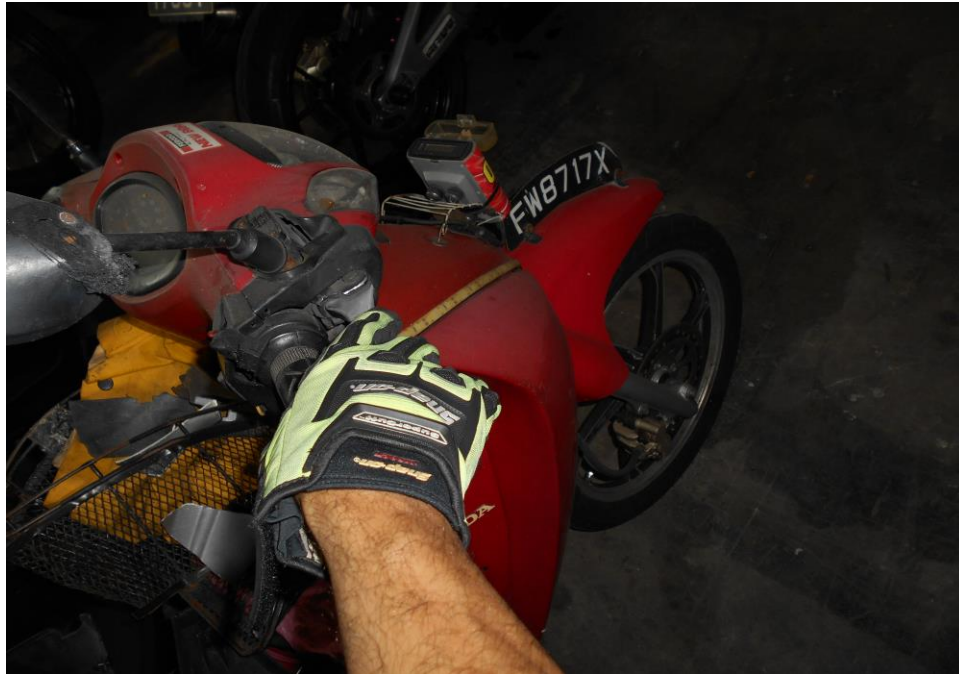
Photo 15 shows testing of the braking of the front brake in progress. There was some resistance felt (spongy like feel) upon pressing the brake lever.
