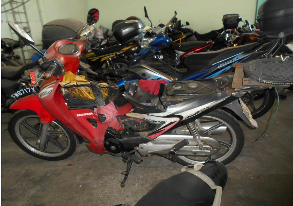
Photo 5 shows a general view of the left body of the Motorcycle at the time of our inspection. The Motorcycle was observed to have sustained relatively minor damages on the left side of the Motor Cycle at time of our inspection.
