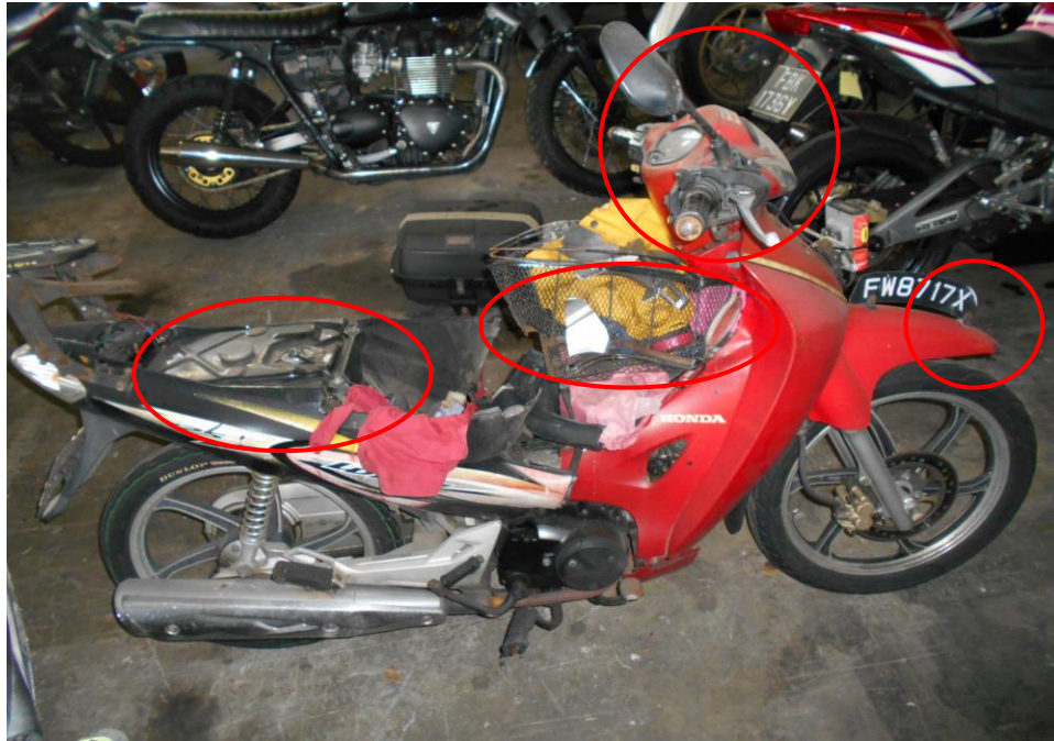
Photo 3 shows a general view of the right body of the Motorcycle at the time of our inspection. The Motorcycle was observed to have sustained relatively minor damages on the right side of the Motor Cycle at time of our inspection.
