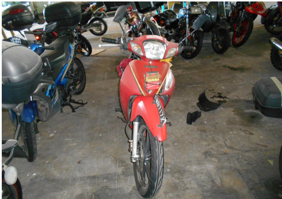
Photo 2 shows a general view of the front body of the Motorcycle at the time of our inspection. The Motorcycle was observed to have sustained relatively minor damages at time of inspection. The damages were observed to be confined to its frontal, left & right side of the Motor Cycle.
