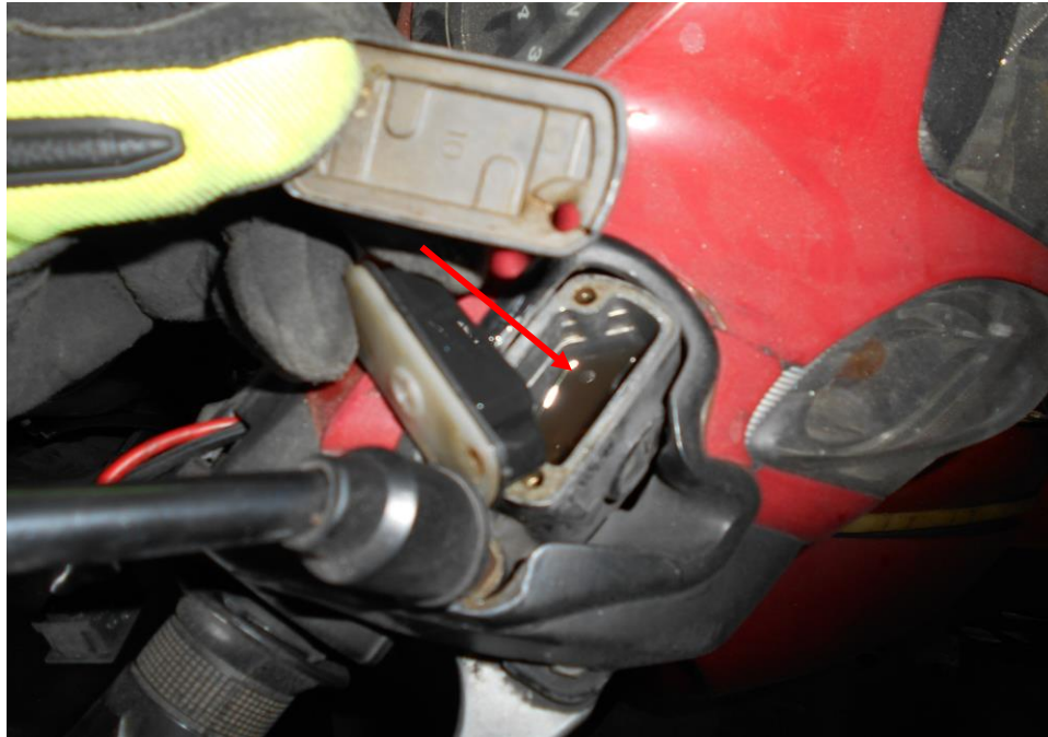
Photo 13 shows our checks on the brake fluid (front) reservoir had also indicated that the brake fluid was of sufficient level for operational purposes, and without contamination.
