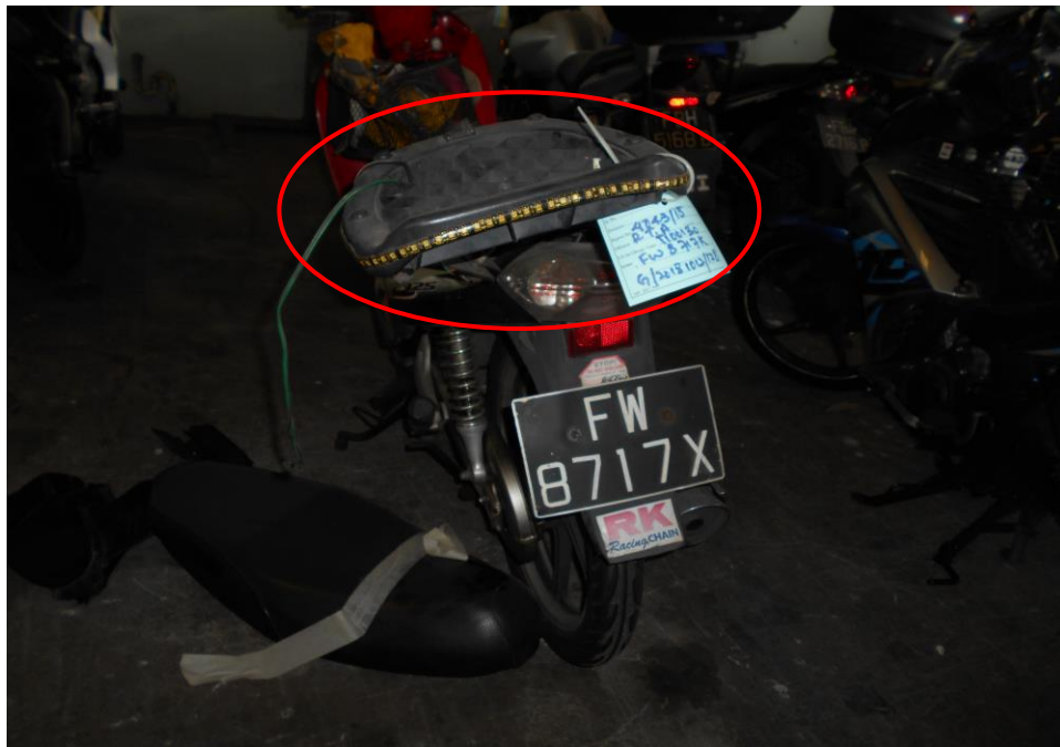
Photo 4 shows a general view of the rear body of the Motorcycle at the time of our inspection. The Motorcycle was observed to have sustained relatively minor damage on the rear compartment bracket at time of our inspection.
