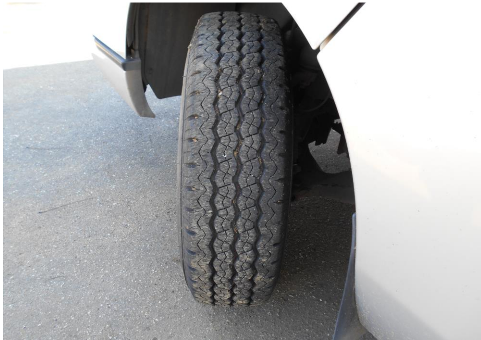
Photo 8 shows the condition of the front left tyre of the Motor Bus, which was observed to be in serviceable condition with remaining tread depth of approximately 8mm. The tyre, which was wrapped around standard wheel rim, was also observed to be sufficiently inflated for vehicular operation.
