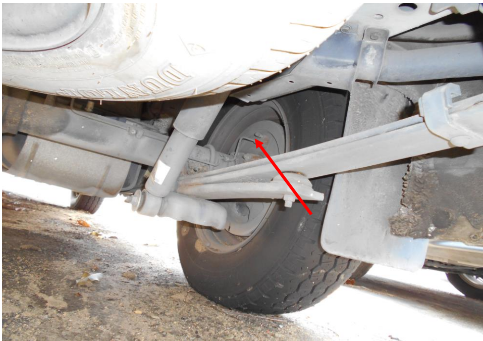
Photo 18 shows the various undercarriage components at the rear right wheel of the Motor Bus. The various steering components were all found to be intact, suggesting that the steering system of the Motor Bus was likely to be in serviceable condition at the material time of accident. There was also no sign of fluid stain(s) observed on the various undercarriage components at the 4 wheels of the Motor Van.
