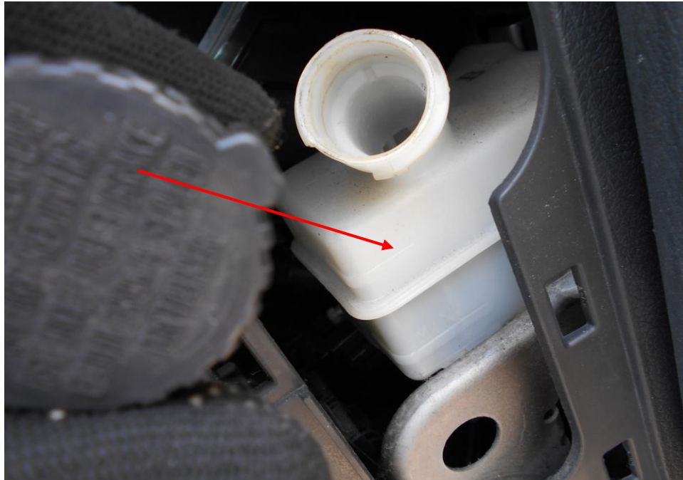
Photo 12 shows the brake fluid reservoir of the Motor Bus at the time of our inspection. The brake fluid was observed to be of sufficient level and without any visible contamination.
