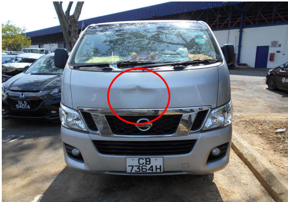
Photo 2 shows a general view of the front body of the Motor Bus at the time of our inspection. The Motor Bus was observed to sustained damages at the front centre portion due to the accident's impact.
