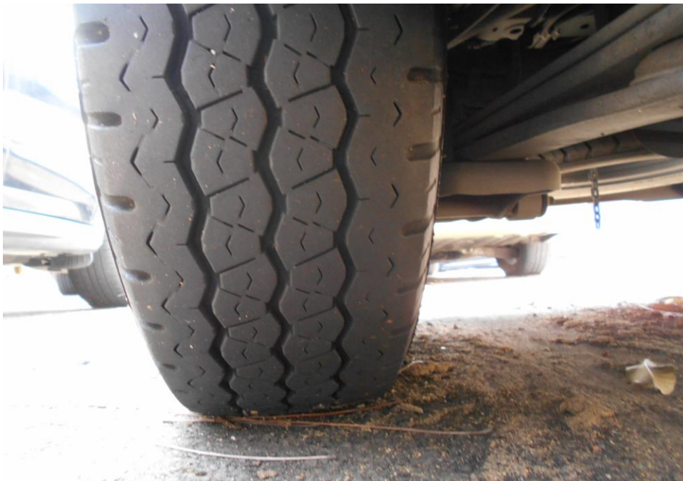
Photo 10 shows the condition of the rear right tyre of the Motor Bus, which was observed to be in serviceable condition with remaining tread depth of approximately 7mm. There was also no tear, cut or burst mark(s) on the outer and the inner sidewalls as well as across the tread of the tyre, which was also sufficiently inflated for vehicular operation.
