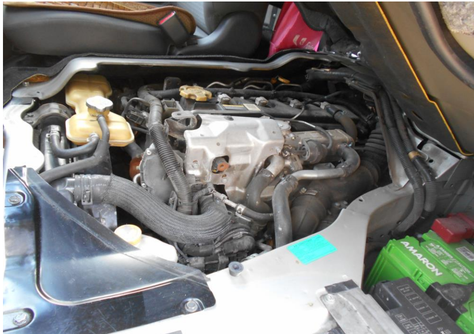
Photo 11 shows a general view of the Motor Bus's engine compartment. The various parts and components inside the engine compartment were unaffected by the accident. There was also no sign(s) or indication(s) of fluid leakage and/or fluid stain within the engine compartment.
