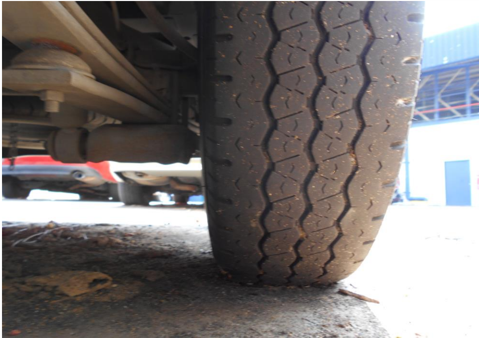
Photo 9 shows the condition of the rear left tyre of the Motor Bus, which was observed to be in serviceable condition with remaining tread depth of approximately 6mm. The tyre, which was wrapped around standard wheel rim, was also observed to be sufficiently inflated for vehicular operation. There was also no significant damage found on the 6 wheel rims of the Motor Bus.
