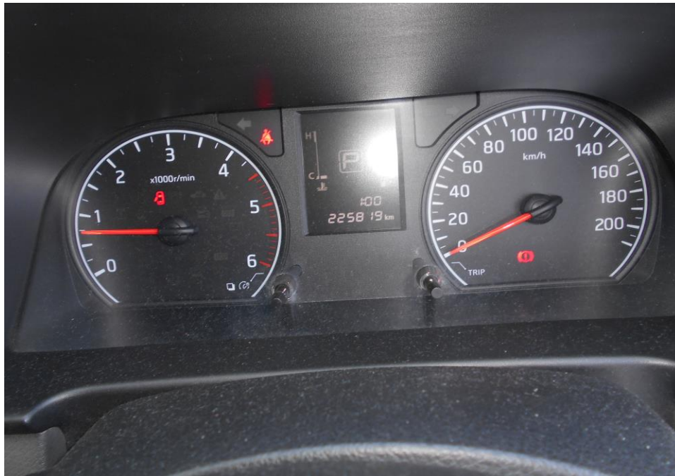
Photo 20 shows no warning lights illuminated on the instrument panel of the Motor Bus after the engine was cranked. This would suggest that there was no abnormality to the various electronic operating systems of the Motor Bus.
