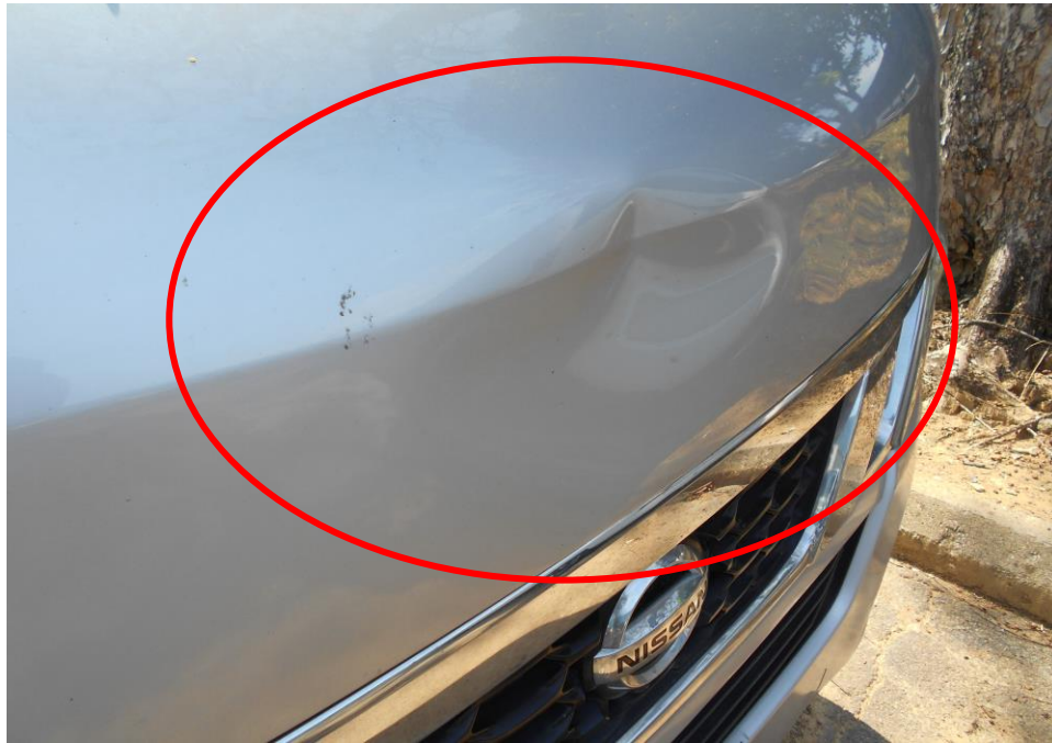
Photo 3 shows a close-up view of the damages on the front centre panel of the Motor Bus at the time of our inspection. It was likely due to the accident's impact collision.
