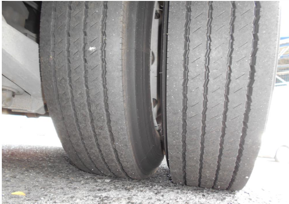
Photo 10 shows the condition of the rear left tyres of the Motor Bus, which were observed to be in serviceable condition with remaining tread depth of approximately 8mm. The tyres, which were wrapped around standard alloy wheel rims, were also observed to be sufficiently inflated for vehicular operation.
