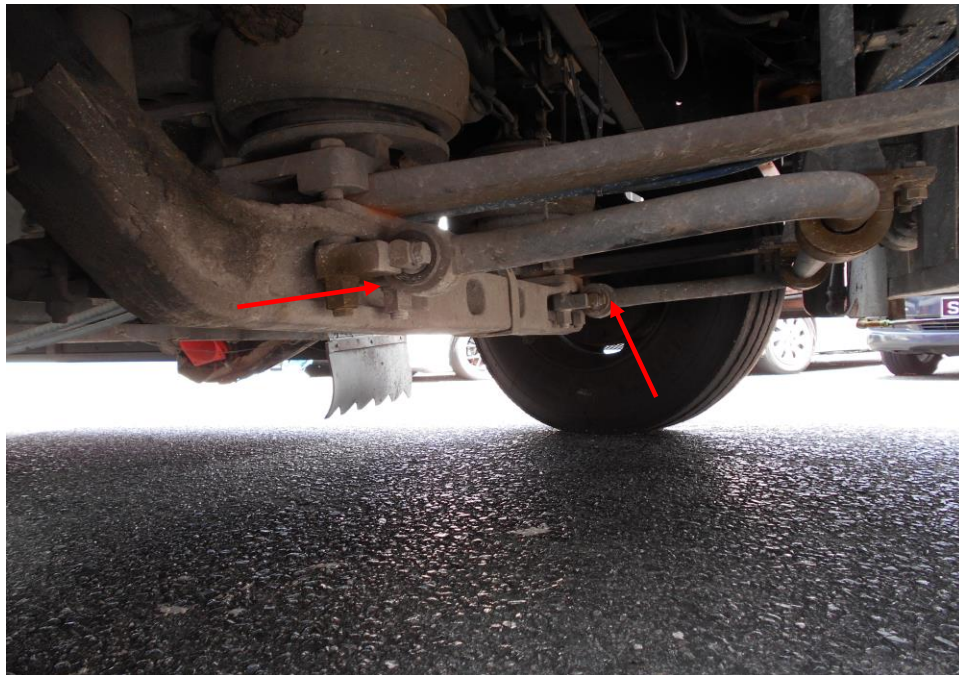
Photo 15 shows some of the mechanical components (arrowed) of the Motor Bus's steering system. Our visual check on the various mechanical components of the steering system revealed all to be intact and in good condition. The steering system of the Motor Bus likely to be in serviceable condition at the time of accident.
