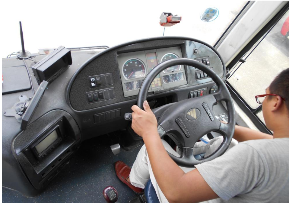
Photo 22 shows the bus driver while conducting the operational test. He was able to steer to the fullest left & right, moving forward, reverse and stop successfully at time of the operational test.
