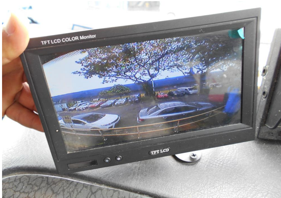
Photo 24 shows the reverse camera monitor which was installed in front the driver's seat for viewing rear portion while reversing the Motor Bus.
