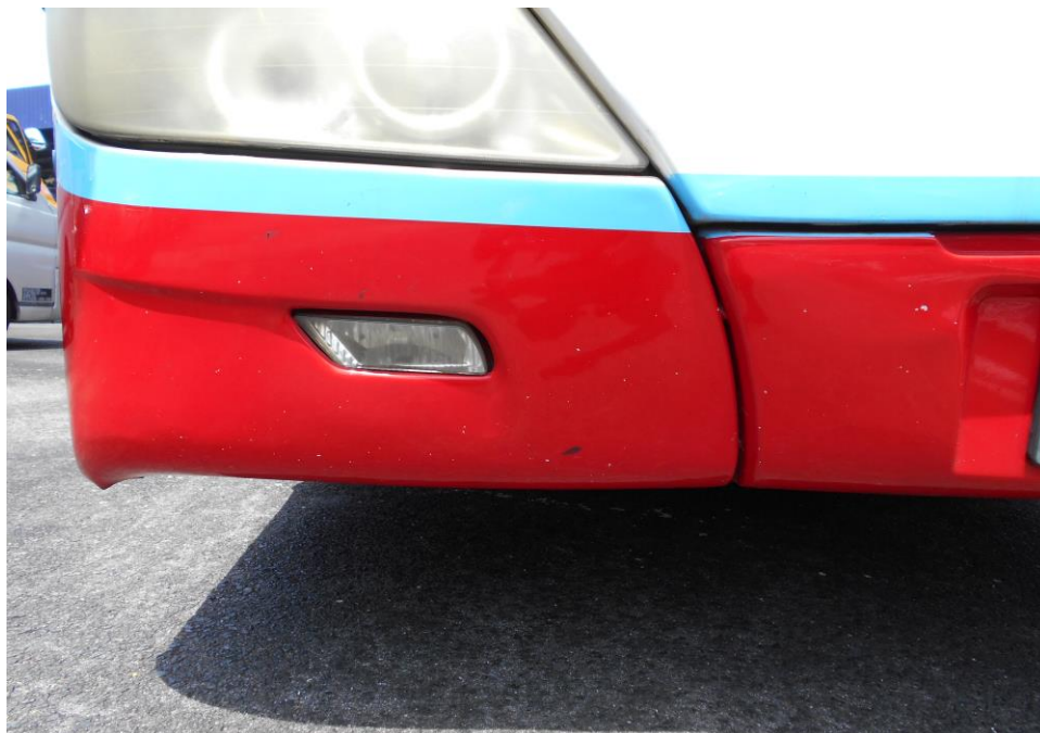
Photo 4 shows a close-up view of the front right lower bumper of the Motor Bus at the time of our inspection. The Motor Bus front right lower bumper was observed to sustained slight dent due to the accident's impact.
