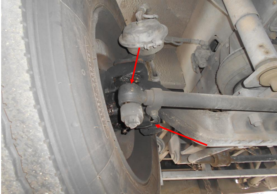
Photo 16 shows the front left wheel components of the front steering system of the Motor Bus. The various undercarriage components of the Motor Bus were all observed to be intact and without any visible damage. This had included the steering rack and steering ball joints (arrowed) of the Motor Bus, which were observed to be securely attached to the front left wheel and front right wheel.
