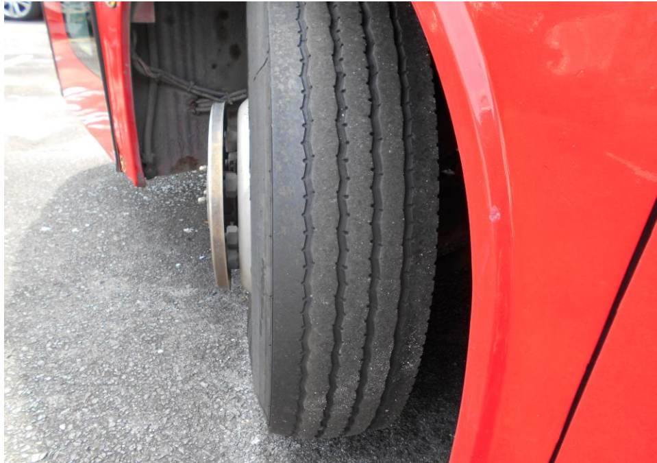
Photo 8 shows the condition of the front left tyre of the Motor Bus, which was observed to be in serviceable condition with remaining tread depth of approximately 7mm. The tyre was also observed to be sufficiently inflated for vehicular operation.
