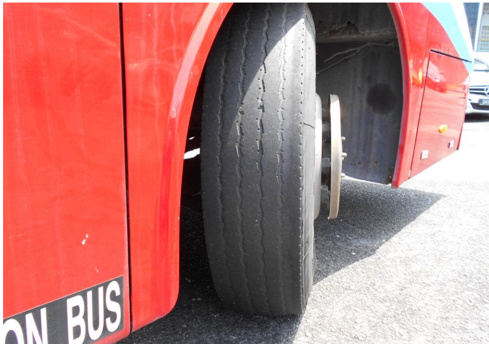
Photo 7 shows the condition of the front right tyre of the Motor Bus, which was observed to be in serviceable condition with remaining tread depth of approximately 2mm. The tyre was also observed to be sufficiently inflated for vehicular operation.
