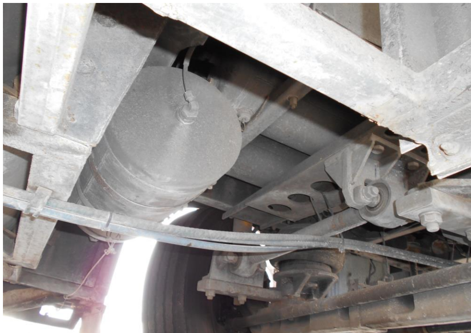
Photo 19 shows a general view of the air tank, valves, pipes and hoses, which are some of the components for the air-assisted braking system of the Motor Bus. This was at the underside of the Motor Bus's body. There were no damages observed at time of our inspection.
