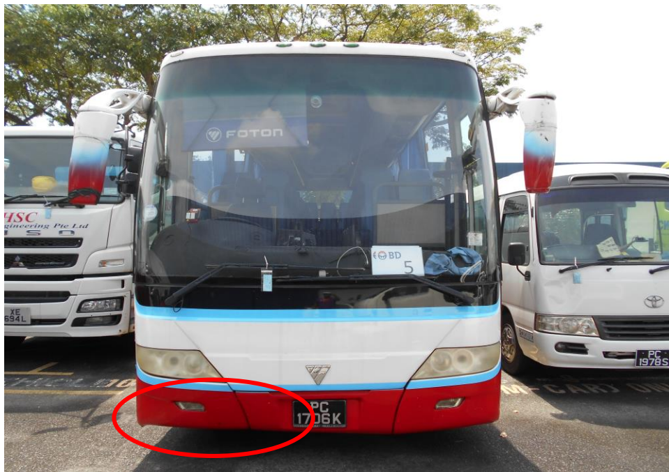
Photo 2 shows a general view of the front body of the Motor Bus at the time of our inspection. The Motor Bus was observed to have sustained minor damage at its front lower right portion as a result of the accident's collision.
