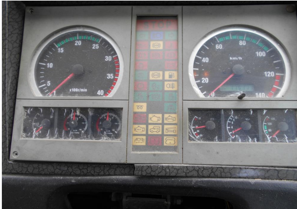
Photo 21 shows the indicators at the driver's seat, these systems were in working condition. This can be established from the warning lights disappearing from the instrument panel after the self-test.
