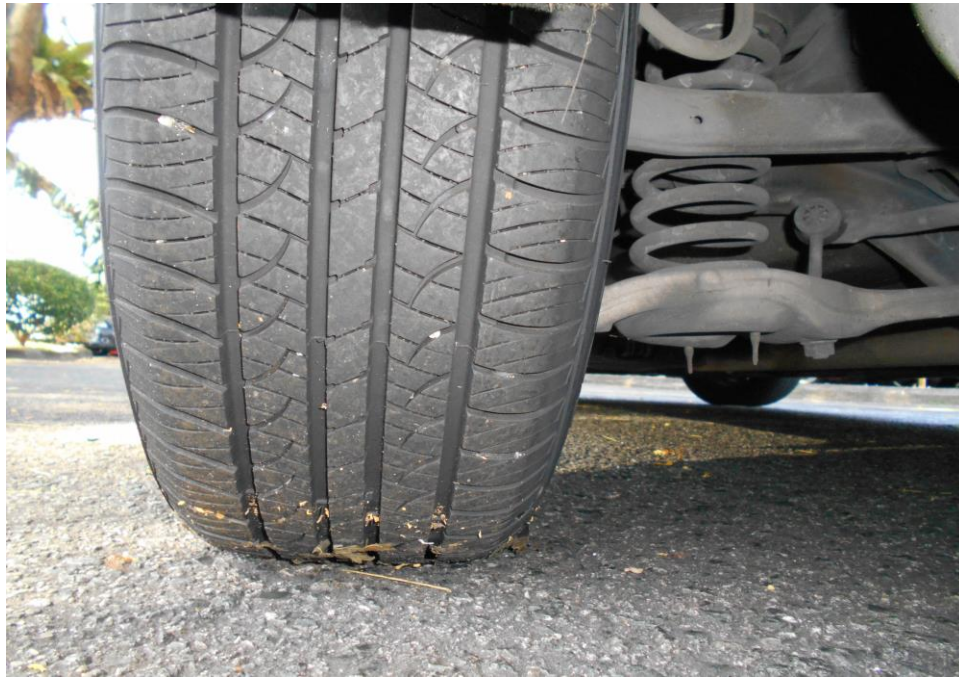
Photo 11 shows the condition of the rear left tyre of the Motor Taxi, which was observed to be in serviceable condition with remaining tread depth of approximately 6mm.
