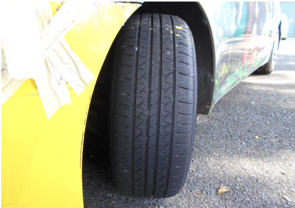
Photo 10 shows the condition of the front left tyre of the Motor Taxi, which was observed to be in serviceable condition with remaining tread depth of approximately 5mm. The tyre, which was wrapped around alloy wheel rim, was also observed to be sufficiently inflated for vehicular operation.
