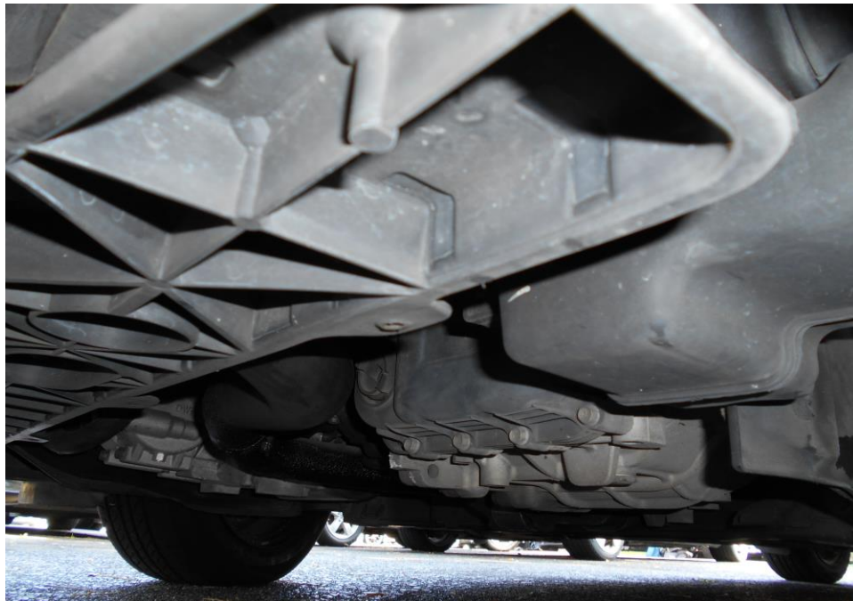
Photo 17 shows the engine underside of the Motor Taxi engine. The engine was observed to be free from fluid leakage at time of our inspection.
