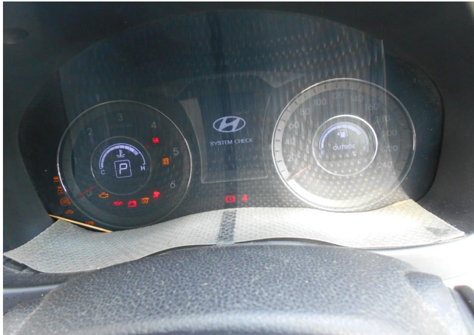
Photo 22 shows the warning lights for the various electronic operating systems of the Motor Taxi appearing on its instrument panel during the self-test when the engine is cranked, in particular the ABS light, SRS light, engine check light, battery light and diesel glow plug amongst others.
