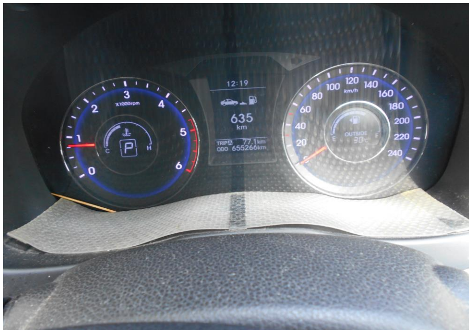
Photo 23 shows no warning lights illuminated on the instrument panel of the Motor Taxi after the engine was cranked. This would suggest that there was no abnormality to the various electronic operating systems of the Motor Taxi, like the ABS light engine check light, battery light and diesel glow plug.
