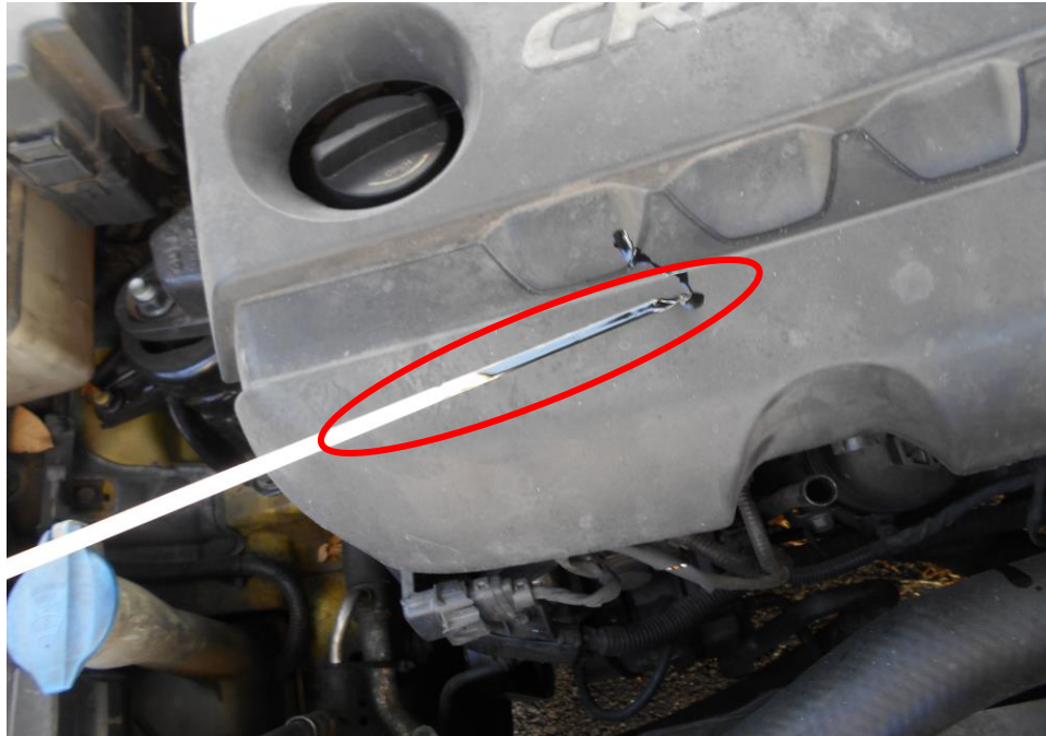
Photo 16 shows the engine oil dip stick of the Motor Taxi at the time of our inspection. The engine oil was observed to be of sufficient level and without any visible contamination.
