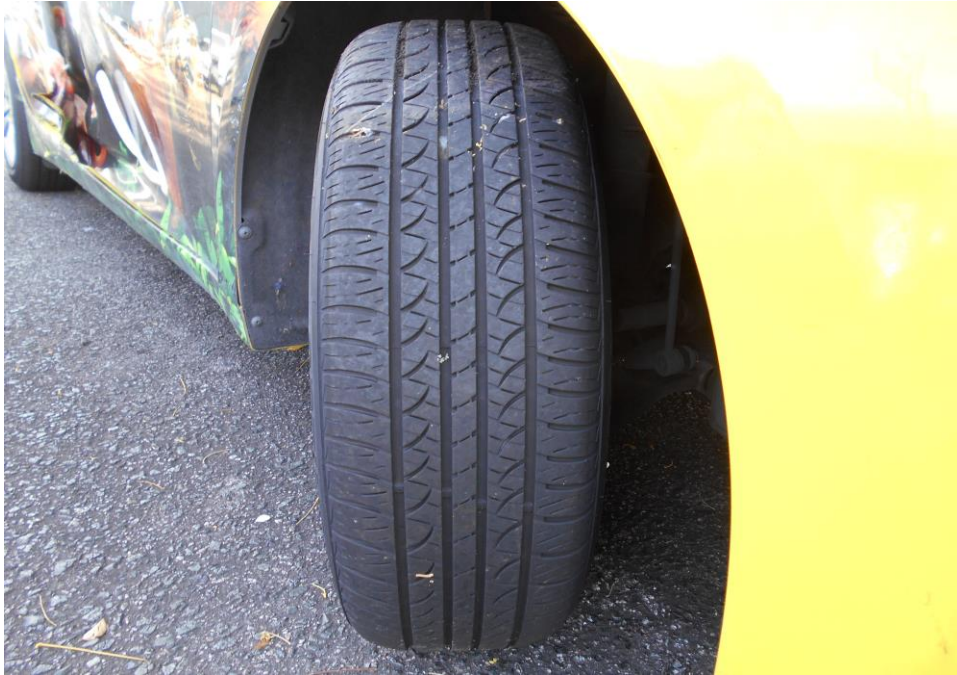
Photo 9 shows the condition of the front right tyre of the Motor Taxi, which was observed to be in serviceable condition with remaining tread depth of approximately 5mm. There was no tear, cut or burst mark(s) on the outer and the inner sidewalls.
