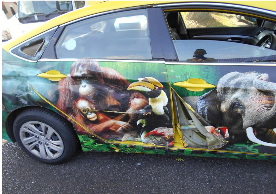
Photo 7 shows a semi close up view of the driver and passenger's door, rear quarter glass of the Motor Taxi at the time of our inspection. It had sustained damages likely due to the accident.
