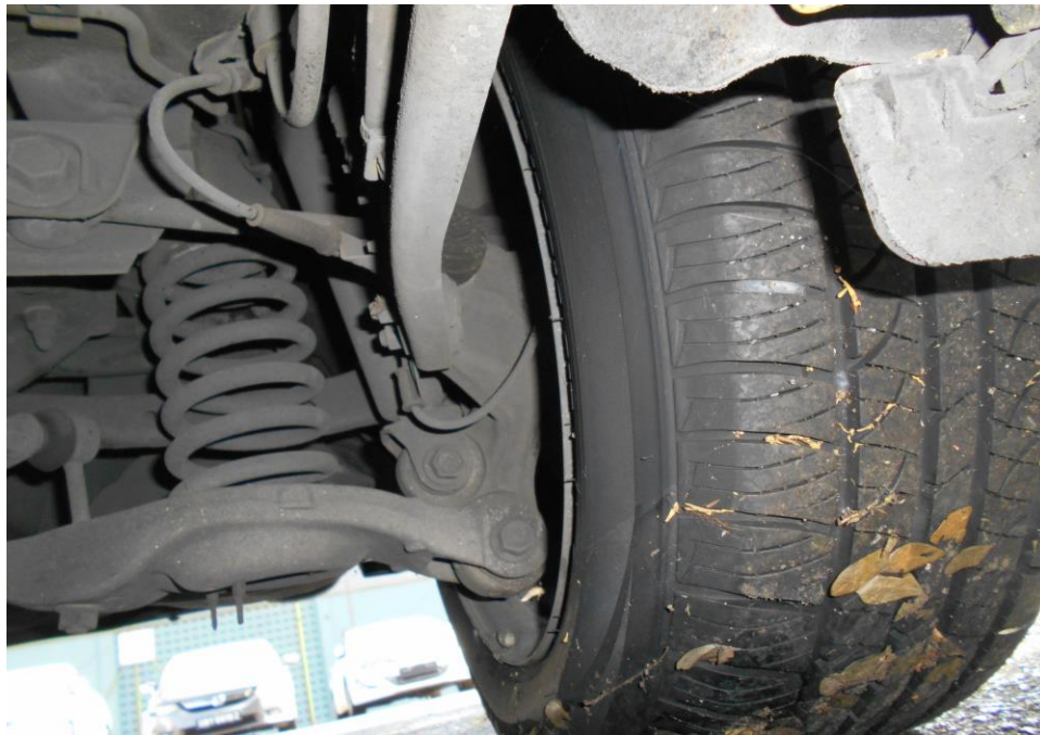
Photo 18 shows the rear left wheel of the Motor Taxi. We did not observe any leakage of brake fluid at the time of our inspection of the Motor Taxi. Our visual inspection of the various mechanical components of the Motor Taxi's braking system revealed all to be intact without visible damage.
