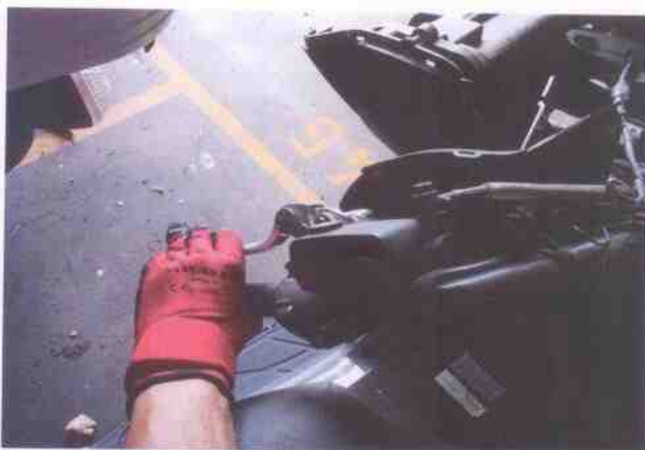
Photo 15 shows the steering system was observed to be in a serviceable condition. It was able to be steered to the full left & right at time of our inspection.
