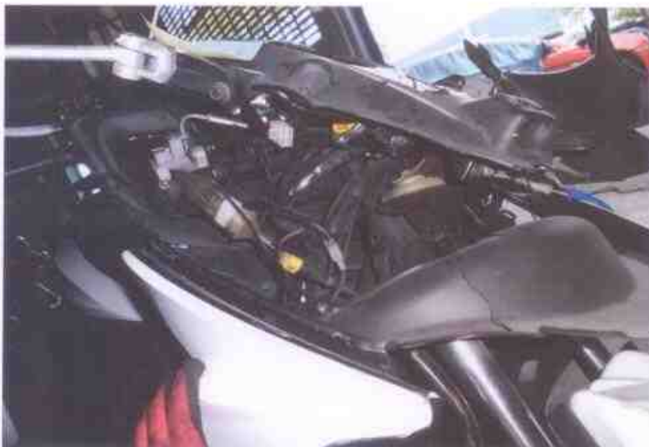
Photo 6 shows a close-up view of the frontal portion of the Motorcycle at the time of our inspection was observed to have sustained dislodged outer front fairing cover due to the accident collision. (Circled)
