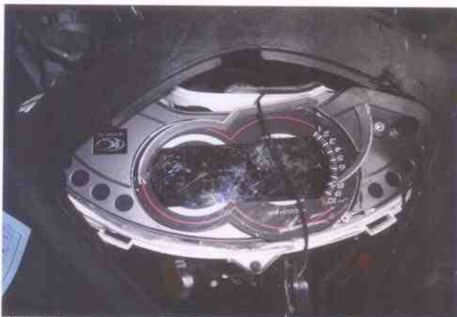
Photo 1 shows a close-up view of the speedometer of the Motorcycle at the time of our inspection. It was observed to have sustained with damages due to the accident collision.
