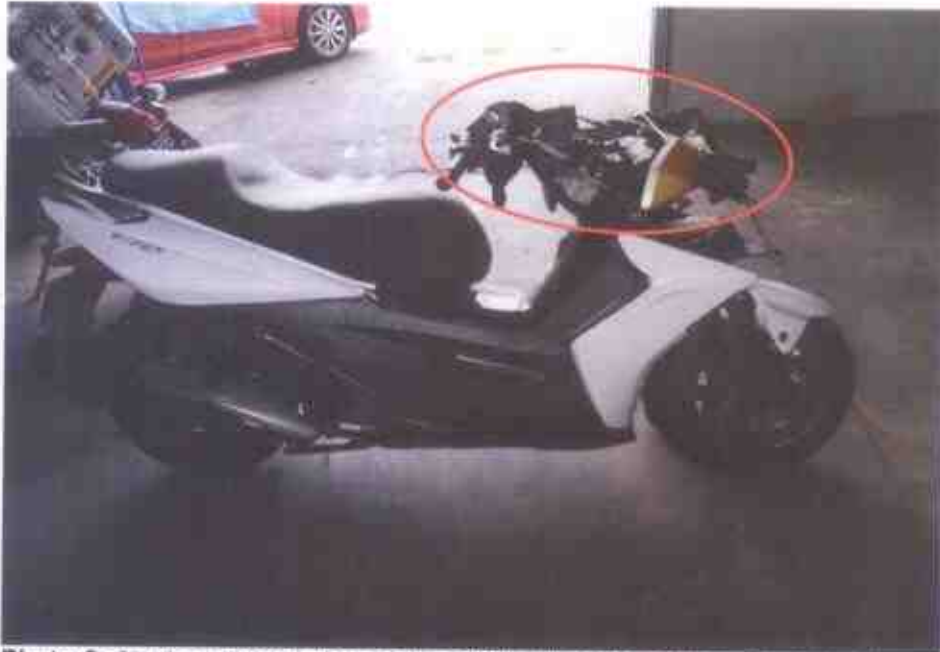
Photo 2 shows a general view of the right body of the Motorcycle at the time of our inspection. The Motorcycle frontal portion was observed to have sustained with damages due to the accident collision. (Circled)
