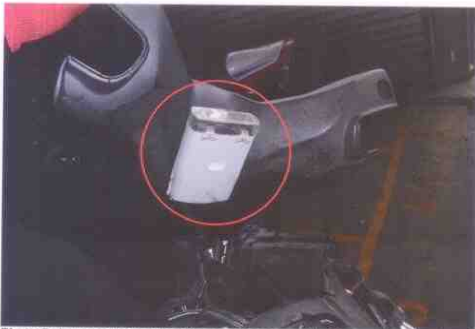
Photo 5 shows a closer view of the frontal portion of the Motorcycle at the time of our inspection. The Motorcycle was observed to have sustained dislodged In-Vehicle unit due to the accident collision. (Circled)
