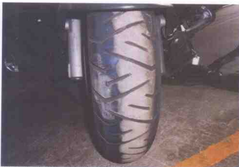
Photo 11 shows the front tyre of the Motorcycle. The pattern of the tread was clearly visible with remaining tread depth of approximately 3mm. There was no tear, burst mark(s) and/or punctured hole(s) on the sidewalls as well as across the tread of the front tyre.
