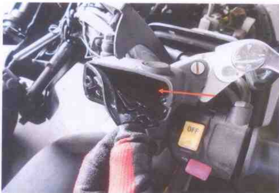
Photo 18 shows the brake fluid reservoir for front wheel brake on the right hand was noted to be of sufficient level for operational purposes, and without contamination.
