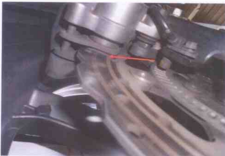
Photo 19 shows the brake pad for front wheel brake of the Motorcycle. The frictional material was observed to be at an adequately sufficient level at time of our inspection.
