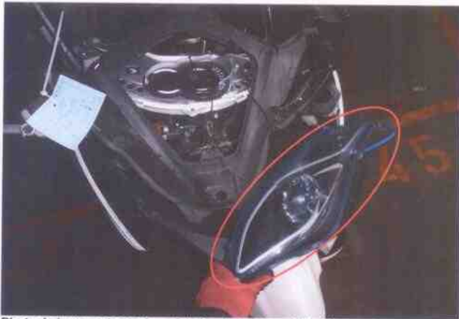
Photo 4 shows a closer view of the frontal portion of the Motorcycle at the time of our inspection. The headlamp Motorcycle was observed to be dislodged from the original installation due to the accident collision. (Circled)
