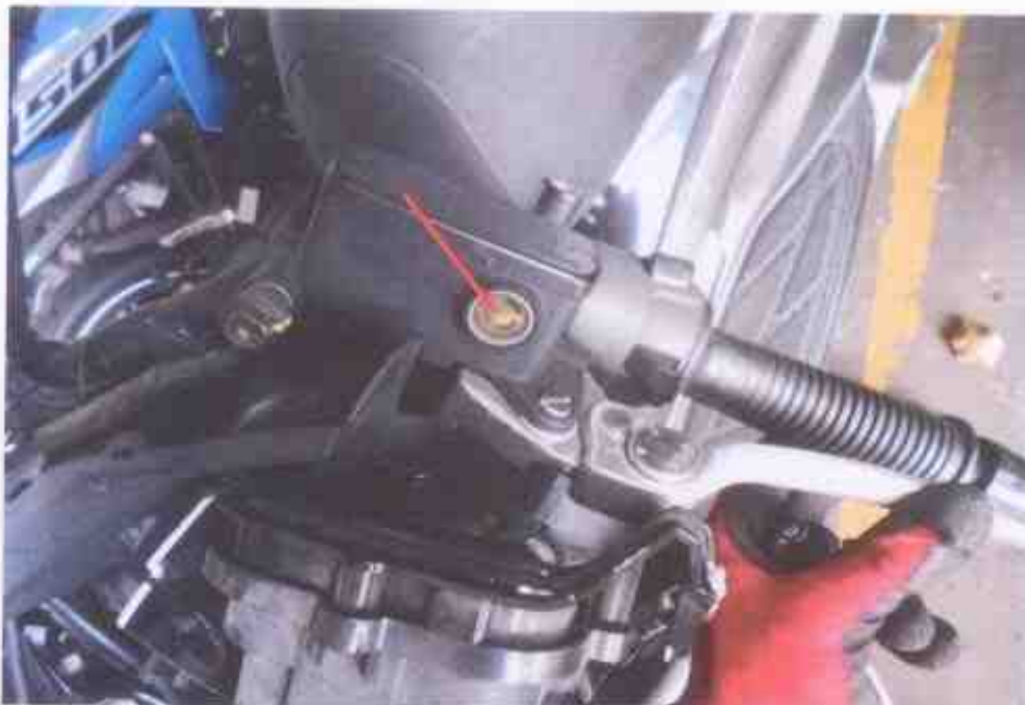
Photo 17 shows the rear brake fluid reservoir. Our checks on the brake fluid had also indicated that the brake fluid was of sufficient level for operational purposes, and without contamination.
