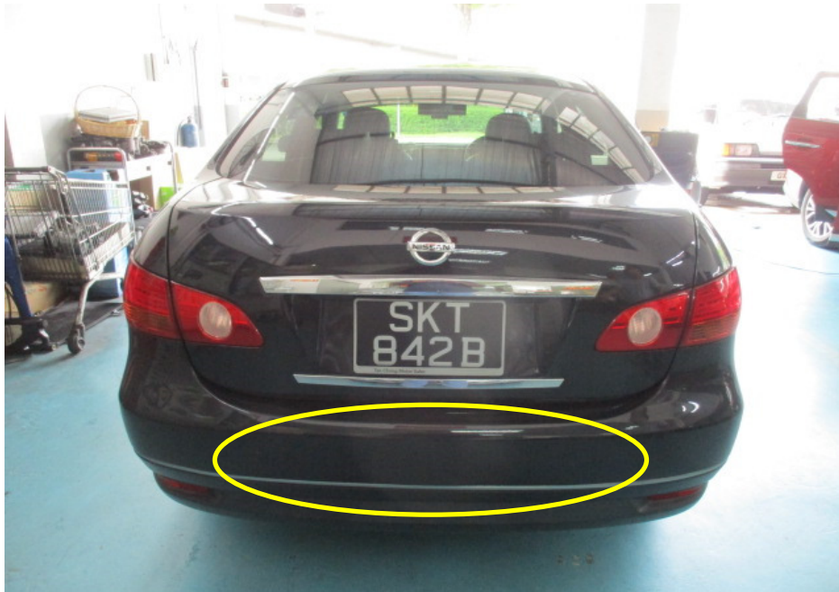
Photo 1 shows the general view of the rear portion of the Nissan upon our inspection. The damage to the Nissan was observed to be confined to its rear portion, at the centre portion (circled).
