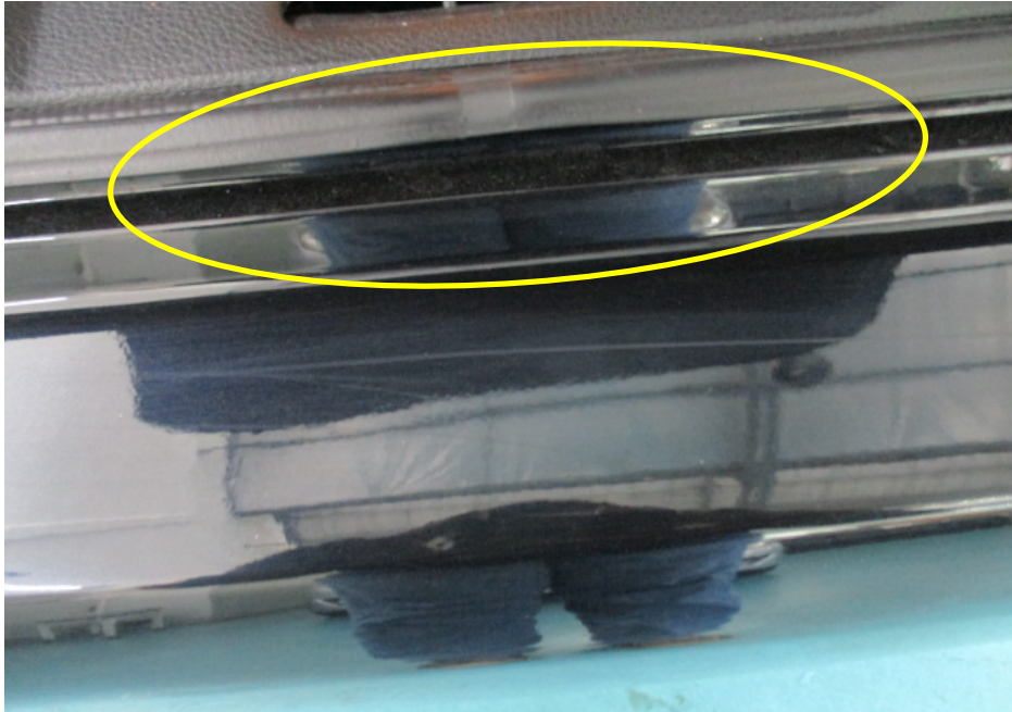
Photo 3 shows a closer view of the gap between the boot lid weather strip and rear bumper at the centre portion, indicating that the rear bumper reinforcement and possibly the rear end panel of the Nissan had been pushed slightly inwards (circled).
