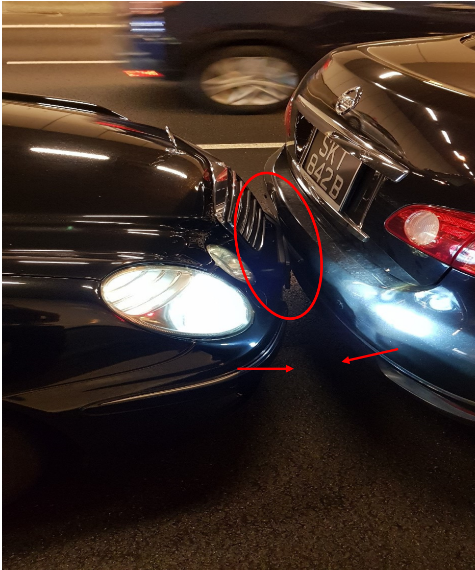
Photo 14 shows a right side view of the final position of the Involved Motor Cars at the accident location. The front centre portion of the Mercedes was observed to be directly in contact with the rear centre portion of the Nissan (circled). It can be observed that there was no contact between the rear right portion of the Nissan and the front right portion of the Mercedes (arrowed).
