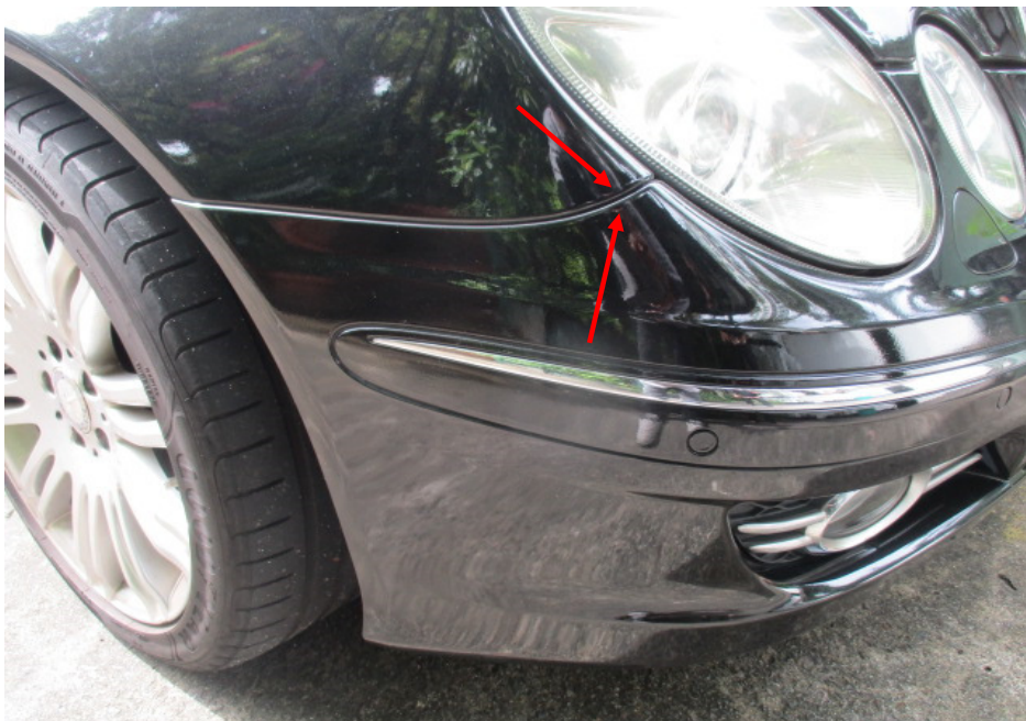
Photo 11 shows a closer view of the right corner edge of the front bumper of the Mercedes. We observed that there was no misalignment at the corner edges (arrowed).
