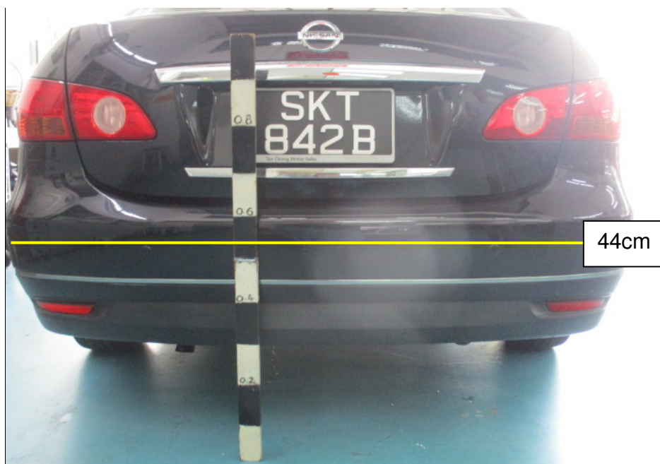
Photo 17 shows the height measurement being conducted on the rear portion of the Nissan. The height above ground level of the centre portion of the rear bumper of the Nissan, at the area where the paint scratch marks were found was measured to be approximately 44cm.
