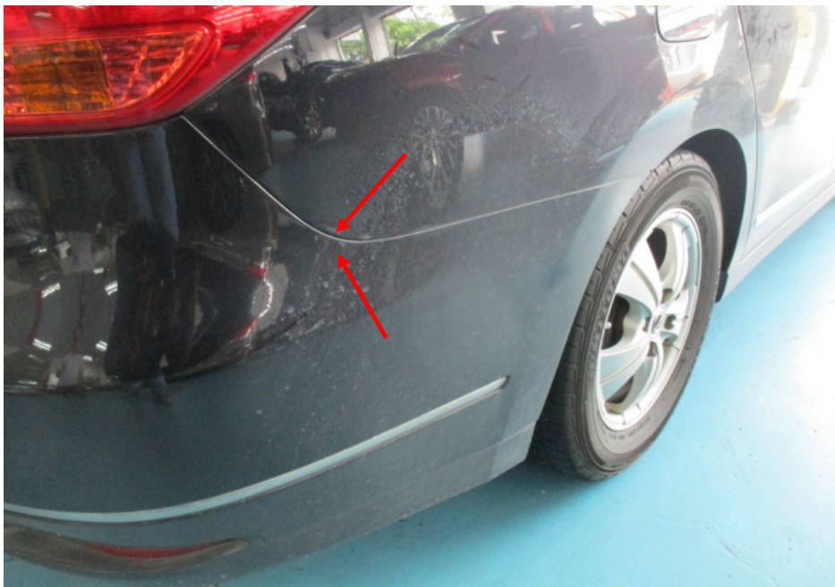
Photo 6 shows a closer view of the right corner edge of the rear bumper of the Nissan. We observed that there was no misalignment at the corner edges (arrowed).
