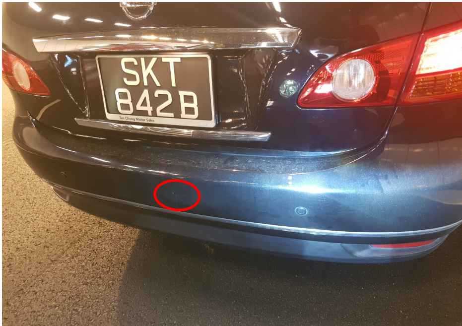
Photo 16 shows the position of the Nissan after the accident. The paint scratch marks on the centre portion of the rear bumper can be seen (circled). However there was no deformity observed on the rear bumper of the Nissan as there was no distortion of the reflected objects.
