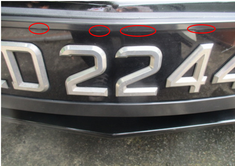
Photo 8 shows a closer view of the faint whitish distortion marks on the top centre portion of the Mercedes's front number plate frame (circled). We also observed that there were no dents or cracks on its front number plate.
