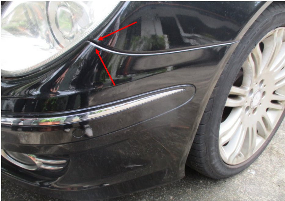
Photo 10 shows a closer view of the left corner edge of the front bumper of the Mercedes. We observed that there was no misalignment at the corner edges (arrowed).
