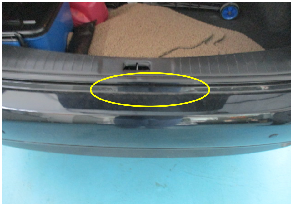
Photo 2 shows upon closer examination, we noted a gap between the boot lid weather strip and rear bumper at the centre portion (circled).
