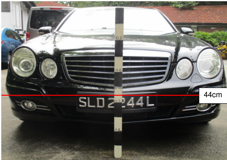
Photo 18 shows the height measurement being conducted on the frontal portion of the Mercedes. The body part at 44cm above ground was the top portion of the Mercedes' front number plate frame where the faint whitish distortion marks were found.
