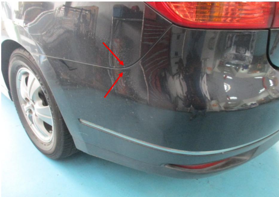
Photo 5 shows a closer view of the left corner edge of the rear bumper of the Nissan. We observed that there was no misalignment at the corner edges (arrowed).
