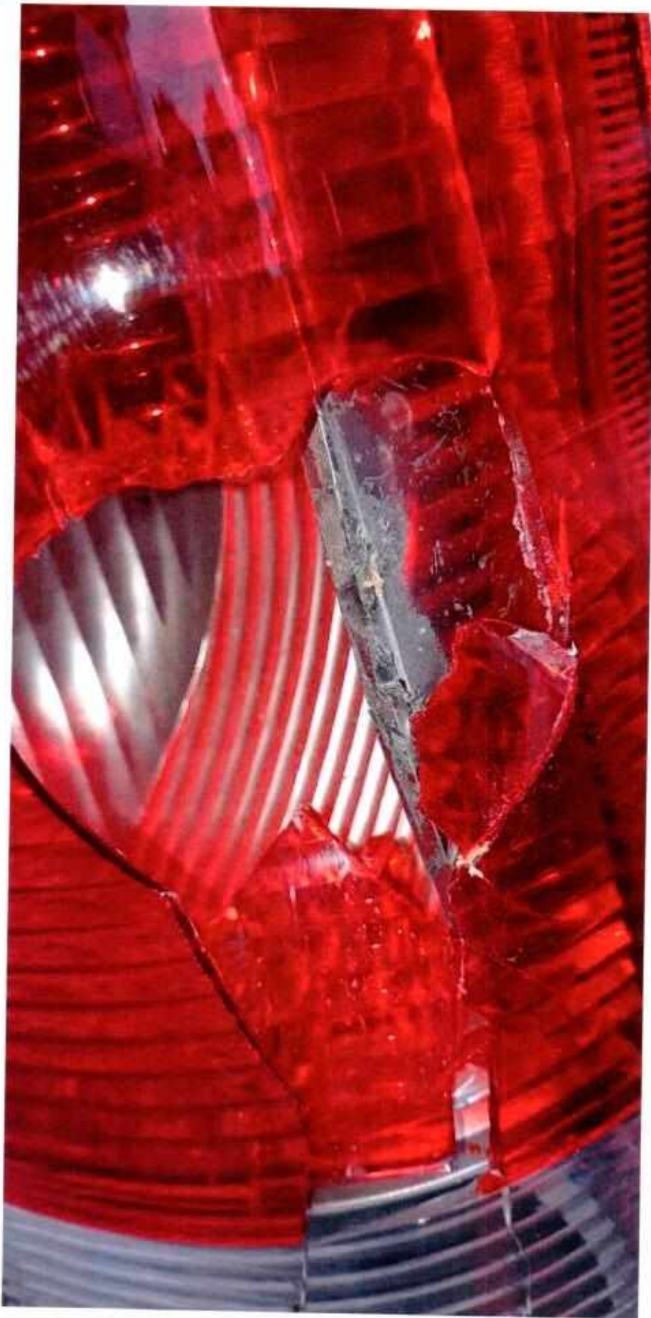
Debris of wood found on cracked lamp
