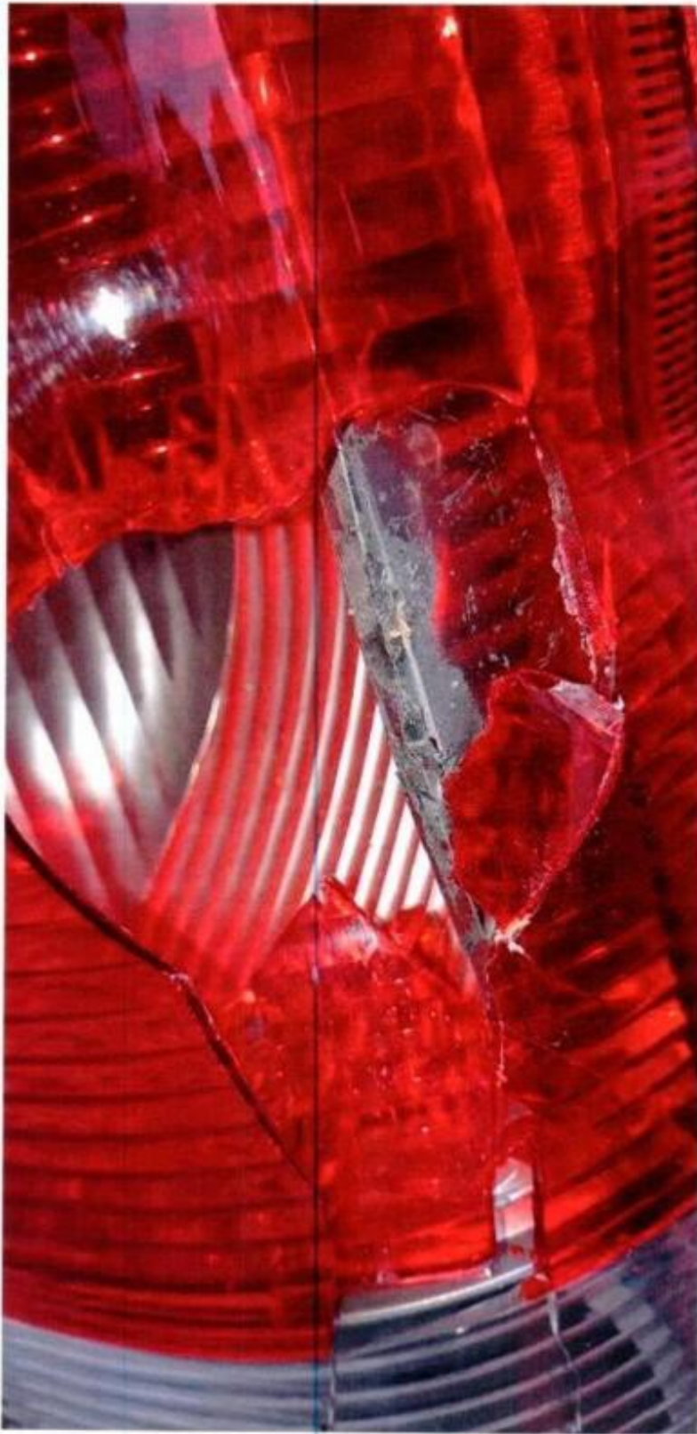
Debris of wood found on cracked lamp
