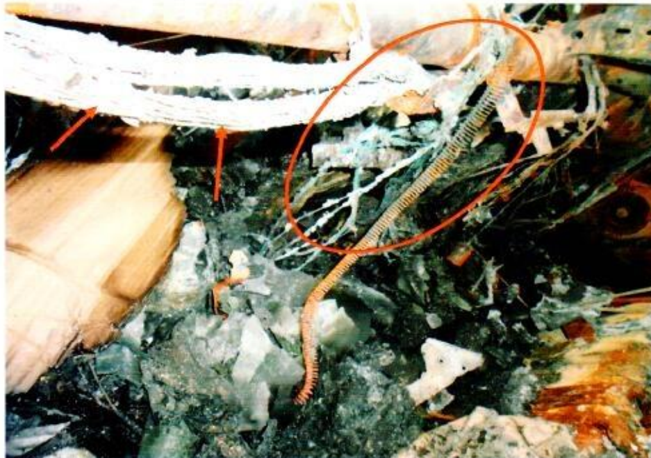
Photo 11 shows the original stretch wirings located at the centre portion of the dashboard (circled) of the Insured Vehicle. We observed greenish residue on these wirings (arrowed).
