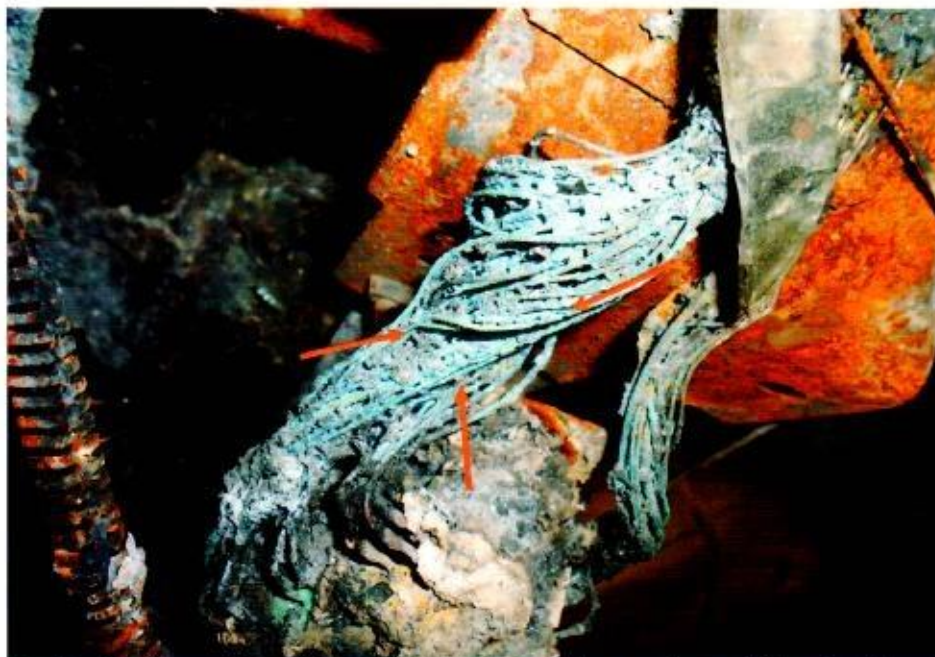
Photo 9 shows the wirings around the centre portion of the dashboard compartment which is near to the vicinity where the fire to the Insured Vehicle had likely started. We observed greenish residue on the wirings at the centre portion of the dashboard compartment (arrowed).
