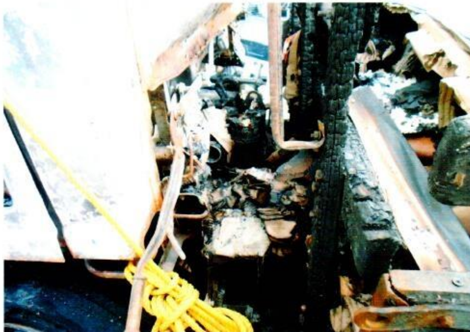
Photo 7 shows part of the engine compartment of the Insured Vehicle at the time of our inspection. The entire engine compartment of the Insured Vehicle was observed to be severely burnt. Most of the parts inside the engine compartment were found to be burnt and/or melted as a result of the fire.
