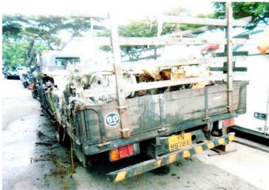
Photo 3 shows the general view of the rear body of the Insured Vehicle at the time of our inspection. The Insured Vehicle was observed to have sustained extensive fire damage at the rear storage compartment. Carton boxes, plastics, steel materials were found to be burnt which were located at the rear compartment affected by the fire.
