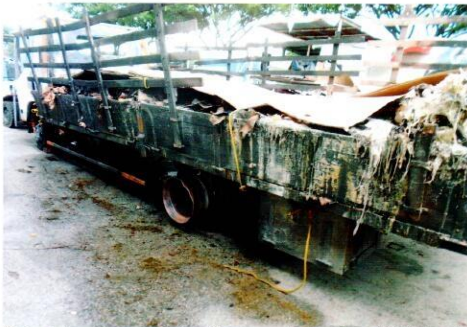
Photo 4 shows the general view of the rear body of the Insured Vehicle at the time of our inspection. The Insured Vehicle was observed to have sustained extensive fire damage at the rear storage compartment. Carton boxes, plastics, steel materials were found to be burnt which were located at the rear compartment affected by the fire.
