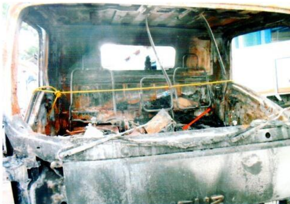
Photo 12 shows a general view of the front dashboard where the possible shot circuit wirings of the Insured Vehicle (arrowed).
