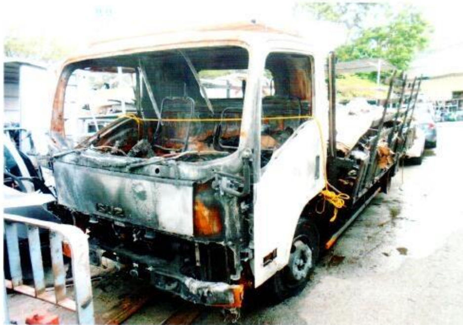
Photo 1 shows the general view of the front left portion of the Insured Vehicle at the time of our inspection. The Insured Vehicle was observed to have sustained extensive fire damage all around. Its engine compartment and interior compartment were completely burnt. Rust had accumulated all over the Insured Vehicle as a result of exposure to environmental condition for a period of time.
