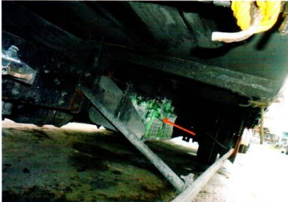
Photo 13 shows a general view of the melted battery of the Insured Vehicle due to the fire incident.
