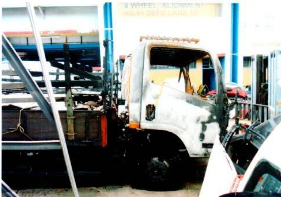
Photo 2 shows the general view of the right front portion of the Insured Vehicle at the time of our inspection. The Insured Vehicle was observed to have sustained extensive fire damage all around. Rust had accumulated all over the Insured Vehicle as a result of exposure to environmental condition for a period of time.
