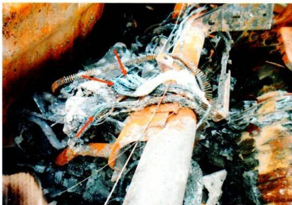
Photo 10 shows a closer view of the greenish residue found on the wirings at the centre portion of the dashboard compartment (arrowed). This seems to suggest the occurrence of an electrical short circuit.
