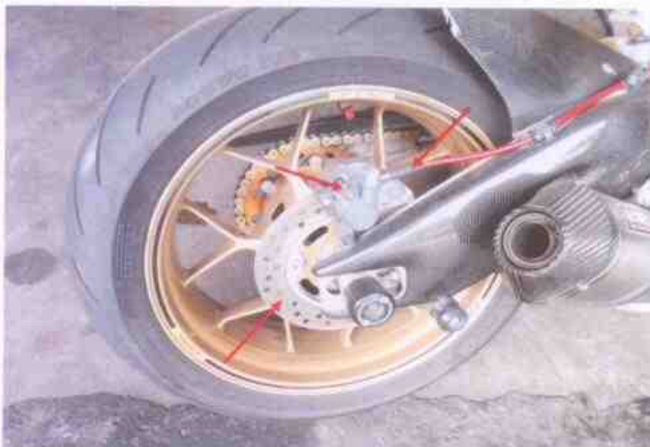
Photo 18 shows the rear brake calliper, rear brake disc and rear brake hose of the Motorcycle, which are all part of the components in the rear brake system of the Motorcycle. Our observation found that the rear braking components were unaffected by the accident.
