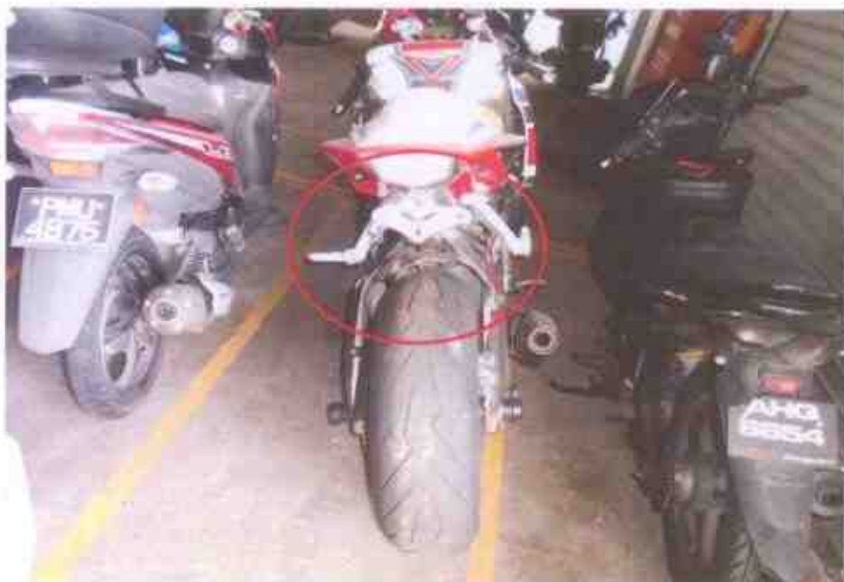
Photo 3 shows a general view of the rear body of the Motorcycle at the time of our inspection. The Motorcycle was observed to sustain with damages which affects the rear mudguard, rear licence plate & rear left signal lamp due to the accident.
