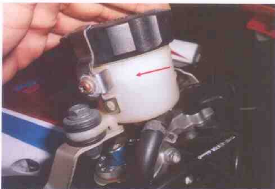
Photo 14 shows the front brake fluid reservoir had indicated that the brake fluid was of sufficient level for operational purposes, and without contamination.
