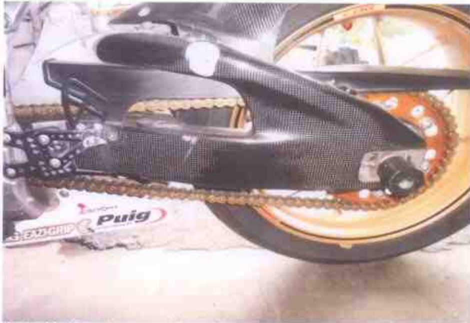
Photo 11 shows the general view of the gear train of the Motorcycle, which was observed to be intact with no misalignment. It was also adequately lubricated for operating purposes.
