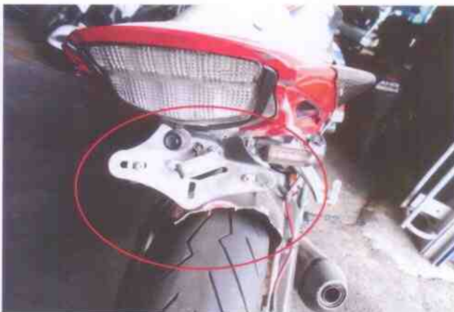
Photo 4 shows a close-up view of the rear portion of the Motorcycle at the time of our inspection. The Motorcycle was observed to sustain with damages which affects the rear mudguard, rear licence plate & rear left signal lamp due to the accident.
