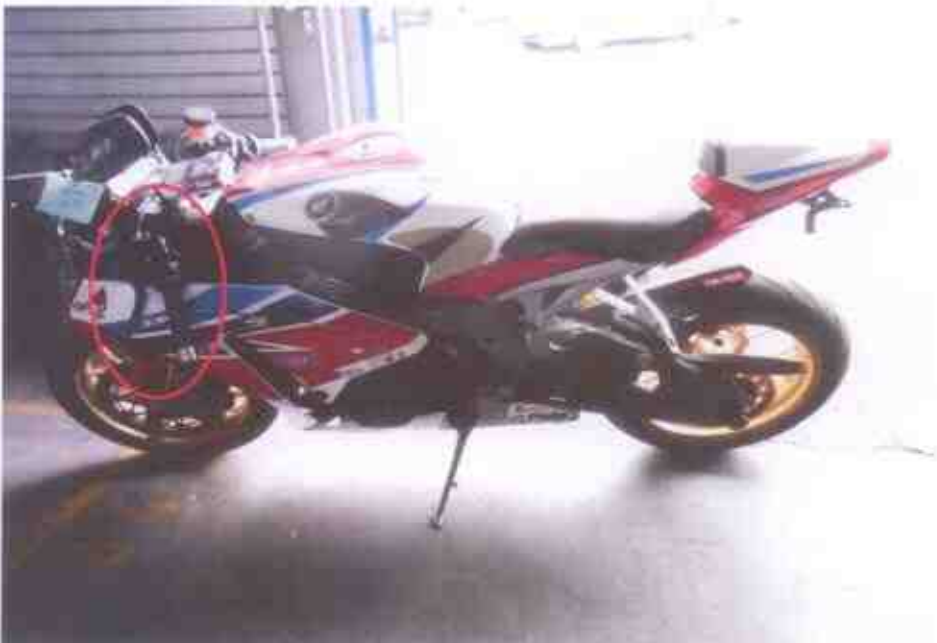
Photo 2 shows a general view of the front left body of the Motorcycle at the time of our inspection. The Motorcycle was observed to be sustained with damages due to the accident collision. Amongst the body parts damaged was its left handle bar, which was observed to be dislodged from the original structure.
