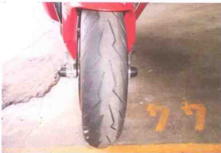
Photo 8 shows the front tyre of the Motorcycle. The pattern of the tread was clearly visible with remaining tread depth of about 2mm. There was no tear, burst mark(s) and/or punctured hole(s) on the sidewalls as well as across the tread of the rear tyre unaffected by the accident's impact collision.
