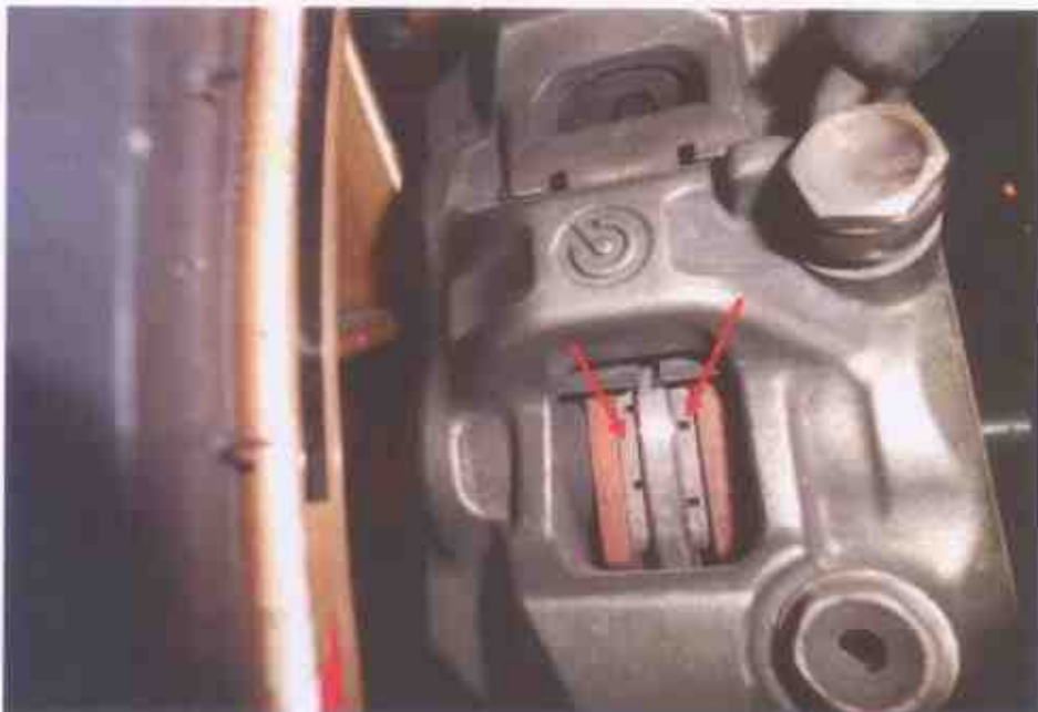
Photo 16 shows the front brake pad of the Motorcycle (arrowed), which are part of the components in the front brake system of the Motorcycle reveal to be adequately sufficient for operational purposes.
