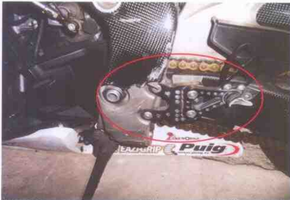
Photo 7 shows a semi close-up view of the left portion of the Motorcycle at the time of our inspection. The Motorcycle was observed to have sustained with dislodged left side foot rest & gear shift pedal due to the accident collision.
