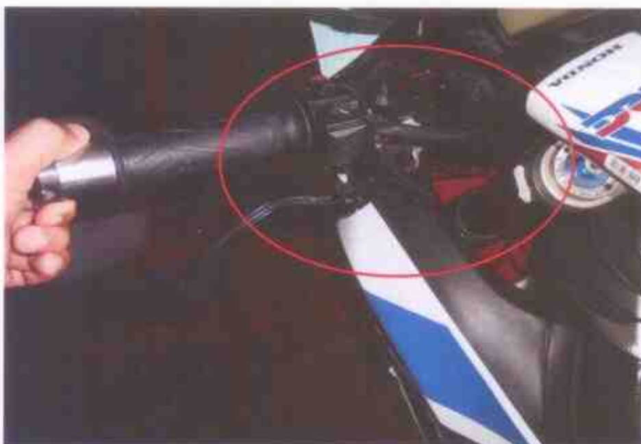
Photo 5 shows a semi close-up view of the frontal portion of the Motorcycle at the time of our inspection. The Motorcycle was observed to be sustained with dislodged left hand side handle bar due to the accident collision.
