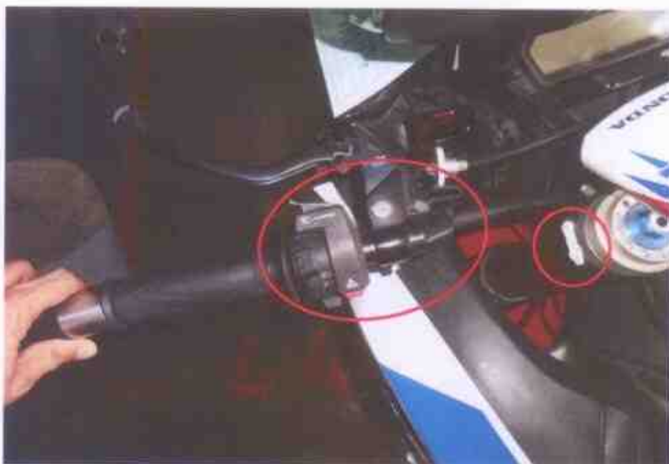
Photo 13 shows the front left side handle bar was observed to be dislodged as a result of the accident. Hence, we are not able to conduct any tests on the steering system of the Motorcycle.
