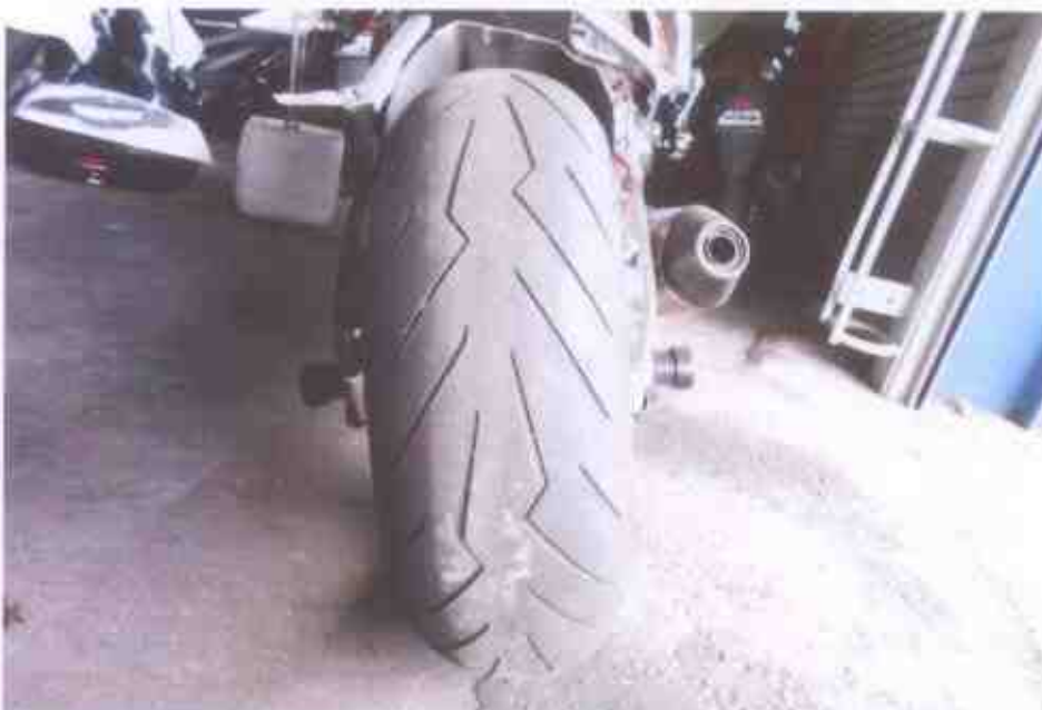
Photo 9 shows the rear tyre of the Motorcycle. The pattern of the tread was clearly visible with remaining tread depth of about 3mm. There was no tear, burst mark(s) and/or punctured hole(s) on the sidewalls as well as across the tread of the rear tyre unaffected by the accident's impact collision.
