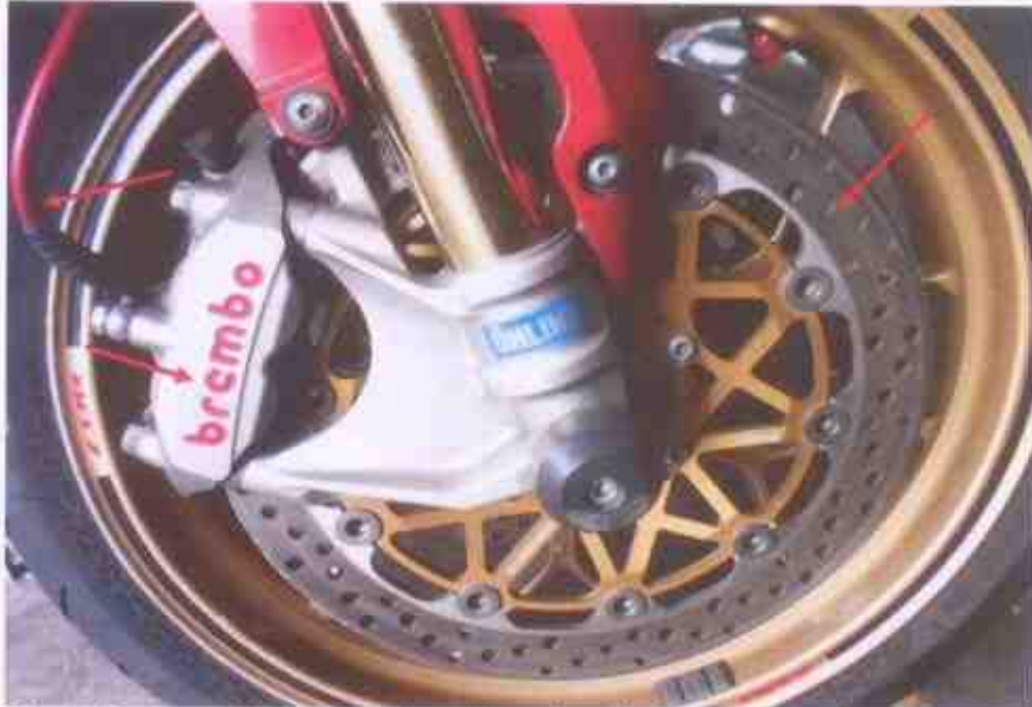
Photo 15 shows the front brake caliper, front brake disc, front brake pad and front brake hose of the Motorcycle, which are all part of the components in the front brake system of the Motorcycle. Our observation found that the front braking components were unaffected by the accident.
