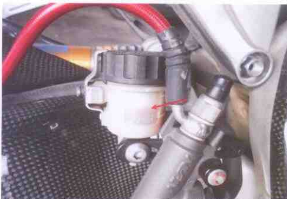
Photo 17 shows the rear brake fluid reservoir had indicated that the brake fluid was of sufficient level for operational purposes, and without contamination.
