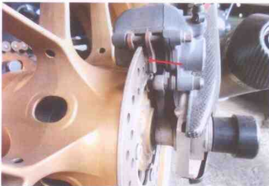
Photo 19 shows the rear brake pad of the Motorcycle (arrowed), which are part of the components in the rear brake system of the Motorcycle reveal to be adequately sufficient for operational purposes.
