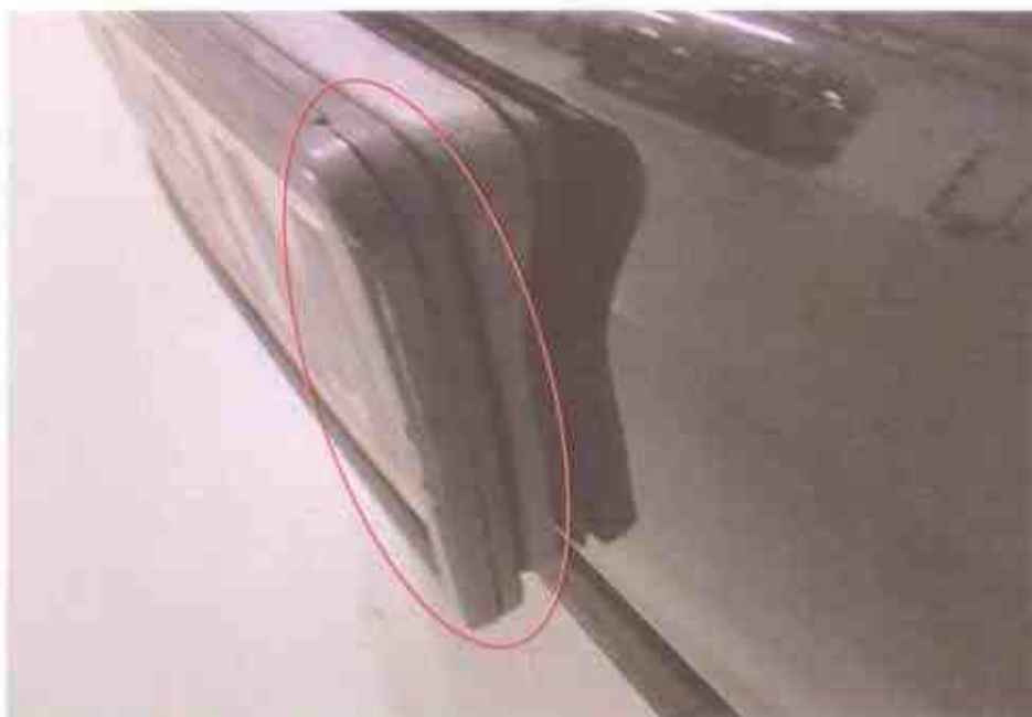
Photo 10 shows a closer view of the distortion on the left portion of the E200's front number plate frame (circled).
