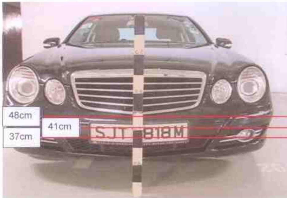
Photo 19 shows the height measurement being conducted on the front portion of the E200. The height range above ground level of the vertical indentation found on the left portion of the E200's front bumper was measured to be approximately between 37cm to 48cm. The bodypart at 41cm above ground level was the top portion of the alpha- numeric letterings of the front number plate where the whitish marks were found.
