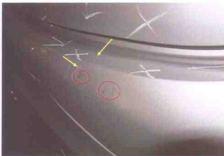
Photo 2 shows the paint cracks (arrowed) as well as the vertical black marks on the right portion of the rear bumper (circled).
