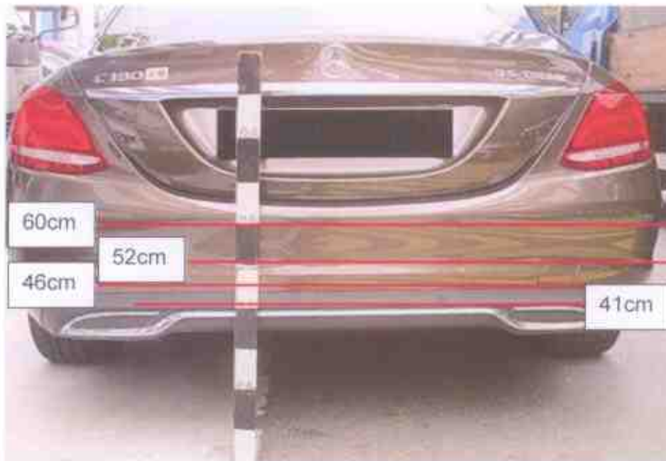
Photo 18 shows the height measurement being conducted on the rear portion of the C180 (using a similar make and model). The height above ground level of the C180's dislodged right reverse sensor was measured to be approximately 41cm. The height range above ground level of the C180's dislodged tow hook cover was measured to be between 46cm to 52cm. The height above ground level of the top portion of the C180's rear bumper at the area where the black marks and paint cracks were found was measured to be approximately 60cm.
