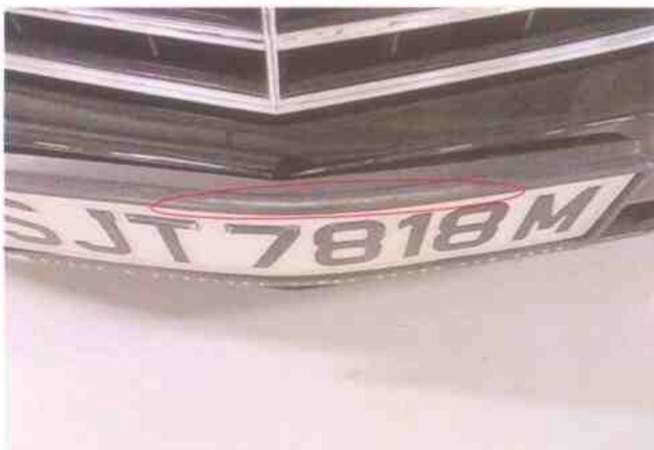
Photo 9 shows a closer view of the distortion on the top portion of the E200's front number plate frame (circled).
