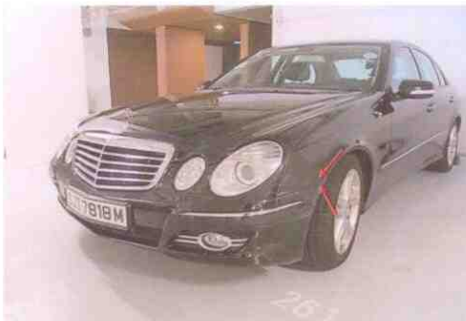
Photo 15 shows a closer view of the left corner edge of the front bumper of the E200. We observed that there was no misalignment at the corner edges (arrowed).
