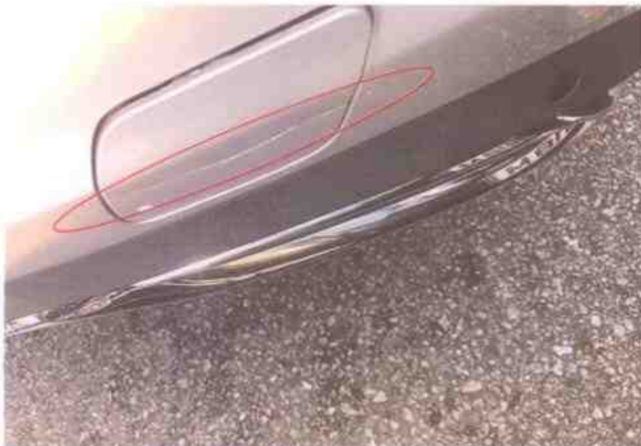
Photo 17 shows a close up view of the damaged tow hook cover of the C180 post- accident. We observed a horizontal indentation on the tow hook cover (circled)
