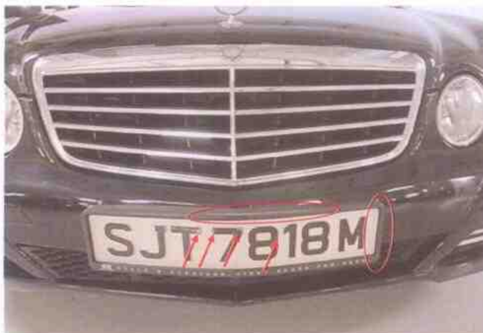
Photo 8 shows the distortion on the top and left portion of the E200's front number plate frame (circled), indicating that it had sustained an impact directly onto its front number plate. Upon closer examination, we observed whitish marks on the top alpha-numeric letterings of the front number plate (arrowed).
