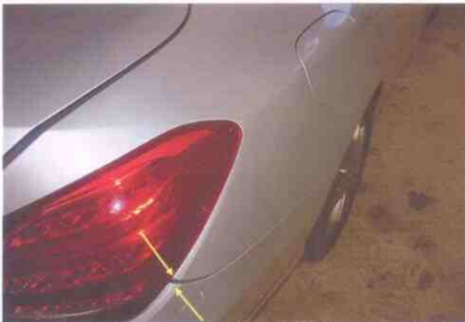
Photo 5 shows a closer view of the misalignment at the right corner edges of the rear bumper (arrowed).
