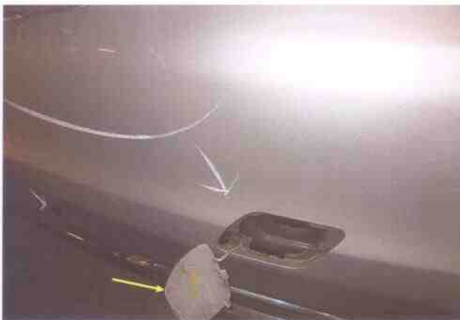
Photo 3 shows a close up view of the dislodged tow hook cover (arrowed).
