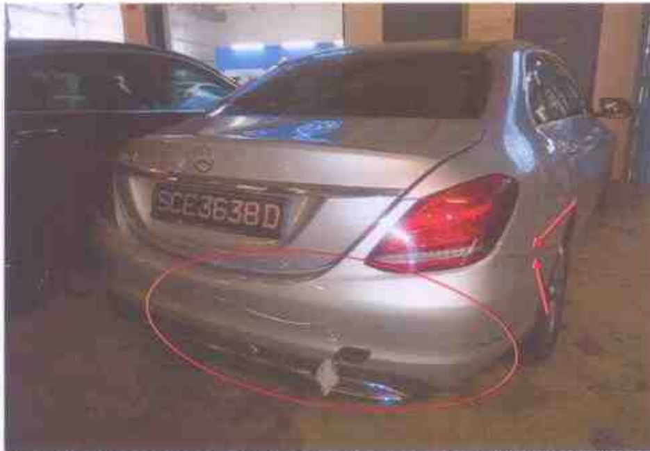
Photo 1 shows a right view of the rear portion of the C180 at the time of the Pre-Repair Survey conducted by LKK Auto Consultants Pte. Ltd. taken 5 days after the accident. The damages were concentrated on the right portion of the rear bumper (circled). There was a slight misalignment at the right corner edges of the rear bumper (arrowed).
