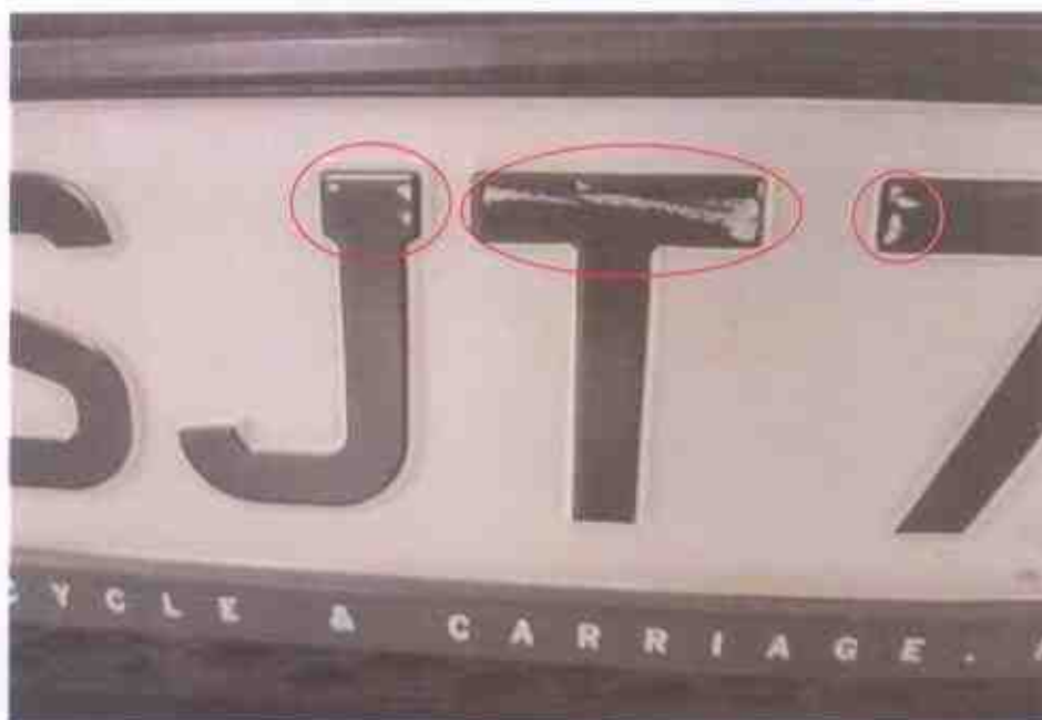
Photo 11 shows a close up view of the whitish marks on some of the top alphanumeric letterings of the front number plate (circled).
