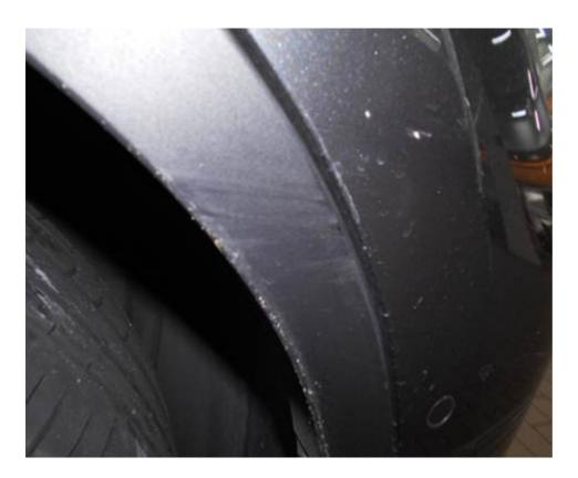
The above photos show a closer look on the thrid party vehicle which shows damages in grazing nature. The front bumper surface were scratch all the way to the wheel arch trim. Our surveyor in view that these damages were beyond repair and these parts were recommended to be replaced (see attached survey report).
