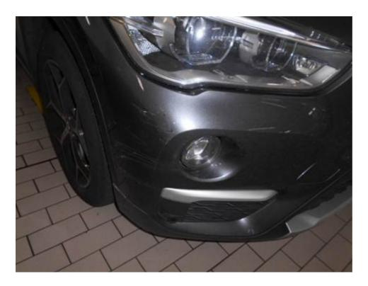
The above photo shows the front right portion of the third party vehicle that sustained damages as a result of the collision.
