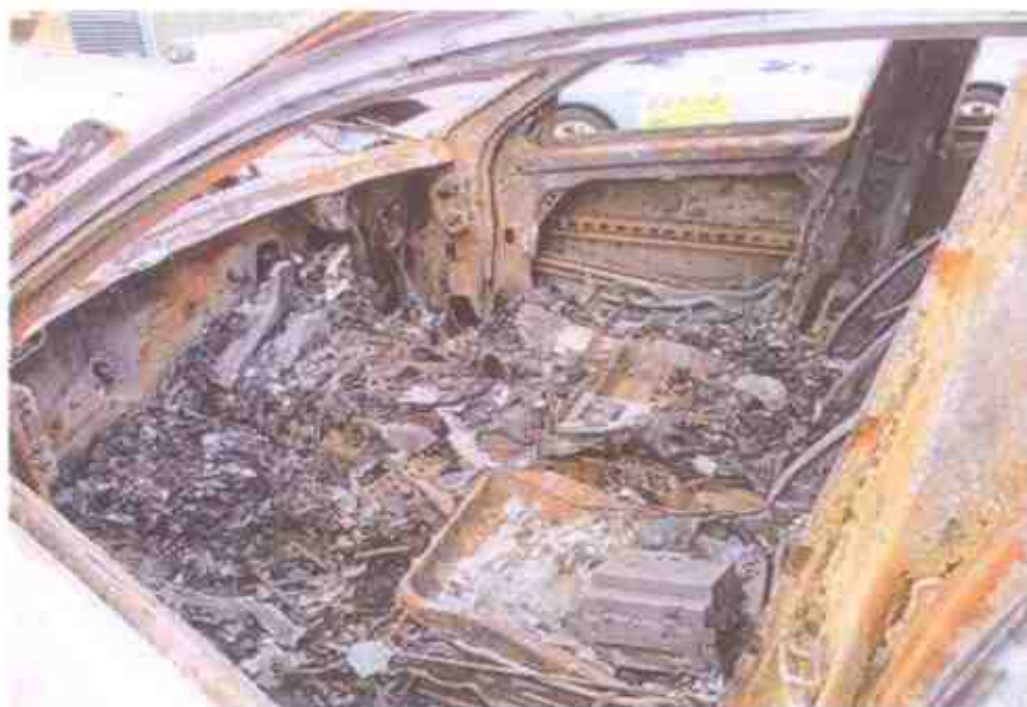
Photo 6 shows the general view of the interior compartment of the Insured Vehicle at the time of our inspection. Its interior compartment was completely burnt as a result of the fire.
