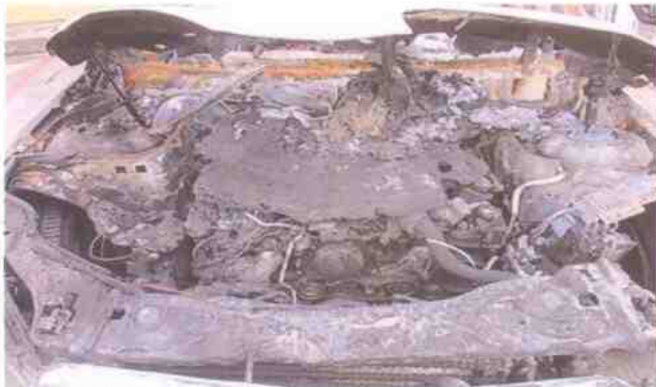
Photo 7 shows the engine compartment of the Insured Vehicle at the time of our inspection. The entire engine compartment of the Insured Vehicle was observed to be severely burnt. Most of the parts inside the engine compartment were found to be burnt and/or melted as a result of the fire.
