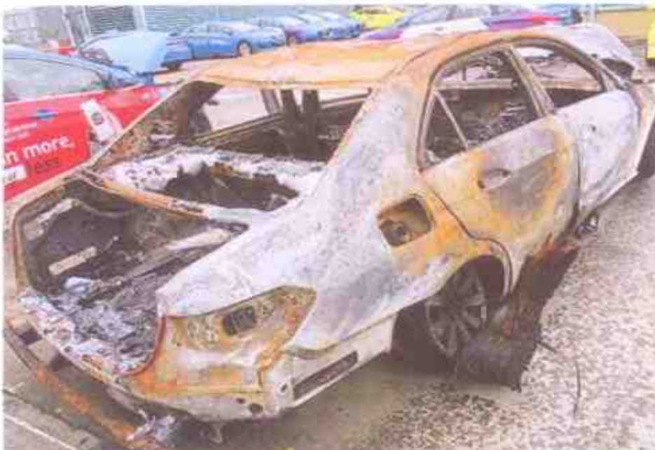
Photo 4 shows the general view of the rear right body of the Insured Vehicle at the time of our inspection. The Insured Vehicle was observed to have sustained extensive fire damage all around. Rust had accumulated all over the rear and centre portion of the Insured Vehicle as a result of exposure to environmental condition for a period of time.
