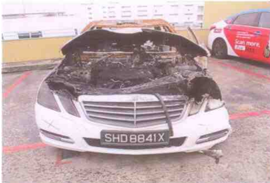
Photo 1 shows the general view of the front portion of the Insured Vehicle at the time of our inspection. The Insured Vehicle was observed to have sustained extensive fire damage all around. Its engine compartment and interior compartment were completely burnt. Rust had accumulated all over the rear and centre portion of the Insured Vehicle as a result of exposure to environmental condition for a period of time.
