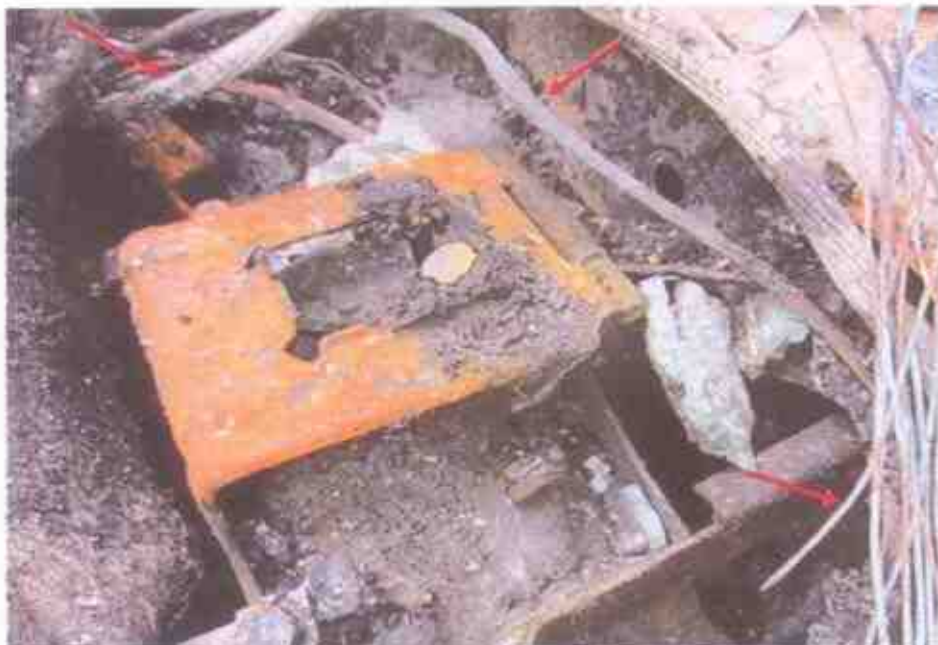
Photo 11 shows a close up view of the greenish residue found on some of the burnt stretches of original factory fitted wirings (arrowed) leading from the battery. The presence of such greenish residue suggests occurrence of an electrical short circuit.
