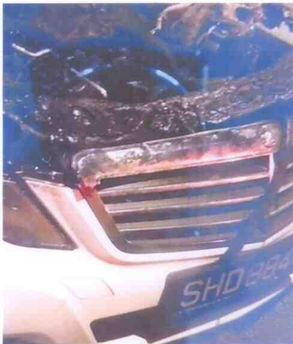
Photo 13 shows the front portion of the Insured Vehicle after the fire was extinguished. In general, the damages sustained to the front portion had corresponded to the events that were related to us by Mr Ho, which is the fire had not started from the front bonnet.
