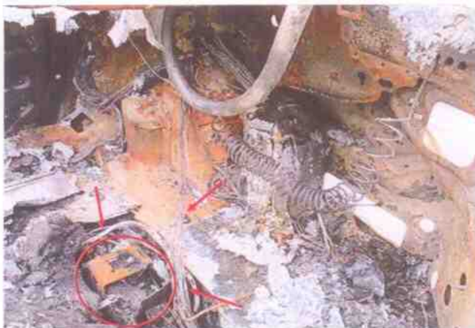
Photo 9 shows a closer view of the greenish residue found on some of the burnt stretches of original factory fitted wirings (arrowed) leading from the battery (circled). The presence of such greenish residue suggests occurrence of an electrical short circuit.
