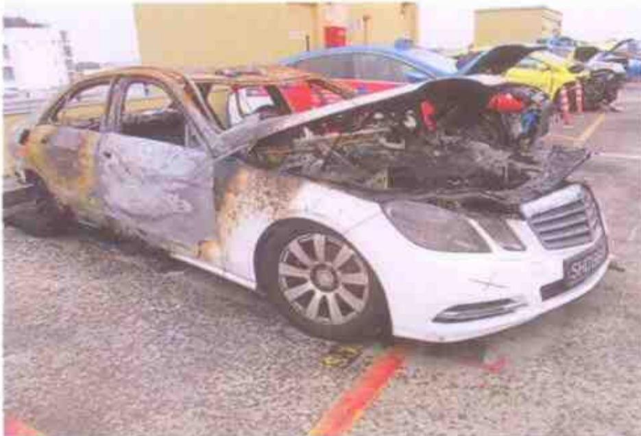
Photo 3 shows the general view of the right body of the Insured Vehicle at the time of our inspection. The Insured Vehicle was observed to have sustained extensive fire damage all around. Rust had accumulated all over the rear and centre portion of the Insured Vehicle as a result of exposure to environmental condition for a period of time.
