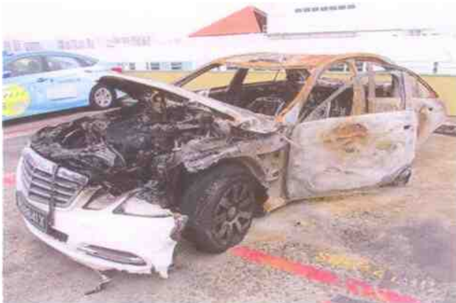
Photo 2 shows the general view of the left body of the Insured Vehicle at the time of our inspection. The Insured Vehicle was observed to have sustained extensive fire damage all around. Rust had accumulated all over the rear and centre portion of the Insured Vehicle as a result of exposure to environmental condition for a period of time.
