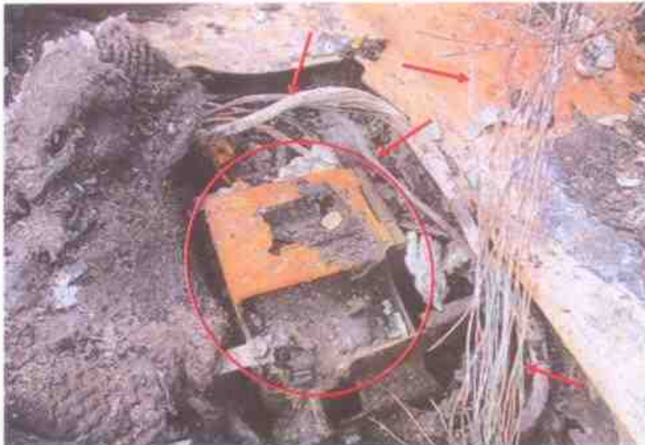
Photo 10 shows a close up view of the greenish residue found on some of the burnt stretches of original factory fitted wirings (arrowed) leading from the battery (circled). The presence of such greenish residue suggests occurrence of an electrical short circuit.
