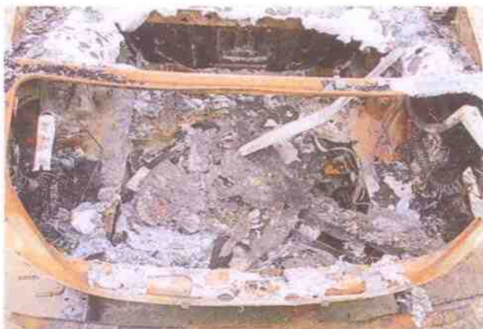
Photo 5 shows the general view of the rear boot compartment of the Insured Vehicle at the time of our inspection. The rear boot compartment sustained extensive fire damage. Rust had accumulated all over the rear portion of the Insured Vehicle as a result of exposure to environmental condition for a period of time.
