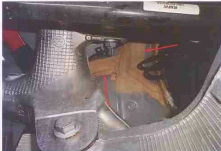
Photo 15 shows the structural body at the underside rear right of the Motor Car. Visually, The original factory sealant (arrowed) at the joints along the chassis body was untouched, indicating no work was done on the chassis body of the Motor Car and that the chassis body was originally fitted.
