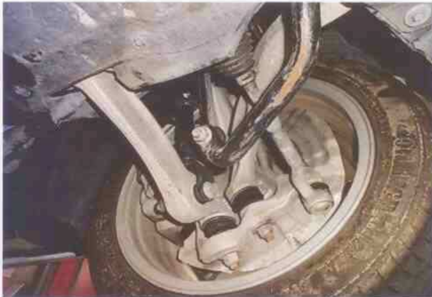
Photo 11 shows the various undercarriage components at the front left wheel of the Motor Car. The mechanical components, control arms and linkages were all found to be intact and secured in an appropriate manner.
