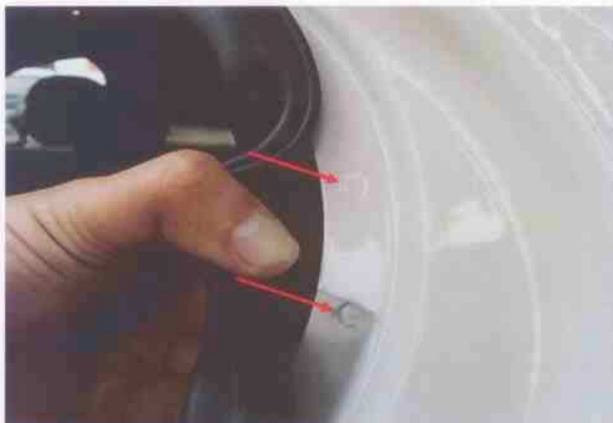
Photo 18 shows the rear left "C" pillar of the Motor Car. I did not find any weld marks other than original spot weld marks (arrowed) on the body panels of the Motor Car, indicating that there was no re-welding works carried out; and that the body panels of the Motor Car were originally fitted.
