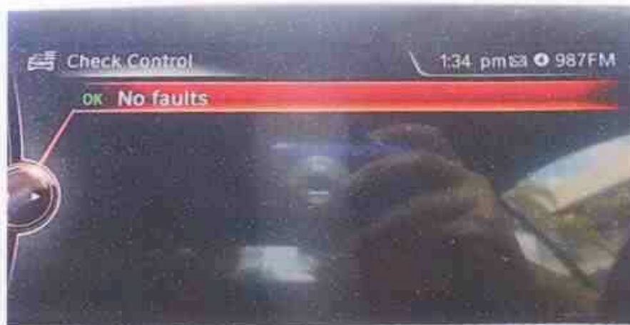
Photo 8 shows no fault(s) was detected to the various controls and systems of the Motor Car after my initiation of the Motor Car's on-board self-diagnostic check.
