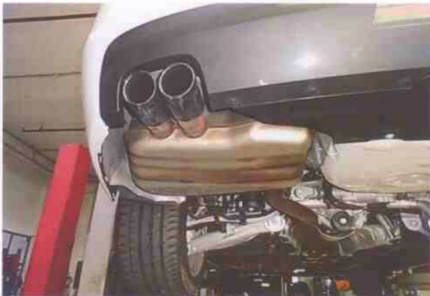
Photo 13 shows the Motor Car's rear exhaust muffler. My examination of the Motor Car's exhaust system revealed no sign(s) or indication(s) of any cut or weld marks along its exhaust pipes and on its rear mufflers.
