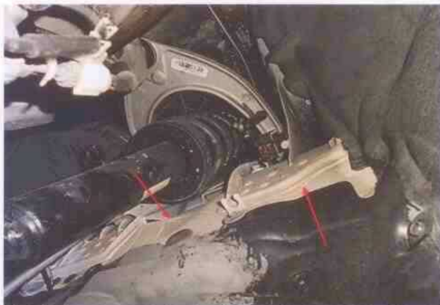
Photo 16 shows the structural body at the underside front left of the Motor Car. The original factory sealant (arrowed) at the joints along the chassis body was untouched, indicating no work was done on the chassis body of the Motor Car and that the chassis body was originally fitted
