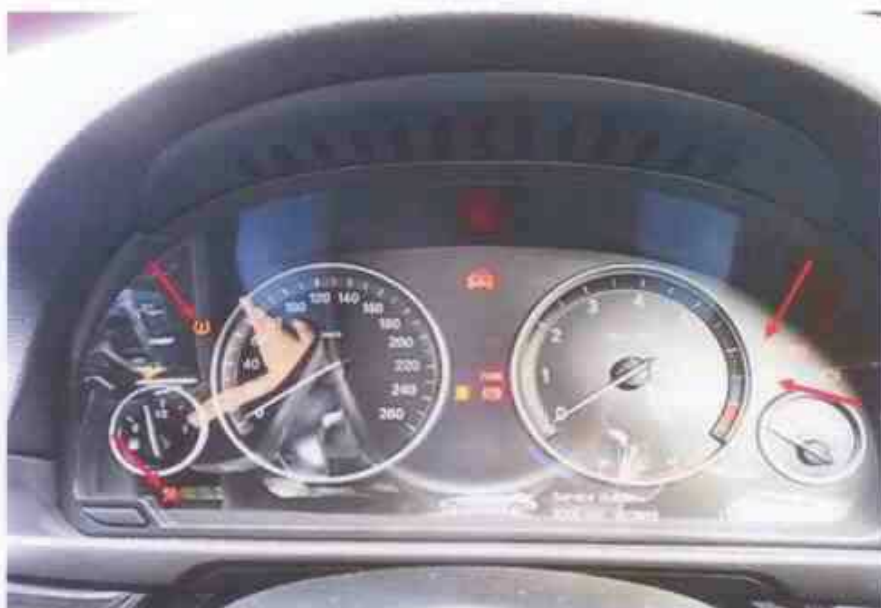
Photo 6 shows the warning lights for the various electronic safety features appearing on the instrument panel of the Motor Car during its self-test when the engine is cranked, in particular the ABS, SRS, TPM and DSC lights (arrowed).
