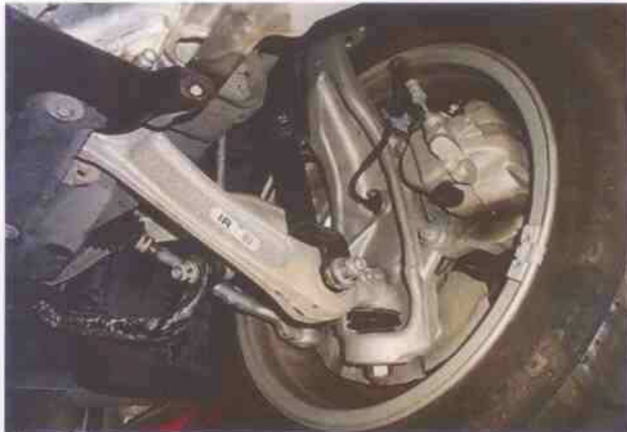
Photo 12 shows the various undercarriage components at the front right wheel of the Motor Car. The mechanical components, control arms and linkages were all found to be intact and secured in an appropriate manner.
