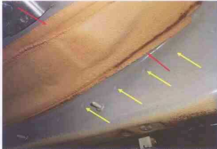
Photo 14 shows the structural body at the underside centre left of the Motor Car. Visually, I did not find any weld marks other than original spot weld marks (yellow arrow) on the chassis body of the Motor Car. The original factory sealant (red arrow) at the joints along the chassis body was also untouched, indicating no work was done on the chassis body of the Motor Car and that the chassis body was originally fitted.
