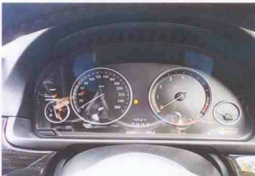
Photo 7 shows the respective warning lights no longer illuminated, indicating that there is no fault detected to the ABS, SRS, TPM and DSC systems of the Motor Car during the self-test. These electronic systems were hence in working condition at the time of my inspection.
