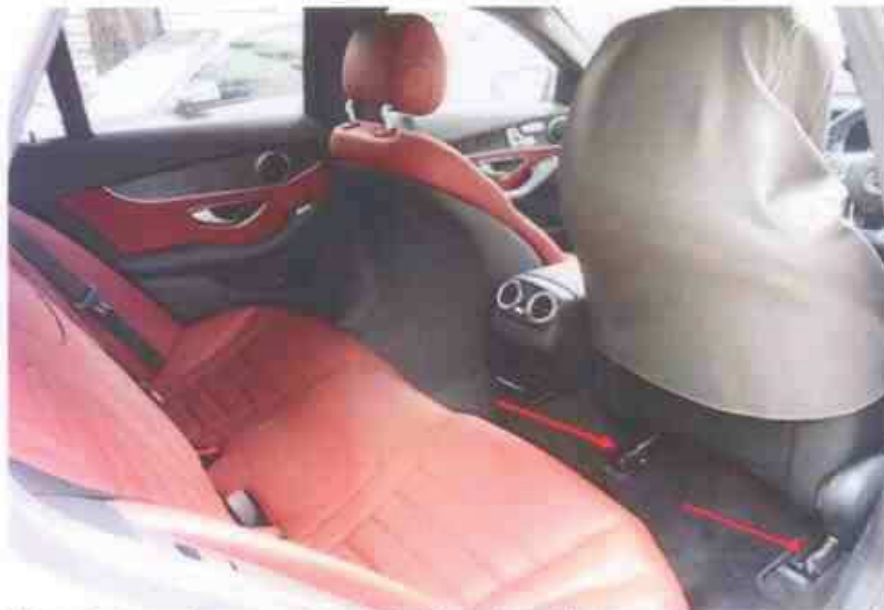
Photo 5 shows the rear seats of the Motor Car. All the seats were secured via seat rails (arrowed) to the floor board. The seats were also fitted with a retractable seat belt reel and pre-tensioner. The seat belts were tested and able to be fastened to the pretensioners that were fitted on the side of each individual seat.
