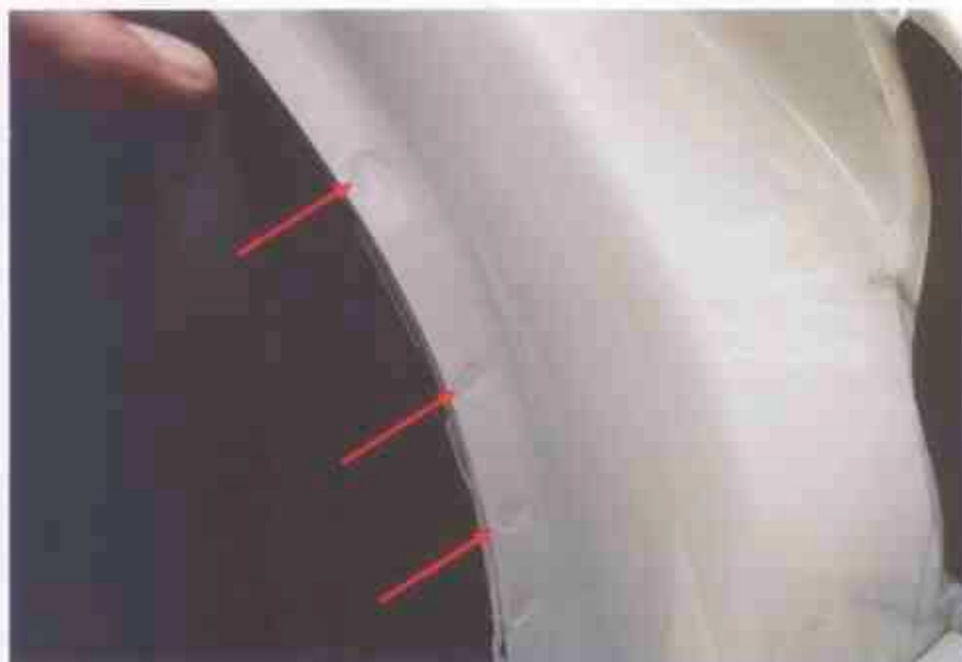
Photo 17 shows the right "A" pillar of the Motor Car. I did not find any weld marks other than original spot weld marks (arrowed) on the body panels of the Motor Car, indicating that there was no re-welding works carried out; and that the body panels of the Motor Car were originally fitted.
