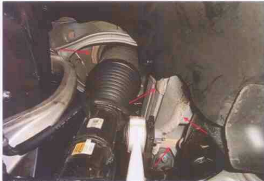
Photo 15 shows the structural body and wheel house panel at the front left of the Motor Car. The original factory sealant (arrowed) at the joints along the chassis body was untouched, indicating no work was done on the chassis body of the Motor Car and that the chassis body was originally fitted.
