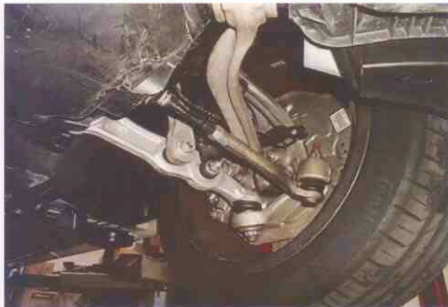
Photo 10 shows the various undercarriage components at the front left wheel of the Motor Car. The mechanical components, control arms and linkages were all found to be intact and secured in an appropriate manner.
