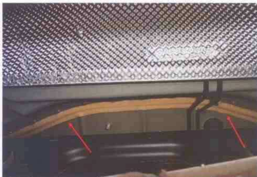
Photo 13 shows the structural body at the rear floorboard of the Motor Car. The original factory sealant (arrowed) at the joints along the chassis body was untouched, indicating no work was done on the chassis body of the Motor Car and that the chassis body was originally fitted.
