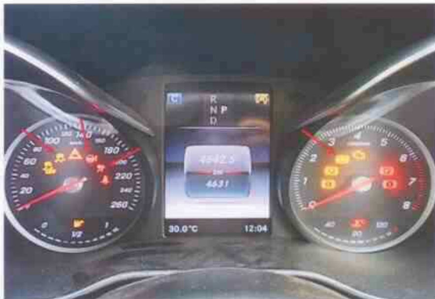
Photo 6 shows the warning lights for the various electronic safety features appearing on the instrument panel of the Motor Car during its self-test when the engine is cranked, in particular the ABS, SRS, PSA and TCS lights (arrowed).
