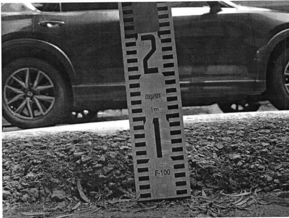
Photo 8: Shows the height measurement of the road hump.
