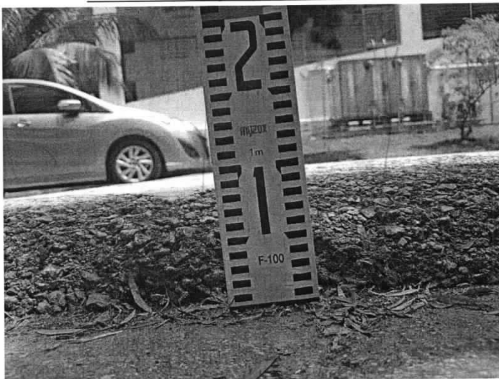
Photo 7: Shows the height measurement of the road hump.
