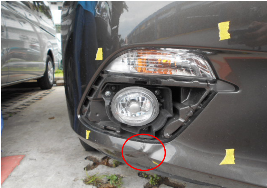
Photo 3 shows a closer view of the dislodged right front fog lamp garnish and deformed/dented (circled) front bumper, at the area directly below the right front fog lamp.
