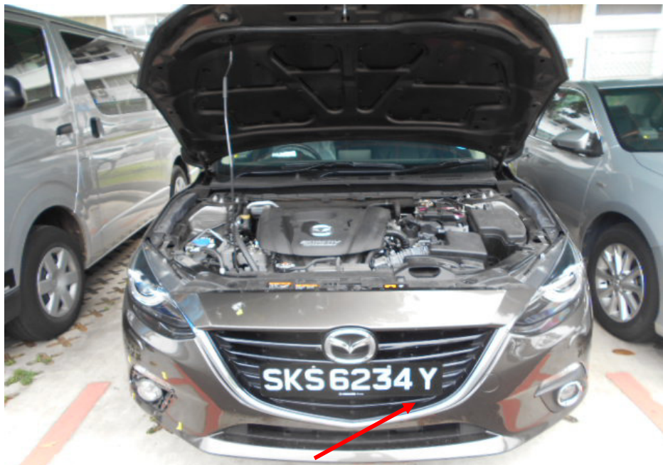
Photo 11 shows the approximate location where the other air intake opening of the Insured Vehicle is located. This was at the lower part of the front bumper (approximately arrowed), behind the radiator fan. Air for engine combustion enters the intake manifold from this opening, which is one of 2 openings for such purpose. Water had likely entered the engine of the Insured Vehicle from this opening given its relatively low height above ground level.
