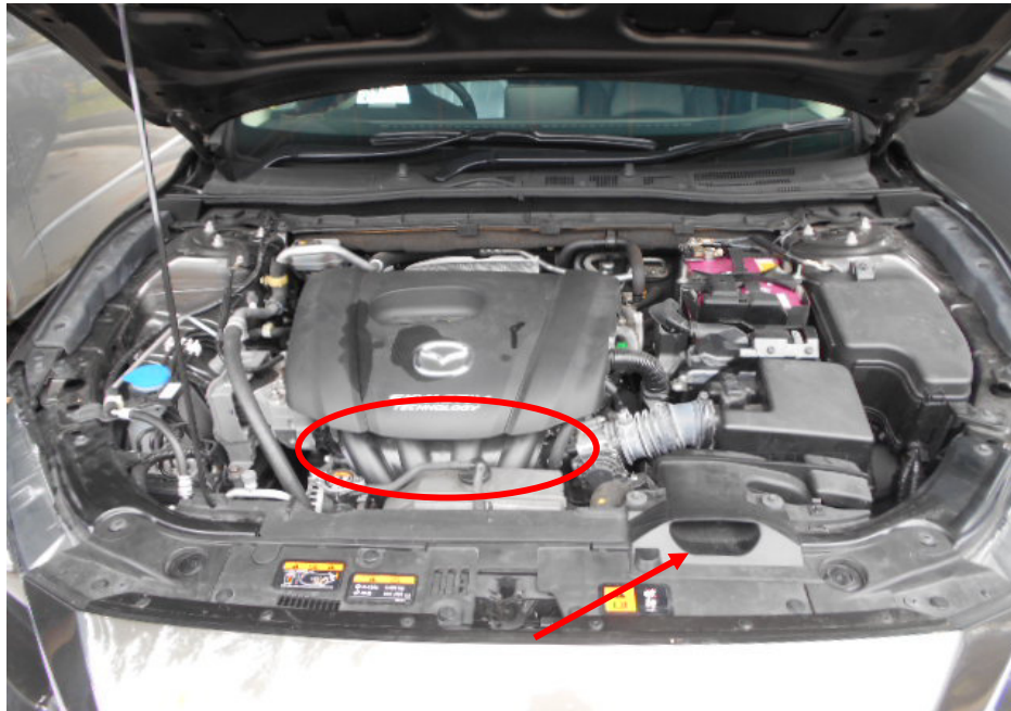
Photo 10 shows the air intake opening (arrowed) of the Insured Vehicle that is located at the front bonnet height. Air for engine combustion enters the intake manifold (circled) from this opening, which is one of 2 openings for such purpose.
