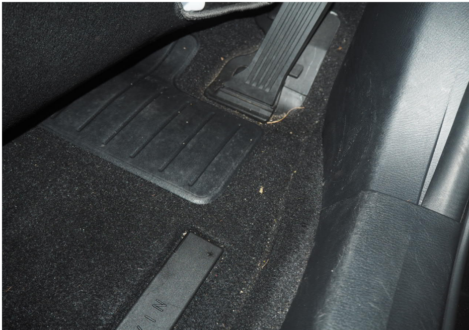
Photo 8 shows the upholstery at the driver's side of the Insured Vehicle. The upholstery was damp at the time of my inspection. This was another observation gathered from my inspection of the Insured Vehicle that corresponds to its involvement in a flood incident.
