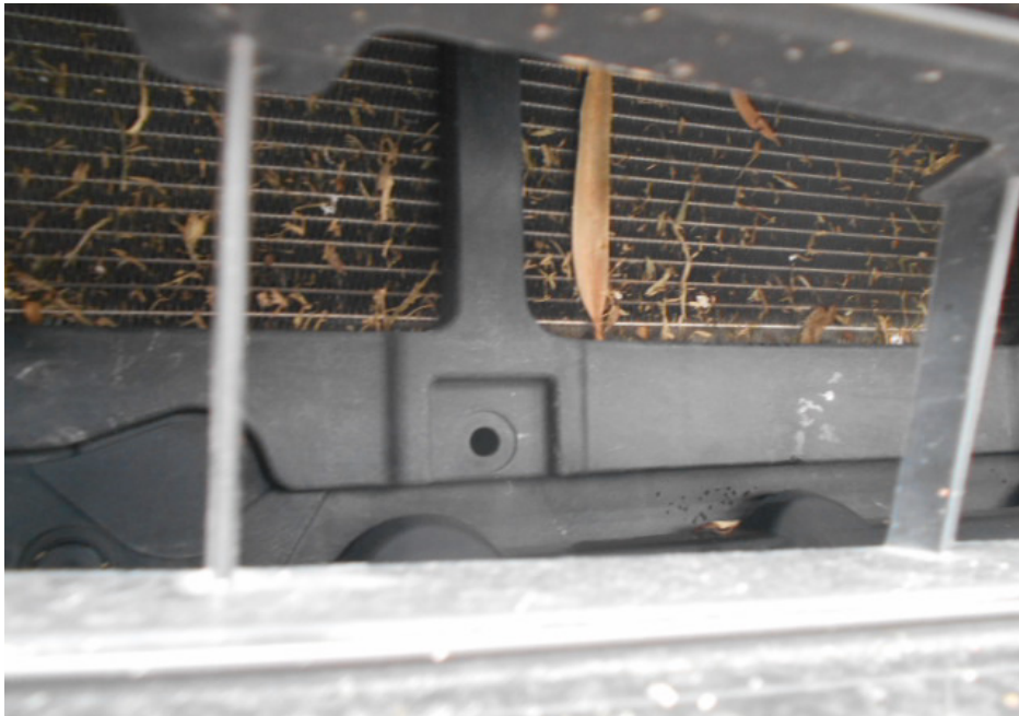
Photo 7 shows the dried leaves that were all trapped on the fins of the air condenser of the Insured Vehicle. The condition of the air condenser corresponds to the Insured Vehicle being involved in a flood incident.
