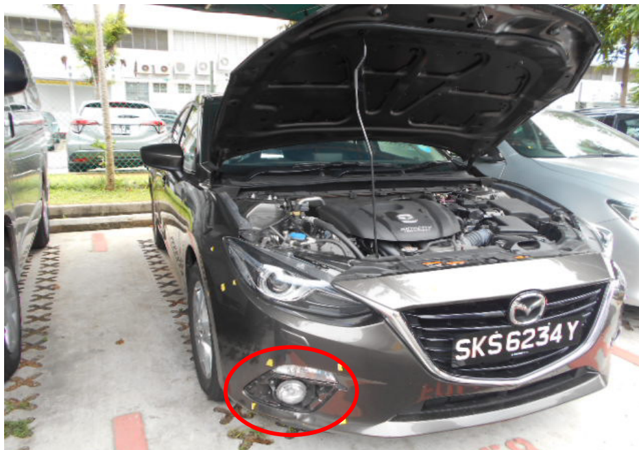
Photo 2 shows a general view of the front right body of the Insured Vehicle. Its right front fog lamp garnish was observed to be dislodged. Its front bumper, at the area directly below the right front fog lamp, was also observed to be deformed/dented (circled).
