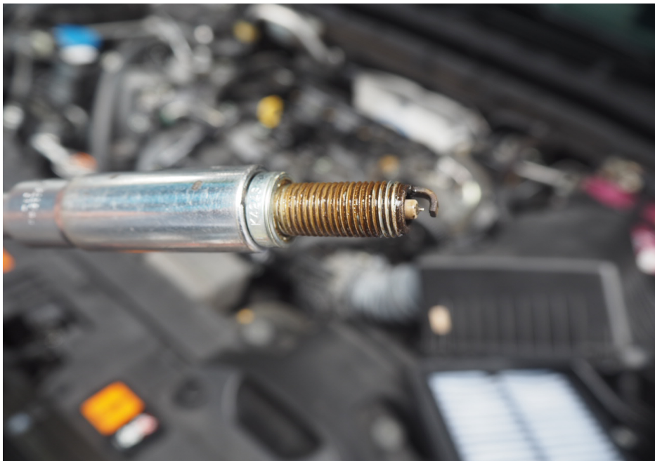
Photo 6 shows a close view of the Insured Vehicle's spark plugs. The spark plugs were seen covered with water, indicating that the Insured Vehicle was involved in a flood incident.
