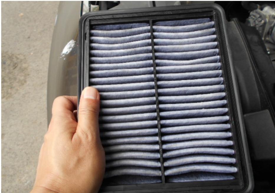
Photo 5 shows a closer view of the air filter of the Insured Vehicle. The air filter was found to be damp, which was one of the signs observed at the time of my inspection that indicate the Insured Vehicle was indeed involved in a flood incident.
