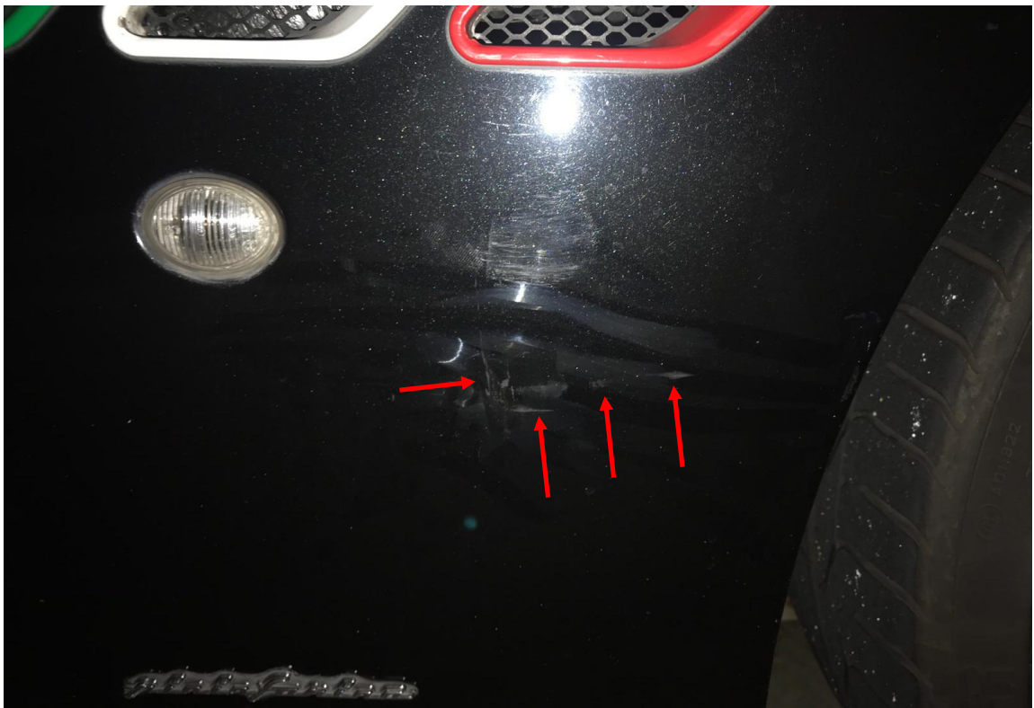
Photo 2 shows a closer view of the damaged area where the “L” shape imprint mark (arrowed) was found on the front right fender of the Third Party Vehicle. The imprint mark was a result of a load/force from a similarly shaped object pressing onto the front right fender, in a right to left direction.
