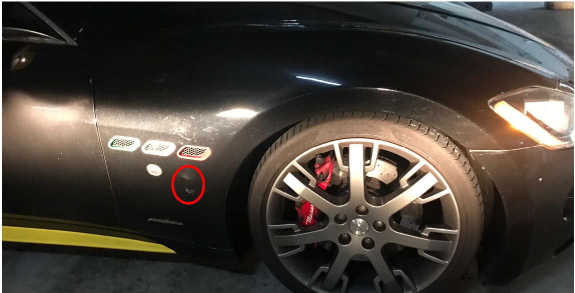
Photo 1 shows a general view of the front right body of the Third Party Vehicle at the incident scene. From the photographs at the incident scene, I had observed what appears to be an “L” shape imprint mark on the lower area of its front right fender (circled), just after the front right wheel. No other damage was seen from the photographs that I had reviewed.
