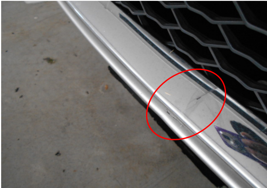
Photo 6 shows a closer view of the distorted front bumper and cracked front bumper lower grille chrome moulding (circled). These damages were at the front centre lower area of the Insured Vehicle.
