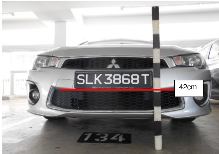
Photo 8 shows the height measurement that was conducted on the frontal body of the Insured Vehicle. The bottom horizontal end of the Insured Vehicle's front number plate casing was measured to be approximately 42cm above ground level.
