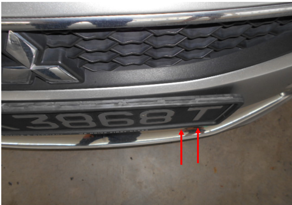
Photo 7 shows the bent front number plate and front number plate casing (arrowed) of the Insured Vehicle. This was at the left side of the front number plate, adjacent to the bottom left corner.
