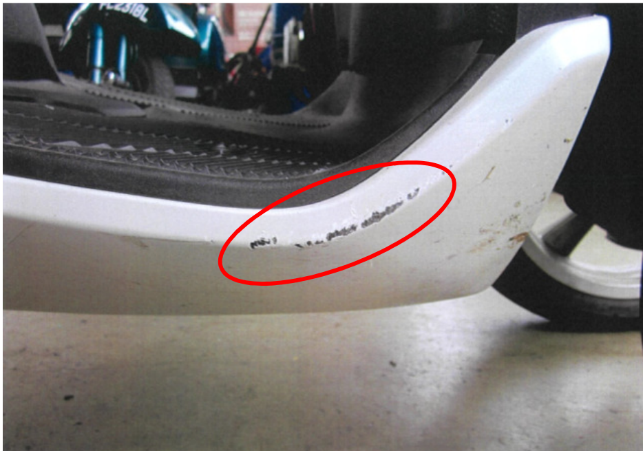
Photo 4 shows marks of grazing nature (circled) that was observed on the right side lower cover of the Motorcycle. Again, these grazing marks were a result of the Motorcycle falling and sliding along the road surface.
