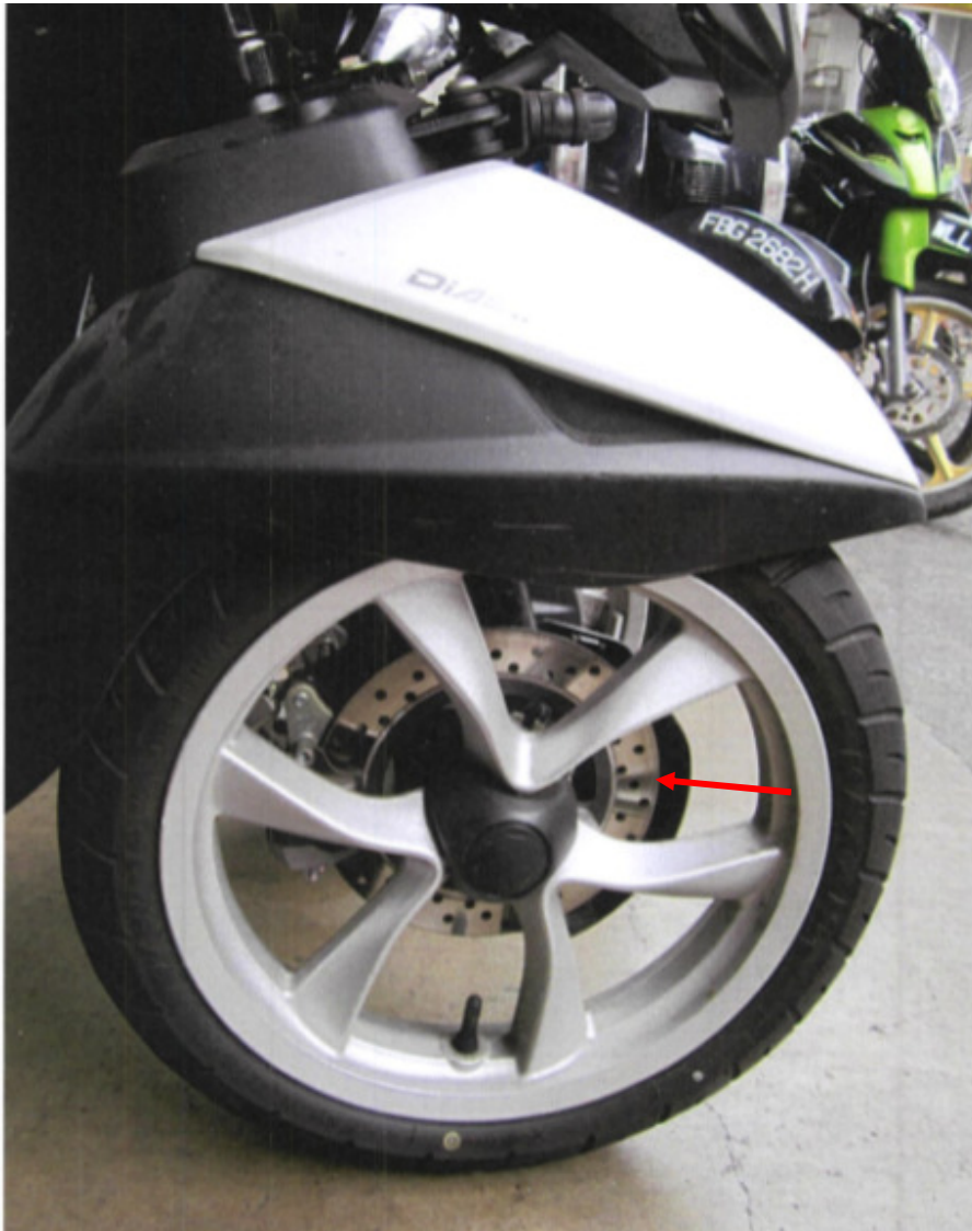
Photo 11 shows the brake disc (arrowed) at the front right wheel of the Motorcycle. The front left wheel and rear wheel of the Motorcycle were similarly fitted with such brake disc as part of the Motorcycle's braking system.
