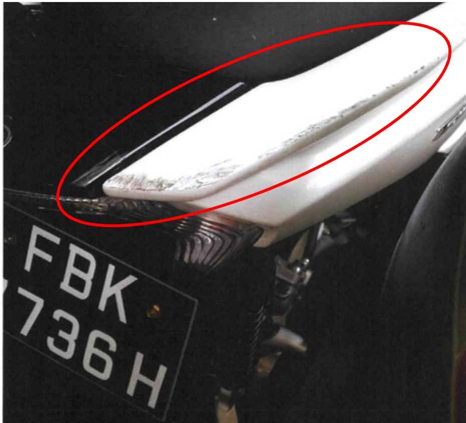
Photo 6 shows marks of grazing nature that was observed on the right side rear cover of the Motorcycle. From the damage pattern seen on the Motorcycle, it can be established that the Motorcycle had fell on its right side and thereafter slid along the road surface at the material time.
