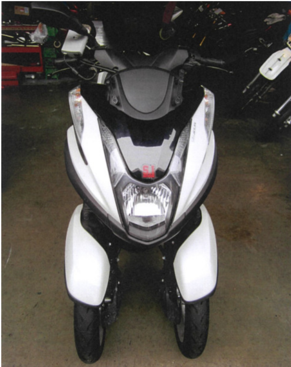
Photo 7 shows a frontal view of the Motorcycle, which is a tri-wheel type of motorcycle. Such type of motorcycle is generally more stable in terms of road handling as compared to a 2-wheel motorcycle. This is another factor that does not seem to suggest that it was possible for the Motorcycle to self-skid at the material time, especially when travelling along a straight stretch of roadway.
