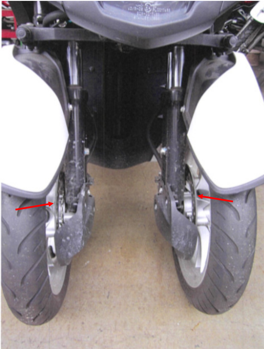
Photo 10 shows a frontal view of the Motorcycle. The braking system of the Motorcycle was of hydraulic pressure type with brake disc at all the wheels. The front wheels of the Motorcycle will stop rotating faster as compared to the rear wheel given that the frontal wheels are individually fitted with its own brake disc (arrowed).
