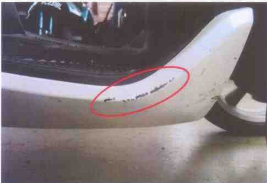
Photo 4 shows marks of grazing nature (circled) that was observed on the right side lower cover of the Motorcycle. Again, these grazing marks were a result of the Motorcycle falling and sliding along the road surface.
