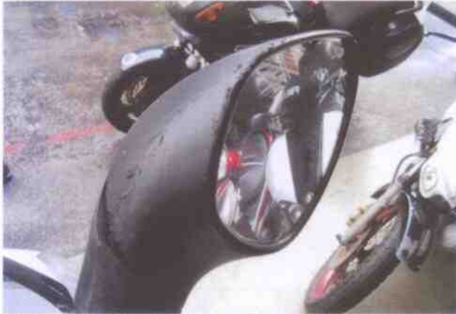
Photo 3 shows marks of grazing nature that was observed on the right side wing mirror of the Motorcycle. The grazing marks are a result of the Motorcycle falling and sliding along the road surface.
