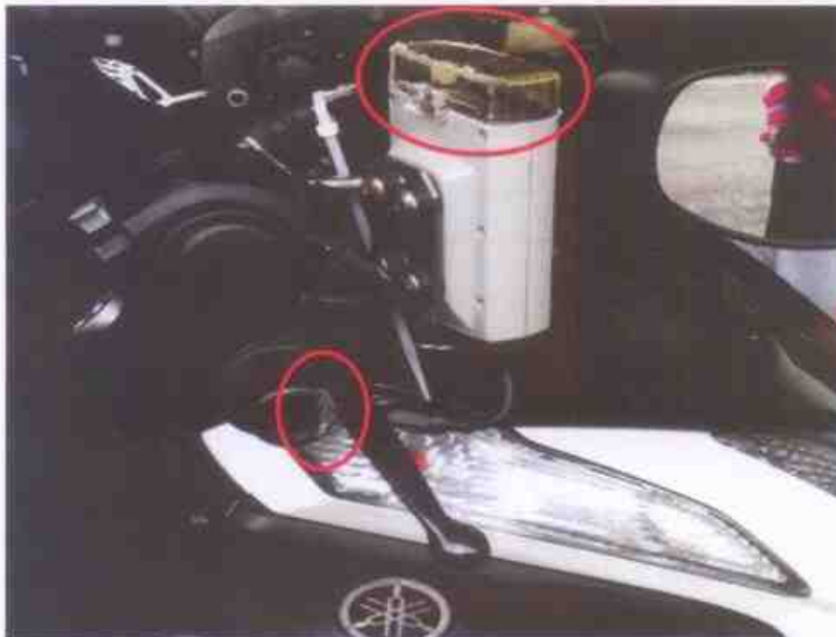
Photo 2 shows marks of grazing nature that was observed on the right side of the Motorcycle, in particular to the right side handle bar and IU cover (circled).
