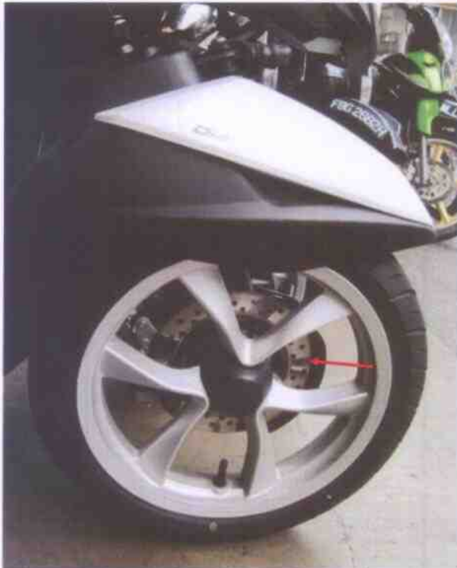
Photo 11 shows the brake disc (arrowed) at the front right wheel of the Motorcycle. The front left wheel and rear wheel of the Motorcycle were similarly fitted with such brake disc as part of the Motorcycle's braking system.
