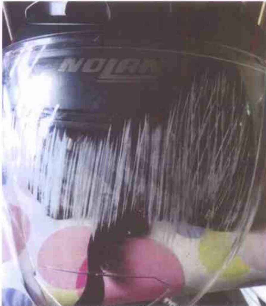
Photo 1 shows Madam Aini's helmet. The grazed/scratched marks seen on Madam Aini's helmet visor are consistent to marks that are formed by the helmet grazing against the road surface.
