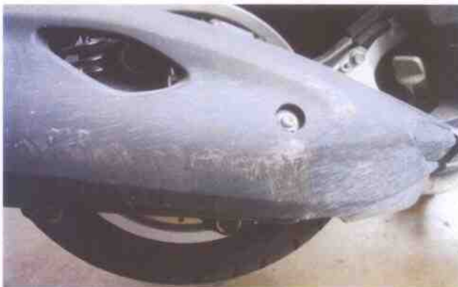
Photo 5 shows marks of grazing nature that was observed on the exhaust guard, which was on the right of the Motorcycle. Such grazing nature marks are commonly associated to a motorcycle falling and thereafter sliding along the ground.
