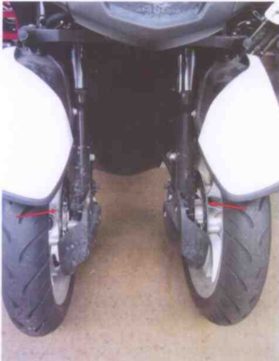
Photo 10 shows a frontal view of the Motorcycle. The braking system of the Motorcycle was of hydraulic pressure type with brake disc at all the wheels. The front wheels of the Motorcycle will stop rotating faster as compared to the rear wheel given that the frontal wheels are individually fitted with its own brake disc (arrowed).
