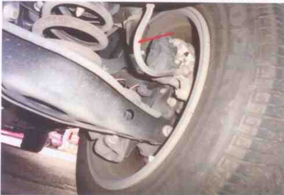
Photo 22 shows the various undercarriage components at the rear right wheel of the Motor Car. We did not observe any leakage of brake fluid at the time of our inspection of the Motor Car. Our visual inspection of the various mechanical components of the Motor Car's braking system revealed all to be intact and without visible damage, indicating that the braking system was likely to be in serviceable condition at the material time of accident.
