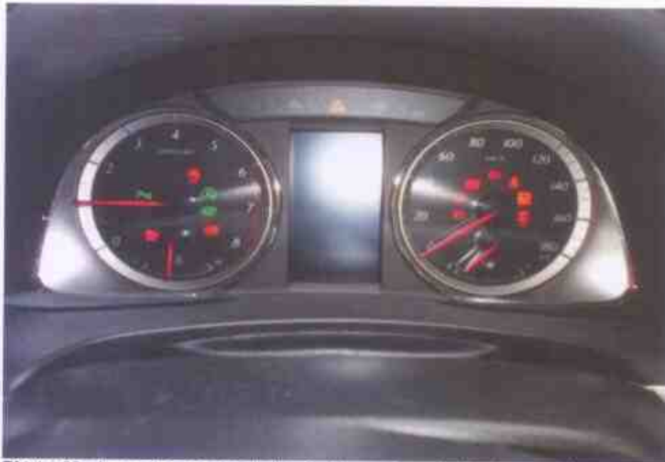
Photo 23 shows the warning lights for the various electronic operating systems of the Motor Car appearing on its instrument panel during the self-test when the engine is cranked, in particular the ABS light and SRS light.
