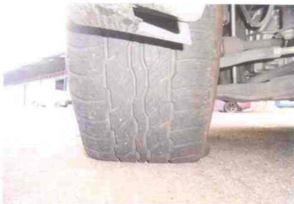
Photo 11 shows the condition of the front left tyre of the Motor Car, which was observed to be deflated as a result of the accident. The remaining tread depth however found to be at approximately 6mm.
