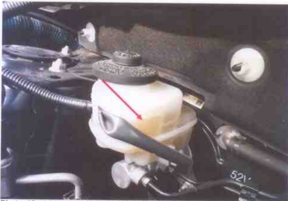
Photo 16 shows the brake fluid reservoir of the Motor Car at the time of our inspection. The brake fluid was observed to be of sufficient level (arrowed) and without any visible contamination.
