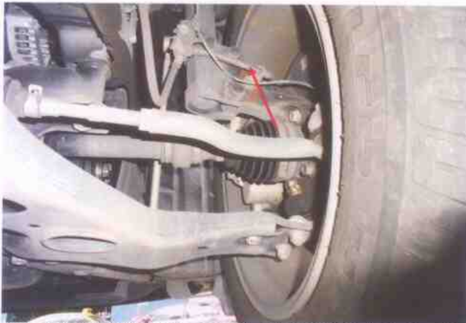
Photo 20 shows the brake hose (arrowed) at the front right wheel of the Motor Car. We did not observe any leakage of brake fluid at the time of our inspection of the Motor Car. Our visual inspection of the various mechanical components of the Motor Car's braking system, including its brake calliper, revealed all to be intact and without visible damage
