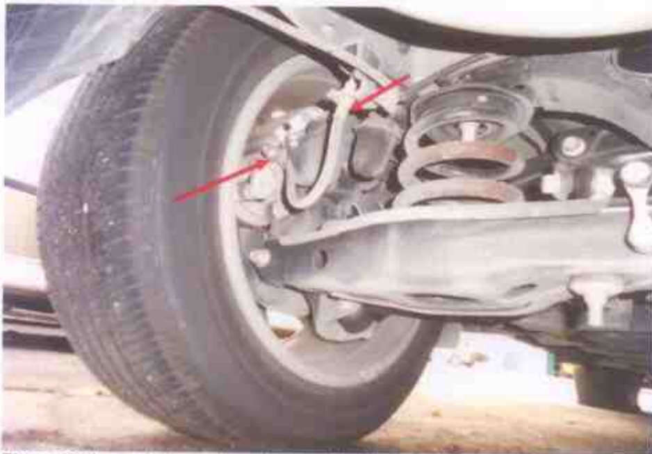
Photo 19 shows the brake hose (arrowed) at the rear left wheel of the Motor Car. We did not observe any leakage of brake fluid at the time of our inspection of the Motor Car. Our visual inspection of the various mechanical components of the Motor Car's braking system revealed all to be intact and without visible damages.
