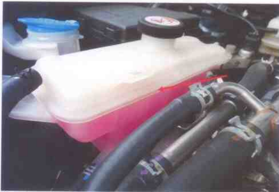
Photo 17 shows the coolant fluid in the radiator tank of the Motor Car at the time of our inspection. The coolant fluid was observed to be of sufficient level and without any visible contamination.
