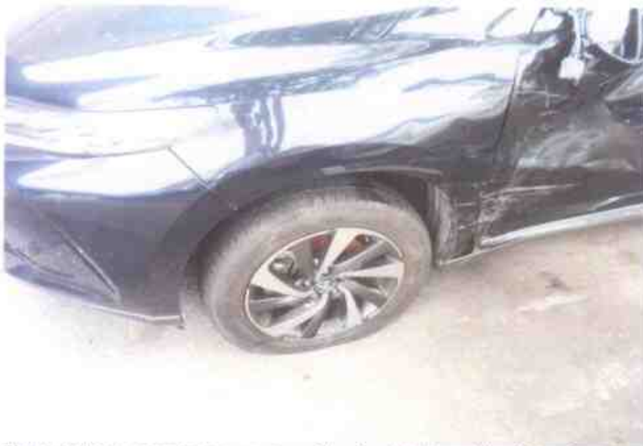
Photo 6 shows a semi-close up view of the front left tyre of the Motor Car at the time of our inspection. It was observed to be deflated as a result of the accident.
