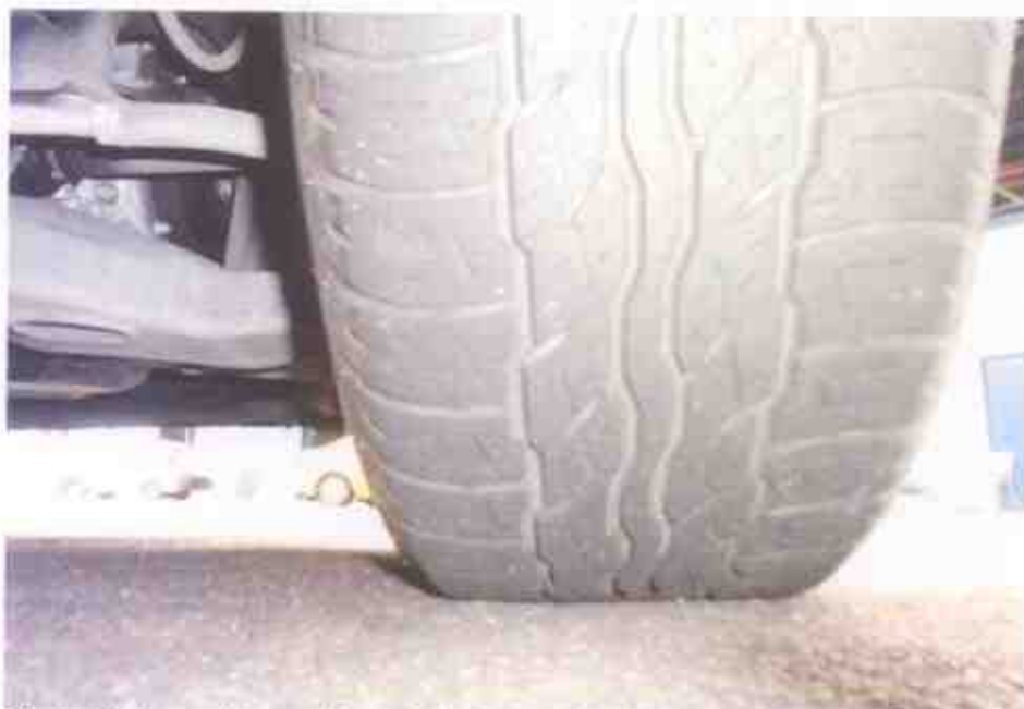
Photo 12 shows the condition of the front right tyre of the Motor Car, which was observed to be in serviceable condition with remaining tread depth of approximately 6mm. The tyre, which was wrapped around alloy wheel rim, was also observed to be sufficiently inflated for vehicular operation.
