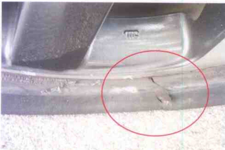
Photo 10 shows the condition of the front left tyre of the Motor Car, which was observed to be deflated as a result of the accident. Torn mark was found at the outer sidewall. The remaining tread depth of approximately 6mm.
