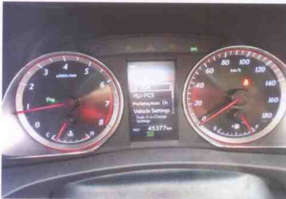
Photo 24 shows: no warning lights illuminated on the instrument panel of the Motor Car after the engine was cranked. This would suggest that there was no abnormality to the various electronic operating systems of the Motor Car, like the ABS and SRS.
