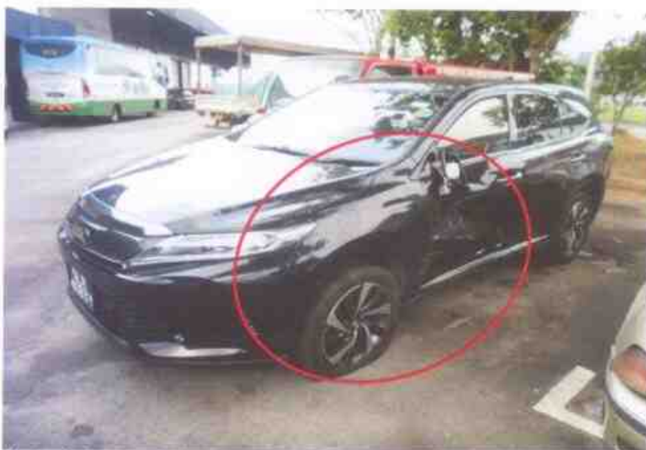
Photo 4 shows a semi close up view of the front left portion of the Motor Car at the time of our inspection. The Motor Car had sustained relatively minor impact at the front left of the Motor Car including the tyre that was observed to be deflated as a result of the accident.
