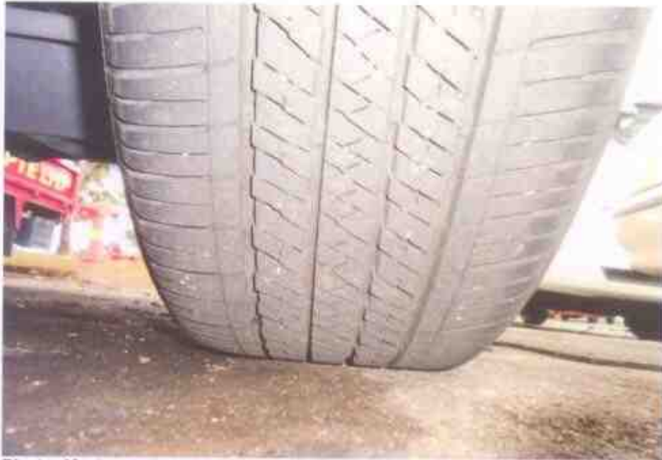
Photo 13 shows the condition of the rear left tyre of the Motor Car, which was observed to be in serviceable condition with remaining tread depth of approximately 7mm. The tyre, which was wrapped around alloy wheel rim, was also observed to be sufficiently inflated for vehicular operation.
