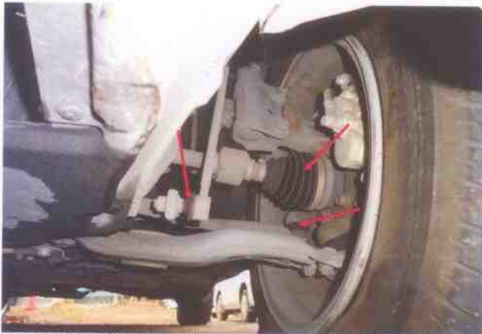
Photo 21 shows the various undercarriage components at the front left wheel of the Motor Car, in particular the steering tie rod (arrowed). The various steering components were all found to be intact, suggesting that the steering system of the Motor Car was likely to be in serviceable condition.
