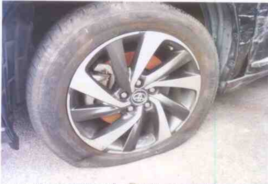
Photo 9 shows the condition of the front left tyre of the Motor Car, which was observed to be deflated as a result of the accident. Torn mark was found at the outer sidewall. The remaining tread depth of approximately 6mm.
