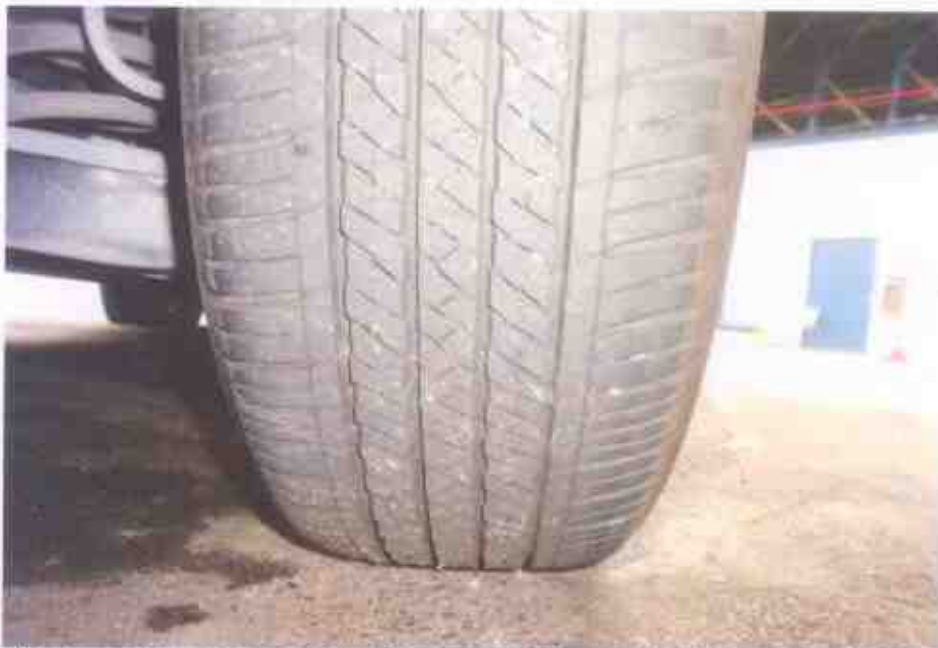
Photo 14 shows the condition of the rear right tyre of the Motor Car, which was observed to be in serviceable condition with remaining tread depth of approximately 7mm. There was also no tear, cut or burst mark(s) on the outer and the inner sidewalls as well as across the tread of the 4 tyres.
