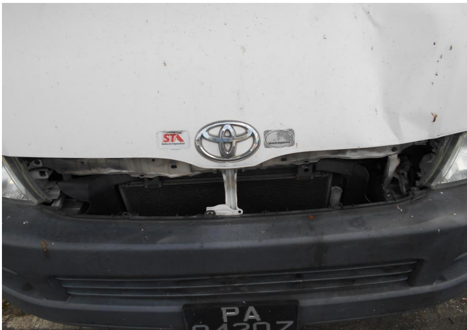
Photo 4 shows a close-up view of the dislodged front grille of the Motor Bus at the time of our inspection. It was observed to have sustained with minor damage likely due to the accident.
