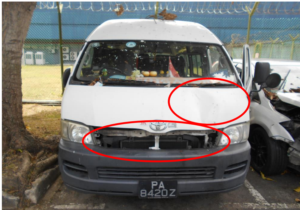
Photo 2 shows a general view of the front right body of the Motor Bus at the time of our inspection. The Motor Bus was observed to sustained minor damage at the front left panel & front grille.
