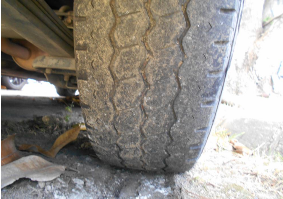
Photo 11 shows the condition of the rear right tyre of the Motor Bus, which was observed to be in serviceable condition with remaining tread depth of approximately 3mm. There was also no tear, cut or burst mark(s) on the outer and the inner sidewalls as well as across the tread of the tyre, which was also sufficiently inflated for vehicular operation.
