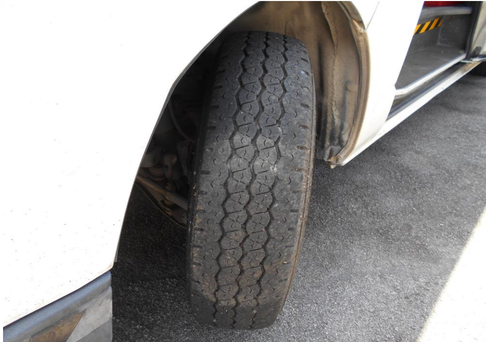
Photo 9 shows the condition of the front left tyre of the Motor Bus, which was observed to be in serviceable condition with remaining tread depth of approximately 7mm. The tyre, which was wrapped around standard wheel rim, was also observed to be sufficiently inflated for vehicular operation.
