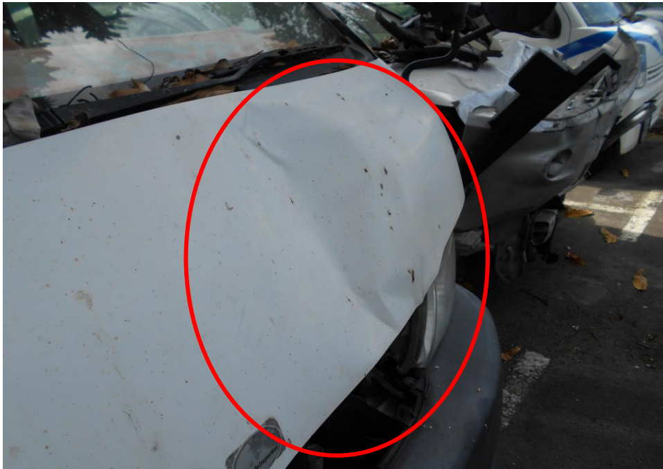
Photo 3 shows a close-up view of the dent on the front left panel of the Motor Bus at the time of our inspection. It was observed to have sustained with minor damage likely due to the accident.
