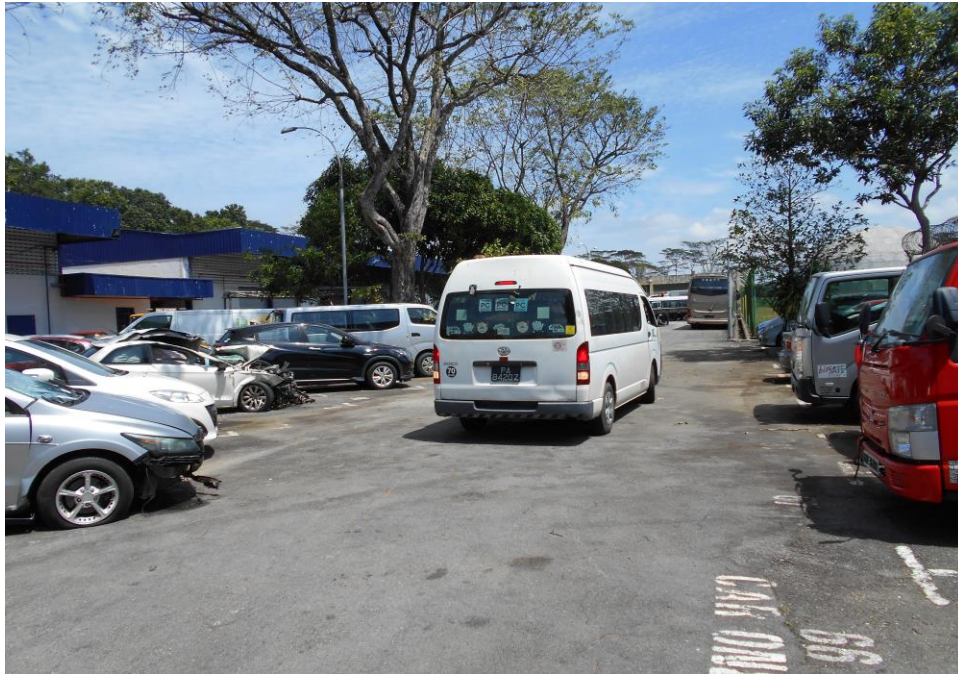
Photo 23 shows a short operational test of the Motor Bus, the test was conducted by driving the Motor Bus forward, stopping, before reversing and coming to a stop again.
