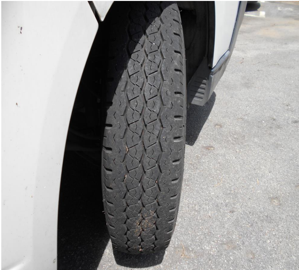
Photo 8 shows the condition of the front right tyre of the Motor Bus, which was observed to be in serviceable condition with remaining tread depth of approximately 8mm. The tyres were all observed to be sufficiently inflated for vehicular operation with no tear, cut or burst mark(s) on the outer and the inner sidewalls as well as across the tread.
