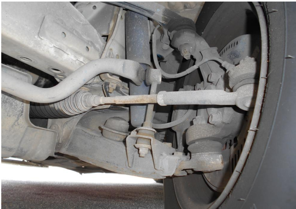
Photo 18 shows the brake hose at the front left wheel of the Motor Bus. We did not observe any leakage of brake fluid. Our visual inspection of the various mechanical components of the Motor Bus's braking system revealed all to be intact and without visible damage, indicating that the braking system was likely to be in serviceable condition at the material time of accident.
