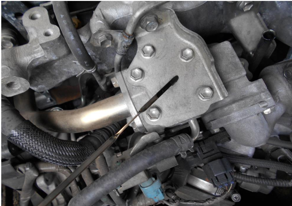
Photo 16 shows the engine dip stick of the Motor Bus at the time of our inspection. The engine oil was observed to be of sufficient level and without any visible contamination.
