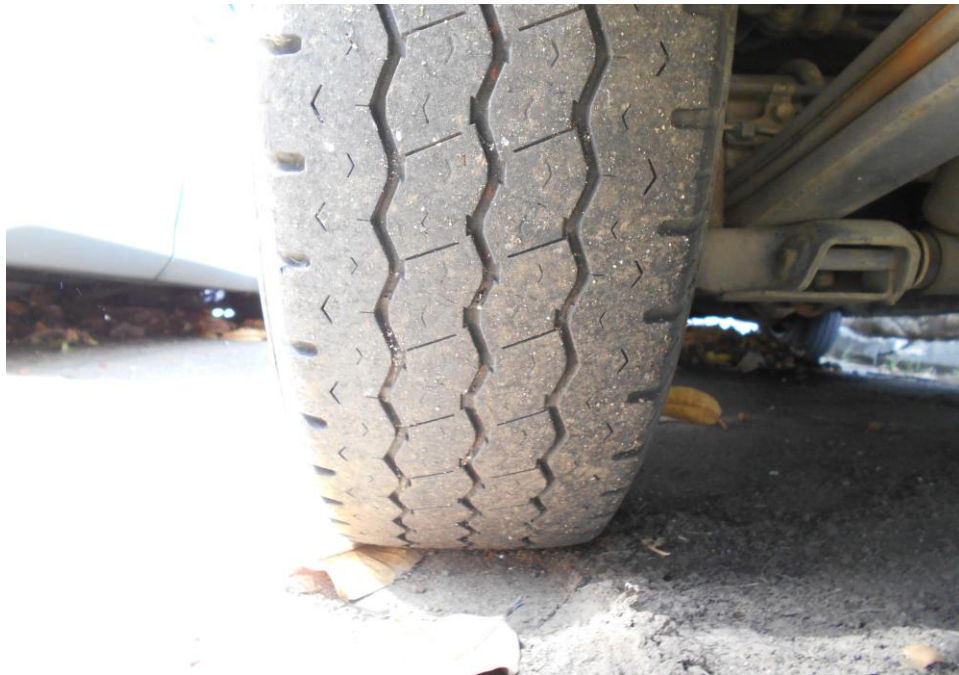
Photo 10 shows the condition of the rear left tyre of the Motor Bus, which was observed to be in serviceable condition with remaining tread depth of approximately 5mm. The tyre, which was wrapped around standard wheel rim, was also observed to be sufficiently inflated for vehicular operation. There was also no significant damage found on the 4 wheel rims of the Motor Bus.
