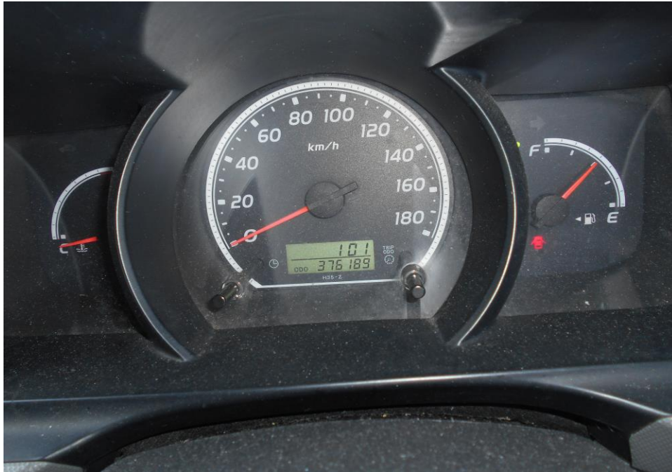
Photo 22 shows no warning lights illuminated on the instrument panel of the Motor Bus after the engine was cranked. This would suggest that there was no abnormality to the various electronic operating systems of the Motor Car.
