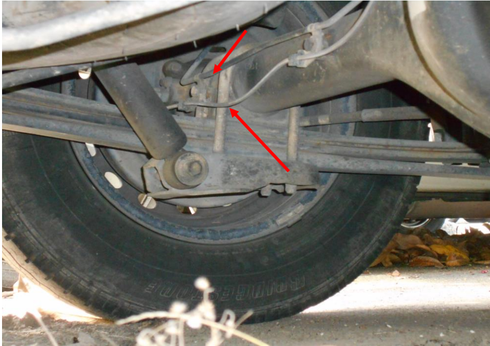
Photo 17 shows the various undercarriage components at the rear left wheel of the Motor Bus, in particular the brake hose (arrowed). We did not observe any leakage of brake fluid at the time of our inspection of the Motor Bus.
