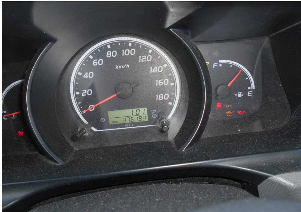
Photo 21 shows the warning lights for the various electronic operating systems of the Motor Bus appearing on its instrument panel during the self-test when the engine was cranked.
