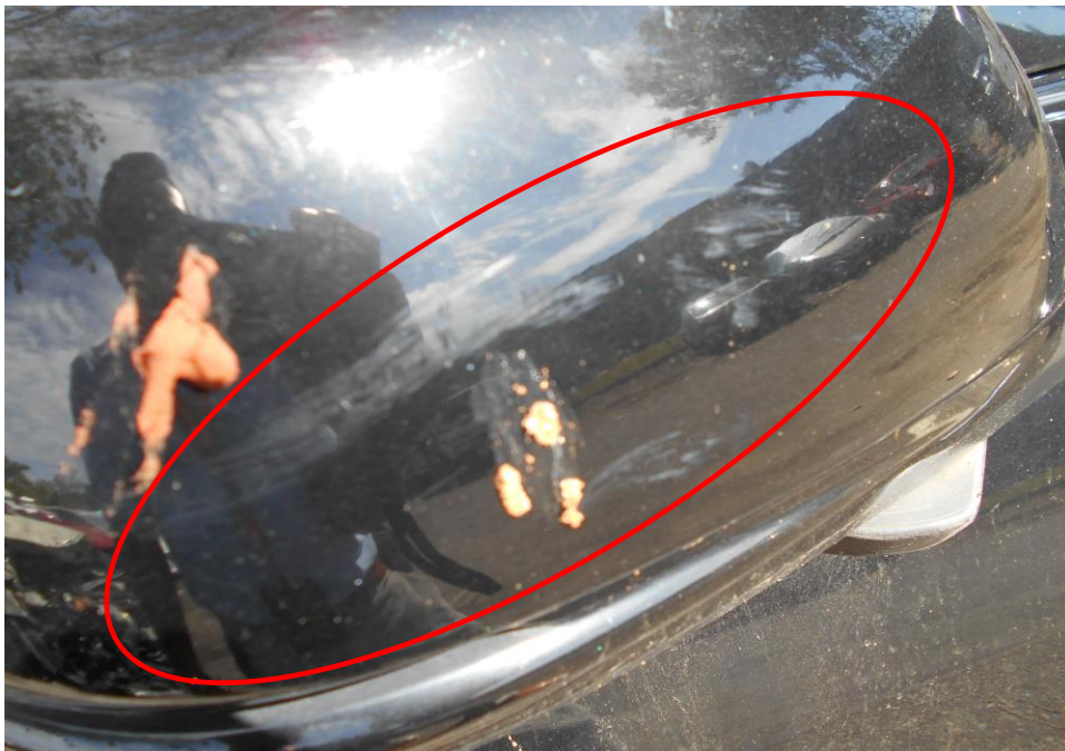
Photo 6 shows a close up view of the right wing mirror at the time of our inspection. It had sustained minor scratches at the right side portion due to the accident.
