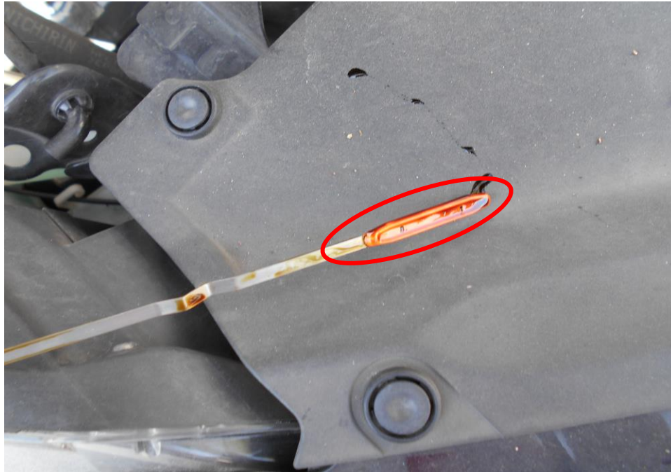
Photo 15 shows the engine oil dip stick of the Motor Car at the time of our inspection. The engine oil was observed to be of sufficient level and without any visible contamination.
