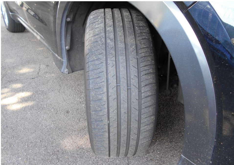
Photo 9 shows the condition of the front right tyre of the Motor Car, which was observed to be in serviceable condition with remaining tread depth of approximately 4mm. The tyre was also observed to be sufficiently inflated for vehicular operation.
