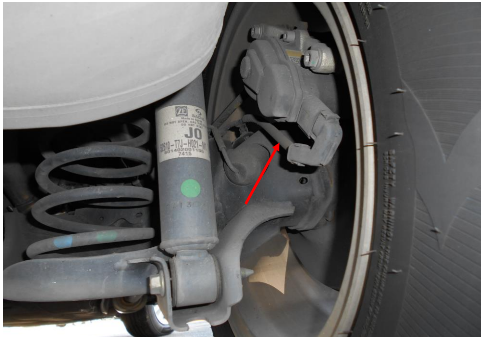
Photo 19 shows the various undercarriage components at the rear right wheel of the Motor Car. We did not observe any leakage of brake fluid at the time of our inspection of the Motor Car. Our visual inspection of the various mechanical components of the Motor Car's braking system revealed all to be intact and without visible damage, indicating that the braking system was likely to be in serviceable condition at the material time of accident.
