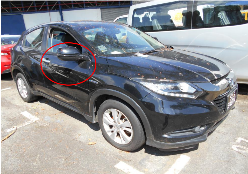
Photo 3 shows a general view of the right front body of the Motor Car at the time of our inspection. The Motor Car was observed to be in good general condition except for minor scratches at the right side portion.
