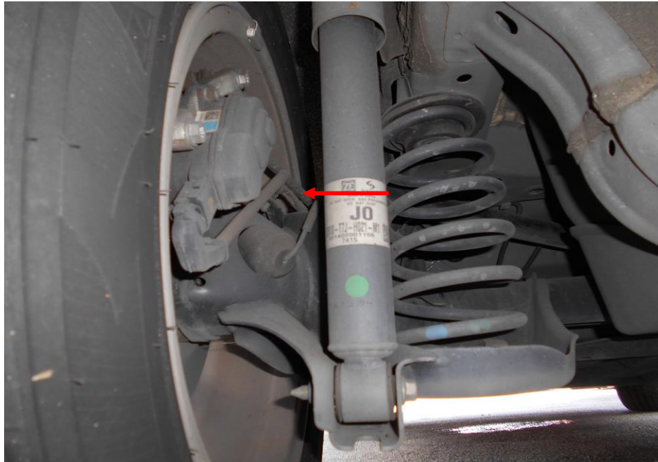
Photo 16 shows the brake hose (arrowed) at the rear left wheel of the Motor Car. Our visual inspection of the various mechanical components of the Motor Car's braking system revealed all to be intact and without visible damage, indicating that the braking system was likely to be in serviceable condition at the material time of accident.
