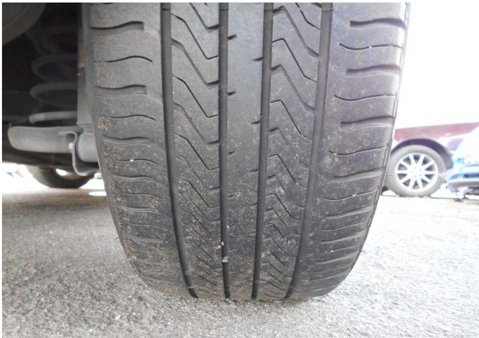
Photo 11 shows the condition of the rear right tyre of the Motor Car, which was observed to be in serviceable condition with remaining tread depth of approximately 7mm.
