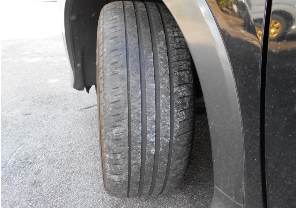
Photo 8 shows the condition of the front left tyre of the Motor Car, which was observed to be in serviceable condition with remaining tread depth of approximately 4mm. The tyre was also observed to be sufficiently inflated for vehicular operation.
