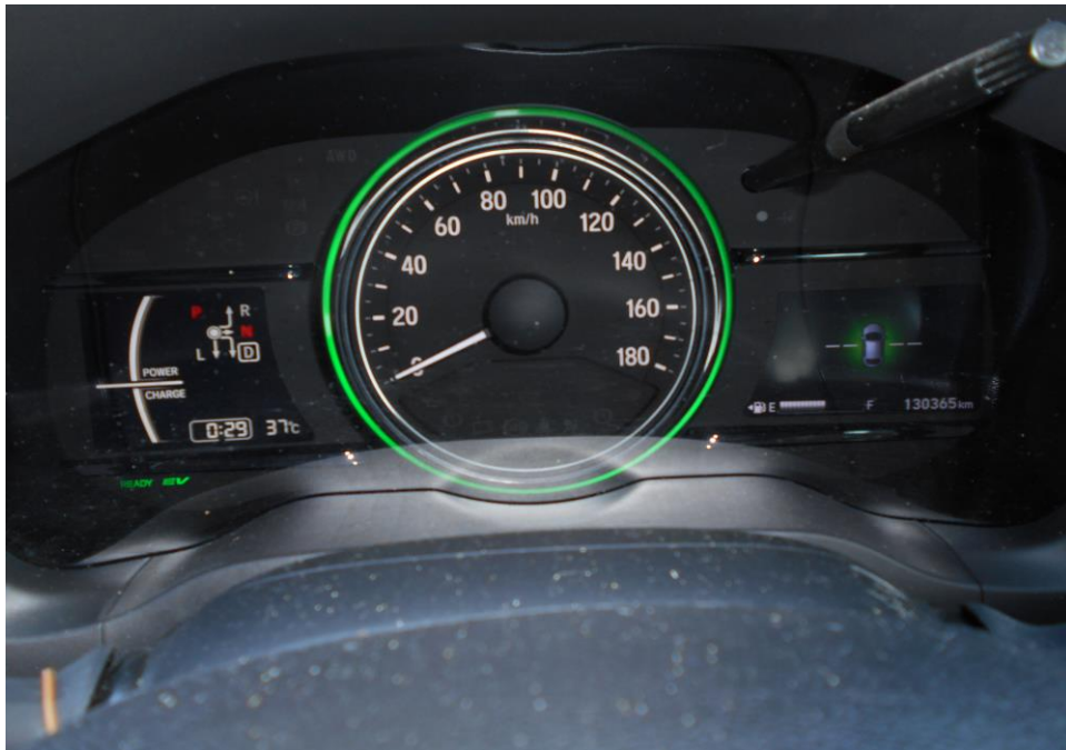
Photo 20 shows no warning lights illuminated on the instrument panel of the Motor Car after the engine was cranked. This would suggest that there was no abnormality to the various electronic operating systems of the Motor Car, like the ABS and SRS.
