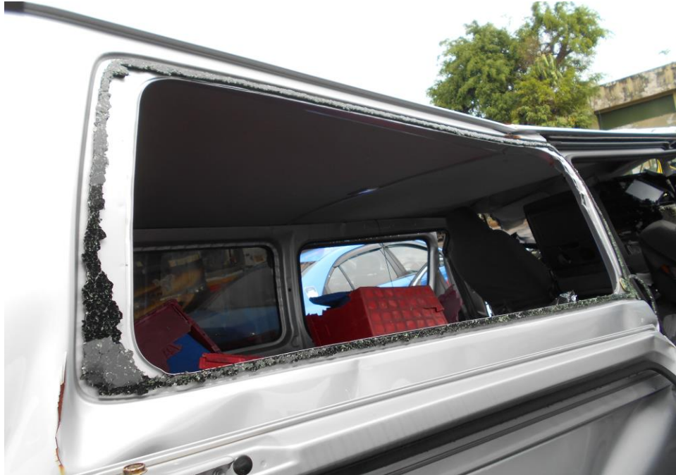
Photo 12 shows a closer view of the damaged left passenger door of the Motor Van. The impact force was significant, causing the window glass to be shattered.
