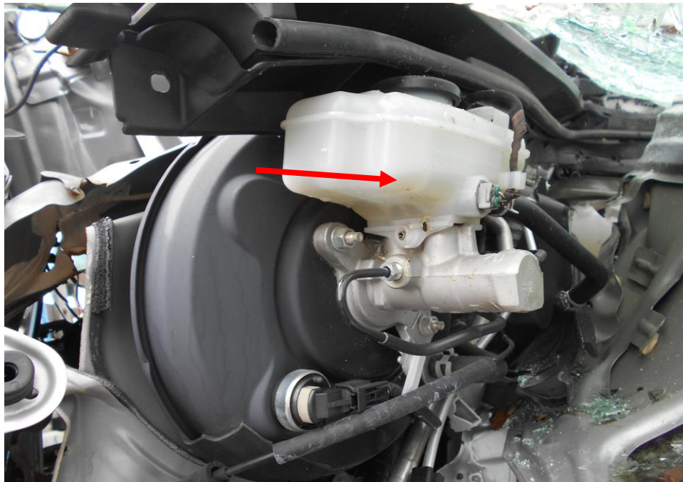
Photo 20 shows the close up view of the brake fluid reservoir that indicates empty content likely due to the accident impact.
