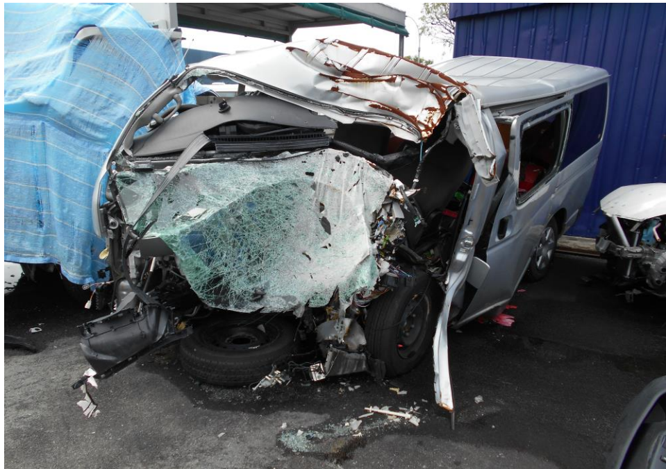
Photo 1 shows a general view of the frontal portion of the Motor Van at the time of our inspection. The Motor Van was observed to have sustained extensive impact damage at its frontal portion. The impact force was significant, causing the various parts and components inside the engine compartment to be damaged.
