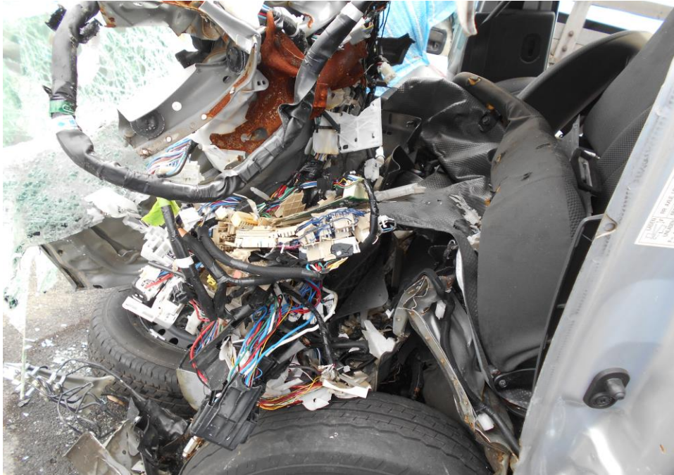
Photo 6 shows a closer view of the damage at the frontal left portion of the Motor Van. The impact force was significant, causing the various parts and components inside the engine compartment to be pushed inwards, towards the rear of the Motor Van.
