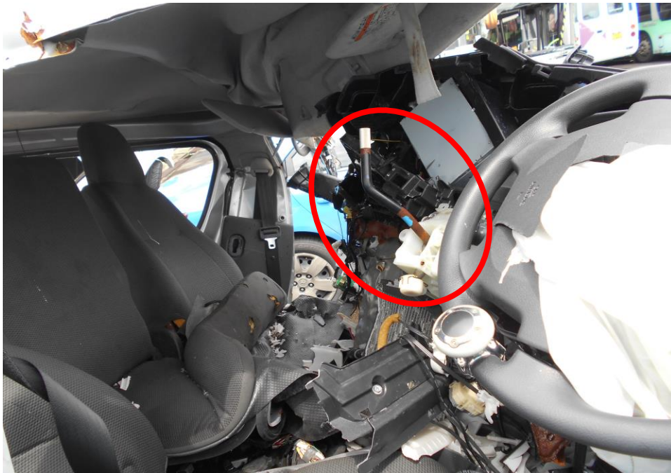
Photo 23 shows the close up view of the gear knob that was observed to be damaged due to the accident's impact.
