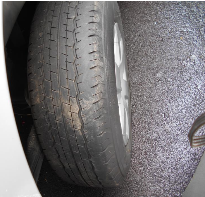
Photo 19 shows the condition of the rear right tyres of the Motor Lorry, which were observed to be in serviceable condition with remaining, tread depth of approximately 5mm.
