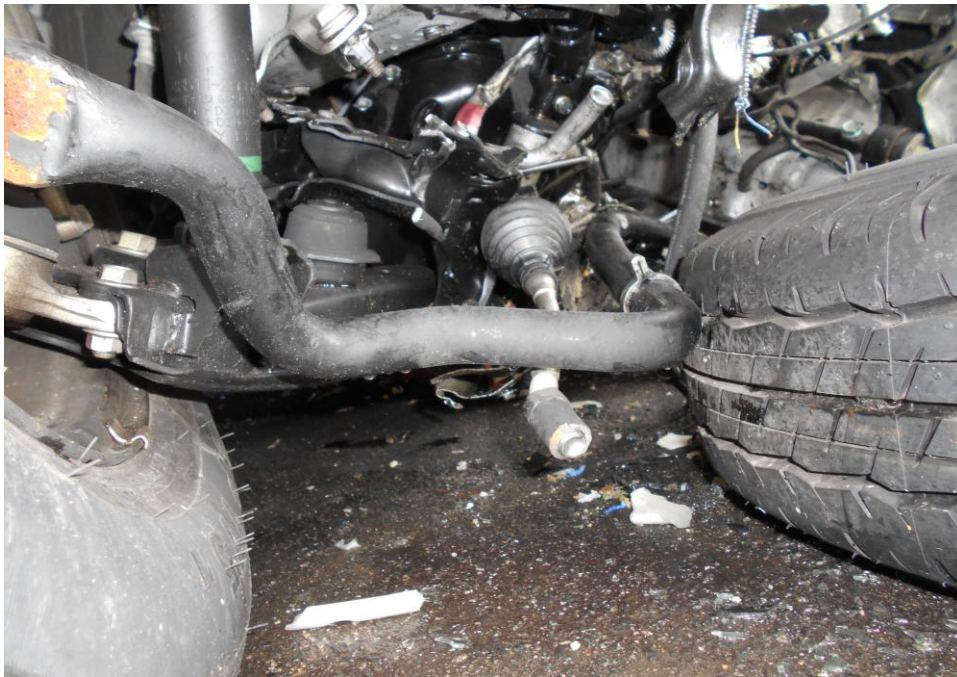
Photo 21 shows the close up view of the undercarriage which was observed to be damaged and fluid leakage observed as a result of the accident.
