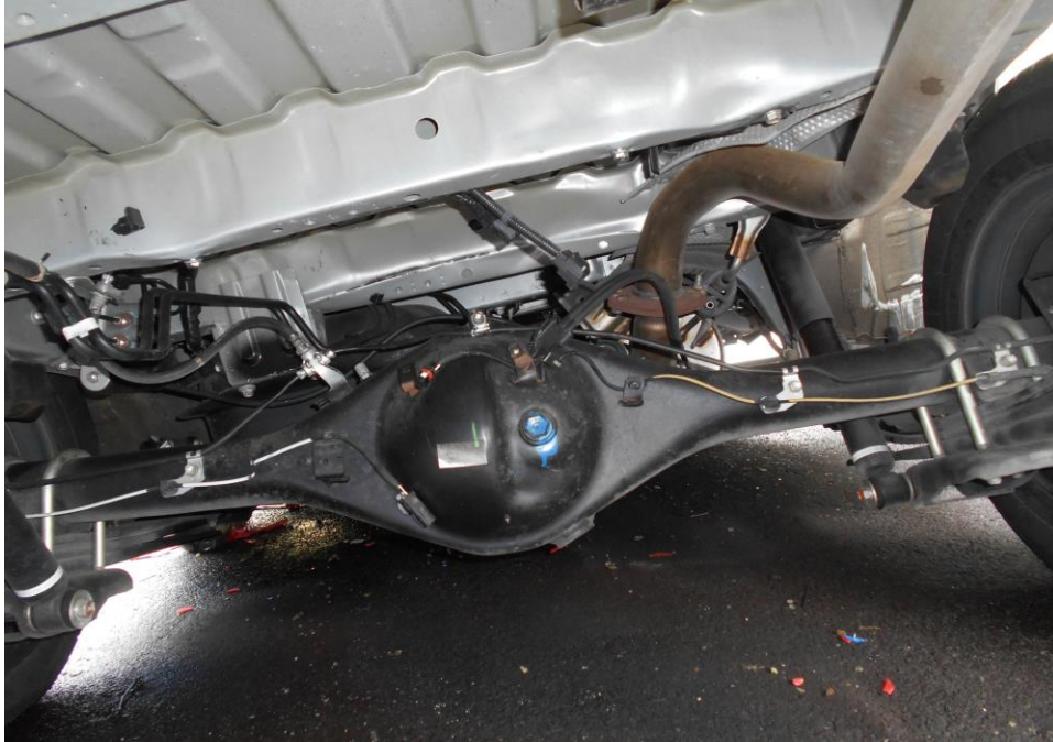
Photo 28 shows the rear axle of the Motor Van. It was observed to be in good condition at the time of our inspection of the Motor Van.
