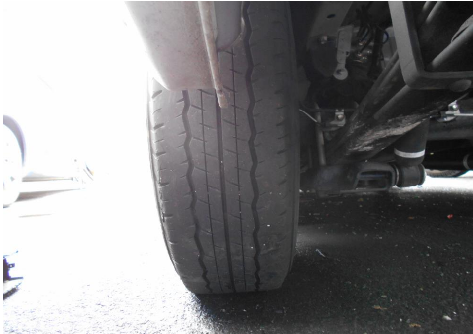
Photo 18 shows the condition of the rear left tyres of the Motor Van, which was observed to be in serviceable condition with remaining tread depth of approximately 5mm. The tyres, which were wrapped around standard alloy wheel rim, were also observed to be sufficiently inflated for vehicular operation.
