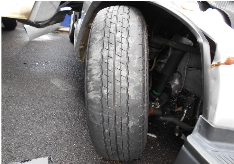
Photo 17 shows the condition of the front right tyre of the Motor Van, which was observed to be in serviceable condition with remaining tread depth of approximately 4mm. The tyre, which was wrapped around standard steel wheel rim, was also observed to be sufficiently inflated for vehicular operation.
