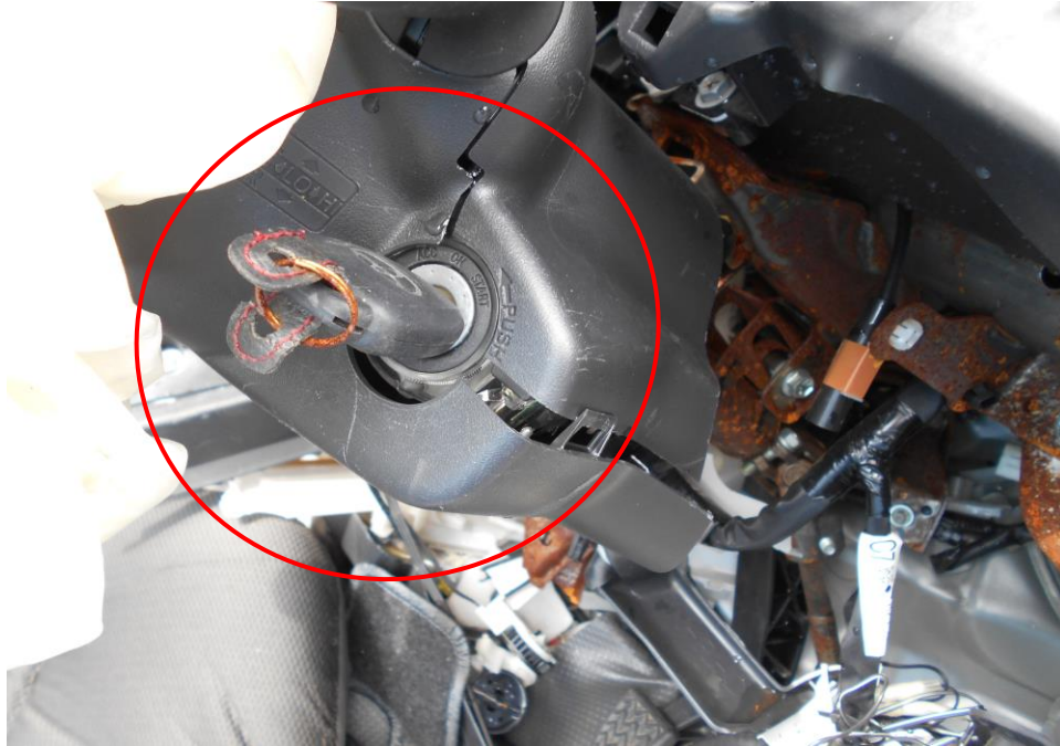
Photo 8 shows a closer view of the damage at the ignition section of the Motor Van. The impact force was significant, causing the various parts and components inside the interior compartment to be pushed inwards, including its ignition system.
