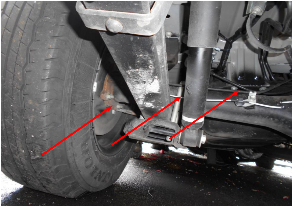
Photo 27 shows the braking component at the left right wheel of the Motor Van. We did not observe any leakage of brake fluid at the time of our inspection of the Motor Van.
