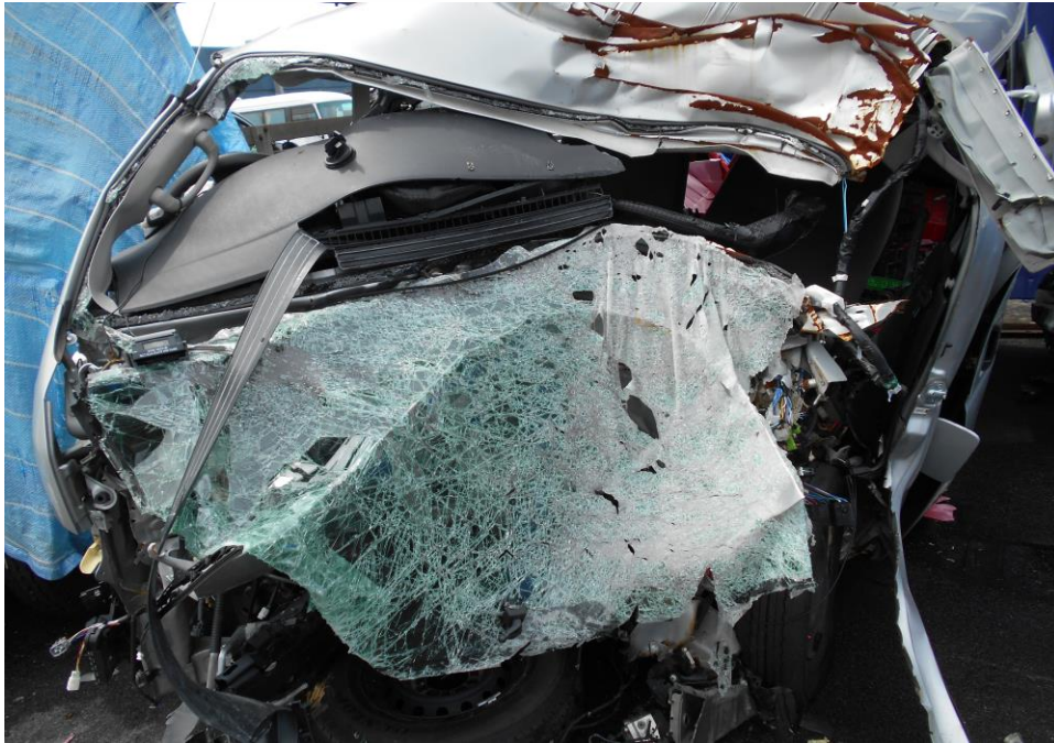
Photo 4 shows a closer view of the damage at the frontal portion of the Motor Van's engine. The impact force was significant, causing the various parts and components inside the engine compartment to be pushed inwards, towards the rear of the Motor Van.
