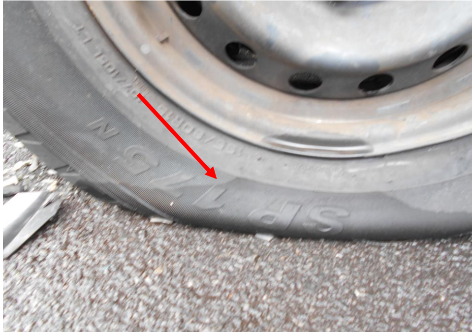
Photo 16 shows the condition of the front left tyre of the Motor Van, which was found to be punctured by the Motor Van's body metal part & deflated as a result of the accident.
