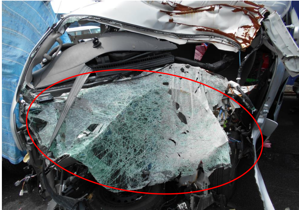
Photo 10 shows a closer view of the damage at the windscreen area of the Motor Van. The impact force was significant, causing the windscreen to sustain a shattering cracked.
