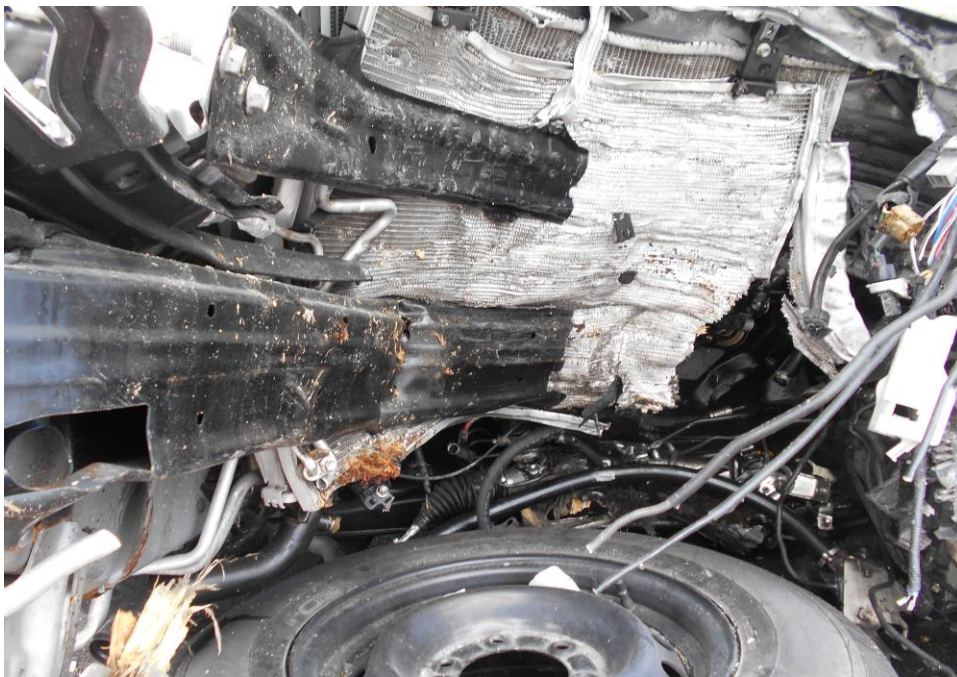
Photo 5 shows a closer view of the damage at the frontal right portion of the Motor Van. The impact force was significant, causing the various parts and components inside the engine compartment to be pushed inwards, towards the rear of the Motor Van.
