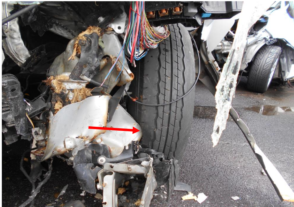
Photo 15 shows the condition of the front left tyre of the Motor Van, which was found to be punctured by the Motor Van's body metal part & deflated. However, the tread pattern was still visible (4mm).
