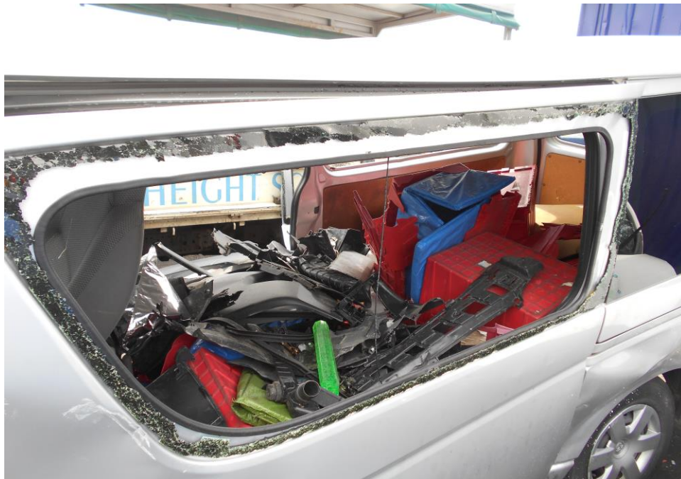
Photo 11 shows a closer view of the damaged left passenger door of the Motor Van. The impact force was significant, causing the window glass to be shattered.
