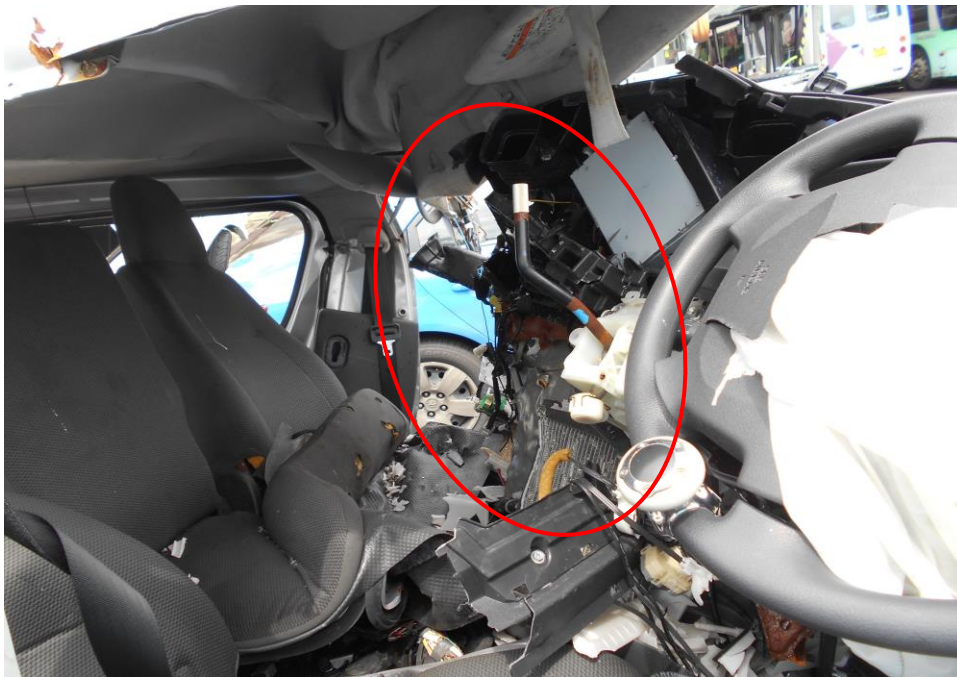
Photo 7 shows a closer view of the damage gear knob at the interior portion of the Motor Van. The impact force was significant, causing the various parts and components inside the engine compartment to be pushed inwards, towards the rear of the Motor Van including its transmission system.
