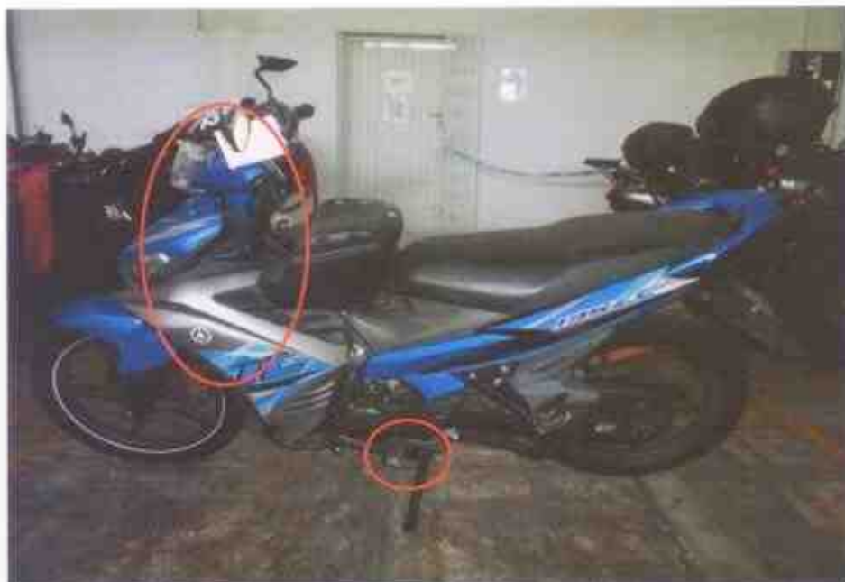
Photo 5 shows a general view of the left body of the Motorcycle at the time of our inspection. The Motorcycle was observed to have sustained relatively minor damages on the left side at time of our inspection.
