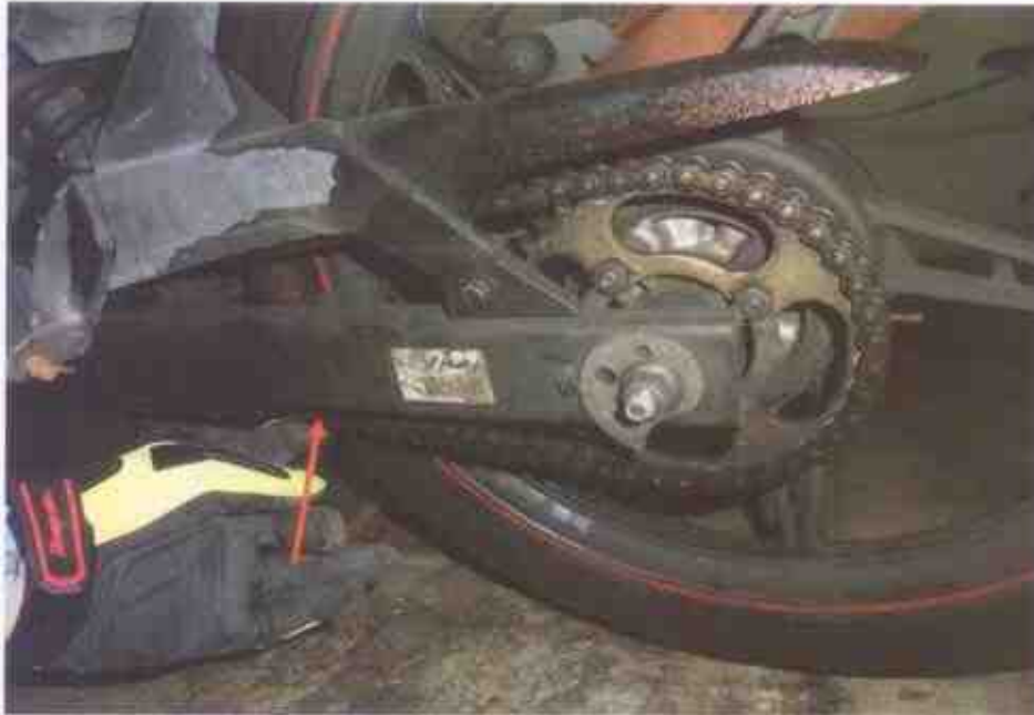
Photo 11 shows the general view of the gear train (arrowed) of the Motorcycle, which was observed to be intact with no misalignment. It was also adequately lubricated for operating purposes. Free play tension was also observed & found adequately acceptable.
