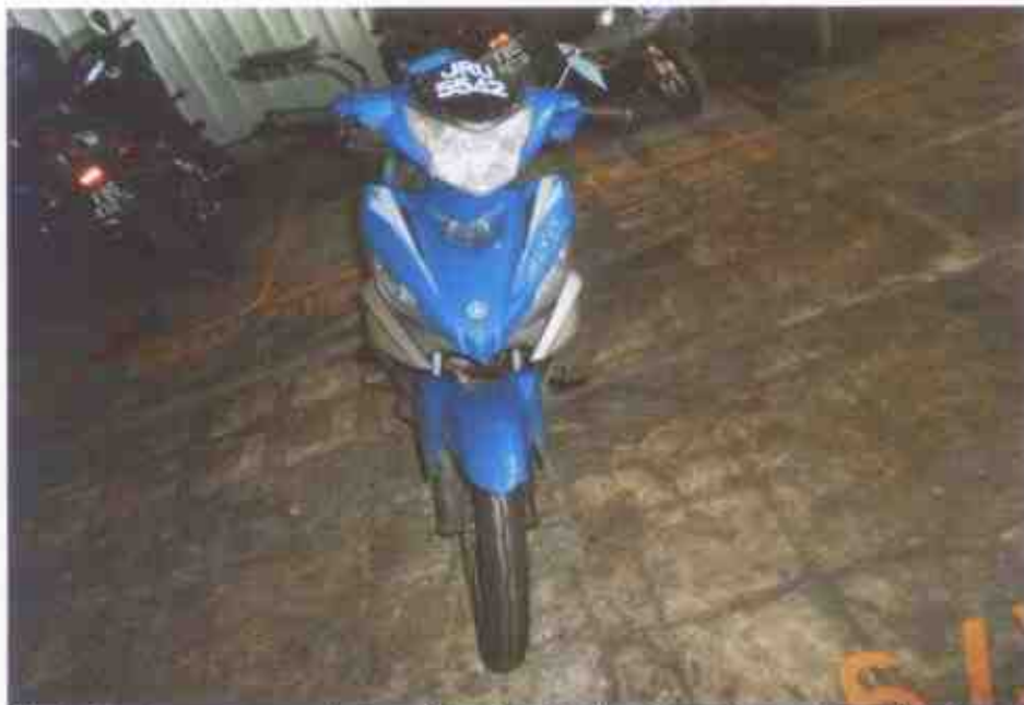
Photo 2 shows a general view of the front body of the Motorcycle at the time of our inspection. The Motorcycle was observed to have sustained relatively minor damages at time of inspection. The damages were observed to be confined to its left side which includes scratches on the left fairing & foot rest.
