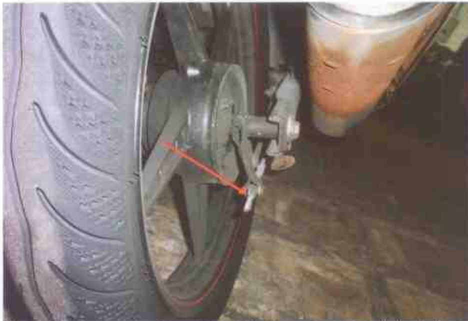
Photo 13 shows our checks on the rear brake components had also indicated that the brake mechanism was in serviceable condition at the material time of the accident.
