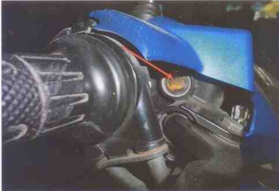
Photo 12 shows our checks on the brake fluid (front) reservoir had also indicated that the brake fluid was of sufficient level for operational purposes, and without contamination.
