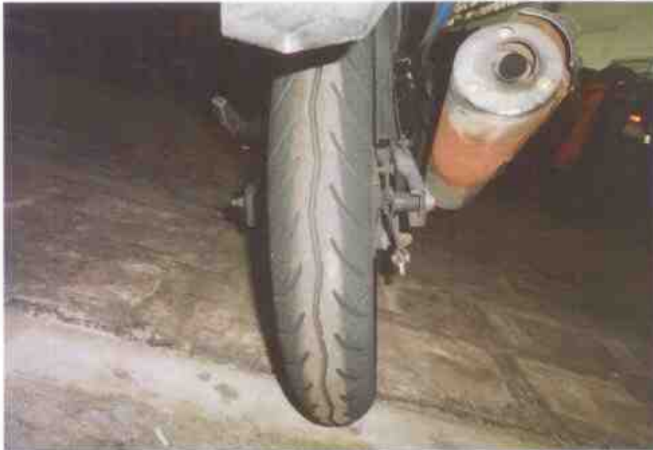
Photo 6 shows the rear tyre of the Motorcycle. The rear tyre was observed to be in serviceable condition with remaining tread depth of approximately 3mm. The tyre was also observed to be sufficiently inflated for vehicular operation.
