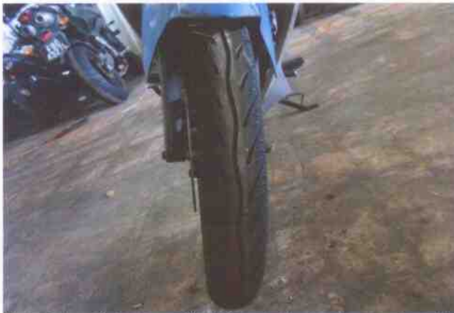
Photo 7 shows the front tyre of the Motorcycle. The front tyre was observed to be in serviceable condition with remaining tread depth of approximately 4mm. The tyre was also observed to be sufficiently inflated for vehicular operation.
