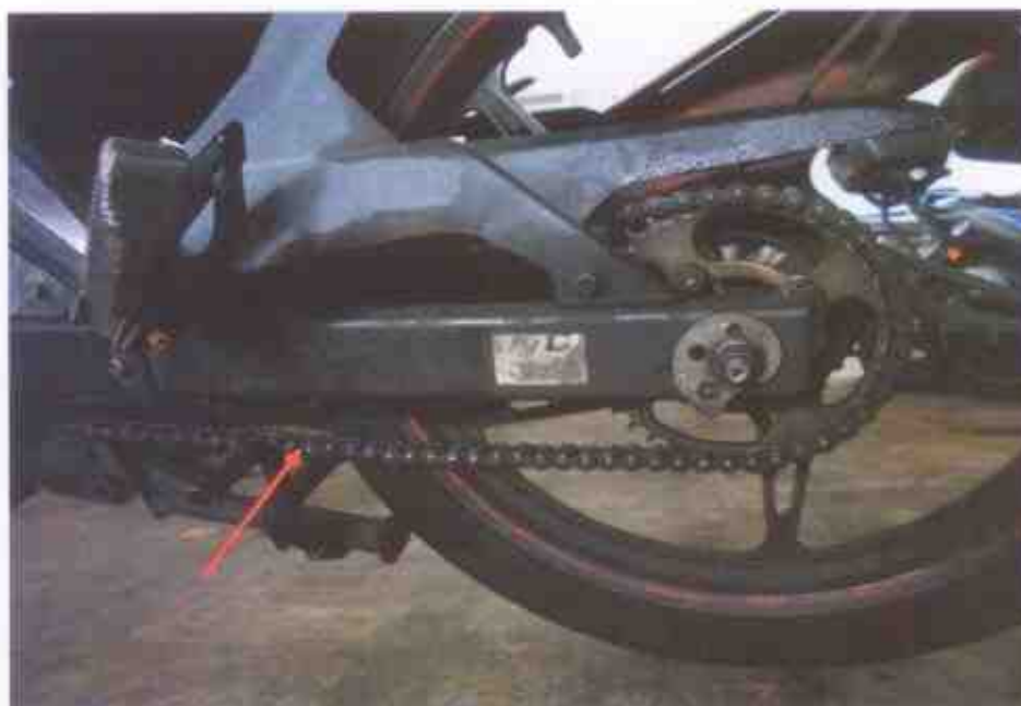
Photo 10 shows the general view of the gear train (arrowed) of the Motorcycle, which was observed to be intact with no misalignment. It was also adequately lubricated for operating purposes.
