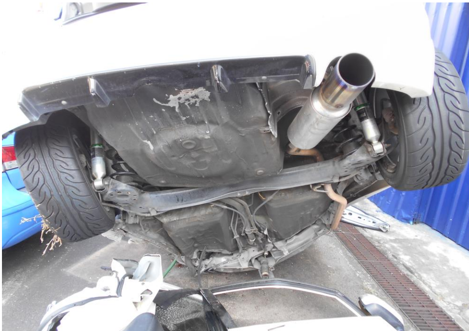
Photo 13 shows a general view of the rear undercarriage portion of the Motor Car at the time of our inspection. The body structure was observed to be distorted and buckled as a result of the accident.
