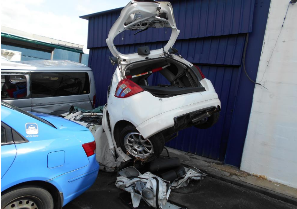
Photo 12 shows a general view of the rear left portion of the Motor Car at the time of our inspection. The rear portion was observed to have sustained with major impact by the accident that caused the rear portion body structure to be distorted.
