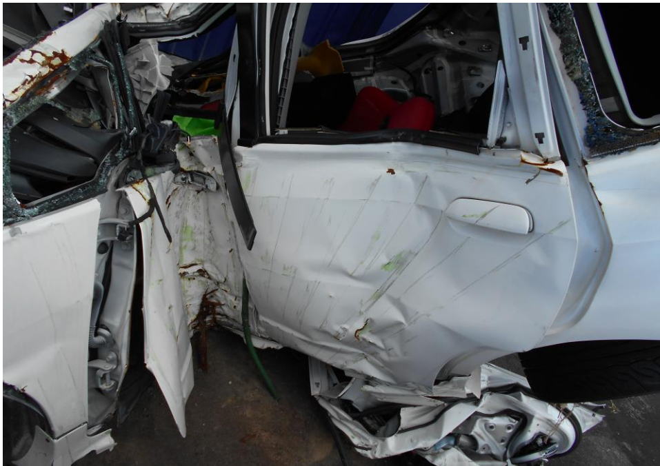
Photo 5 shows a closer view of the damage at the frontal left portion of the Motor Car. The impact force was significant, causing the various parts and components inside the engine compartment to be pushed inwards from left, towards the right of the Motor Car.
