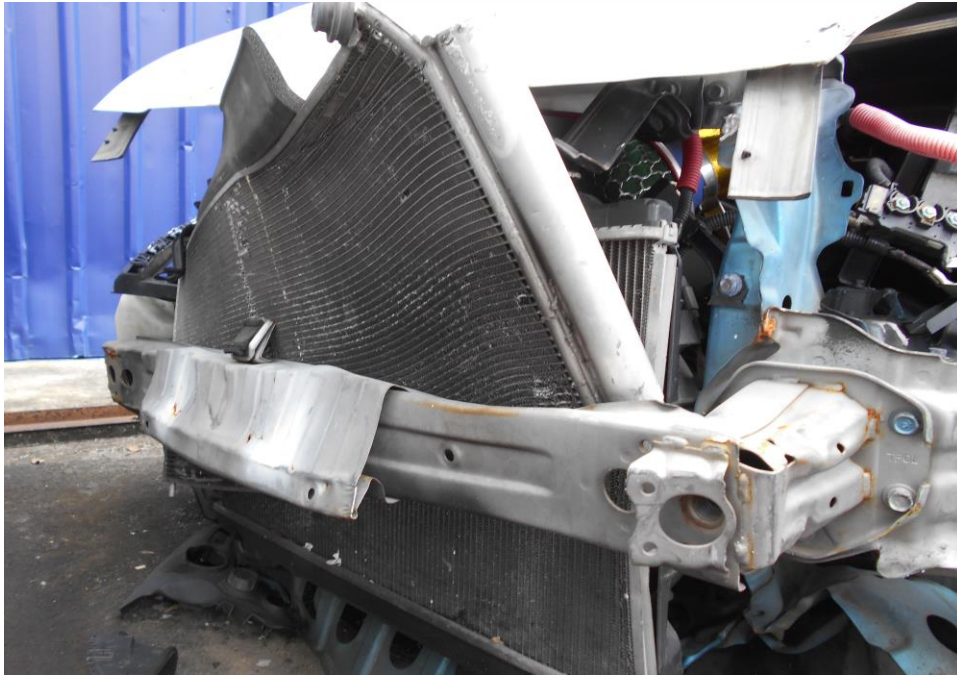
Photo 4 shows a closer view of the damage at the frontal portion of the Motor Car's engine. The impact force was significant, causing the various parts and components inside the engine compartment to be damaged.
