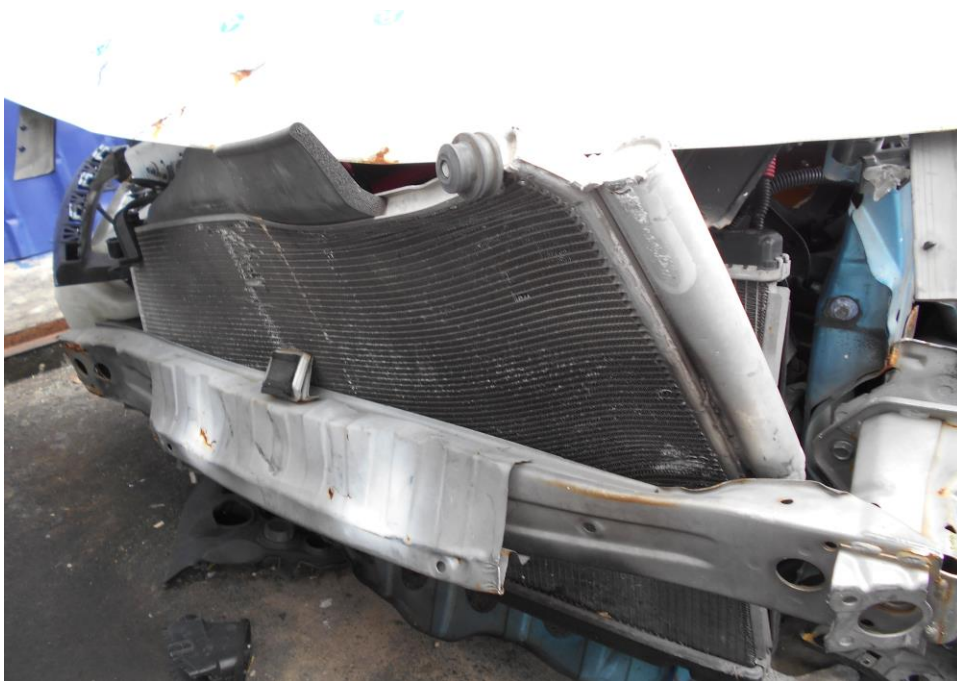
Photo 20 shows the close up view of the radiator's tank that was observed to be damaged likely due to the accident impact.
