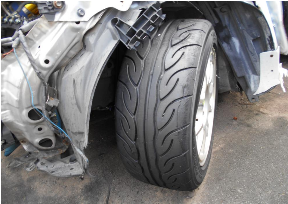
Photo 16 shows the condition of the front left tyre of the Motor Car, which was observed to be in serviceable condition. The 4 tyres were also observed to be sufficiently inflated for vehicular operation.
