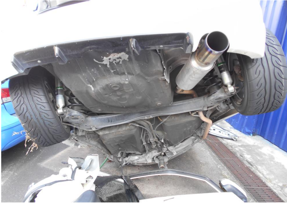
Photo 26 shows the undercarriage components of the Motor Car. It was observe to sustain an extensive damage inclusively affects the body structure of the Motor Car due to the accident.
