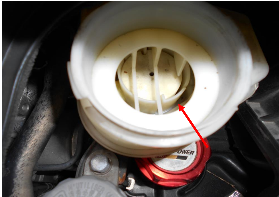
Photo 21 shows the close up view of the empty brake fluid reservoir due to the accident impact.
