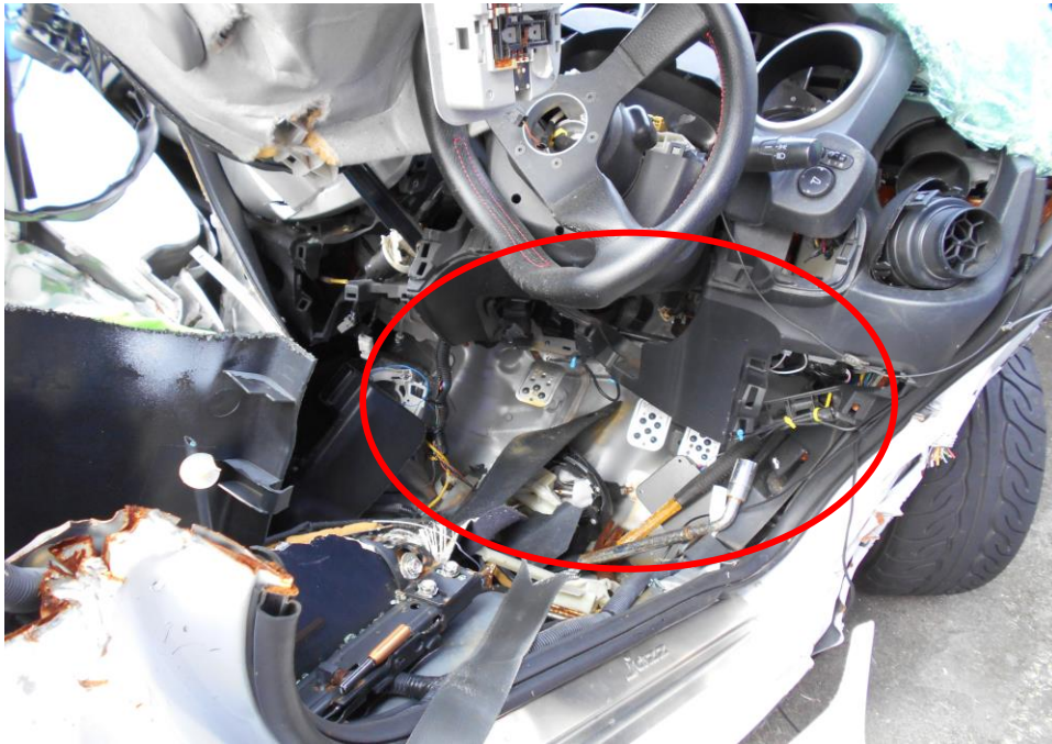
Photo 27 shows the damaged brake pedal of the Motor Car. It was observe to sustained extensive damages at the time of our inspection of the Motor Car due to the accident.
