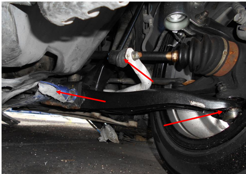
Photo 23 shows a close up view on the front right drive shaft of the Motor Car. We were not able to conduct any tests on the steering system of the Motor Car due to the damage to these components.
