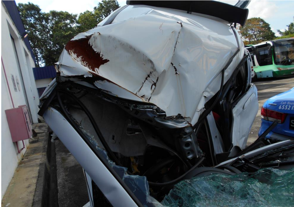
Photo 8 shows a semi-close up view of the damaged roof top of the Motor Car. The impact force was significant, causing the roof portion to be buckled as a result of the accident.
