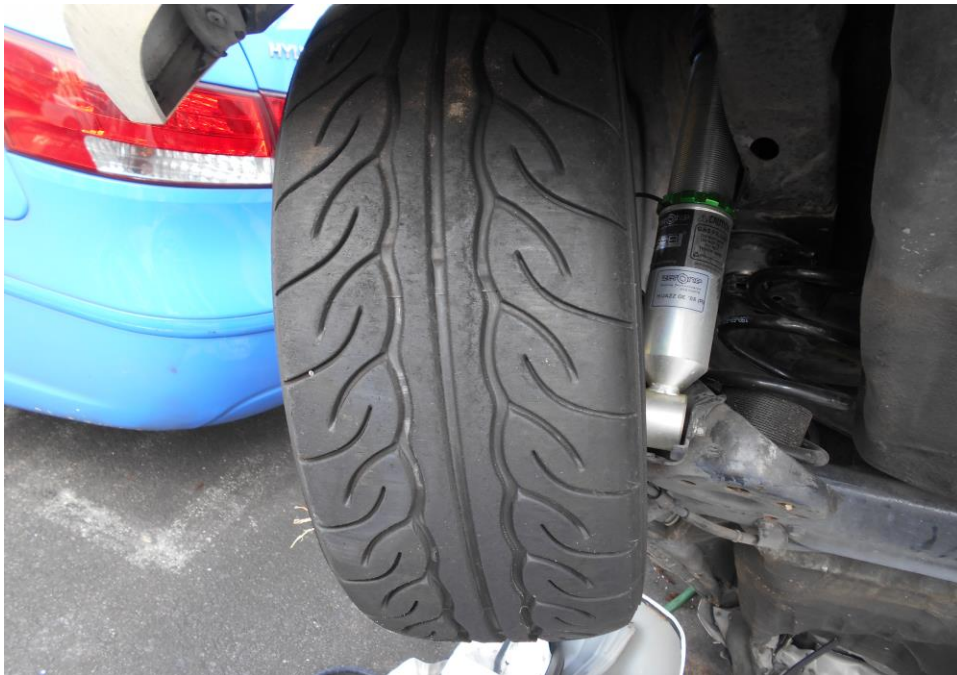
Photo 17 shows the condition of the rear left tyre of the Motor Car, which was observed to be in serviceable condition. The 4 tyres were also observed to be sufficiently inflated for vehicular operation.
