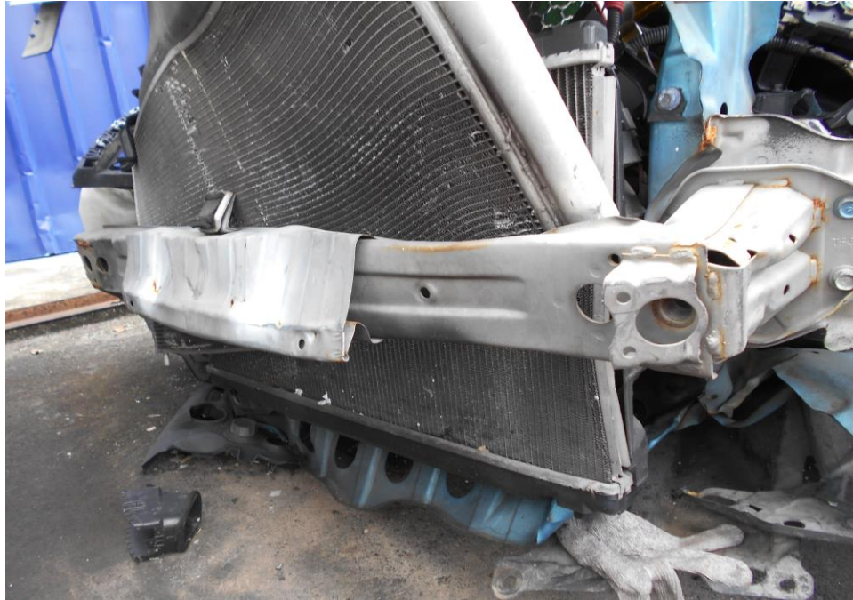
Photo 6 shows a closer view of the damage at the frontal left portion of the Motor Car. The impact force was significant, causing the various parts and components inside the engine compartment to be damaged as a result of the accident.
