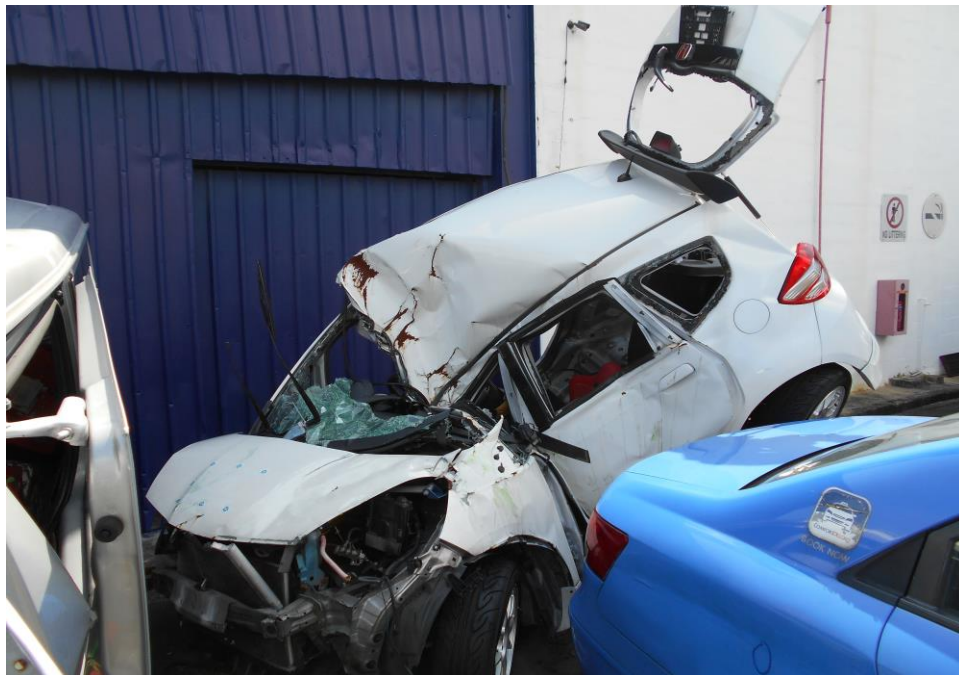
Photo 3 shows a general view of the front left portion of the Motor Car at the time of our inspection. The Motor Car was observed to have sustained with extensive impact damage at its frontal, left, right, top and rear portion.
