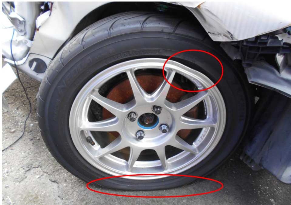
Photo 15 shows the condition of the front right portion of the Motor Car, which was observed to be deflated due to the damages on the wheel rim as a result of the accident's impact.
