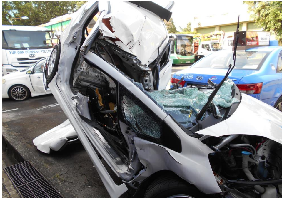
Photo 2 shows a general view of the front right portion of the Motor Car at the time of our inspection. The Motor Car was observed to have sustained extensive impact damage at its frontal, left, right, top and rear portion.
