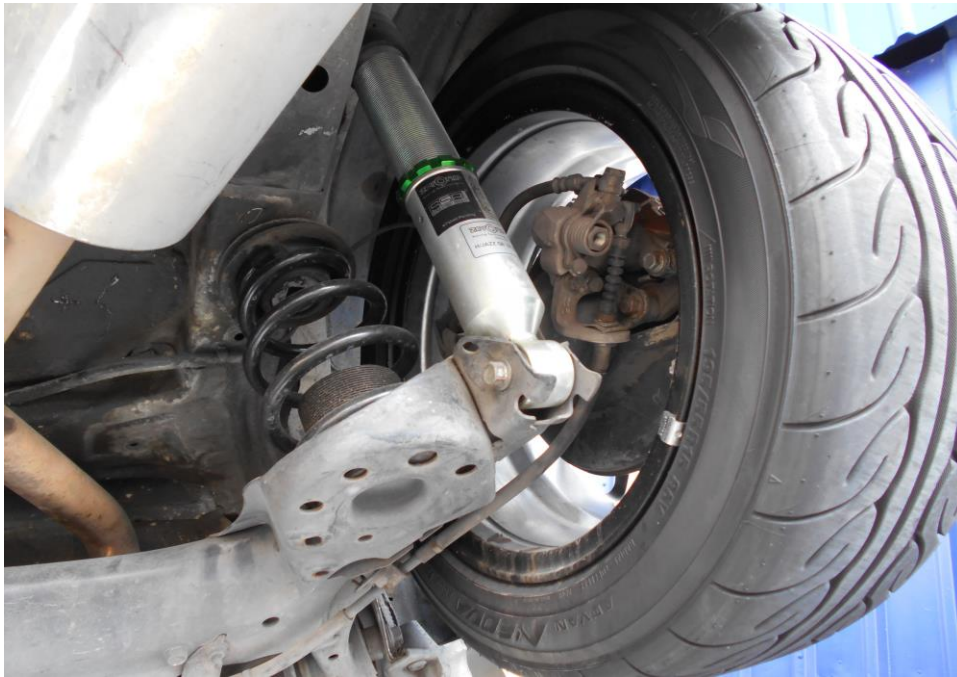
Photo 25 shows the braking & steering components at the rear right wheel of the Motor Car. We did not observe any leakage of brake fluid at the time of our inspection of the Motor Car.
