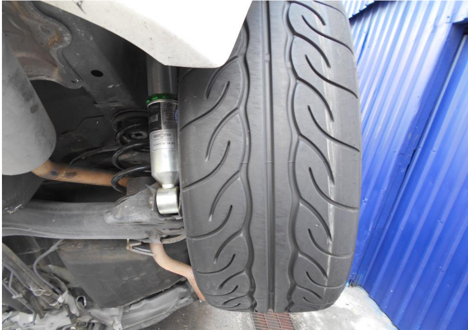
Photo 18 shows the condition of the rear right tyre of the Motor Car, which was observed to be in serviceable condition. The 4 tyres were also observed to be sufficiently inflated for vehicular operation.
