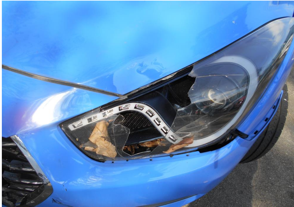
Photo 7 shows a semi close up view of the front left headlamp of the Motor Taxi at the time of our inspection. It had sustained damages likely due to the accident.
