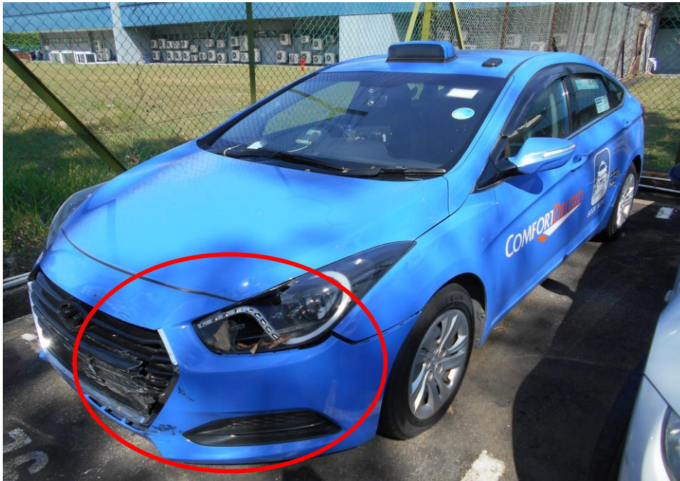
Photo 3 shows a general view of the front left body of the Motor Taxi at the time of our inspection. The Motor Taxi was observed to have sustained a relatively minor impact damages that was confined to its frontal left portion.
