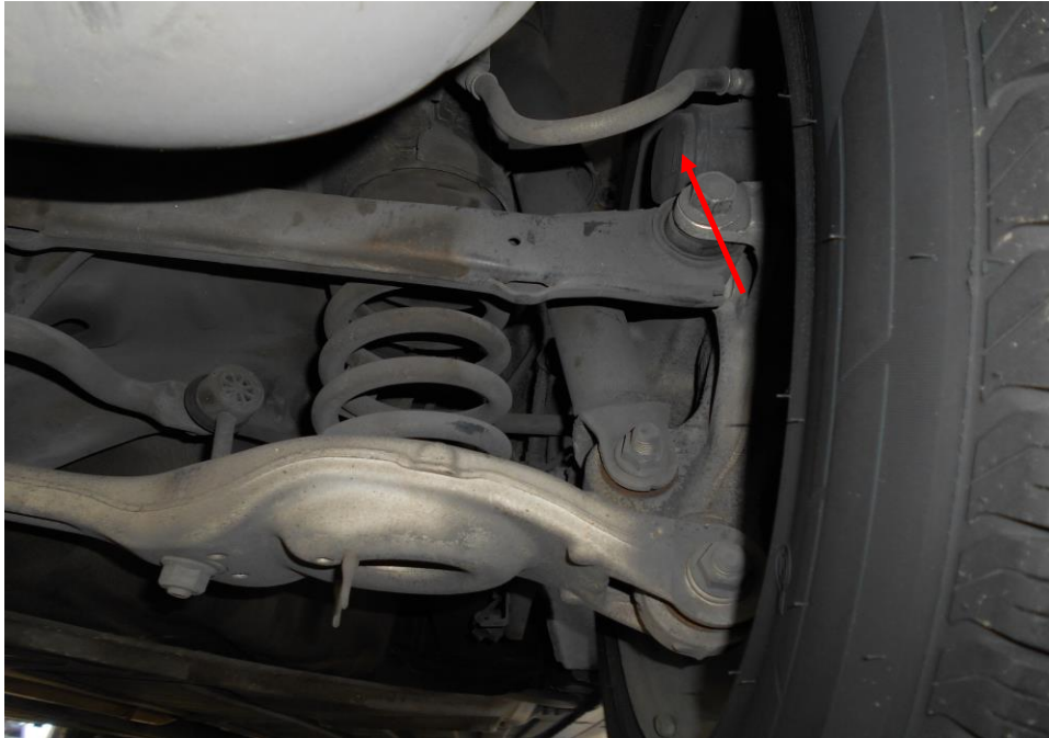
Photo 19 shows the brake hose (arrowed) at the rear right wheel of the Motor Taxi. We did not observe any leakage of brake fluid at the time of our inspection of the Motor Taxi. Our visual inspection of the various mechanical components of the Motor Taxi's braking system revealed all to be intact without visible damage.
