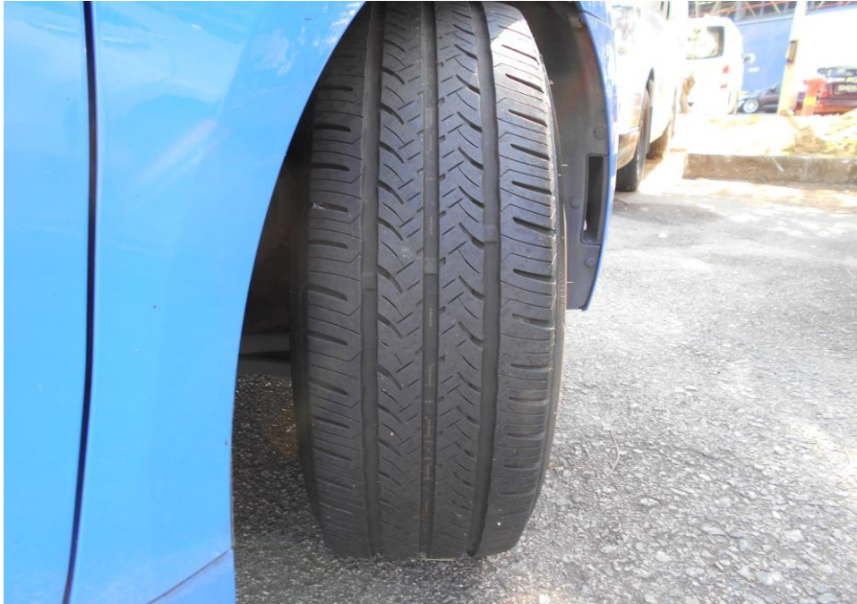
Photo 9 shows the condition of the front right tyre of the Motor Taxi, which was observed to be in serviceable condition with remaining tread depth of approximately 7mm. There was no tear, cut or burst mark(s) on the outer and the inner sidewalls.
