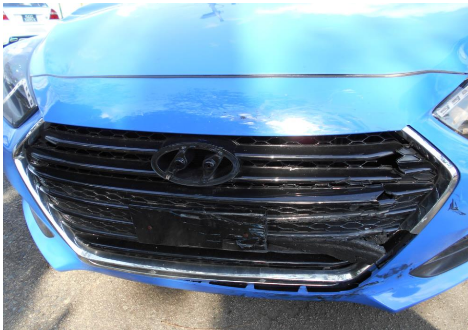
Photo 8 shows a close up view of the front portion of the Motor Taxi. Missing licence plate & damaged bumper was observed at the time of our inspection.
