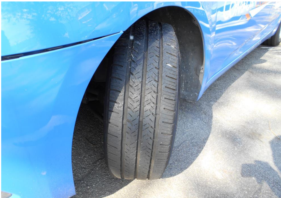
Photo 10 shows the condition of the front left tyre of the Motor Taxi, which was observed to be in serviceable condition with remaining tread depth of approximately 7mm. The tyre, which was wrapped around alloy wheel rim, was also observed to be sufficiently inflated for vehicular operation.
