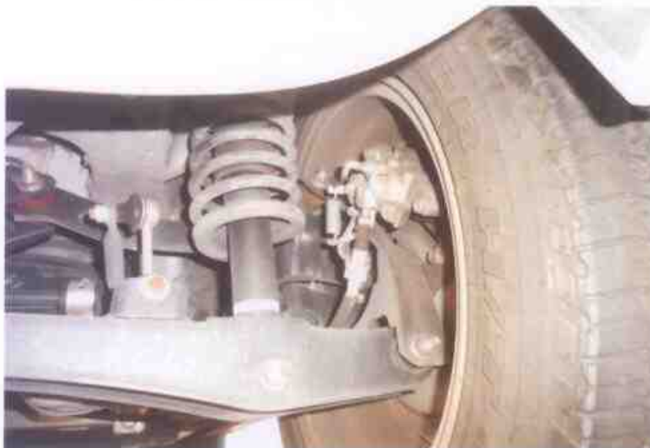
Photo 21 shows the various undercarriage components at the rear right wheel of the Motor Car. We did not observe any leakage of brake fluid at the time of our inspection of the Motor Car. Our visual inspection of the various mechanical components of the Motor Car's braking system revealed all to be intact and without visible damage, indicating that the braking system was likely to be in serviceable condition at the material time of accident.
