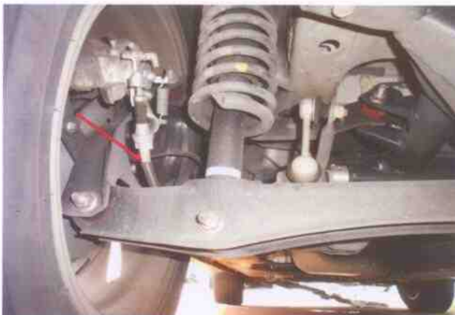
Photo 18 shows the brake hose (arrowed) at the rear left wheel of the Motor Car. We did not observe any leakage of brake fluid at the time of our inspection of the Motor Car. Our visual inspection of the various mechanical components of the Motor Car's braking system revealed all to be intact and without visible damage.
