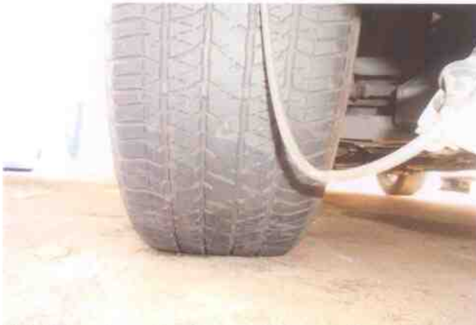
Photo 11 shows the condition of the front right tyre of the Motor Car, which was observed to be in serviceable condition with remaining tread depth of approximately 6mm.
