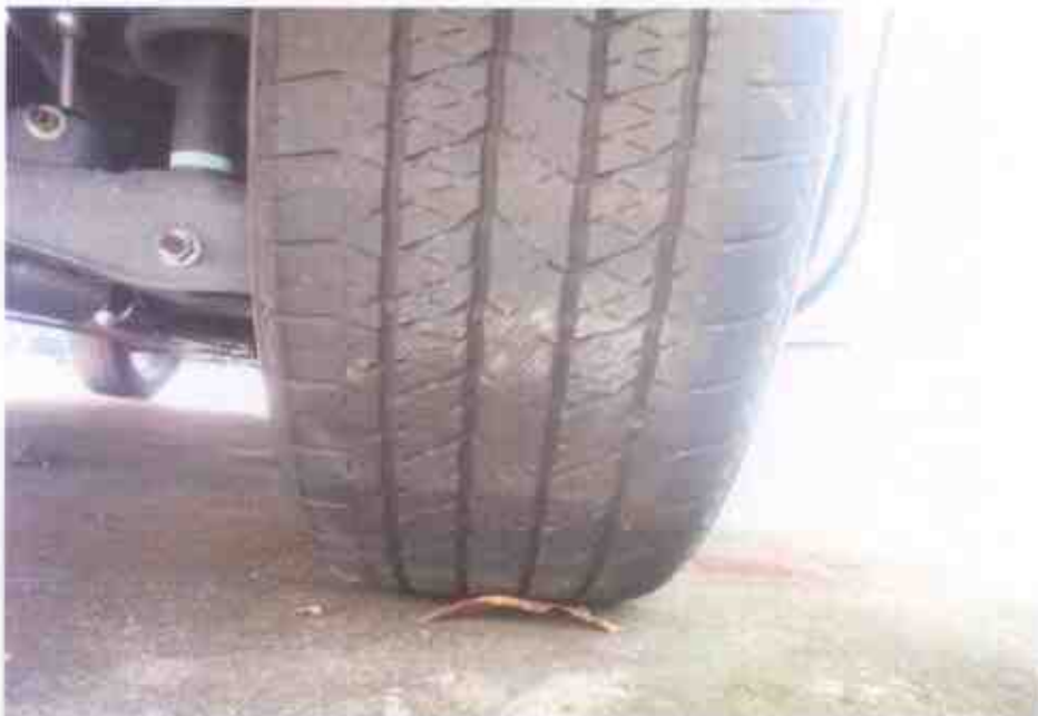
Photo 13 shows the condition of the rear right tyre of the Motor Car, which was observed to be in serviceable condition with remaining tread depth of approximately 5mm. There was also no tear, cut or burst mark(s) on the outer and the inner sidewalls as well as across the tread of the 4 tyres.
