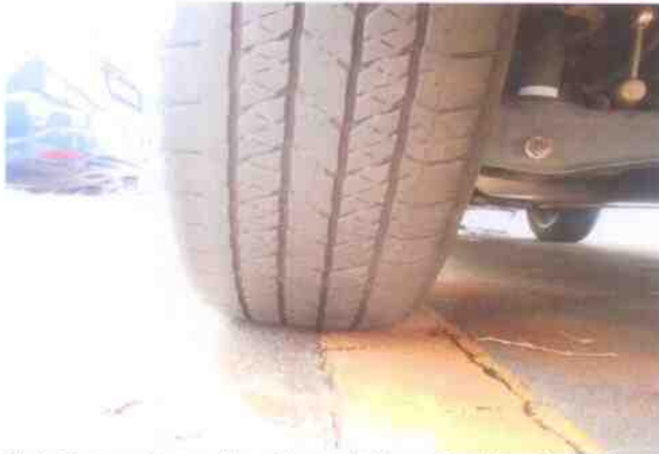
Photo 12 shows the condition of the rear left tyre of the Motor Car, which was observed to be in serviceable condition with remaining tread depth of approximately 5mm. The tyre, which was wrapped around alloy wheel rim, was also observed to be sufficiently inflated for vehicular operation.
