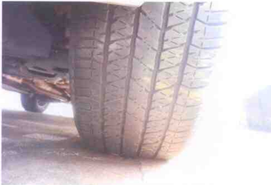
Photo 10 shows the condition of the front left tyre of the Motor Car, which was observed to be in serviceable condition with remaining tread depth of approximately 6mm.
