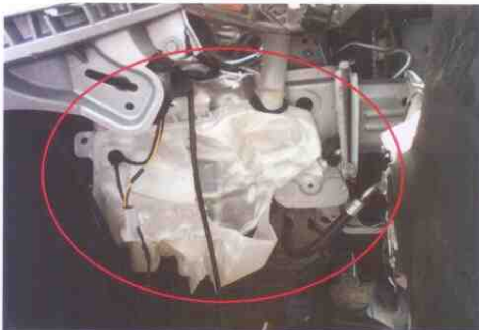
Photo 7 shows a close up view of the crushed wiper fluid reservoir of the Motor Car at the time of our inspection. It was observed to be damaged as a result of the accident.
