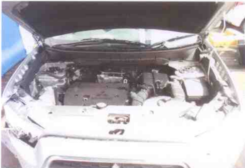
Photo 14 shows a general view of the Motor Car's engine compartment. The various parts and components inside the engine compartment were unaffected by the accident. There was also no sign(s) or indication(s) of fluid leakage and/or fluid stain within the engine compartment.
