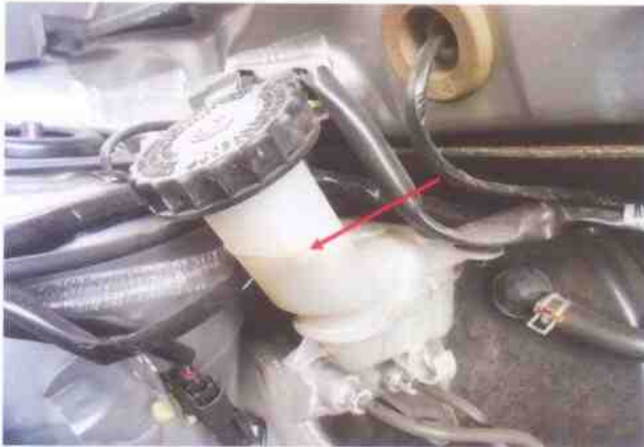
Photo 15 shows the brake fluid reservoir of the Motor Car at the time of our inspection. The brake fluid was observed to be of sufficient level (arrowed) and without any visible contamination.
