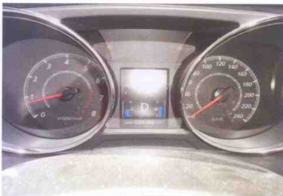
Photo 22 shows no warning lights illuminated on the instrument panel of the Motor Car after the engine was cranked. This would suggest that there was no abnormality to the various electronic operating systems of the Motor Car, like the ABS and SRS.
