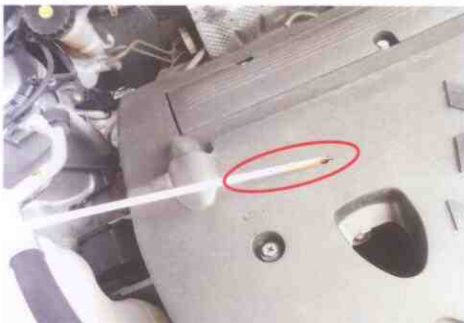
Photo 17 shows the engine oil dip stick of the Motor Car at the time of our inspection. The engine oil was observed to be of sufficient level and without any visible contamination.
