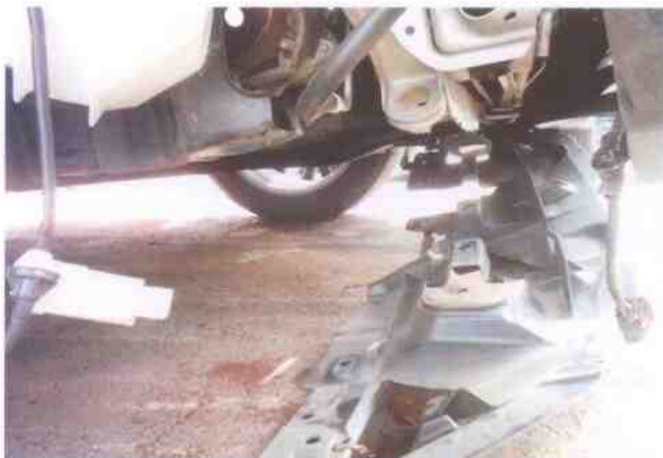
Photo 9 shows a close up view of the front undercarriage cover of the Motor Car at the time of our inspection. It was observed to be dislodged from the original installation likely due to the accident.
