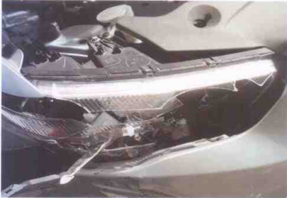
Photo 5 shows a close up view of the headlamp of the Motor Car at the time of our inspection. It was observed to have sustained with damages consistent to the accident's case fact.
