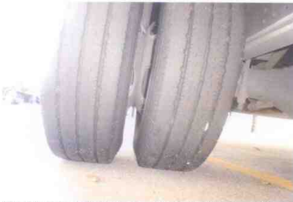
Photo 9 shows the condition of the rear right tyres of the Motor Lorry, which were observed to be in serviceable condition with remaining tread depth of approximately 7mm.
