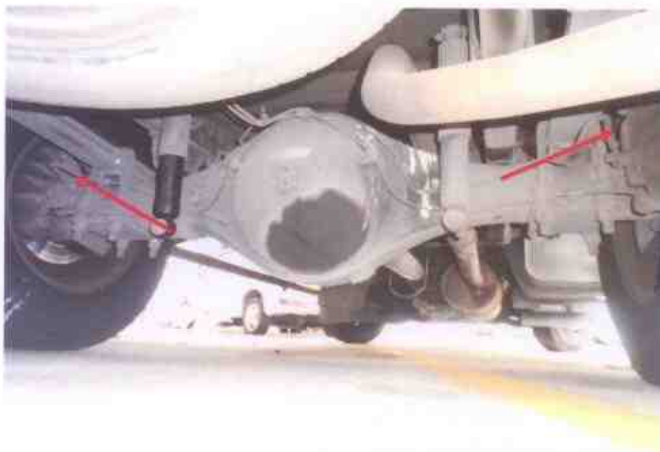
Photo 16 shows the various undercarriage components at the rear wheels of the Motor Lorry. There was no sign(s) of brake fluid leakage along the brake hoses and brake pipes.
