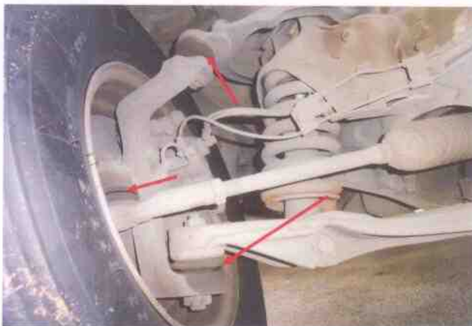
Photo 15 shows the various undercarriage components at the front right wheel of the Motor Lorry, in particular the steering tie rod end (arrowed). The various undercarriage components of the Motor Lorry were all found to be intact without any visible damage. There was also no sign of fluid stain(s) observed on the various undercarriage components.
