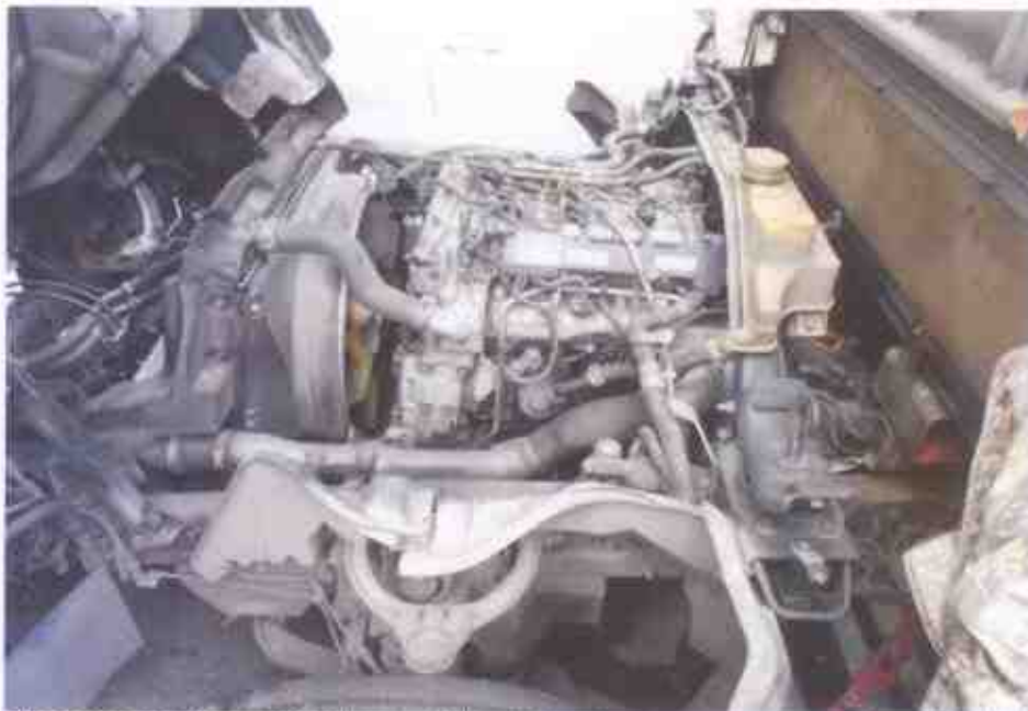
Photo 10 shows a general view of the Motor Lorry's engine compartment, which was accessed by lifting the front cabin of the Motor Lorry. The various parts and components inside the engine compartment were unaffected by the accident. There was also no sign(s) or indication(s) of fresh fluid leakage and/or fluid stain within the engine.
