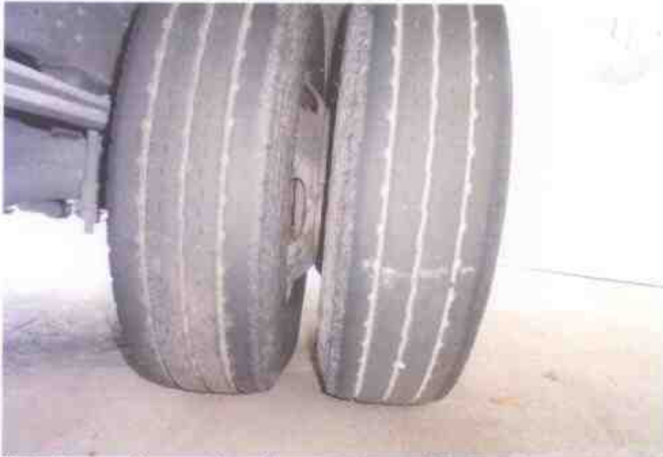
Photo 8 shows the condition of the rear left tyres of the Motor Lorry, which was observed to be in serviceable condition with remaining tread depth of approximately 4mm. The tyres were also observed to be sufficiently inflated for vehicular operation.
