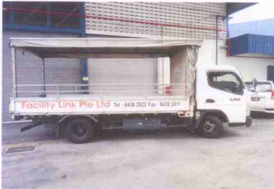
Photo 18 shows the operational test on the Motor Lorry. It was observed to be in serviceable condition. Operational test such as moving forward, turn left & right and also braking test on the Motor Lorry was conducted successfully.
