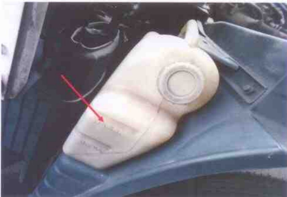
Photo 12 shows the engine coolant reservoir of the Motor Lorry at the time of our inspection. The engine coolant was observed to be of sufficient level and without any visible contamination (arrowed).
