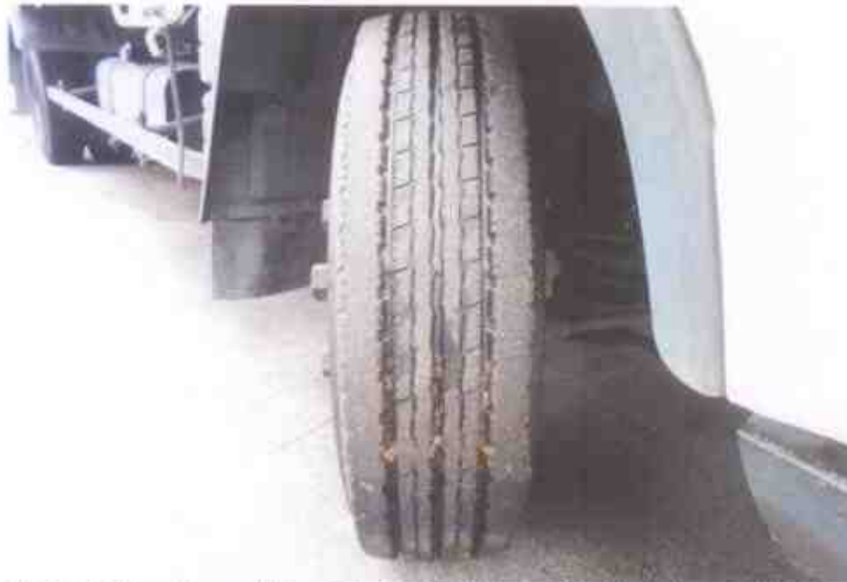
Photo 7 shows the condition of the front right tyre of the Motor Lorry, which was observed to be in serviceable condition with remaining tread depth of approximately 7mm. The tyre was also observed to be sufficiently inflated for vehicular operation.
