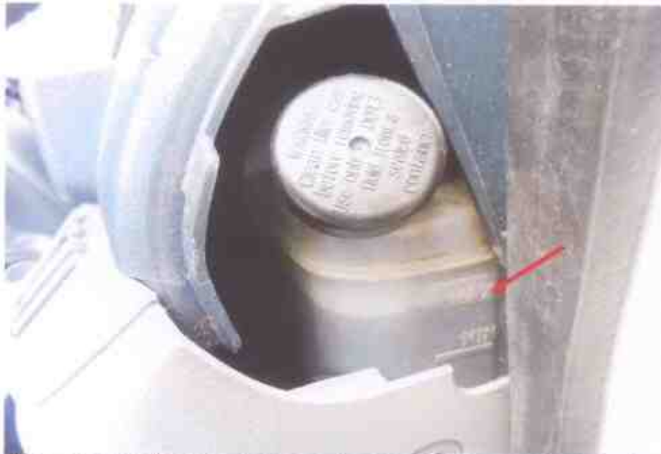
Photo 11 shows the brake fluid reservoir of the Motor Lorry at the time of our inspection. The brake fluid was observed to be of sufficient level and without any visible contamination (arrowed).
