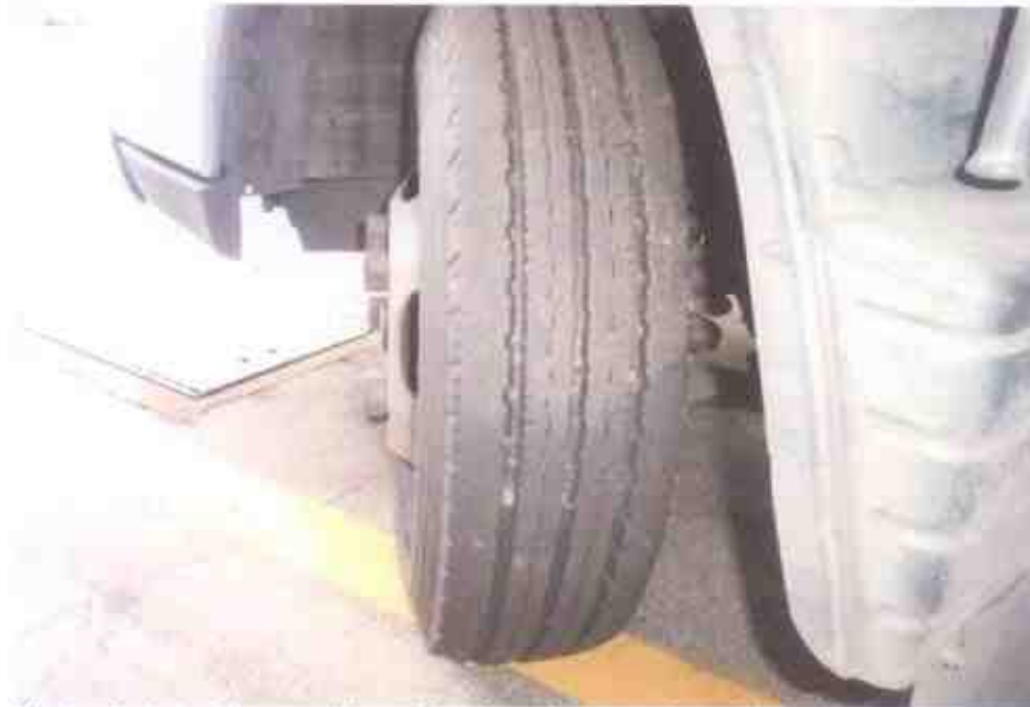
Photo 6 shows the condition of the front left tyre of the Motor Lorry, which was observed to be in serviceable condition with remaining tread depth of approximately 8mm.
