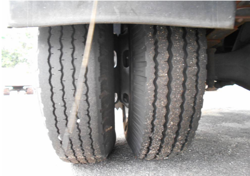
Photo 10 shows the condition of the rear right tyres of the Motor Lorry, which were observed to be in serviceable condition with remaining, tread depth of approximately 8mm.
