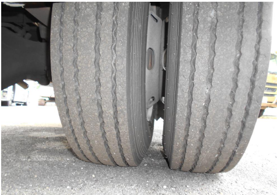
Photo 9 shows the condition of the rear left tyres of the Motor Lorry, which was observed to be in serviceable condition with remaining tread depth of approximately 7mm. The tyres were also observed to be sufficiently inflated for vehicular operation.
