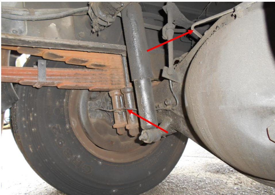
Photo 18 shows the various undercarriage components at the rear left wheels of the Motor Lorry. There was no sign(s) of brake fluid leakage along the brake hoses and brake pipes.
