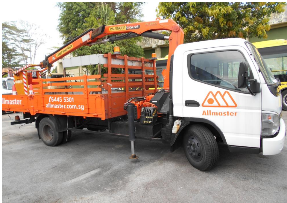
Photo 22 shows the operational test on the Motor Lorry. It was observed to be in serviceable condition. Operational test such as moving forward, turn left & right and also braking test on the Motor Lorry was conducted successfully.
