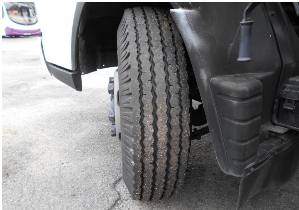
Photo 7 shows the condition of the front left tyre of the Motor Lorry, which was observed to be in serviceable condition with remaining tread depth of approximately 9mm.
