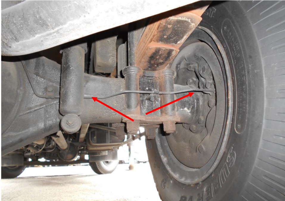
Photo 17 shows the various undercarriage components at the rear right wheels of the Motor Lorry. There was no sign(s) of brake fluid leakage along the brake hoses and brake pipes.
