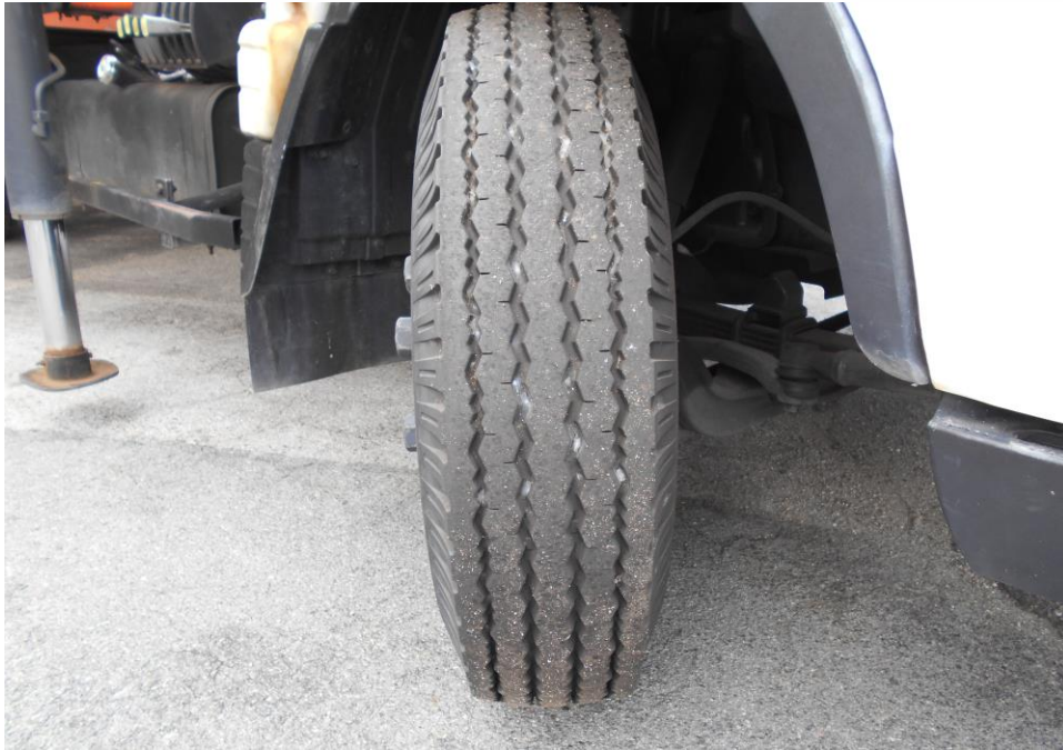
Photo 8 shows the condition of the front right tyre of the Motor Lorry, which was observed to be in serviceable condition with remaining tread depth of approximately 9mm. The tyre was also observed to be sufficiently inflated for vehicular operation.
