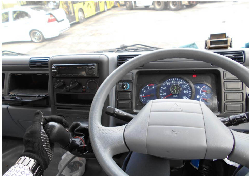
Photo 21 shows the operational test on the Motor Lorry. It was observed to be in serviceable condition. Operational test such as moving forward, turn left & right and also braking test on the Motor Lorry was conducted successfully.
