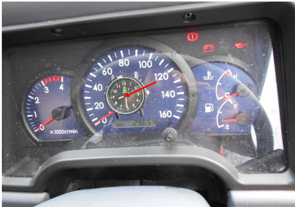
Photo 19 shows the warning lights for the various electronic operating systems of the Motor Car appearing on its instrument panel during the self-test when the engine was cranked.
