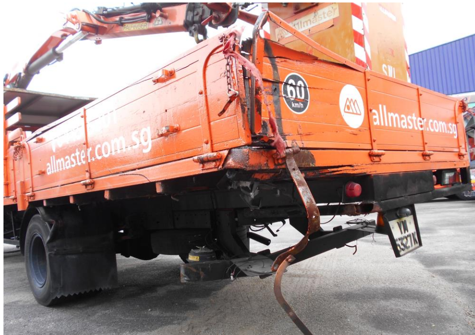
Photo 6 shows a general view of the Motor Lorry's rear body at the time of our inspection. It was observed to sustained damages at the rear left portion of Motor Lorry as a result of the accident.
