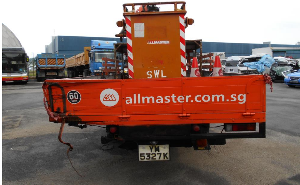
Photo 5 shows a general view of the Motor Lorry's rear body at the time of our inspection. It was observed to sustained damages at the rear left portion of Motor Lorry as a result of the accident.
