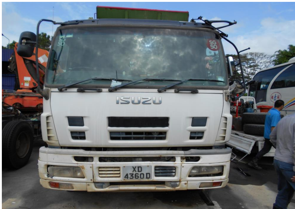
Photo 2 shows a general view of the front body of the Tipper Truck at the time of our inspection. The Tipper Truck was observed to sustain minor damages at its top left portion due to the accident impact.
