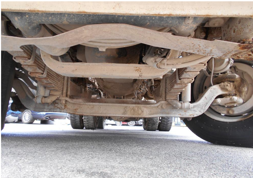
Photo 21 shows a general view of the undercarriage at the engine compartment area of the Tipper Truck. It was observed to be intact and unaffected by the collision. There was also no sign(s) or indication(s) of fluid leak and/or fluid stain found.
