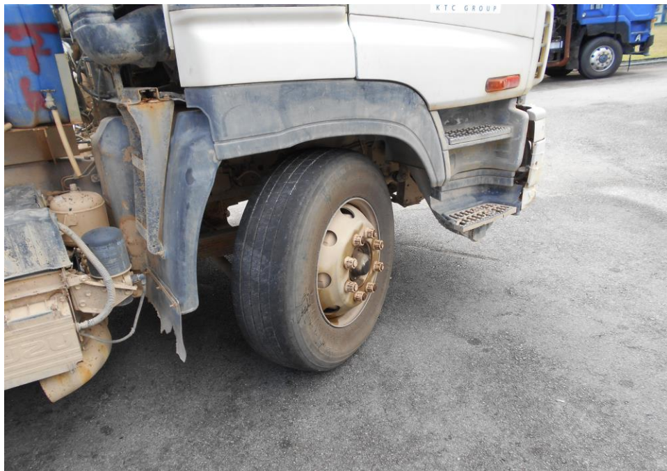
Photo 26 shows that we did not experience any abnormal free play and/or other resistance when turning the steering wheel left and right to full lock positions.
