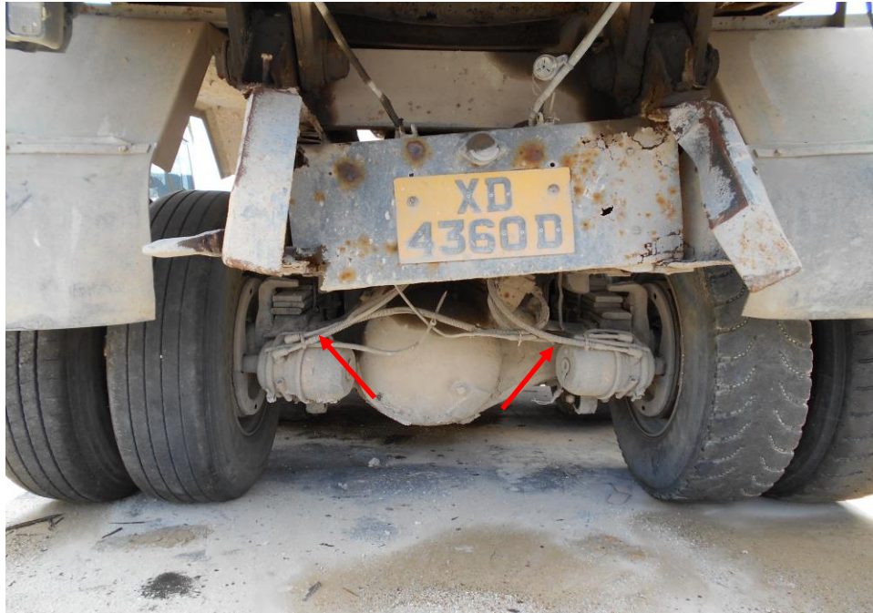
Photo 29 shows the brake hoses (arrowed) leading to the rear left wheel and rear right wheel of the Tipper Truck. At the time of our inspection, the various mechanical components of the air-assisted hydraulic braking system of the Tipper Truck were all found to be in good general condition and securely fitted.
