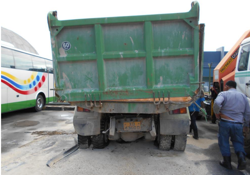
Photo 5 shows a general view of the rear body of the Tipper Truck at the time of our inspection. The Tipper Truck's rear container was observed to sustain misalignment due to the accident.
