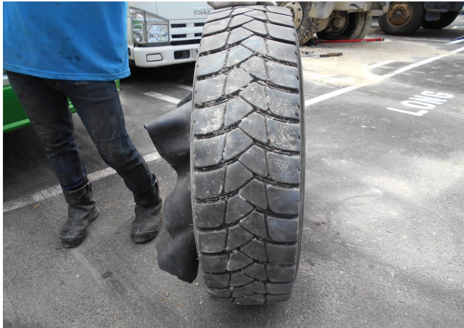
Photo 11 shows the condition of the rear left tyres of the Tipper Truck, which were observed to be in serviceable condition with remaining tread depth of approximately 8mm. The tyres were also observed to be sufficiently inflated for vehicular operation.
