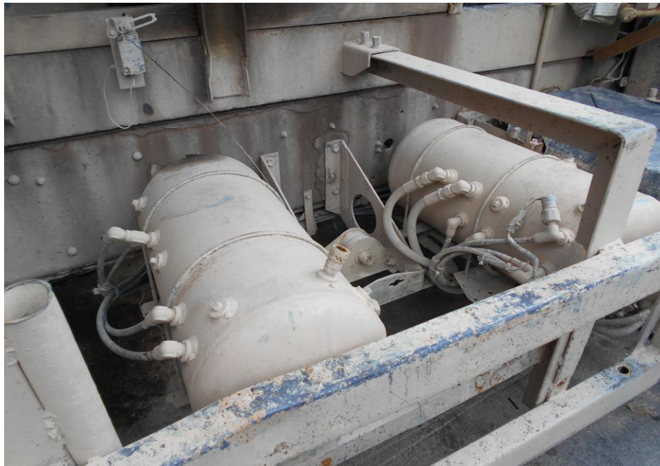
Photo 28 shows the air tanks, valves, pipes and hoses, which are some of the components for the air-assisted braking system of the Tipper Truck. These components were mainly located around the right centre body of the Tipper Truck, and were unaffected by the accident.
