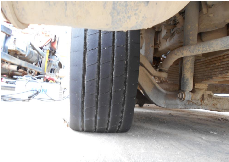
Photo 10 shows the condition of the front right tyre of the Tipper Truck, which was observed to be in serviceable condition with remaining tread depth of approximately 7mm.
