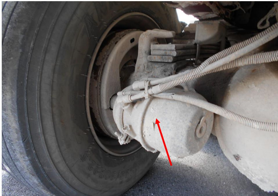
Photo 30 shows the brake air cylinder (arrowed) at the rear left rear wheel of the Tipper Truck. Such air cylinder, which is amongst the various components for the air-assisted hydraulic braking system, can be found attached to all the front wheels and all the rear wheels of the Tipper Truck. Upon our checks, we had found all the brake air cylinders to be undamaged and securely fitted to all the wheels of the Tipper Truck.
