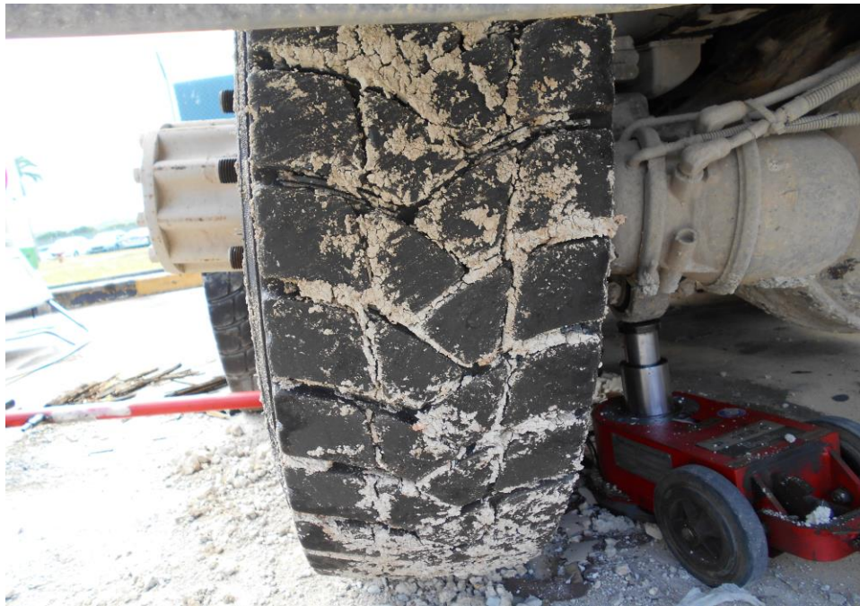
Photo 12 shows the condition of the rear left tyres of the Tipper Truck, which were observed to be in serviceable condition with remaining tread depth of approximately 8mm. The tyres were also observed to be sufficiently inflated for vehicular operation.
