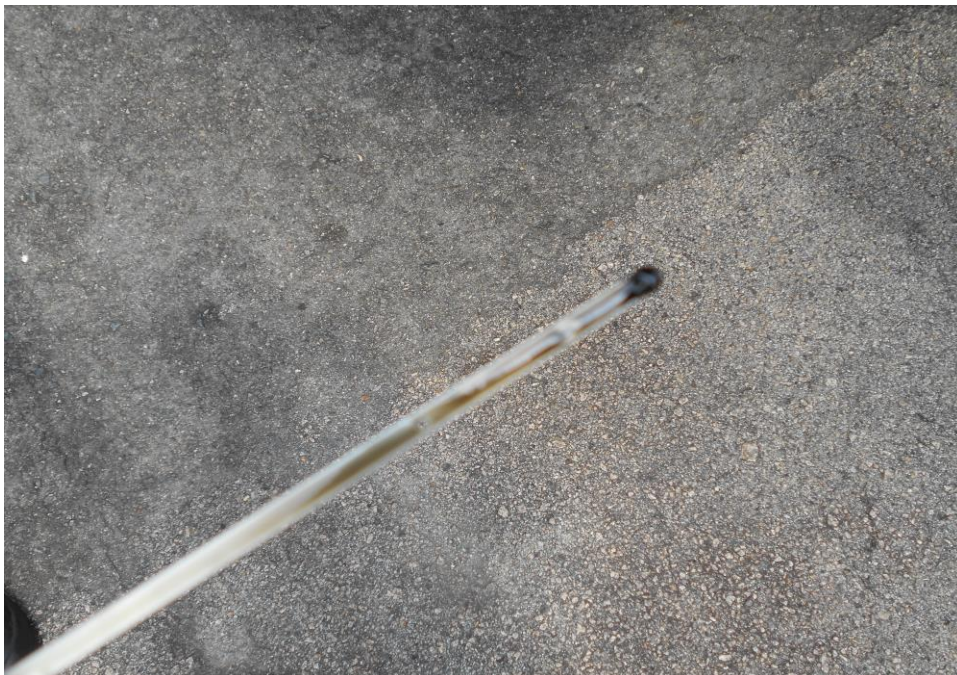
Photo 19 shows a close-up view of the dip stick which indicated the engine fluid was at a sufficient level for operational purposes.
