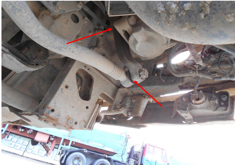
Photo 22 shows some of the mechanical components (arrowed) of the Tipper Truck's steering system. Our visual checks on the various mechanical components of the steering system revealed all to be intact and in good condition. The steering system of the Tipper Truck is hence likely to be in serviceable condition at the time of accident.
