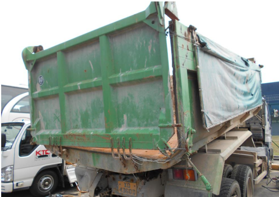
Photo 6 shows a general view of the rear right body of the Tipper Truck at the time of our inspection. The Tipper Truck was observed to have no signs of fresh damages on its front portion except for rear container in recline condition and misaligned due to the accident's impact.
