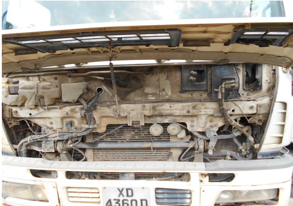
Photo 16 shows a general view of the engine compartment area from the front bonnet of the Tipper Truck. It was observed to be intact and unaffected by the collision. There was also no sign(s) or indication(s) of fluid leak and/or fluid stain found.
