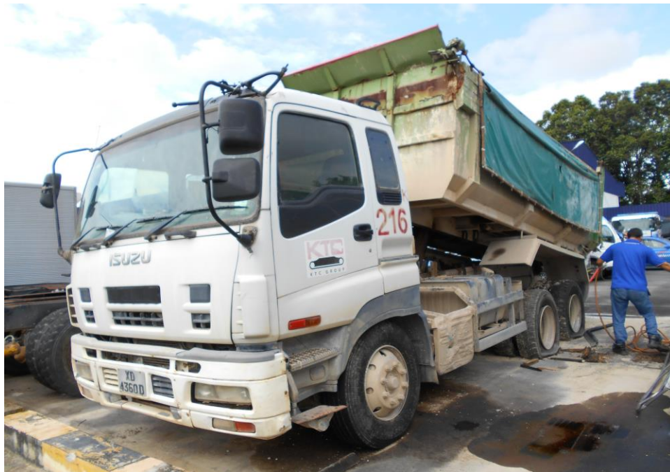
Photo 4 shows a general view of the front left body of the Tipper Truck at the time of our inspection. . The Tipper Truck was observed to have no signs of fresh damages on its front portion except for rear container in recline condition due to the accident's impact.
