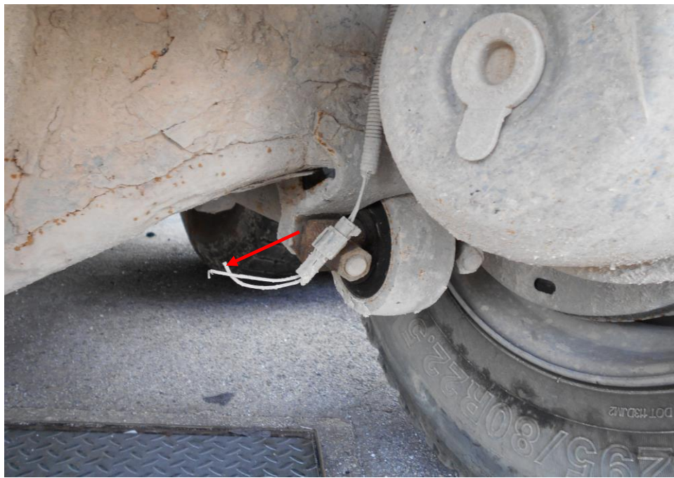
Photo 35 shows the cut off ABS wires found dangling at the rear right wheel area of the Tipper Truck.
