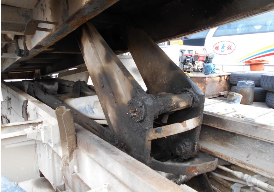
Photo 7 shows a semi close-up view of the damaged bracket for the rear container due to the accident's impact.
