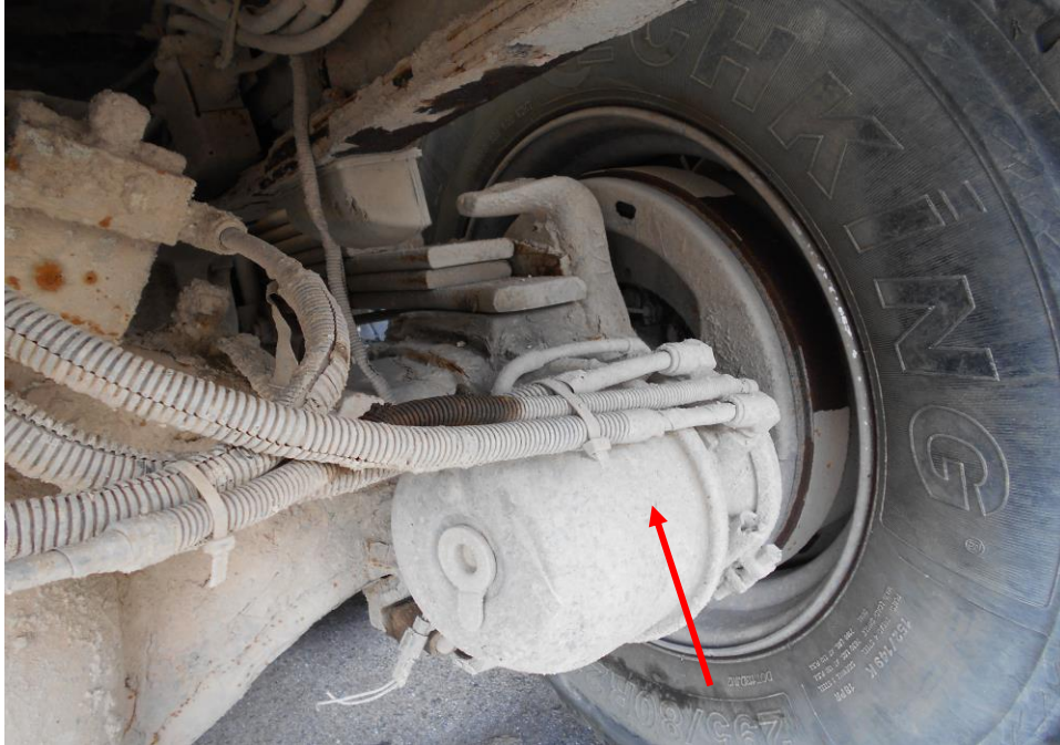
Photo 31 shows the brake air cylinder (arrowed) at the rear right rear wheel of the Tipper Truck. Such air cylinder, which is amongst the various components for the air-assisted hydraulic braking system, can be found attached to all the front wheels and all the rear wheels of the Tipper Truck. Upon our checks, we had found all the brake air cylinders to be undamaged and securely fitted to all the wheels of the Tipper Truck.
