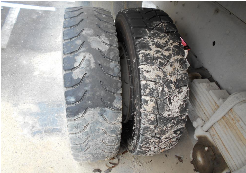
Photo 14 shows the condition of the rear right tyres of the Tipper Truck, which were observed to be in serviceable condition with remaining, tread depth of approximately 6mm. The tyres were also observed to be sufficiently inflated for vehicular operation with no tear, cut or burst mark(s) on the outer and the inner sidewalls.
