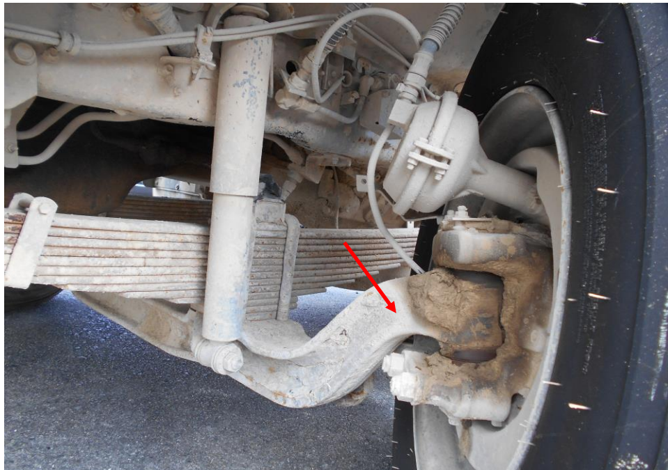
Photo 24 shows the undercarriage components at the front left wheel of the Tipper Truck. The various undercarriage components of the Tipper Truck were all observed to be intact and without any visible damage. This had included the steering rack (arrowed) of the Tipper Truck, which was observed to be securely attached to the front left wheel and front right wheel.
