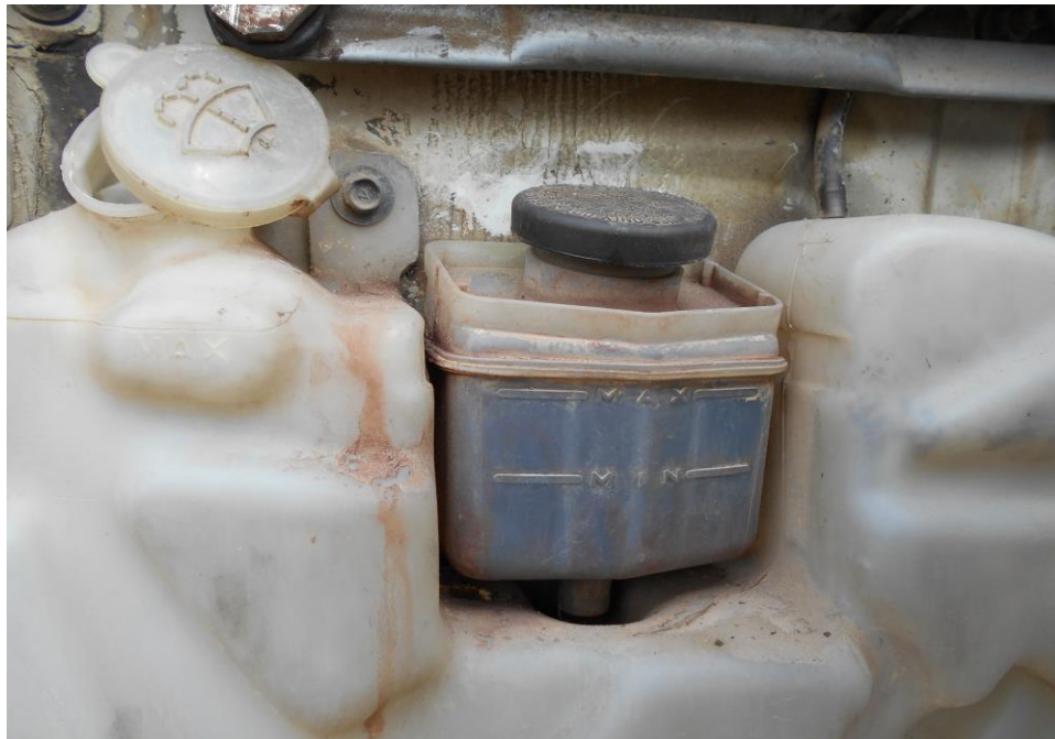
Photo 17 shows a close-up view of the clutch fluid. It was observed to be at sufficient level without any contamination.
