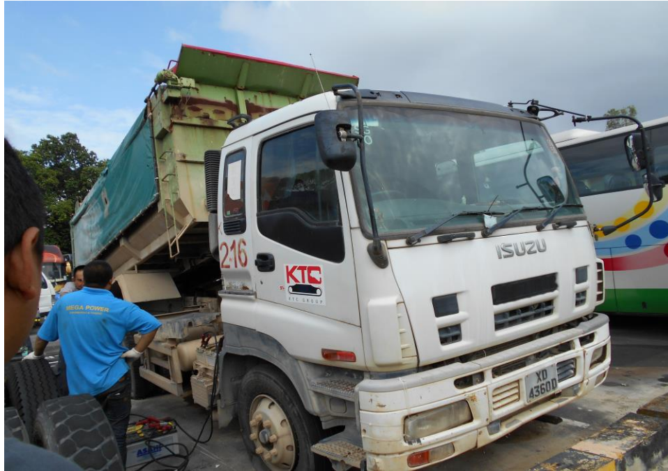
Photo 3 shows a general view of the front right body of the Tipper Truck at the time of our inspection. The Tipper Truck was observed to have no signs of fresh damages on its front portion except for rear container in recline condition due to the accident's impact.
