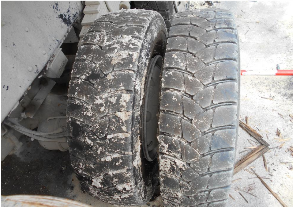
Photo 13 shows the condition of the rear left tyres (centre axle) of the Tipper Truck, which were observed to be in serviceable condition with remaining tread depth of approximately 7mm. The tyres were also observed to be sufficiently inflated for vehicular operation.
