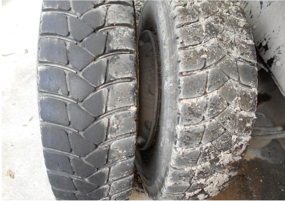
Photo 15 shows the condition of the rear right tyres (centre axle) of the Tipper Truck, which were observed to be in serviceable condition with remaining, tread depth of approximately 8mm. The tyres, which were wrapped around standard alloy wheel rims, were also observed to be sufficiently inflated for vehicular operation.
