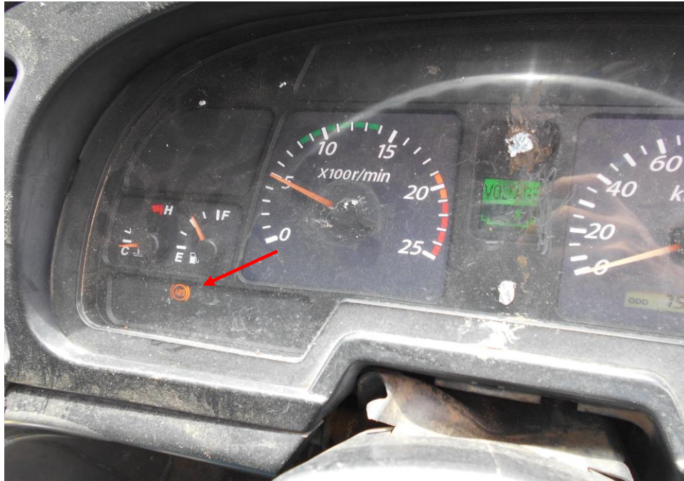
Photo 34 shows the warning indicator for Anti-Brake Lock System (ABS) was observed to be lighted up during cranking & after engine was in idling speed.
