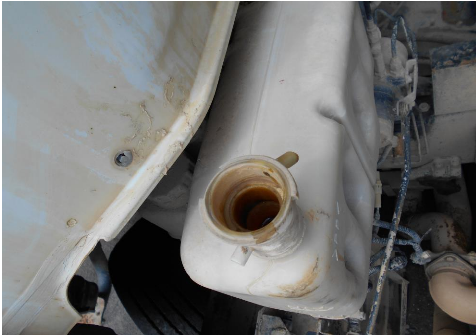
Photo 20 shows the engine coolant reservoir of the Tipper Truck at the time of our inspection. The engine coolant was observed to be of sufficient level and without any visible contamination for operational purposes.
