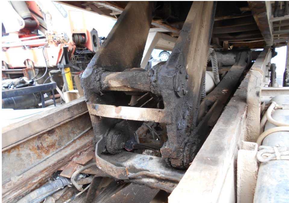
Photo 37 shows a close-up view of the damaged hydraulic system which immobilized the operational of the rear compartment.
