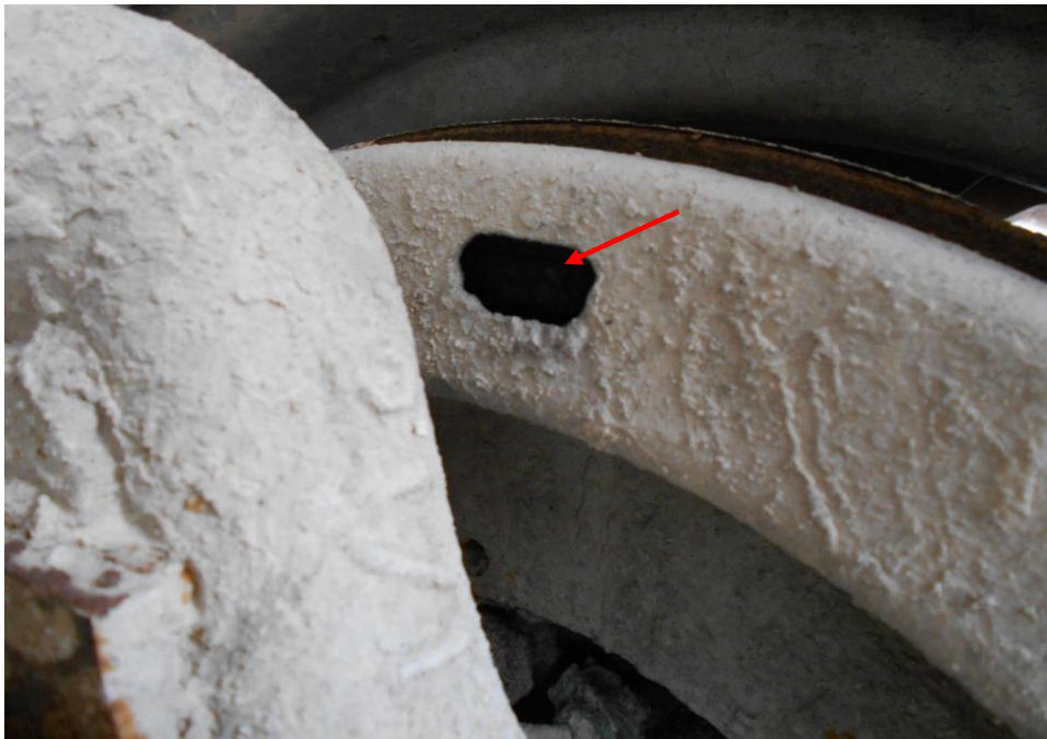
Photo 32 shows the brake shoes (brake pads) at the rear left wheel (rear axle) of the Tipper Truck. The brake shoes (brake pads) of the Tipper Truck were all found to be in serviceable condition with sufficient frictional material for operational purposes.
