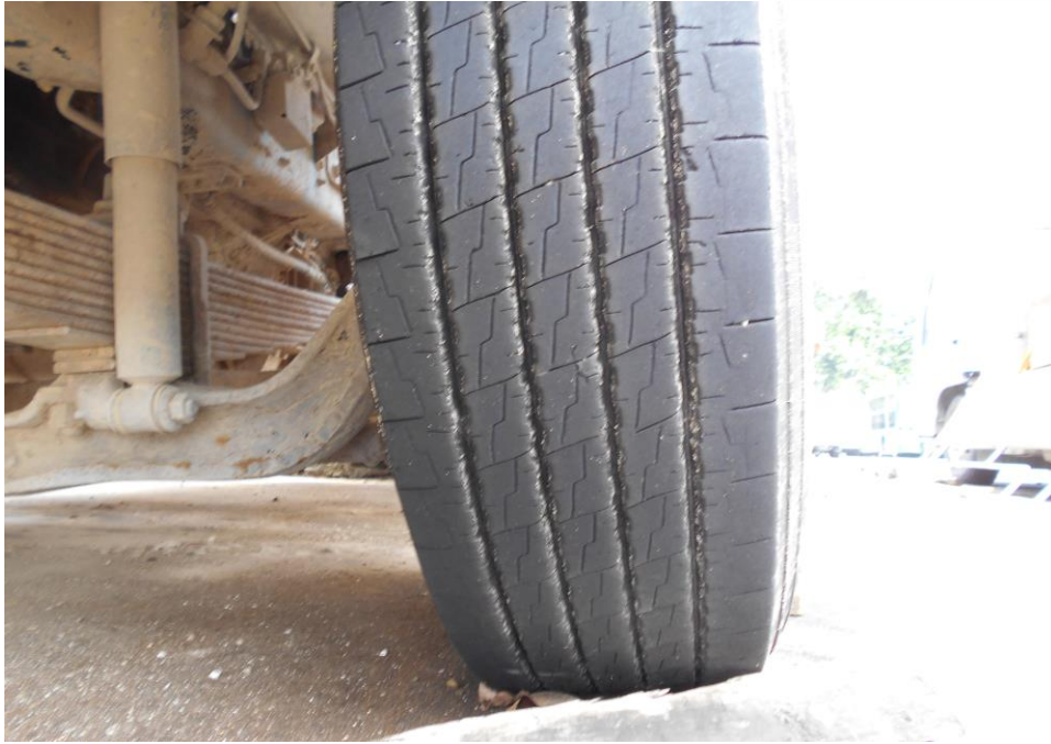
Photo 9 shows the condition of the front left tyre of the Tipper Truck, which was observed to be in serviceable condition with remaining tread depth of approximately 7mm.
