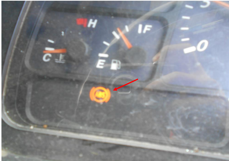
Photo 33 shows the warning indicator for Anti-Brake Lock System (ABS) was observed to be lighted up during cranking & after engine was in idling speed.
