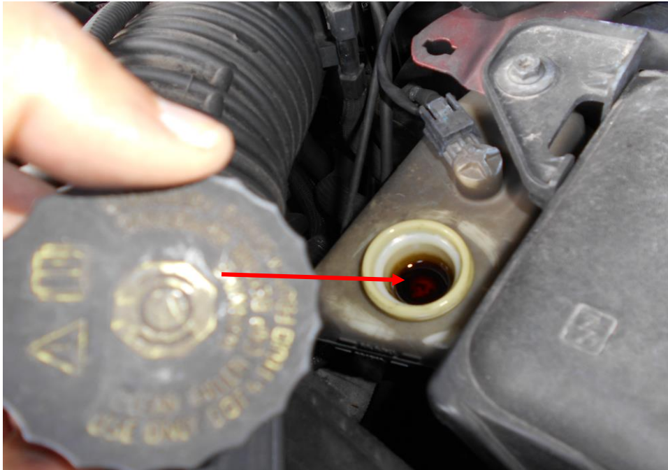
Photo 11 shows the brake fluid reservoir of the Motor Taxi at the time of our inspection. The brake fluid was observed to be of sufficient level (arrowed) and without any visible contamination.
