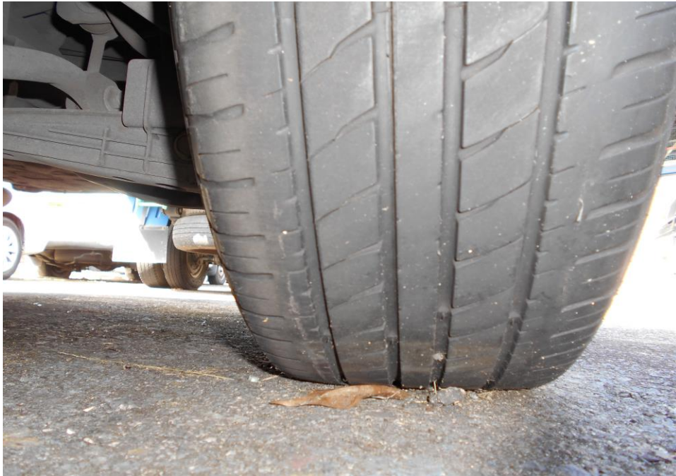
Photo 8 shows the condition of the rear left tyre of the Motor Taxi, which was observed to be in serviceable condition with remaining tread depth of approximately 5mm.
