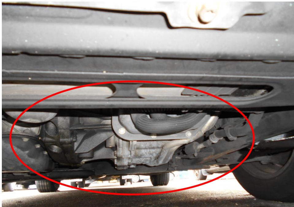
Photo 14 shows the engine underside of the Motor Taxi engine at the time of our inspection. The engine was observed to be with a pre-existed oil stain prior the accident. This was based on the dust that associated with the fluid stain.
