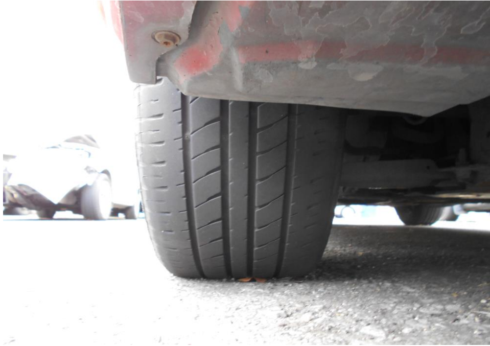
Photo 6 shows the condition of the front right tyre of the Motor Taxi, which was observed to be in serviceable condition with remaining tread depth of approximately 6mm. There was no tear, cut or burst mark(s) on the outer and the inner sidewalls.
