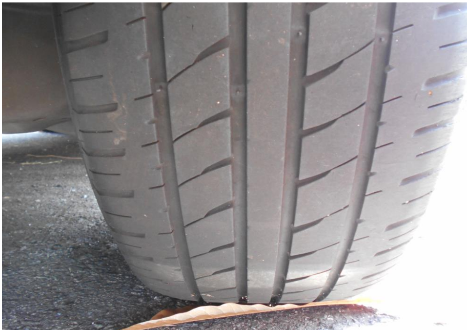
Photo 9 shows the condition of the rear right tyre of the Motor Taxi, which was observed to be in serviceable condition with remaining tread depth of approximately 6mm.
