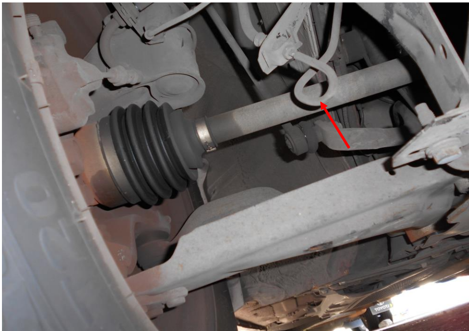
Photo 17 shows the various undercarriage components at the front right wheel of the Motor Taxi, in particular the steering tie rod (arrowed). The various steering components were all found to be intact, suggesting that the steering system of the Motor Taxi was likely to be in serviceable condition.
