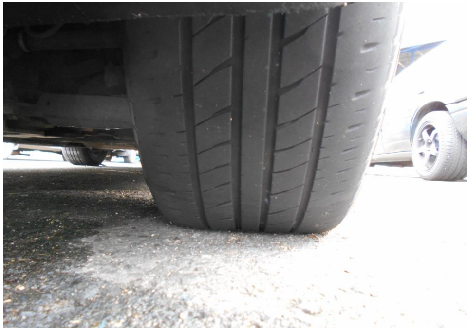
Photo 7 shows the condition of the front left tyre of the Motor Taxi, which was observed to be in serviceable condition with remaining tread depth of approximately 6mm. The tyre, which was wrapped around alloy wheel rim, was also observed to be sufficiently inflated for vehicular operation.
