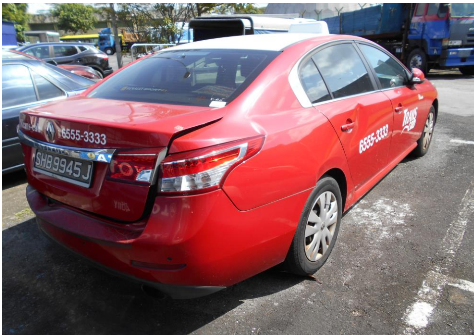
Photo 4 shows a general view of the rear right body of the Motor Taxi at the time of our inspection. The Motor Taxi was observed to have sustained with minor misalignment on the rear bonnet as a result of the accident.
