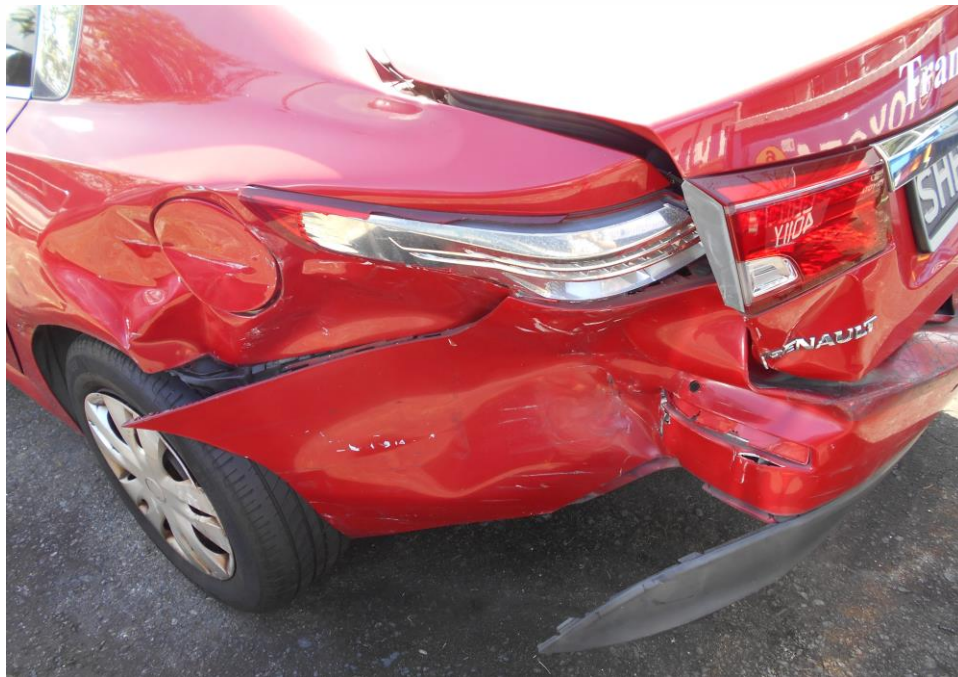
Photo 5 shows a close up view of the rear left of the Motor Taxi at the time of our inspection. The Motor Taxi had sustained extensive impact damages at the rear bumper as a result of the accident.
