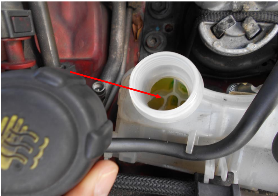
Photo 12 shows the engine coolant fluid reservoir of the Motor Taxi at the time of our inspection. The engine coolant fluid was observed to be of sufficient level and without any visible contamination.
