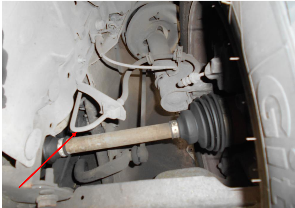
Photo 18 shows the various undercarriage components at the front left wheel of the Motor Taxi. We did not observe any leakage of brake fluid (arrowed) at the time of our inspection of the Motor Taxi. Our visual inspection of the various mechanical components of the Motor Taxi's braking system revealed all to be intact and without visible damage, indicating that the braking system was likely to be in serviceable condition at the material time of accident.
