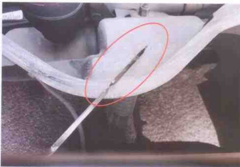
Photo 15 shows the engine dip stick of the Motor Lorry at the time of our inspection. The engine oil was observed to be of sufficient level and without any visible contamination (circled).
