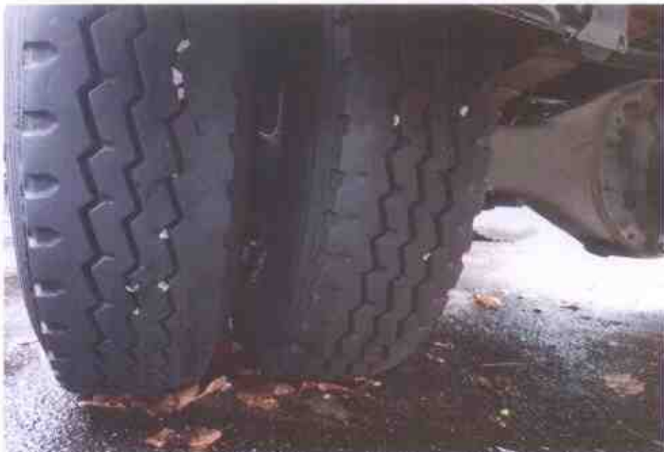
Photo 11 shows the condition of the rear right tyres of the Motor Lorry, which were observed to be in serviceable condition with remaining tread depth of approximately 9mm.
