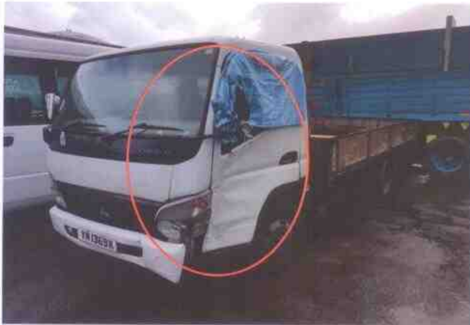
Photo 3 shows a general view of the front left portion of the Motor Lorry at the time of our inspection. The Motor Lorry was observed to have sustained minor impact damages at its front left portion which includes damages to the headlamp, lower bumper amongst others as a result of the accident.
