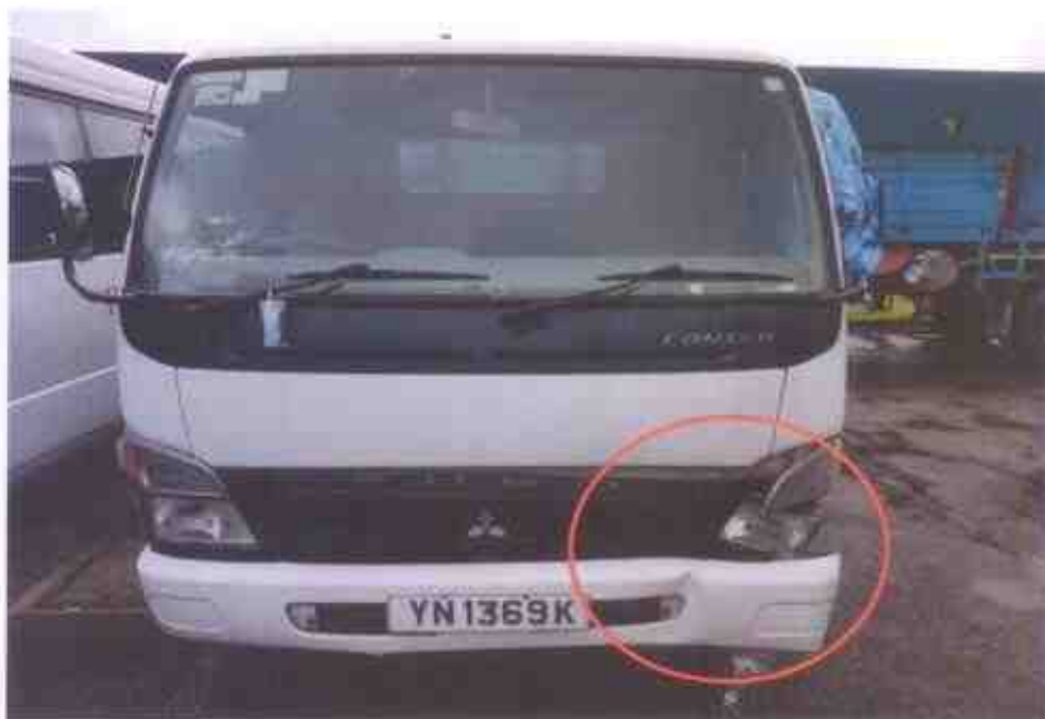
Photo 2 shows a general view of the front portion of the Motor Lorry at the time of our inspection. The Motor Lorry was observed to have sustained minor impact damages at its front left portion which includes damages to the headlamp, lower bumper amongst others as a result of the accident.
