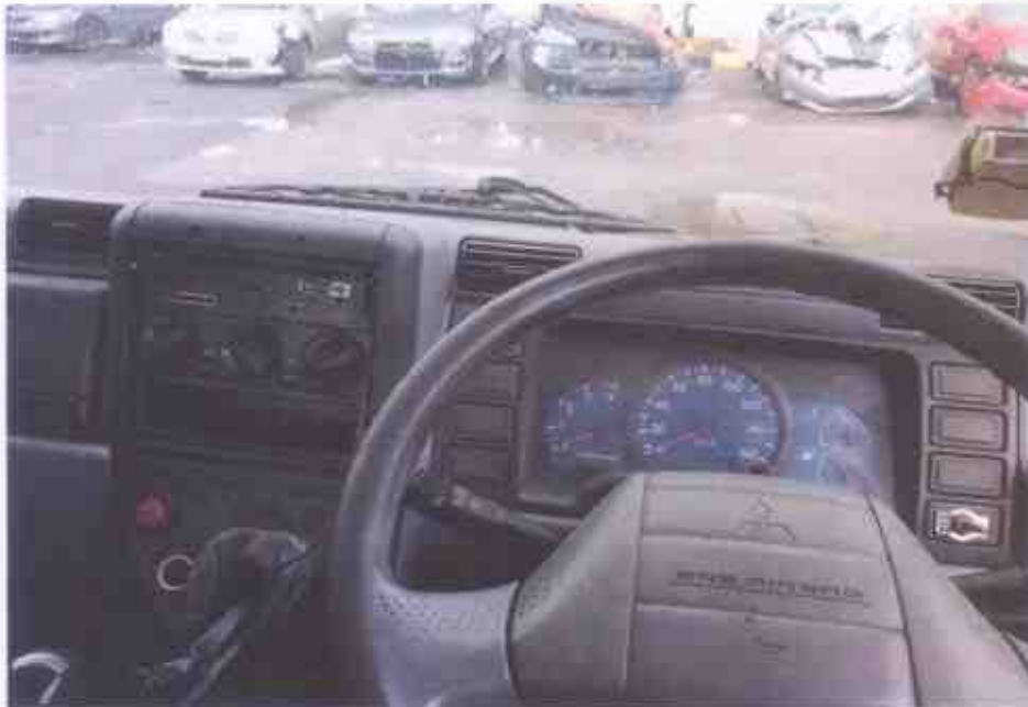
Photo 22 shows its various electronic operating systems like the Battery Check light, Parking Light and Supplemental Restraint System (SRS) during cranking of the engine had indicated that these systems were in working condition and without abnormality. This can be established from the warning lights disappearing from the instrument panel after the self-test.
