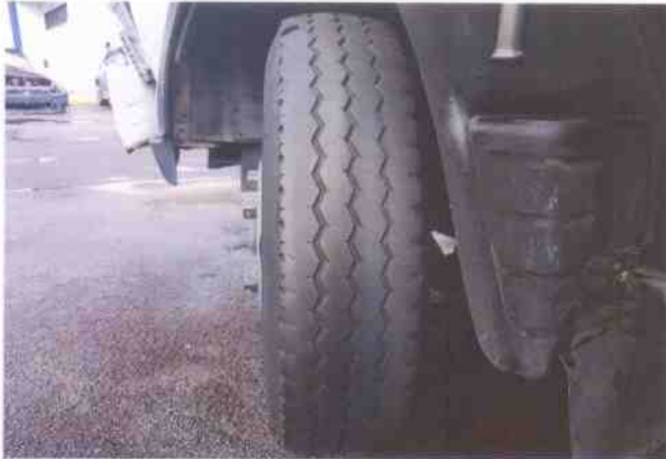
Photo 8 shows the condition of the front left tyre of the Motor Lorry, which was observed to be in serviceable condition with remaining tread depth of approximately 8mm. The tyre, which was wrapped around standard alloy wheel rim, was also observed to be sufficiently inflated for vehicular operation.
