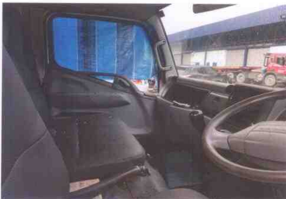
Photo 6 shows the close-up view from inside of the left passenger door window glass of the Motor Lorry. It was observed to be cracked, front dashboard was also found to be pushed inwards as a result of the accidents.
