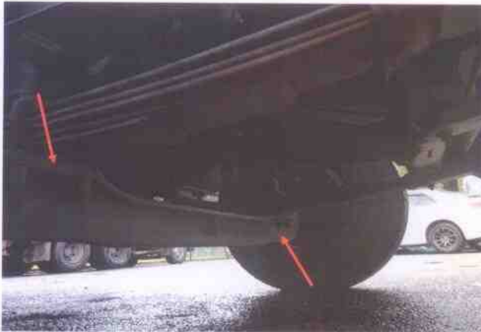
Photo 18 shows the various undercarriage components at the front right wheel of the Motor Lorry, in particular the steering rack (arrowed). The various undercarriage components of the Motor Lorry were all found to be intact without any visible damage. There was also no sign of fluid stain(s) observed on the various undercarriage components.
