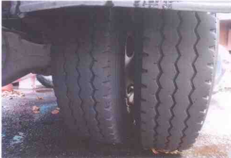
Photo 10 shows the condition of the rear left tyres of the Motor Lorry, which was observed to be in serviceable condition with remaining tread depth of approximately 7mm. The tyres, which were wrapped around standard alloy wheel rim, were also observed to be sufficiently inflated for vehicular operation.
