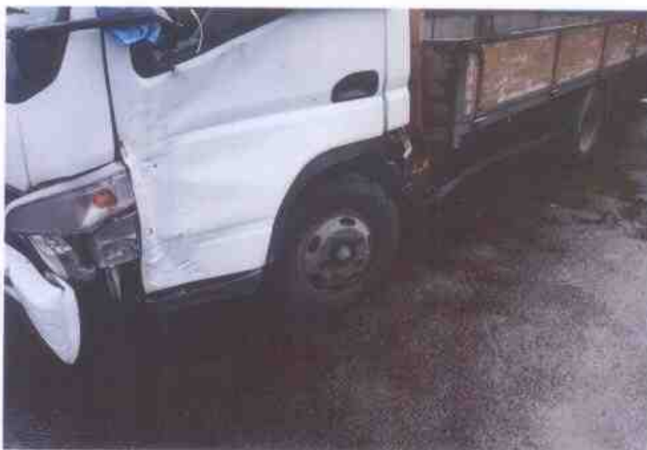
Photo 5 shows the left passenger door of the Motor Lorry. It was observed to be damage as a result of the accidents.
