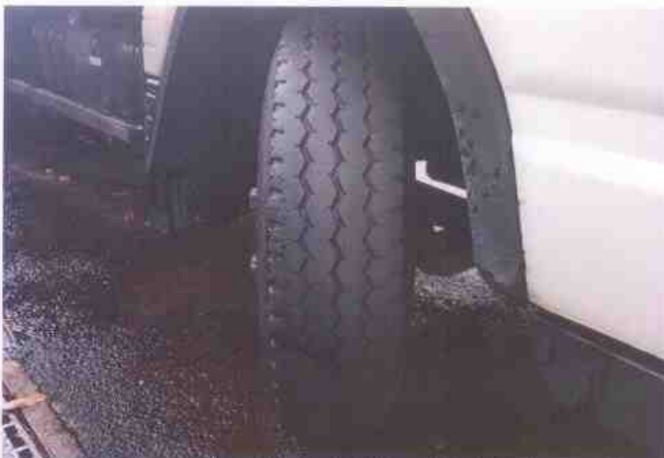
Photo 9 shows the condition of the front right tyre of the Motor Lorry, which was observed to be in serviceable condition with remaining tread depth of approximately 7mm. The tyre, which was wrapped around standard alloy wheel rim, was also observed to be sufficiently inflated for vehicular operation.
