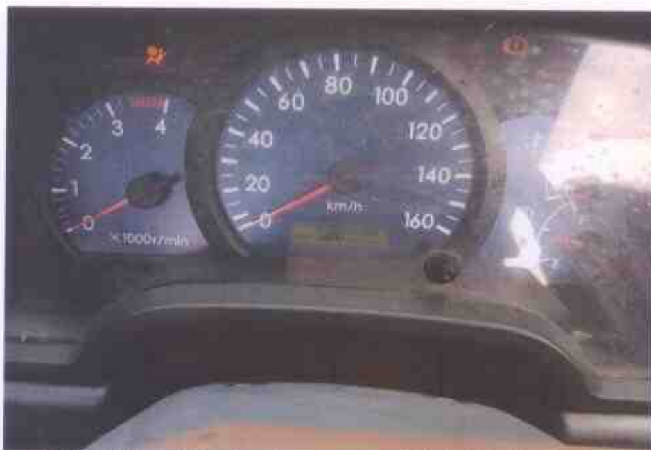
Photo 21 shows the Motor Lorry's automatic self-test of the functionality of its various electronic operating systems like the Battery Check light, Parking Light and Supplemental Restraint System (SRS) during cranking of the engine.
